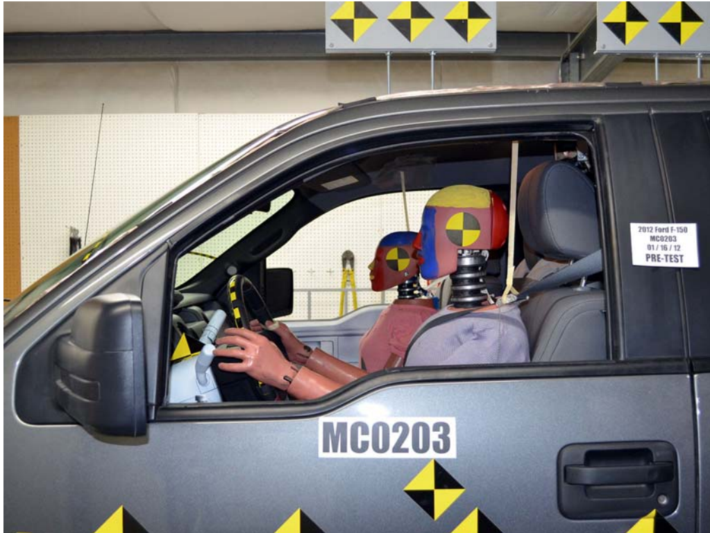
FIGURE 31. Pre-Test Driver Dummy Window View
