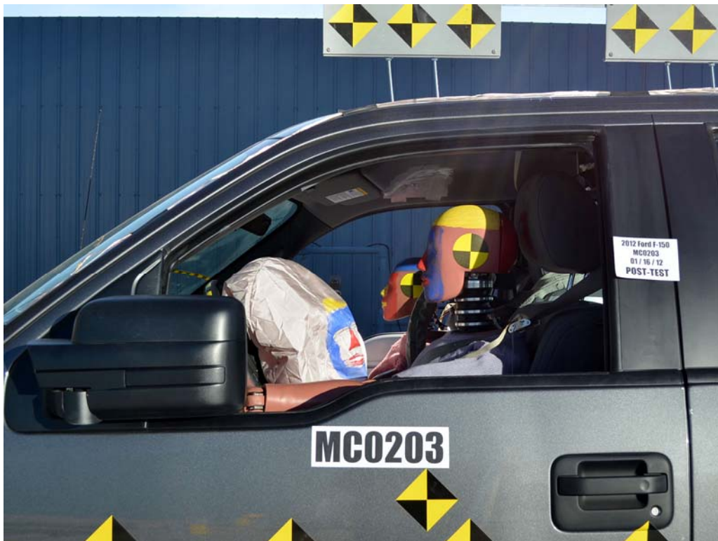
FIGURE 32. Post-Test Driver Dummy Window View
