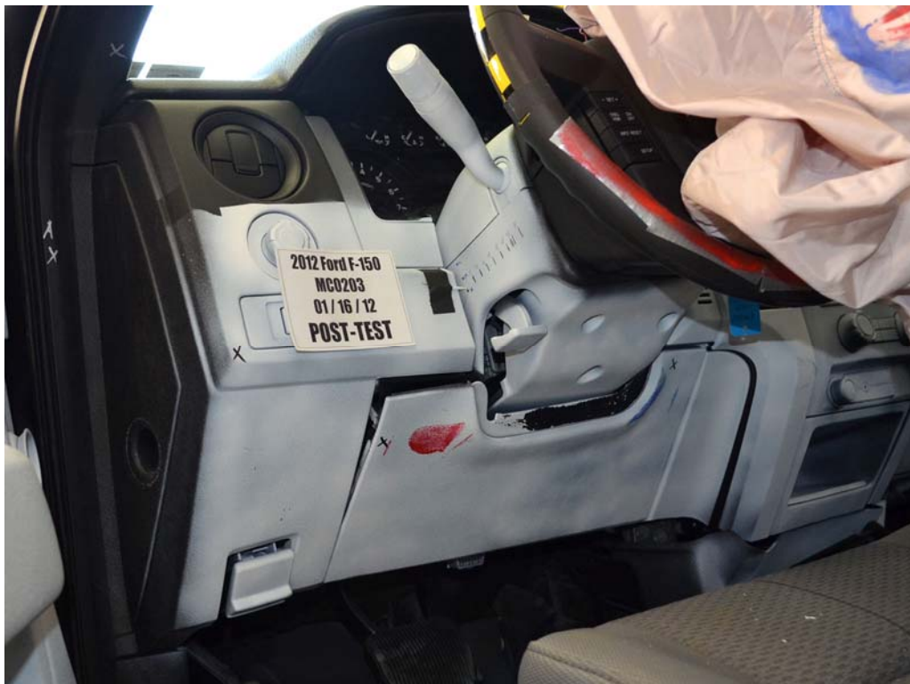
FIGURE 40. Post-Test Driver's Side Knee Bolster
