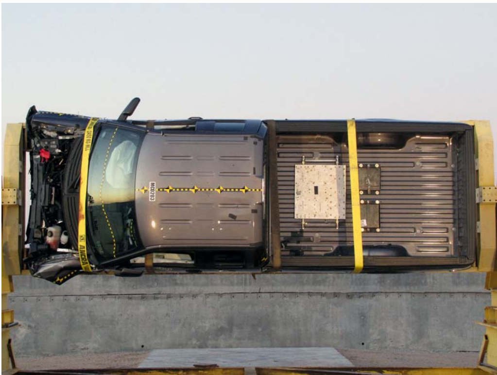
FIGURE 67. Vehicle at 90°on Static Rollover Device
