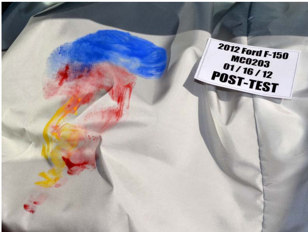
FIGURE 62. Post-Test Passenger Dummy Contact With Airbag
