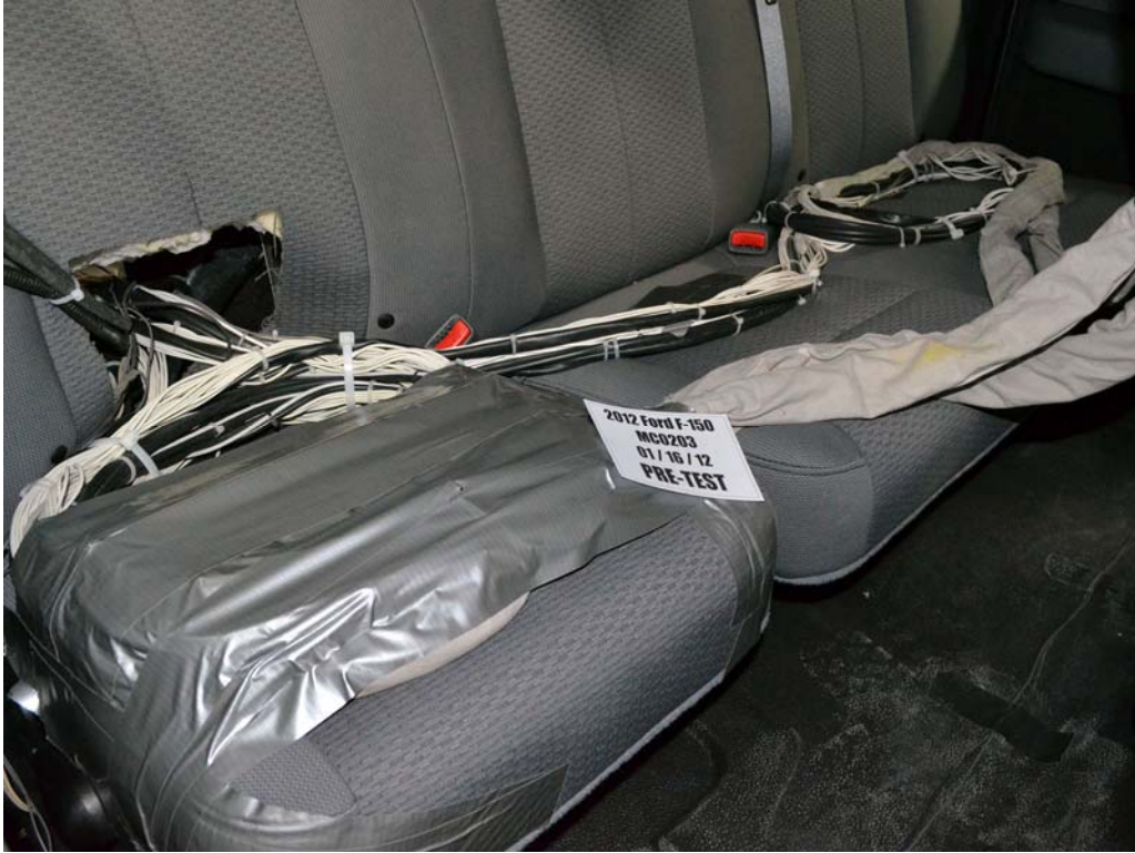
FIGURE 27. Pre-Test Dummy Cable Routing
