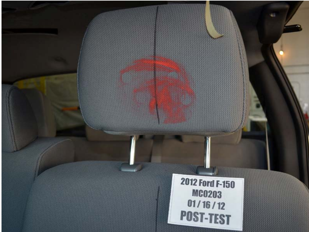
FIGURE 45. Post-Test Driver Dummy Contact With Headrest
