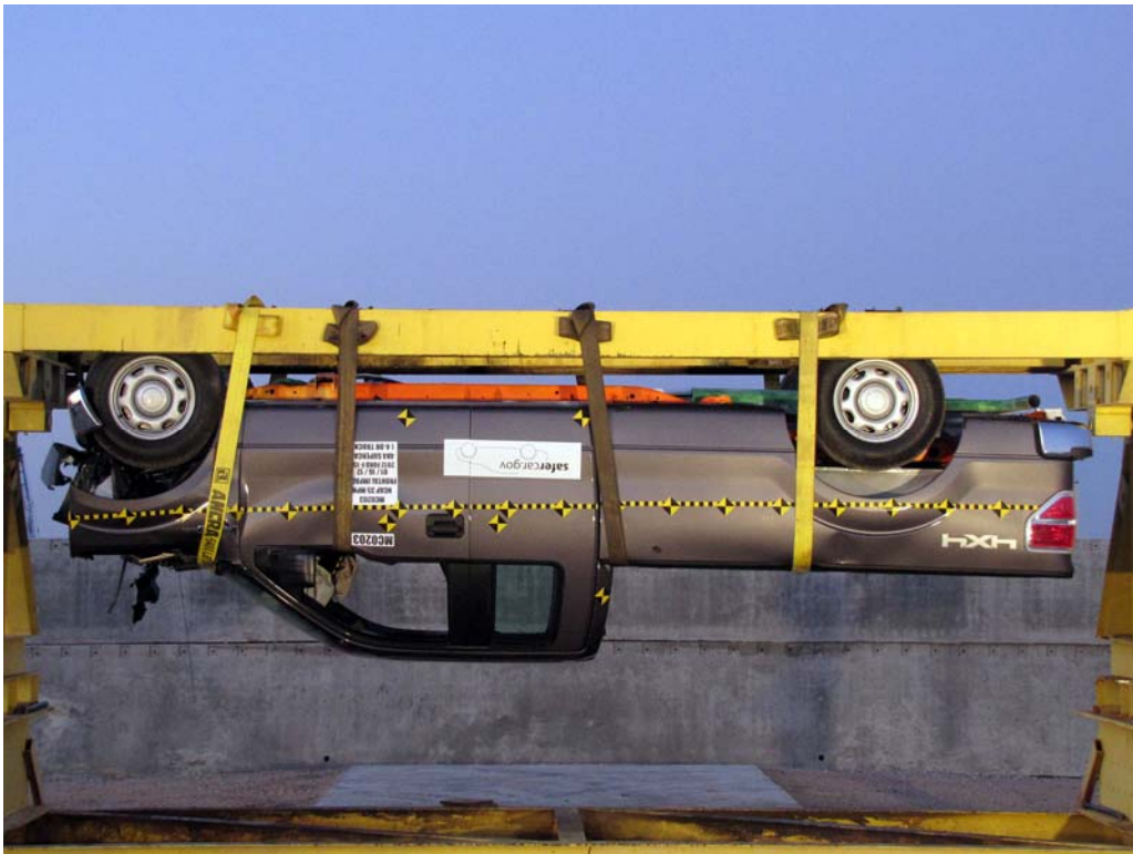
FIGURE 68. Vehicle at 180°on Static Rollover Device
