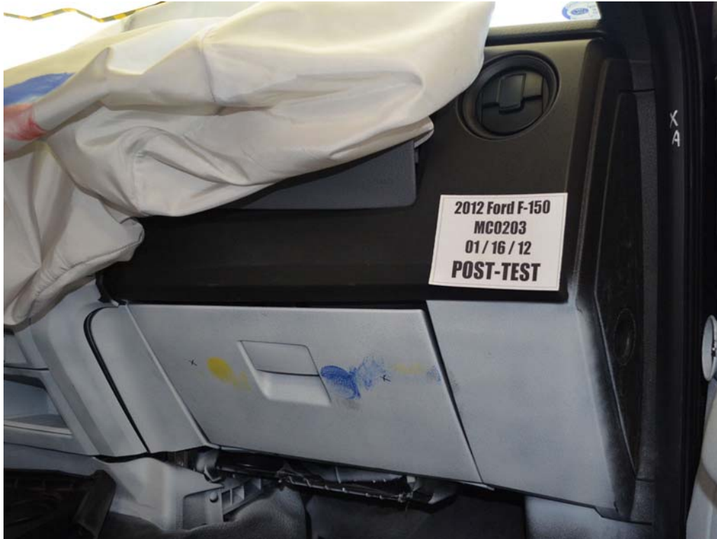
FIGURE 59. Post-Test Passenger's Side Knee Bolster
