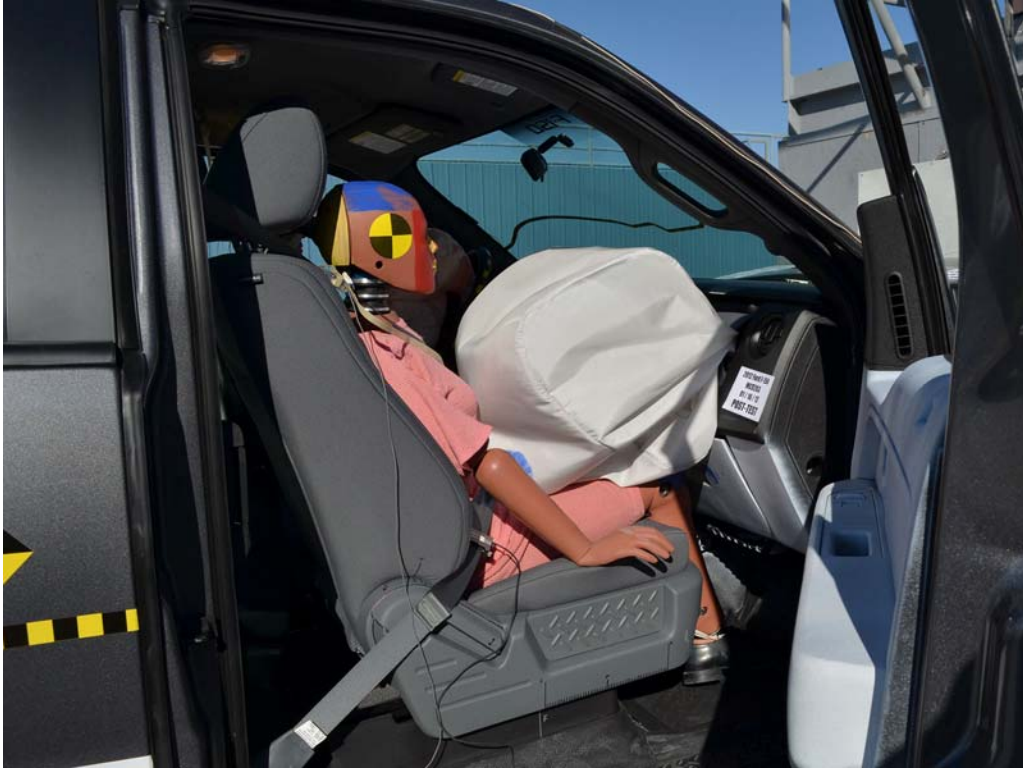
FIGURE 53. Post-Test Passenger Dummy and Vehicle Interior View
