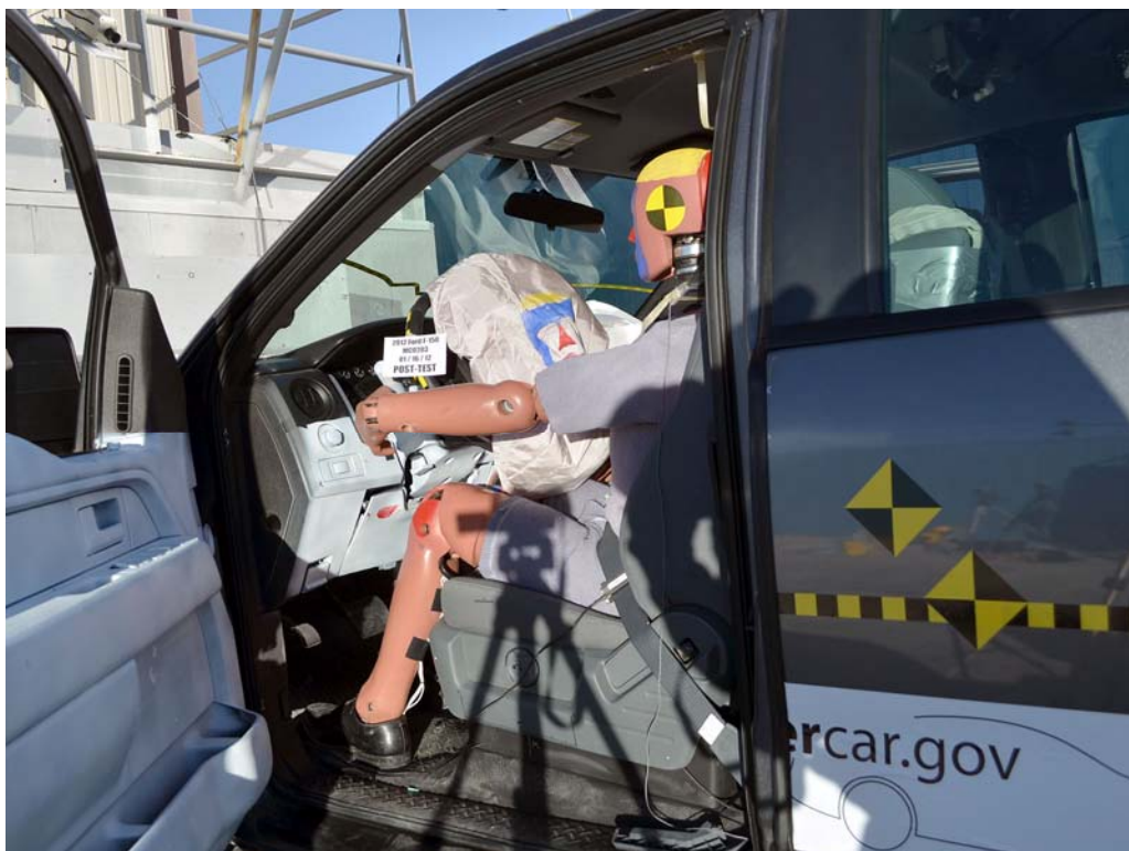
FIGURE 34. Post-Test Driver Dummy and Vehicle Interior View
