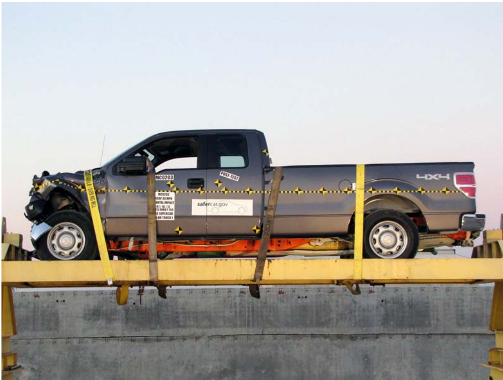
FIGURE 66. Vehicle at 0°on Static Rollover Device
