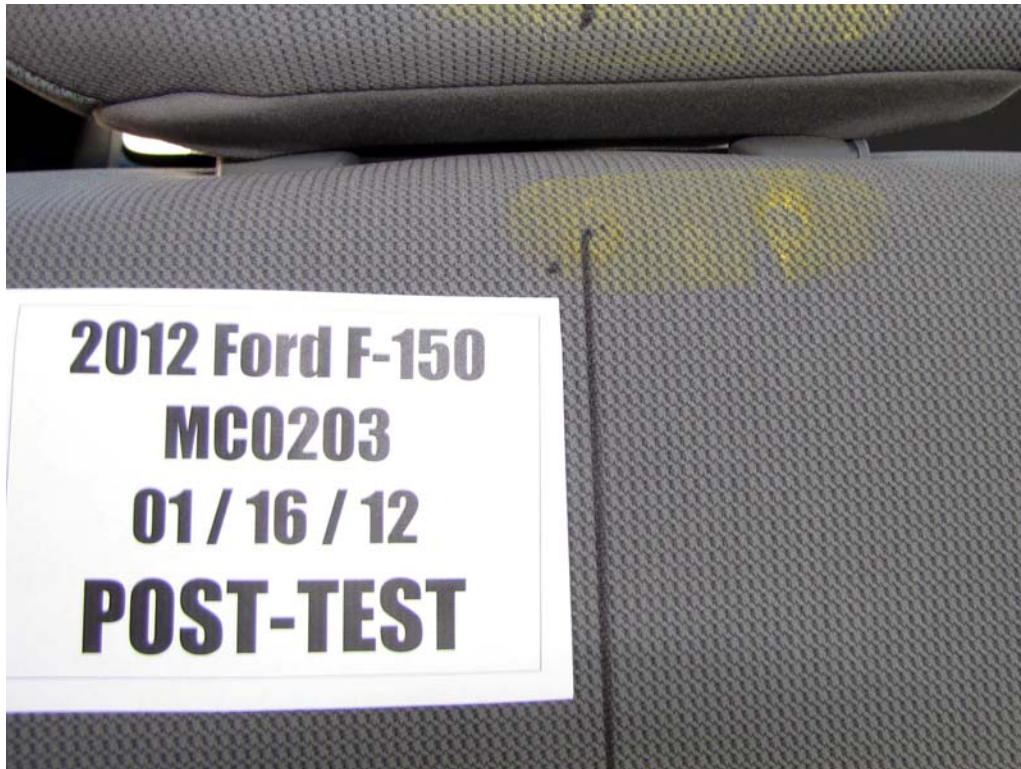
FIGURE 62c. Post-Test Passenger Dummy Contact With Seat Back
