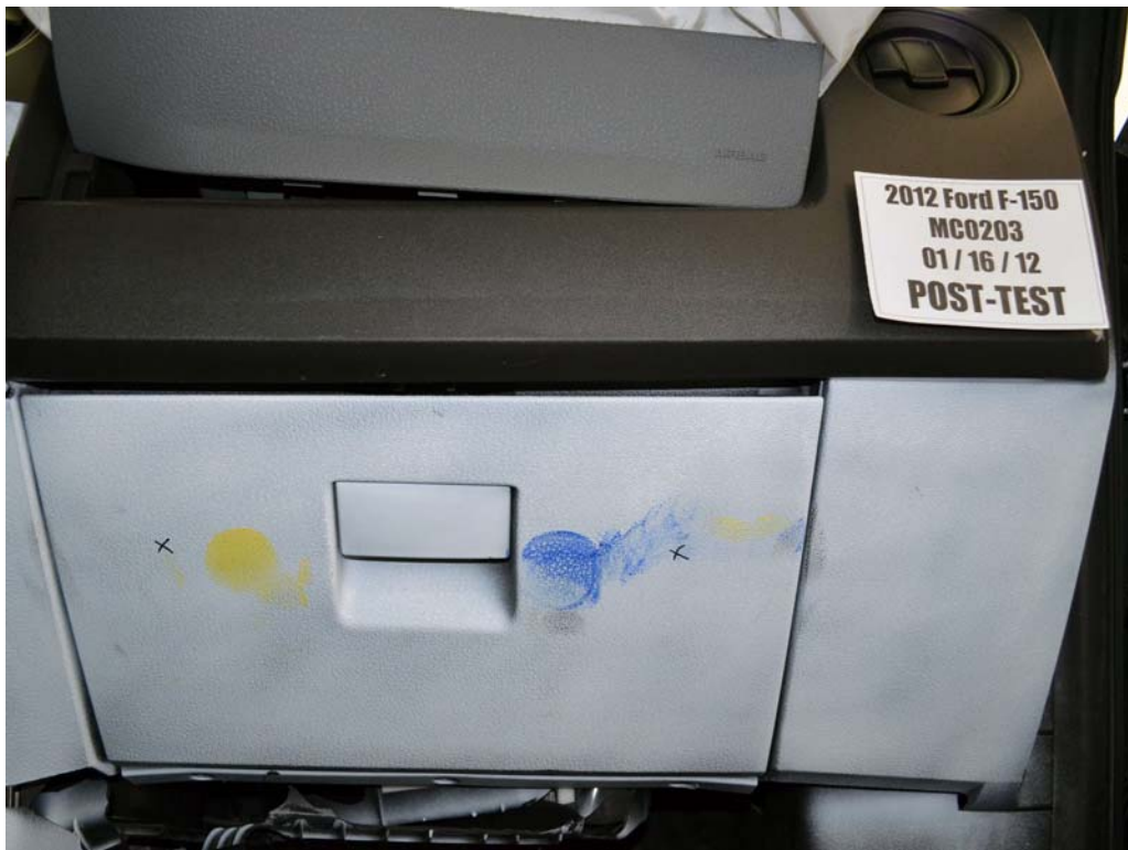
FIGURE 62b. Post-Test Passenger Dummy Contact With Glovebox
