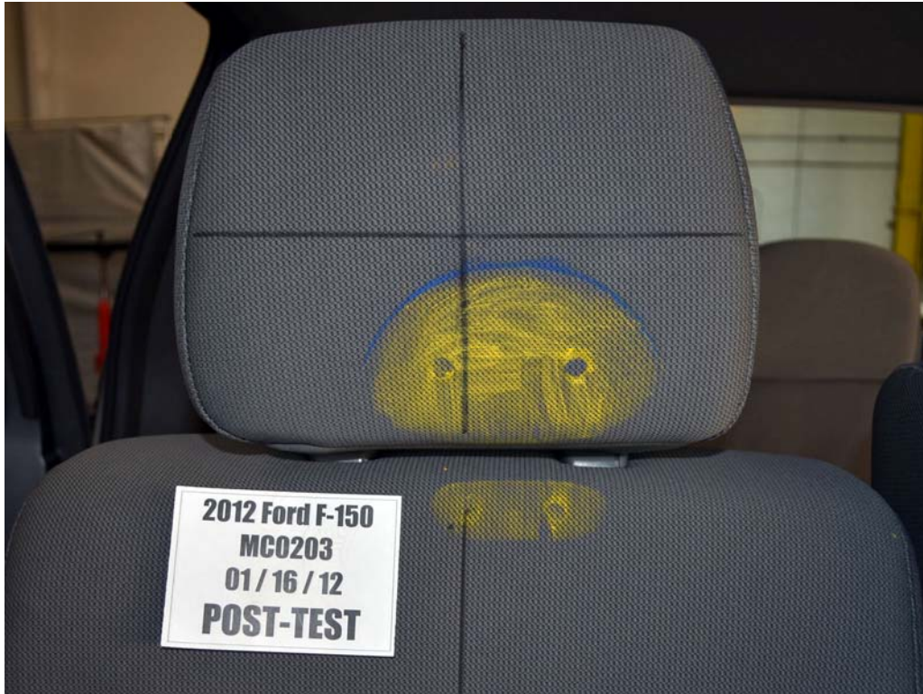
FIGURE 62a. Post-Test Passenger Dummy Contact With Headrest
