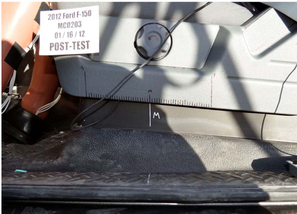
FIGURE 36. Post-Test Driver's Seat Fore-Aft Markings
