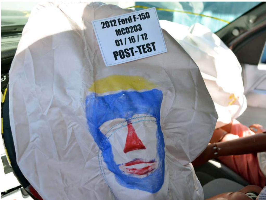
FIGURE 44. Post-Test Driver Dummy Contact With Airbag
