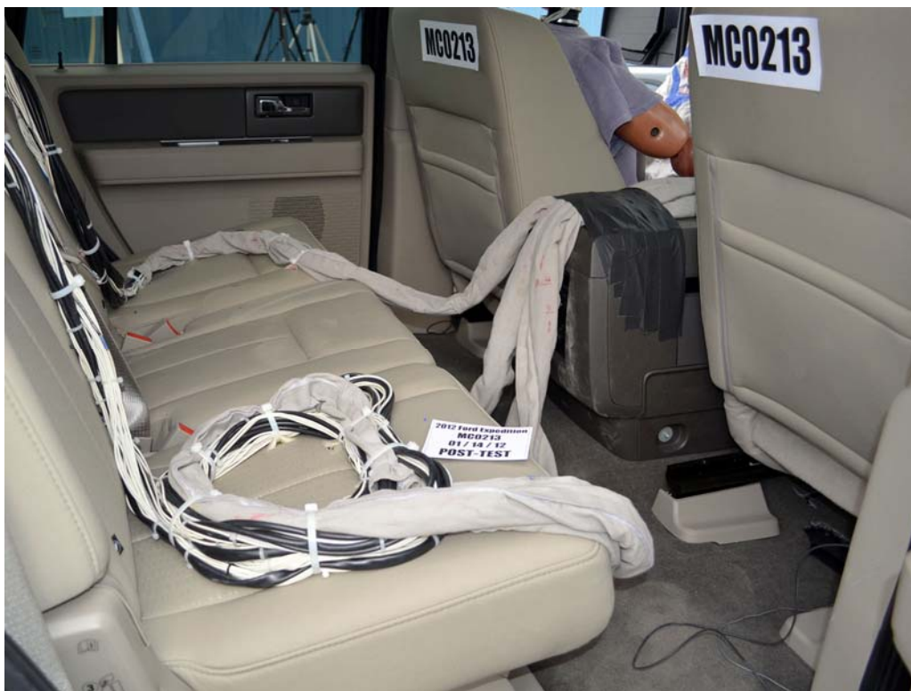
FIGURE 28. Post-Test Dummy Cable Routing
