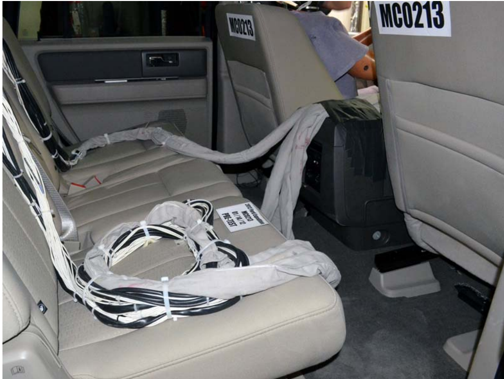
FIGURE 27. Pre-Test Dummy Cable Routing
