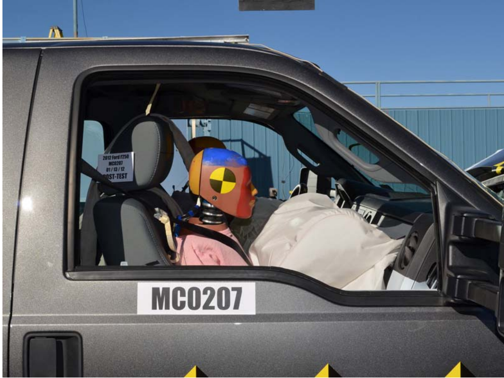
FIGURE 51. Post-Test Passenger Dummy Window View
