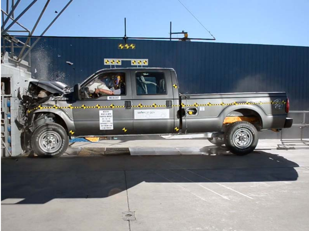
FIGURE 71. 2012 Ford Super Duty F-250 Frontal Impact Event
