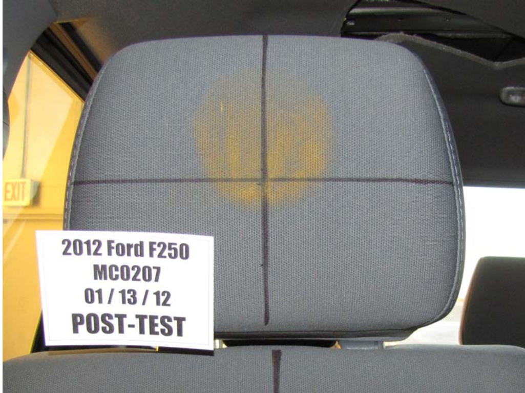
FIGURE 62a. Post-Test Passenger Dummy Contact With Headrest
