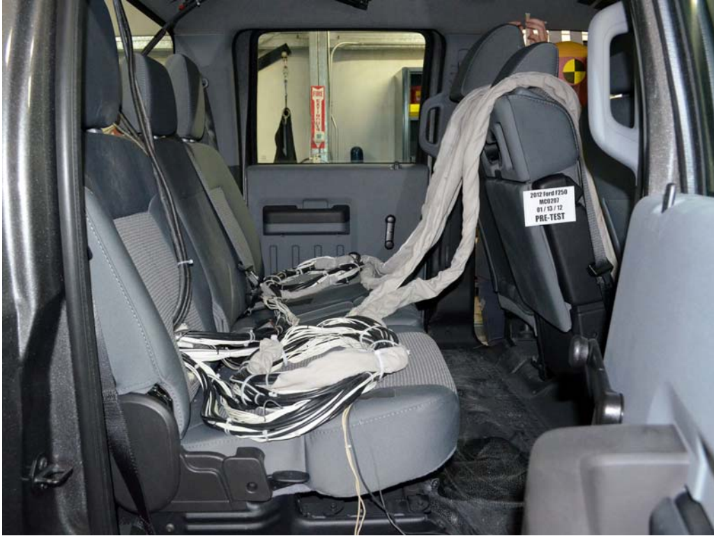
FIGURE 27. Pre-Test Dummy Cable Routing
