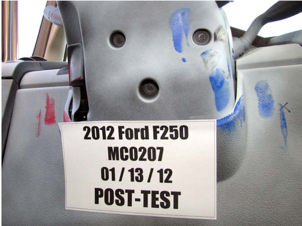
FIGURE 45b. Post-Test Driver Dummy Contact Steering Column
