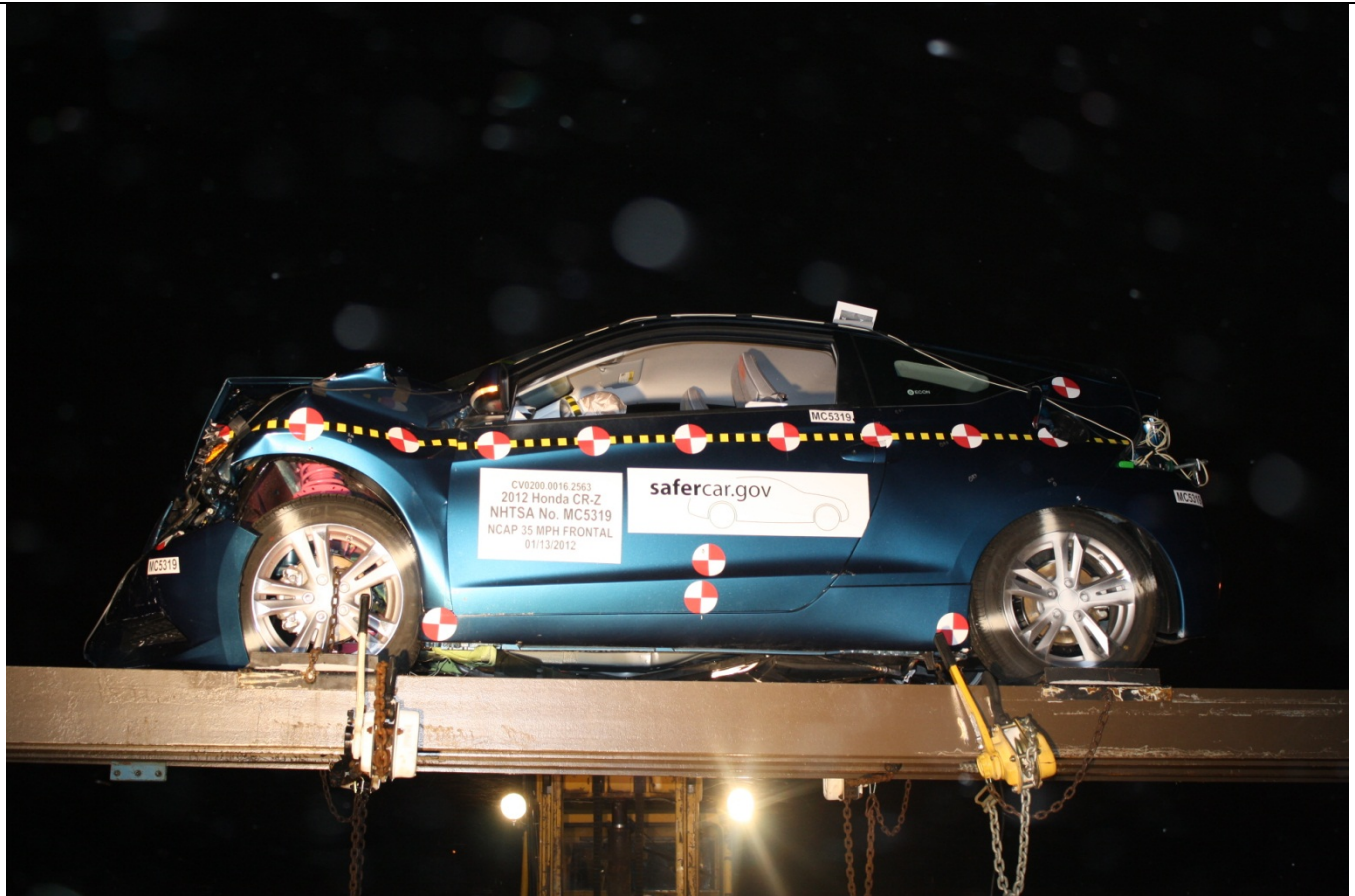
Figure A-31: FMVSS No. 305 Static Rollover at 360°
