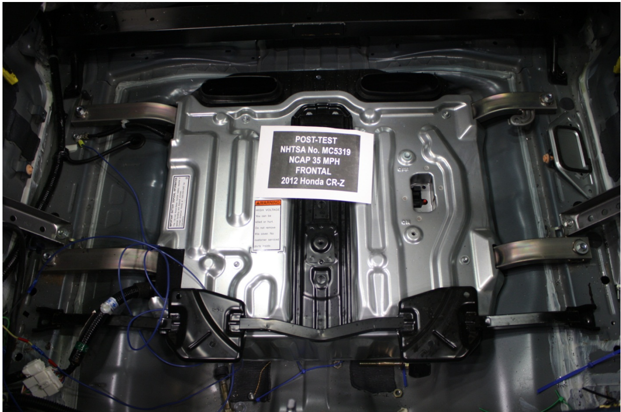
Figure A-15: Post-Impact View of Propulsion Battery Module(s)
