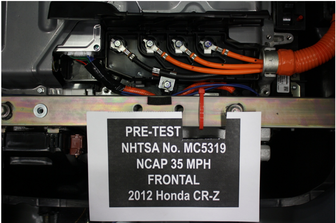
Figure A-23: Pre-Impact Close-Up View of High Voltage Leads Attached
