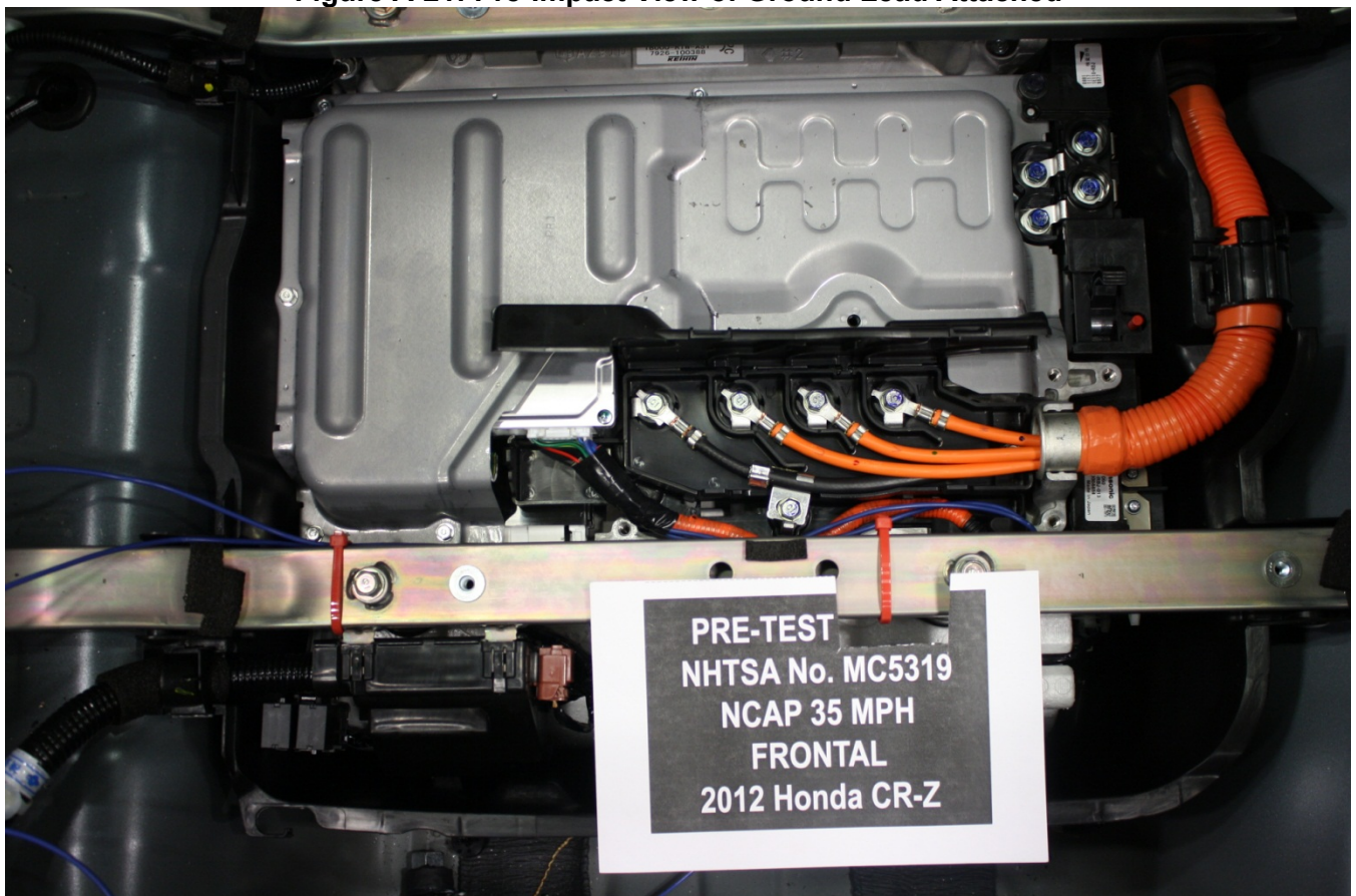
Figure A-22: Pre-Impact View of High Voltage Leads Attached
