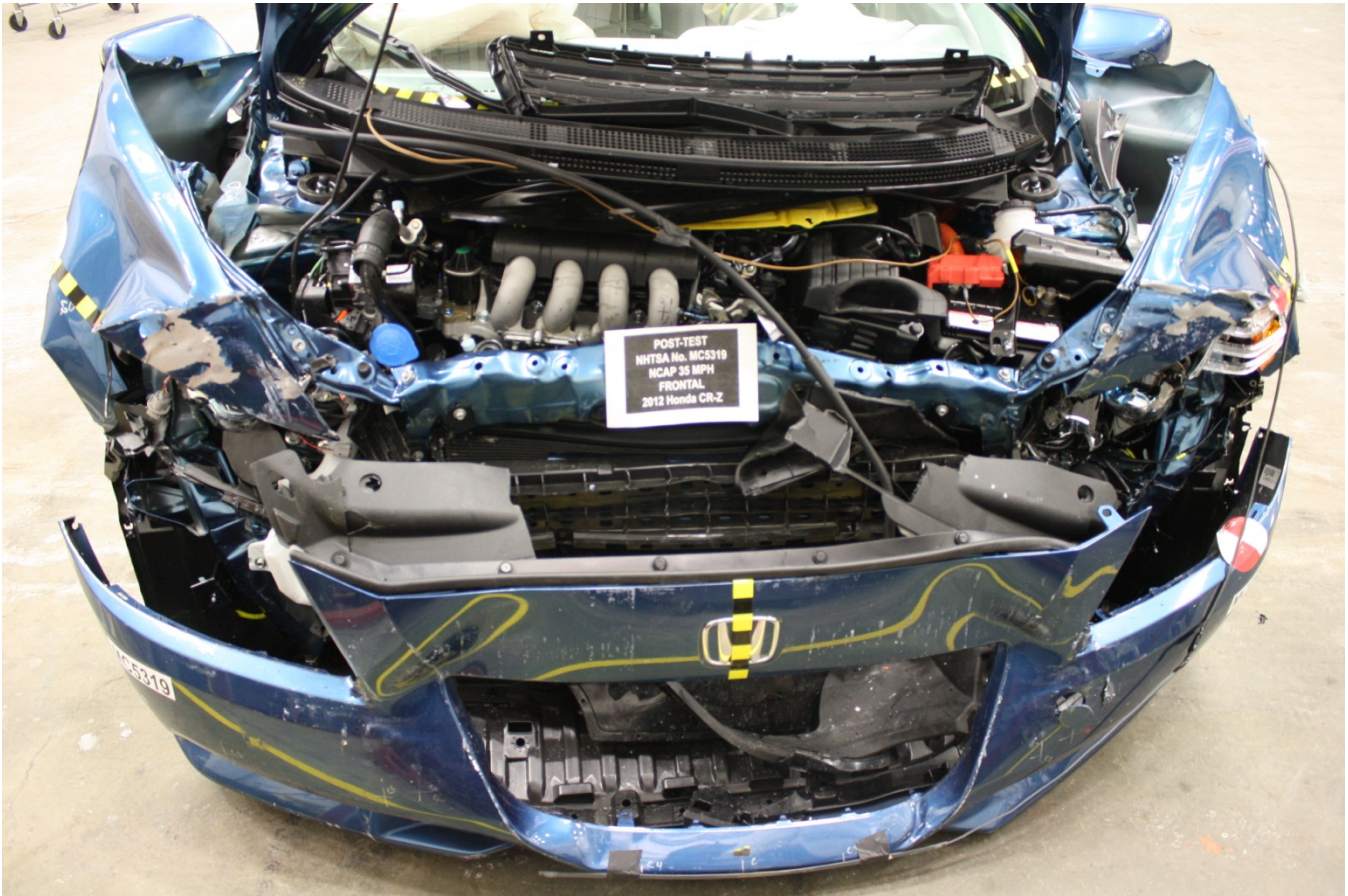
Figure A-17: Post-Impact View of Electric Propulsion Drive
