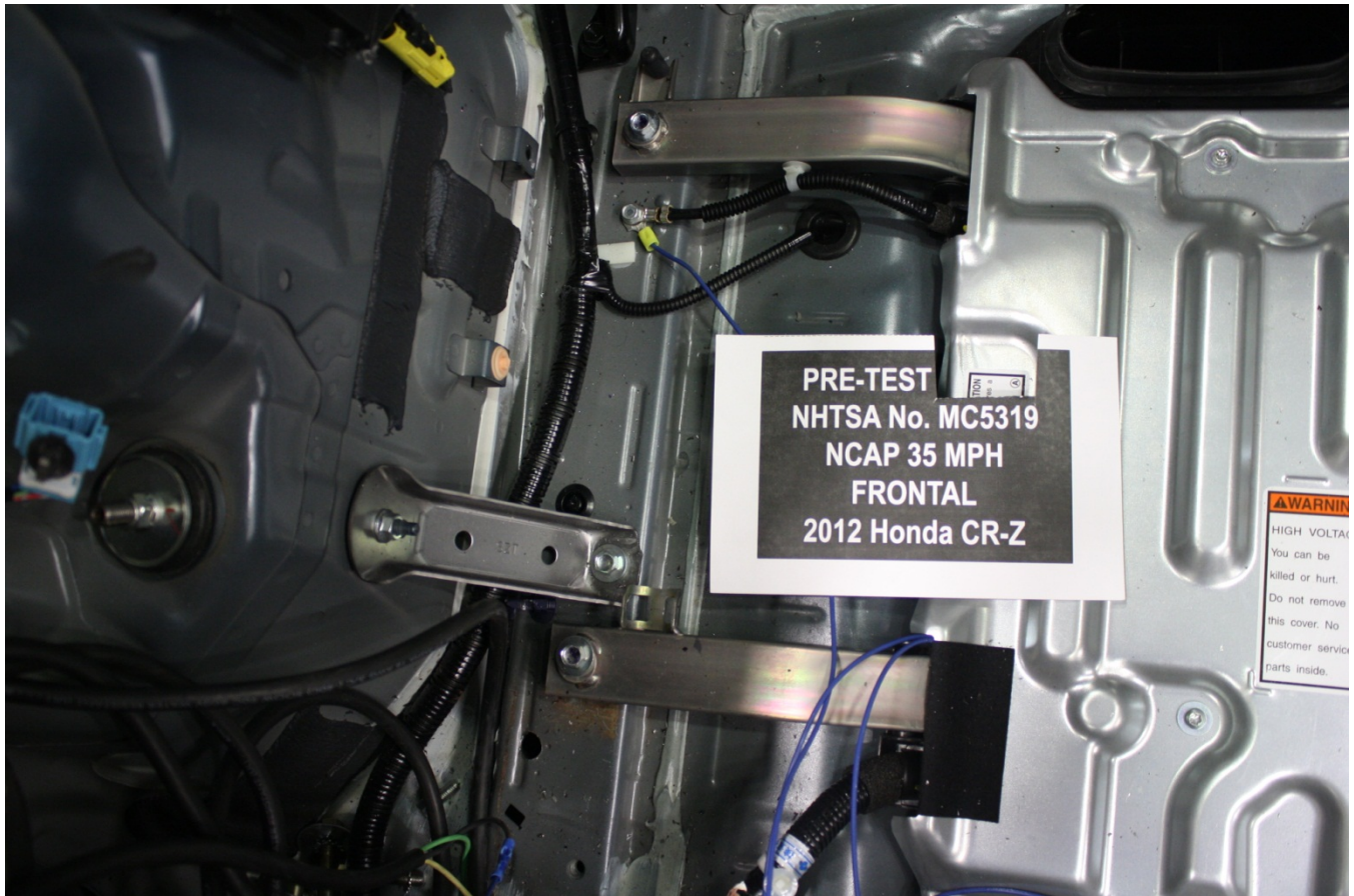
Figure A-21: Pre-Impact View of Ground Lead Attached
