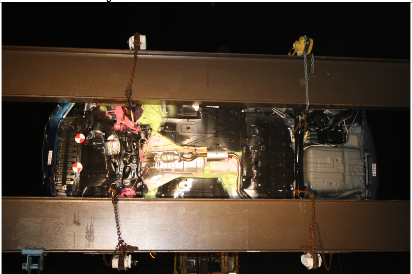
Figure A-30: FMVSS No. 305 Static Rollover at 270°
