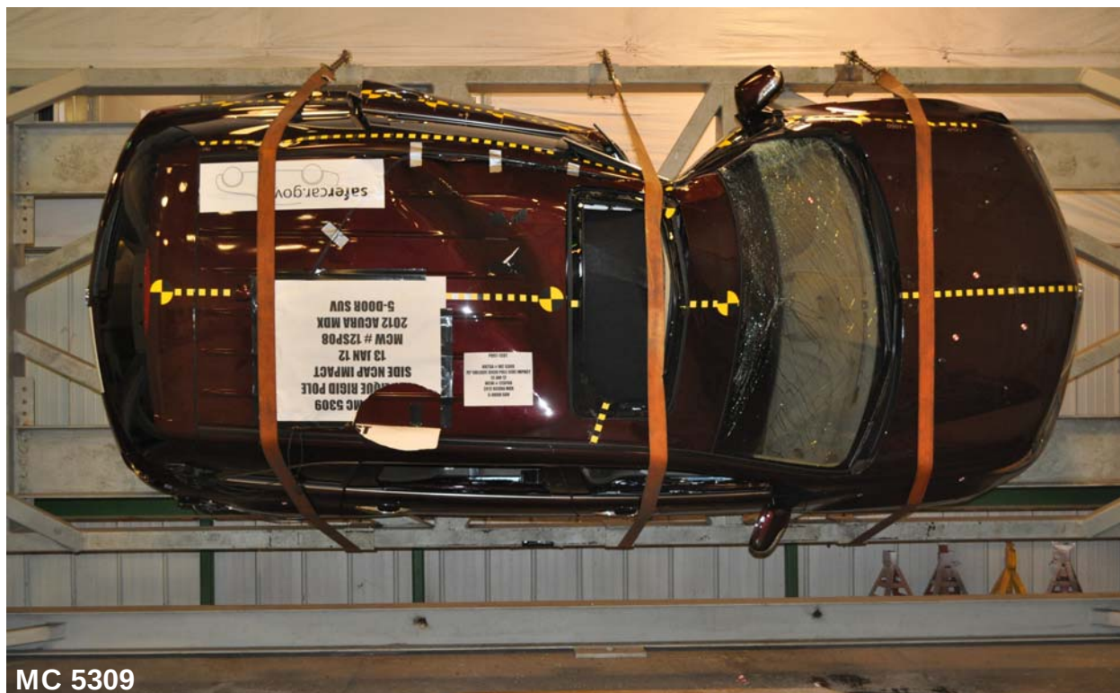
Figure 065: FMVSS No. 301 Static Rollover 270 Degrees
