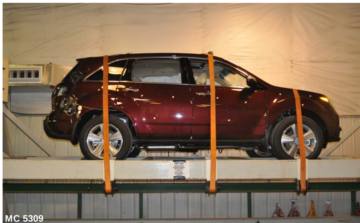
Figure 062: FMVSS No. 301 Static Rollover 0 Degrees
