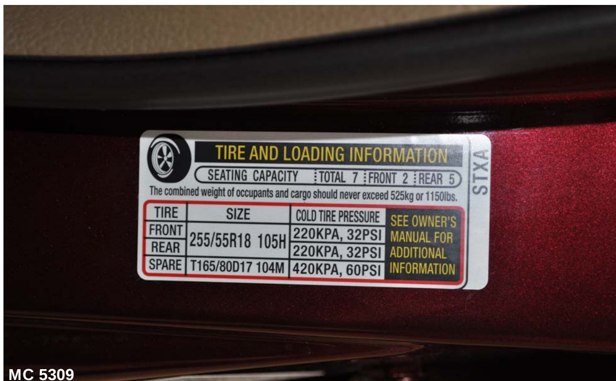
Figure 055: Close-Up View of Vehicle's Tire Information Placard or Label
