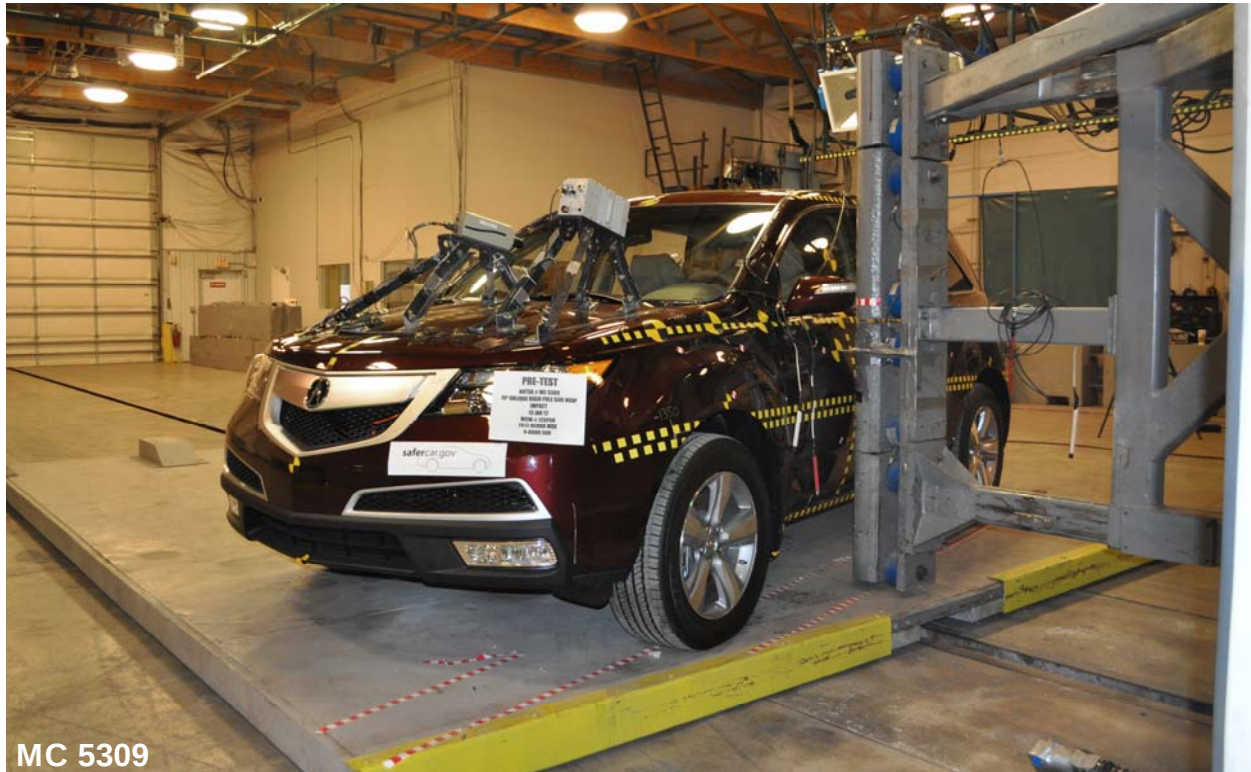
Figure 017: Pre-Test Left Side View of Pole Positioned Against Side of Vehicle
