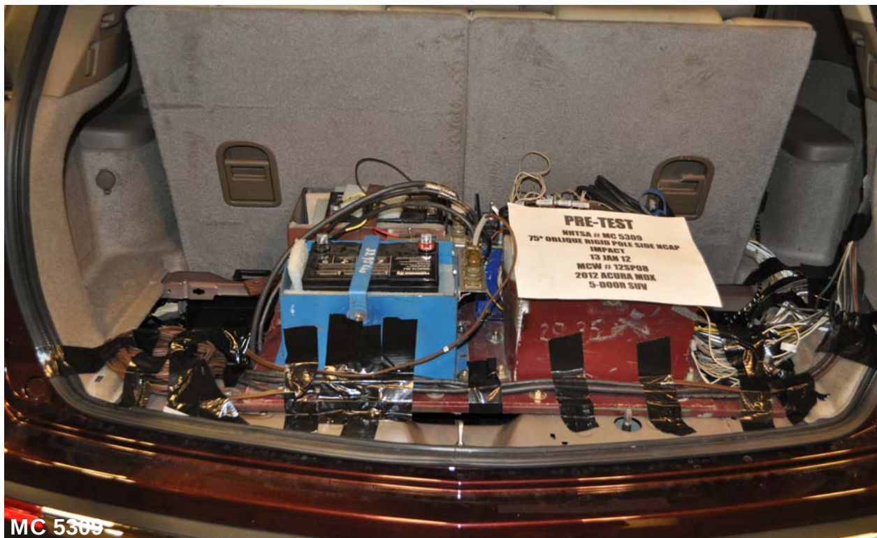
Figure 060: Pre-Test Ballast View
