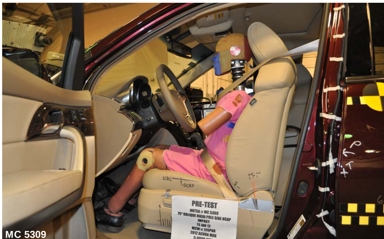
Figure 023: Pre-Test Left Side View of Dummy Showing Belt and Chalking
