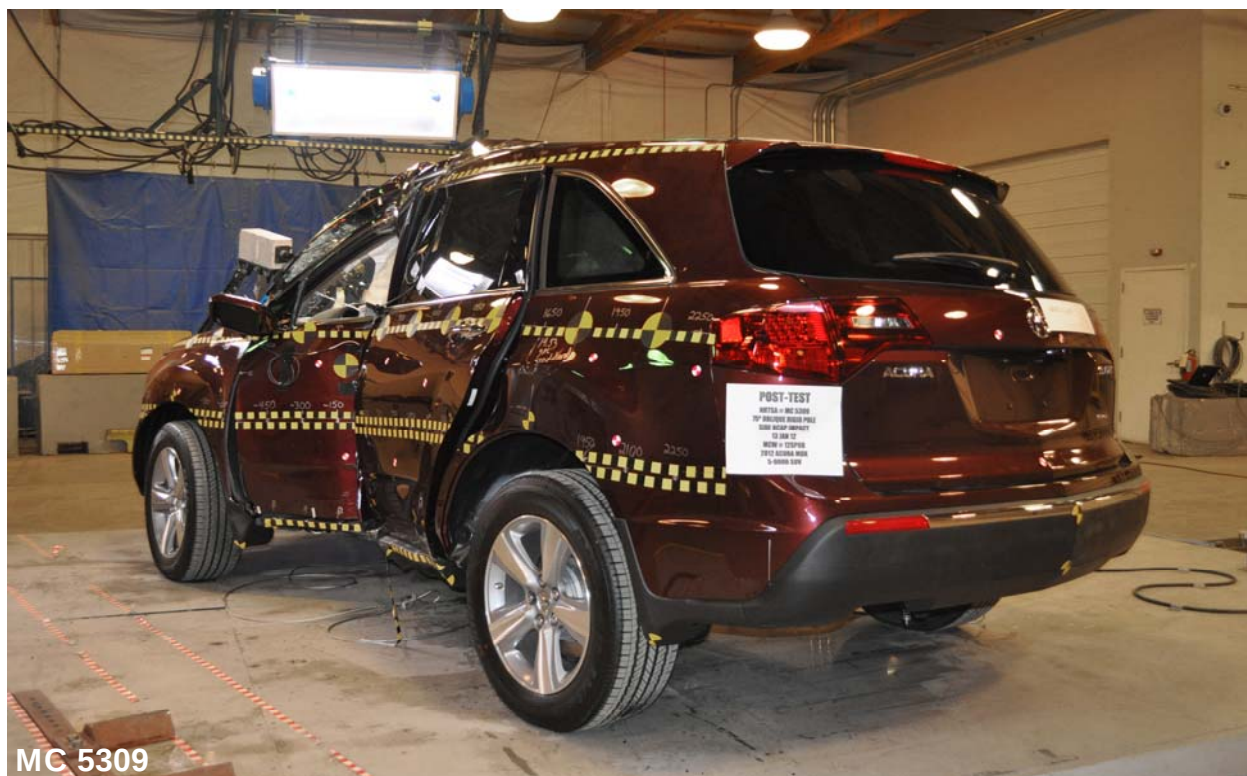
Figure 010: Post-Test Left Rear 3-4 View of Test Vehicle
