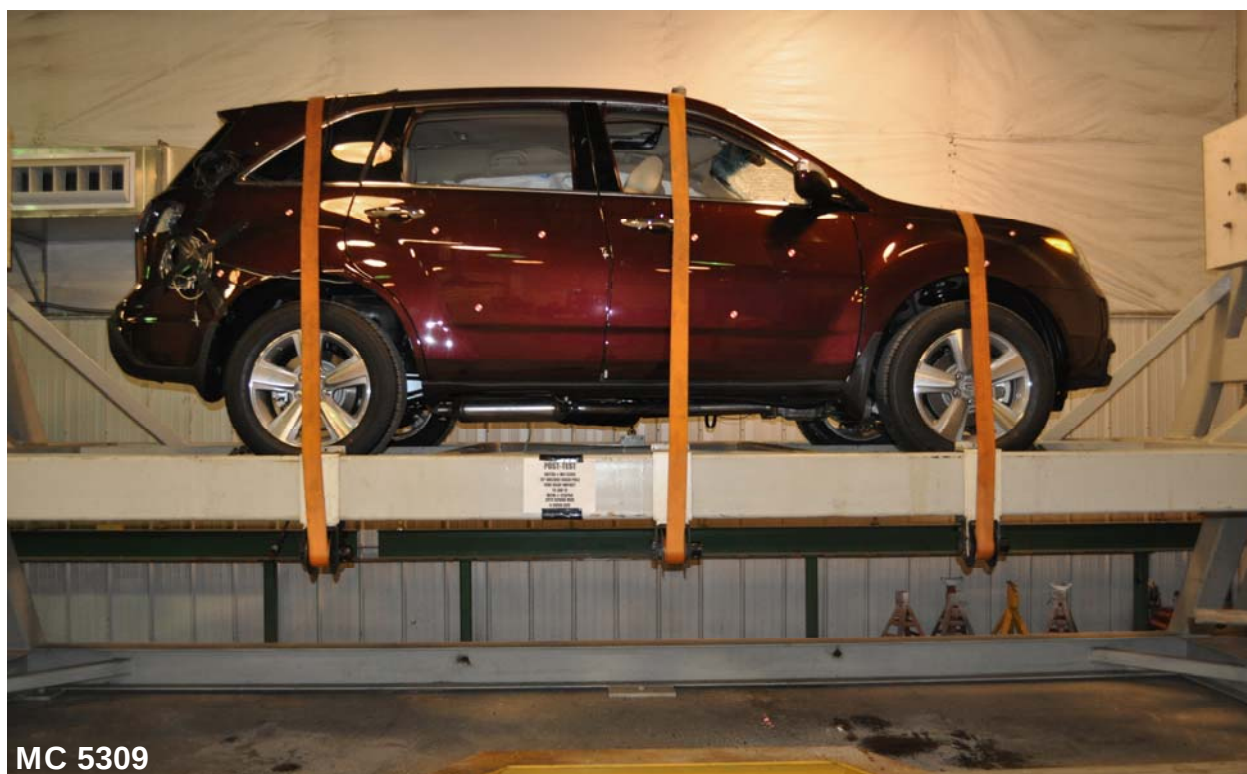
Figure 066: No. 066 FMVSS No. 301 Static Rollover 360 Degrees
