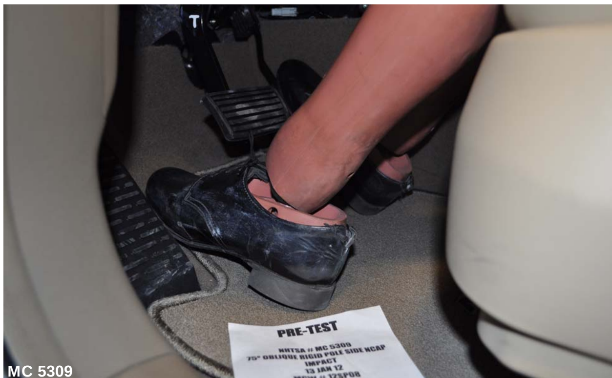
Figure 032: Pre-Test Placement of Dummy's Feet
