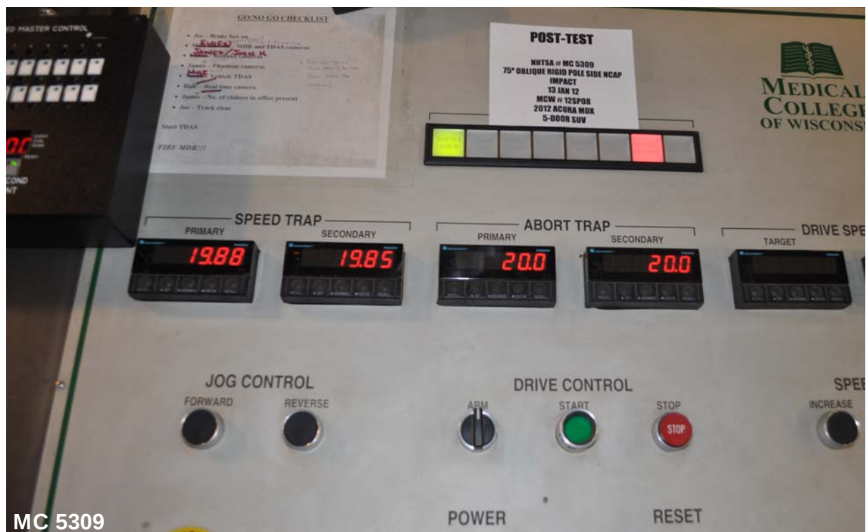
Figure 061: Post-Test Primary and Redundant Speed Trap Read-Out
