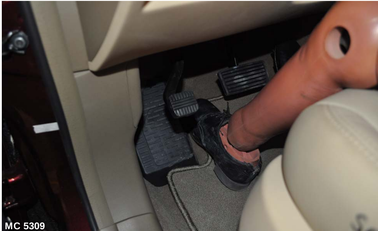
Figure 035: Pre-Test View of Disengaged Parking Brake
