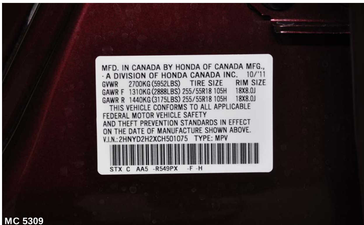
Figure 054: Close-Up View of Vehicle's Certification Label
