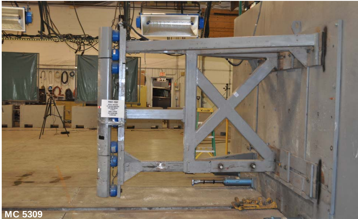
Figure 059: Post-Test Pole Barrier Side View
