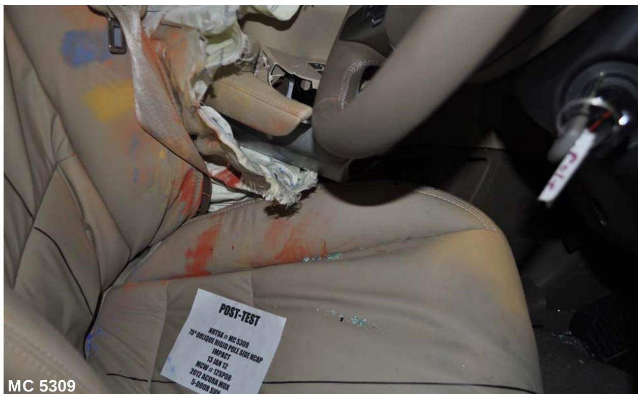
Figure 050: Post-Test Dummy Close-Up Pelvis Contact with Vehicle Interior View - N/a
