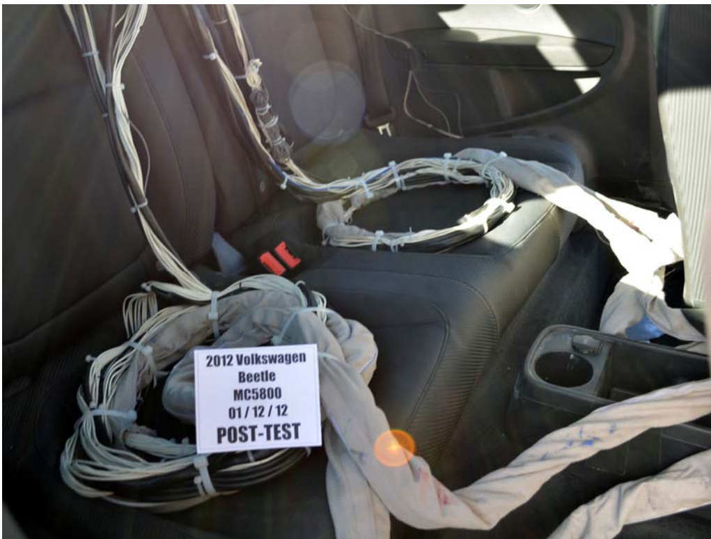
FIGURE 28. Post-Test Dummy Cable Routing
