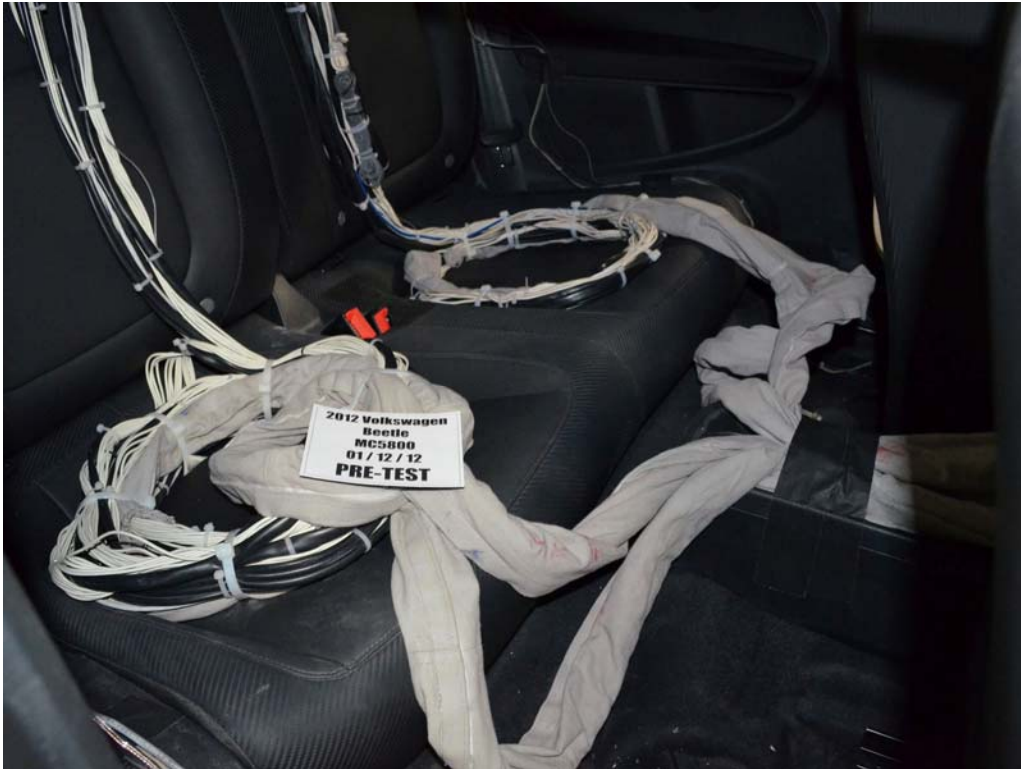
FIGURE 27. Pre-Test Dummy Cable Routing
