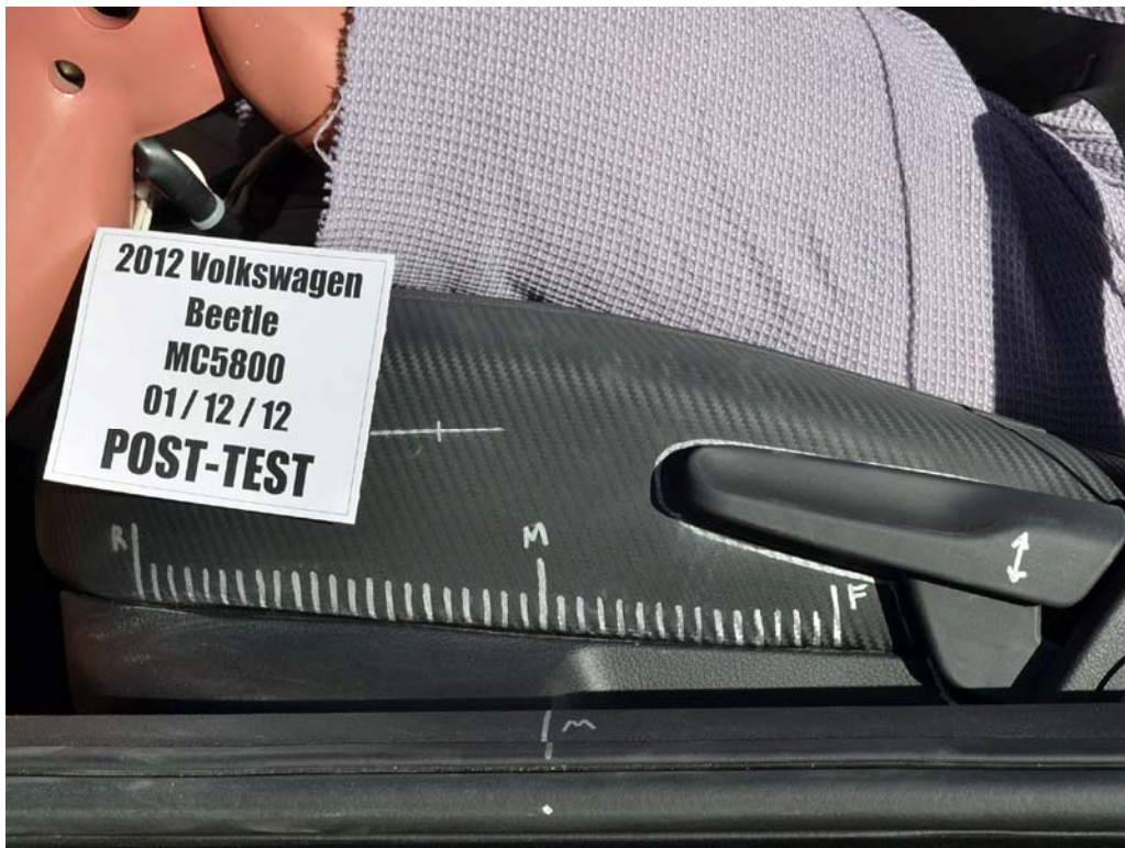
FIGURE 36. Post-Test Driver's Seat Fore-Aft Markings
