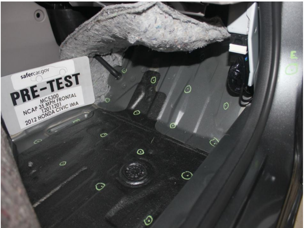
Pre-Test Passenger's Side Floorpan
