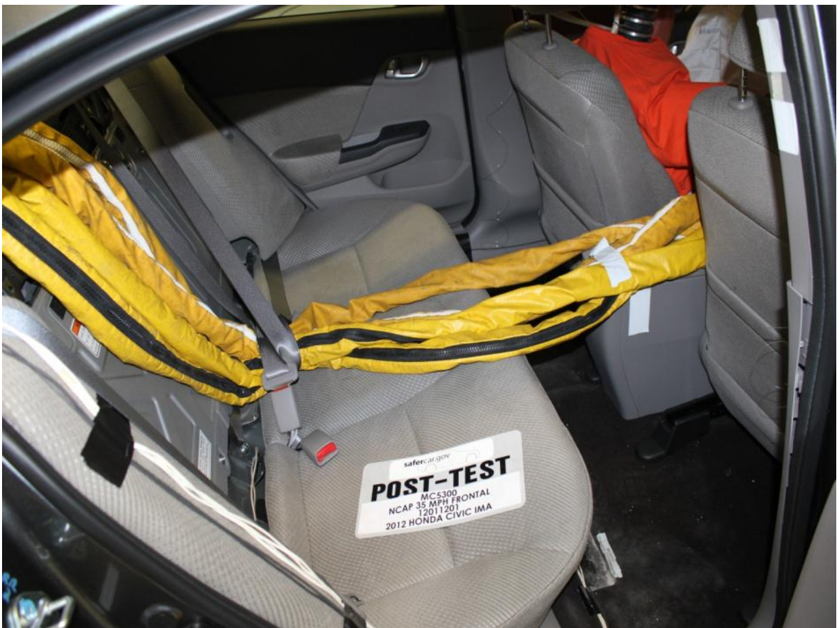
Post-Test Dummy Cable Routing
