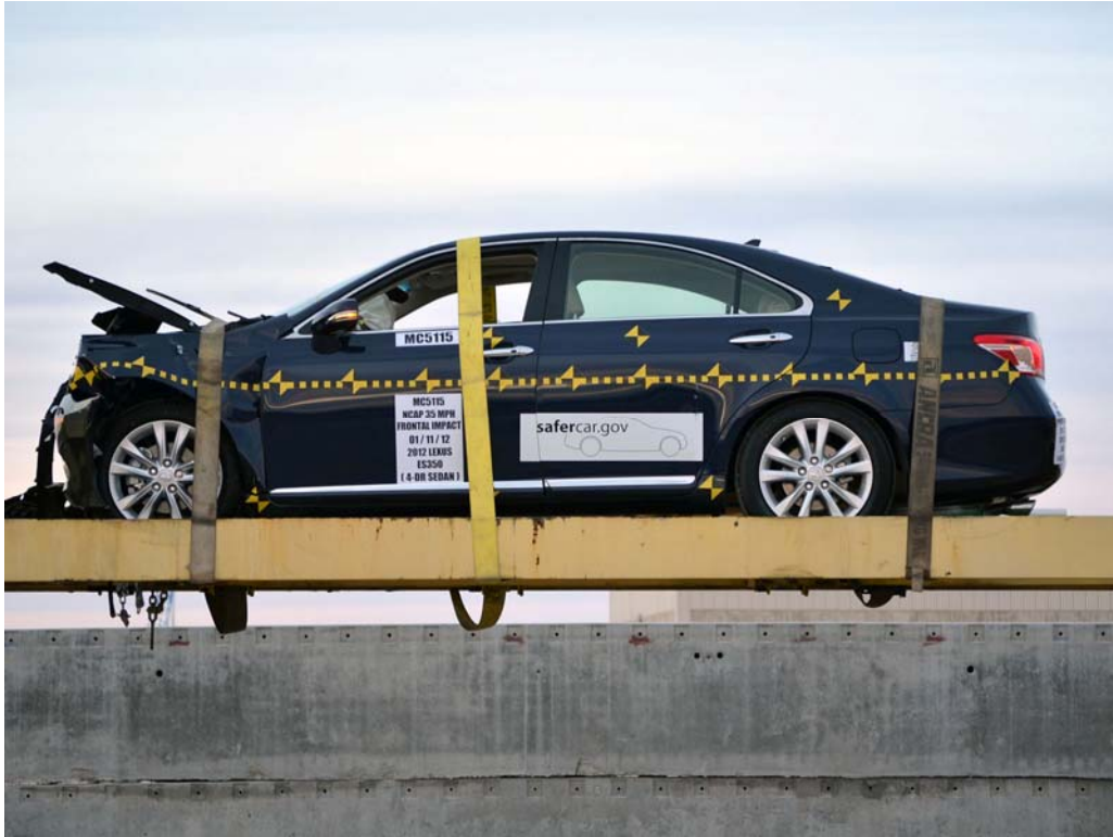
FIGURE 70. Vehicle at 360° on Static Rollover Device
