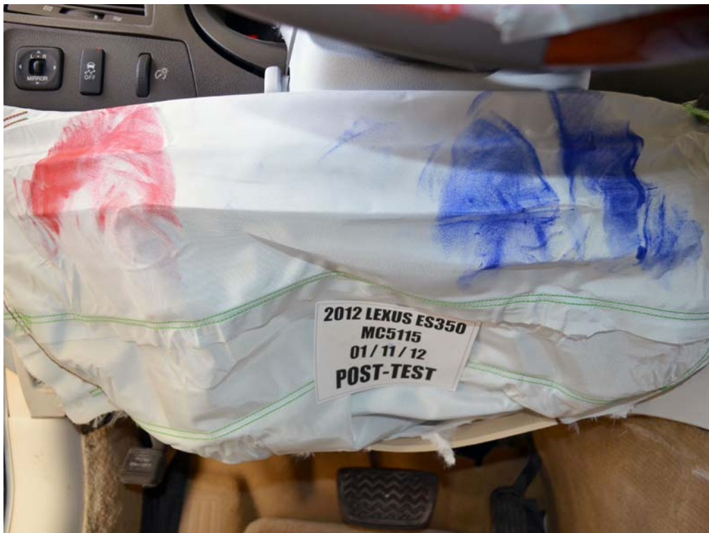
FIGURE 45a. Post-Test Driver Dummy Contact With Knee Airbag
