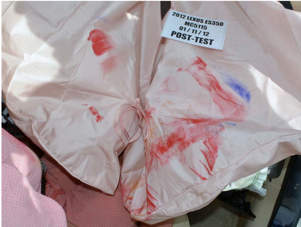
FIGURE 62. Post-Test Passenger Dummy Contact With Airbag
