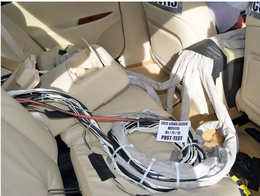
FIGURE 28. Post-Test Dummy Cable Routing
