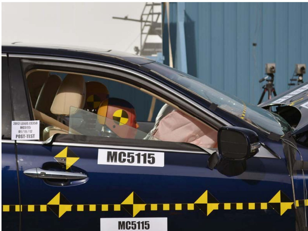
FIGURE 51. Post-Test Passenger Dummy Window View
