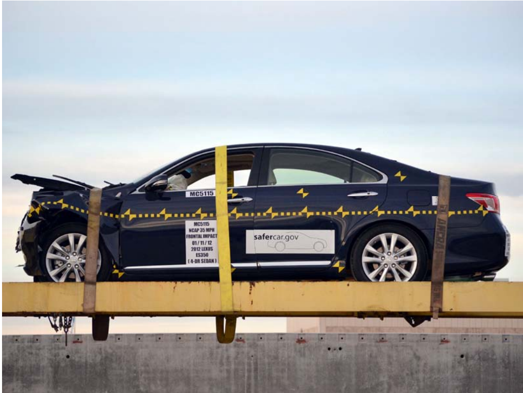
FIGURE 66. Vehicle at 0°on Static Rollover Device
