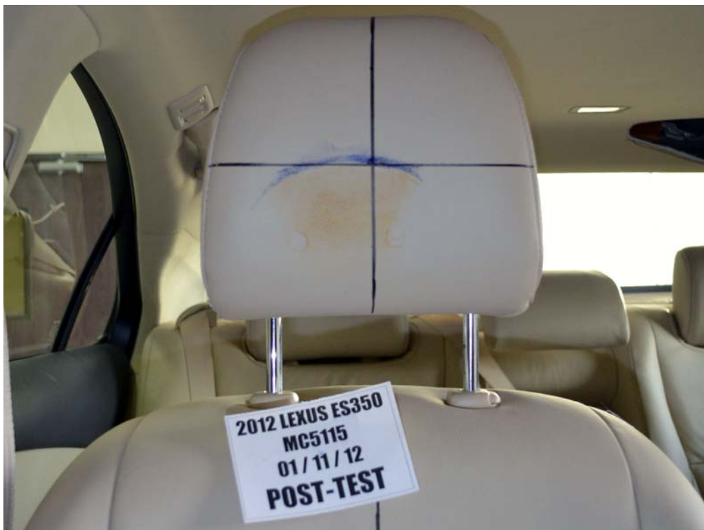
FIGURE 62a. Post-Test Passenger Dummy Contact With Headrest
