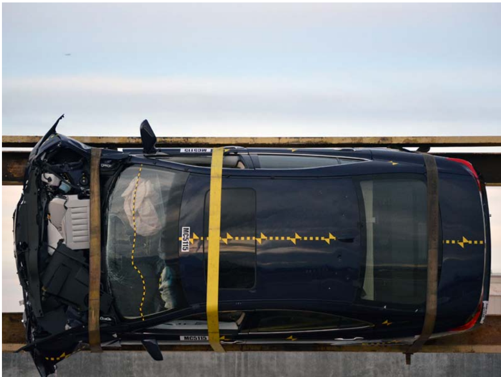
FIGURE 67. Vehicle at 90°on Static Rollover Device
