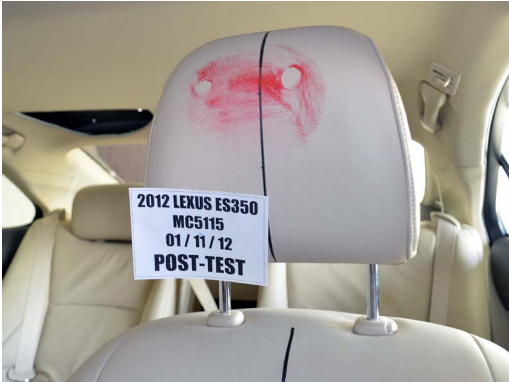
FIGURE 45. Post-Test Driver Dummy Contact With Headrest
