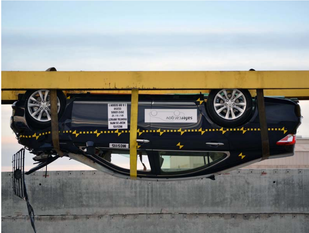
FIGURE 68. Vehicle at 180°on Static Rollover Device
