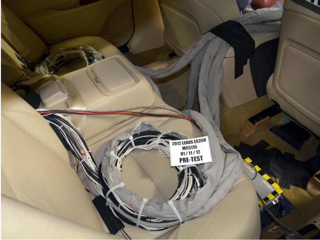
FIGURE 27. Pre-Test Dummy Cable Routing
