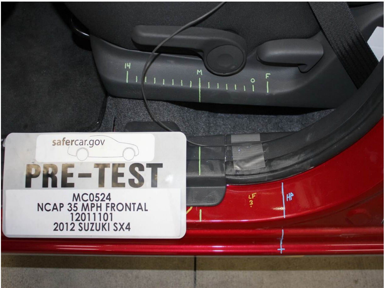
Pre-Test Driver's Seat Fore-Aft Markings
