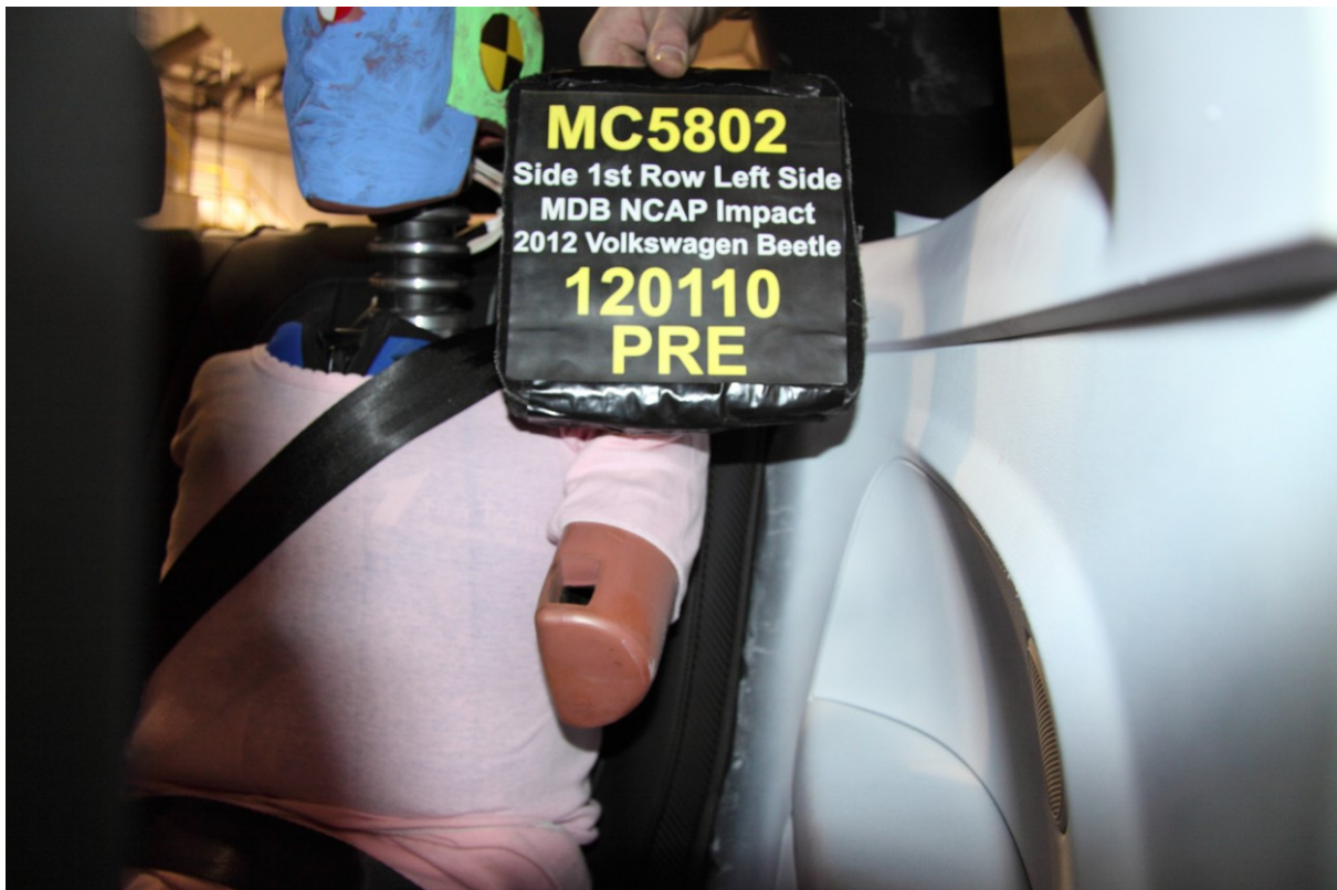
054 Pre-Test Left Side View of Passenger Dummy Showing Belt and Chalking
