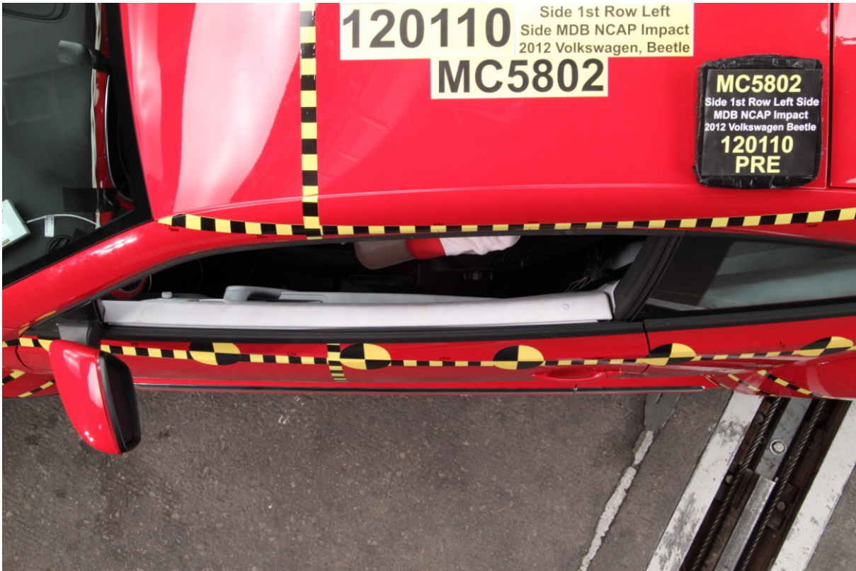
042 Pre-Test Driver Dummy and Door Clearance View
