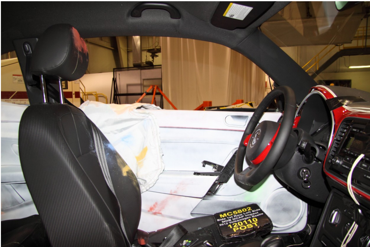
047 Post-Test Driver Inner Door Panel View
