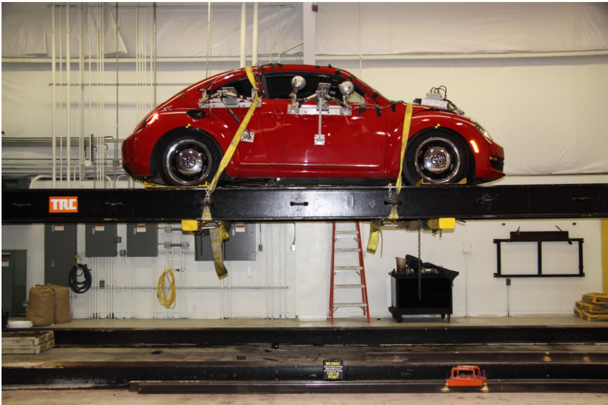
098 FMVSS No. 301 Static Rollover 360 Degrees
