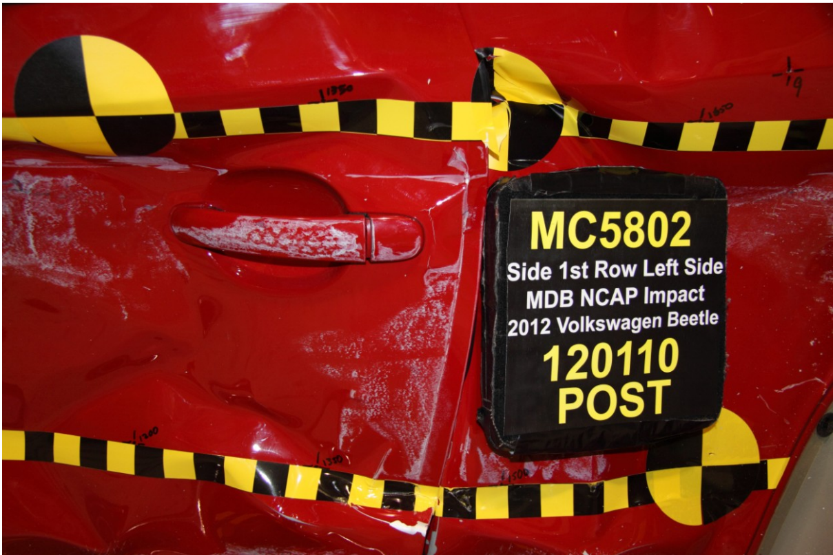
022 Post-Test Left Front Door Latch Close-up
