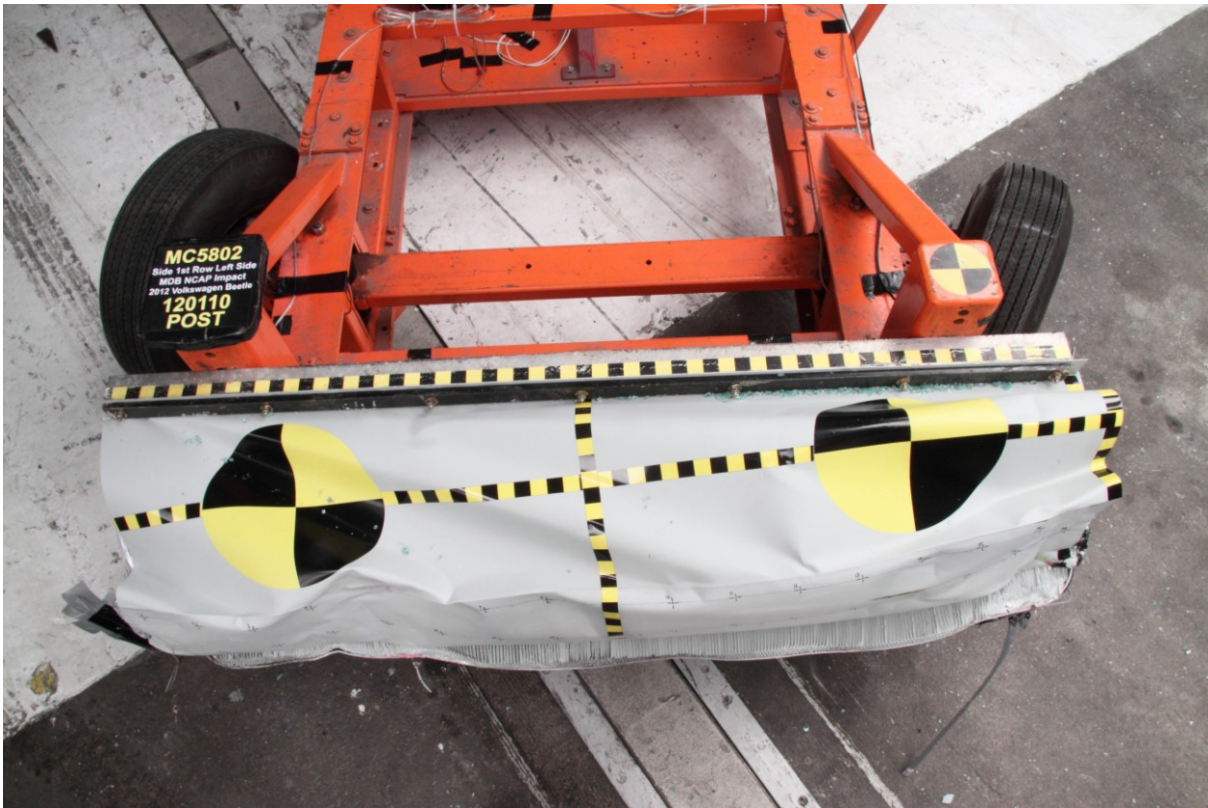
085 Post-Test Top View of MDB Impactor Face
