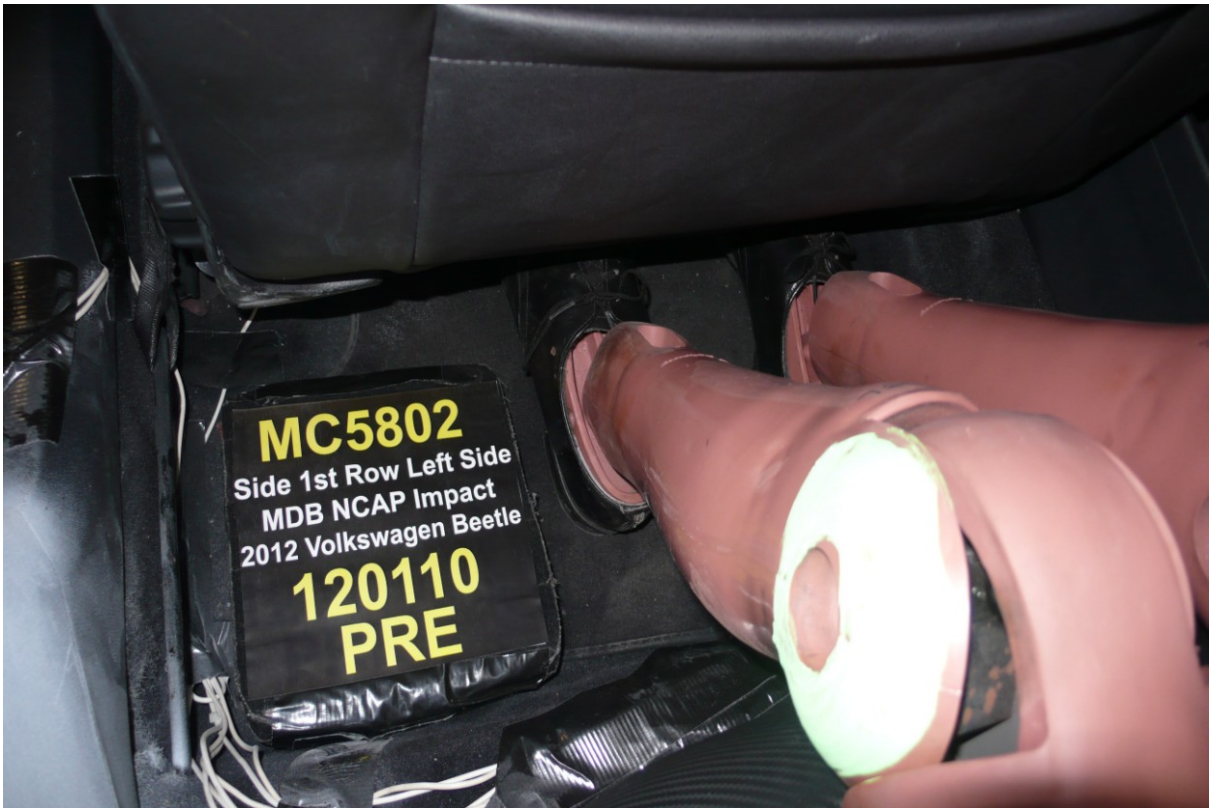
063 Pre-Test Placement of Rear Passenger Dummy Feet
