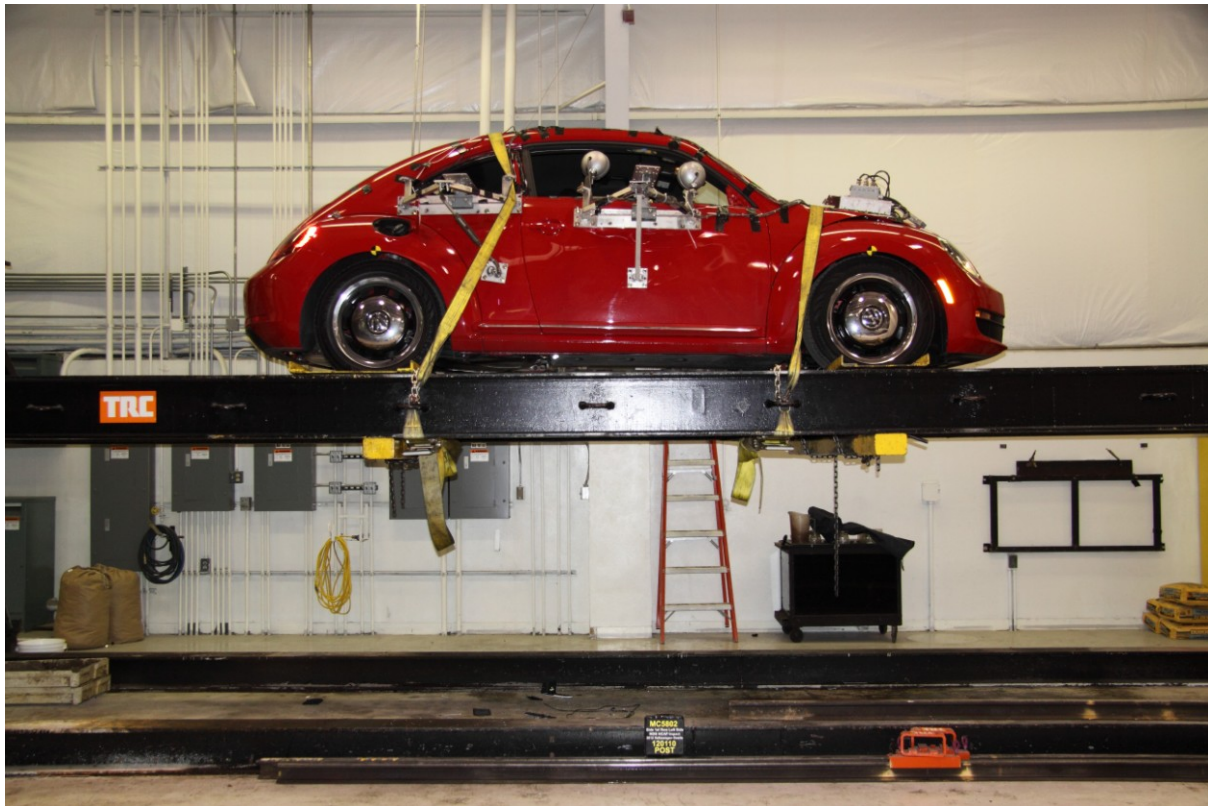
094 FMVSS No. 301 Static Rollover 0 Degrees
