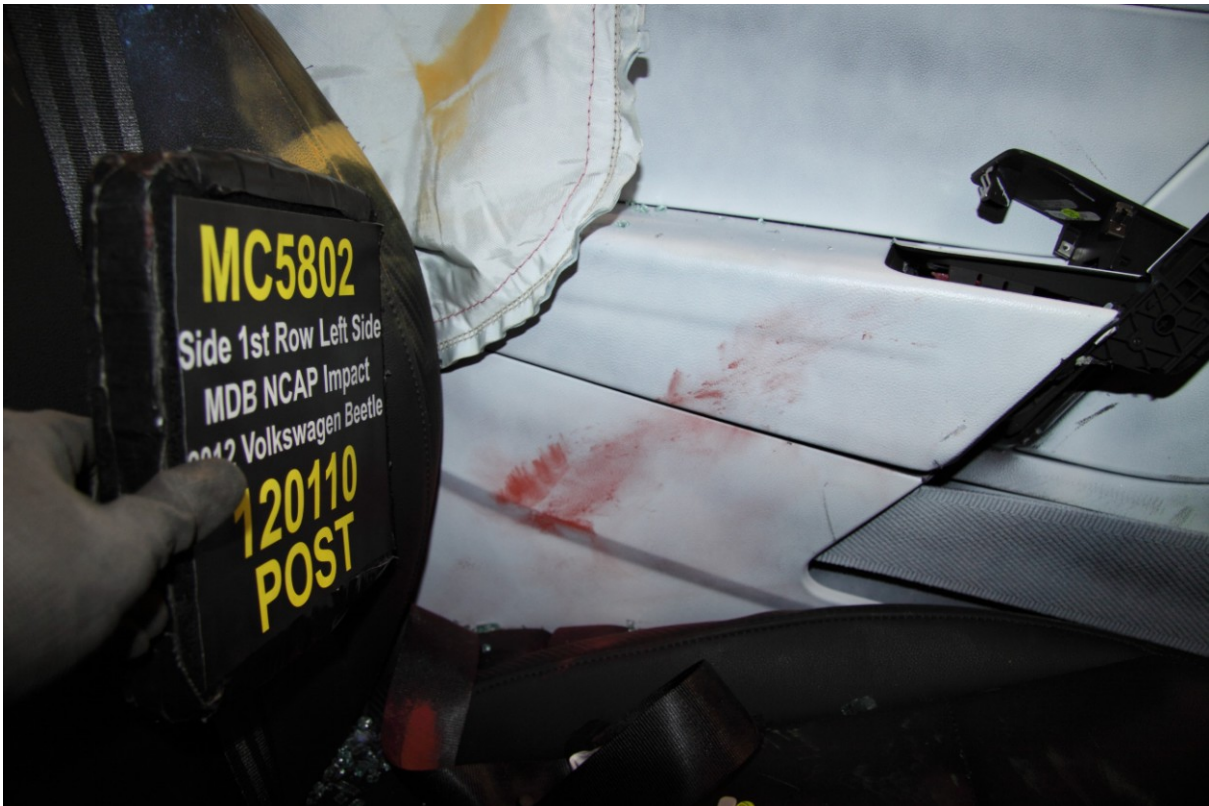
052 Post-Test Driver Dummy Close-Up Pelvis Contact with Vehicle Interior View
