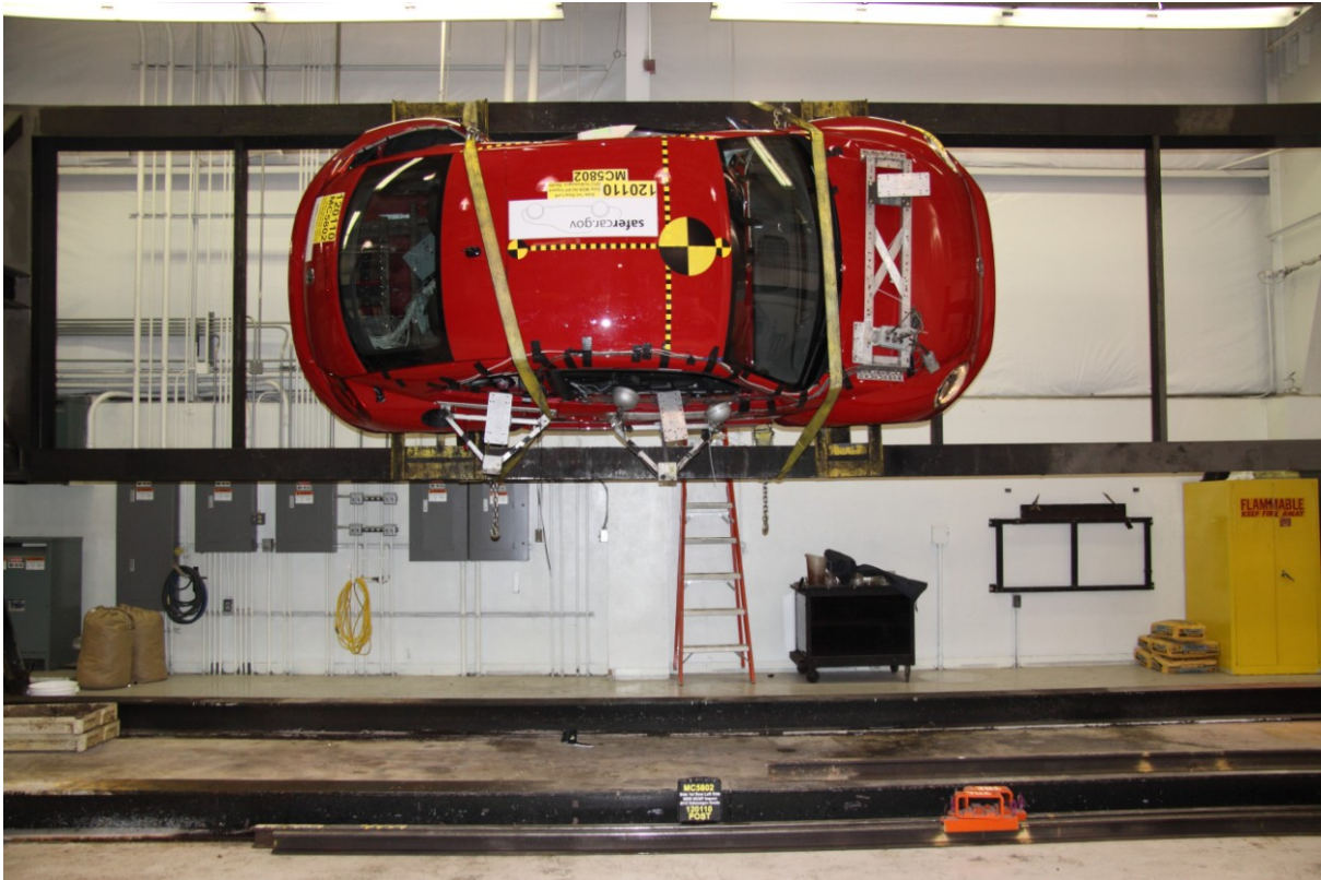
095 FMVSS No. 301 Static Rollover 90 Degrees
