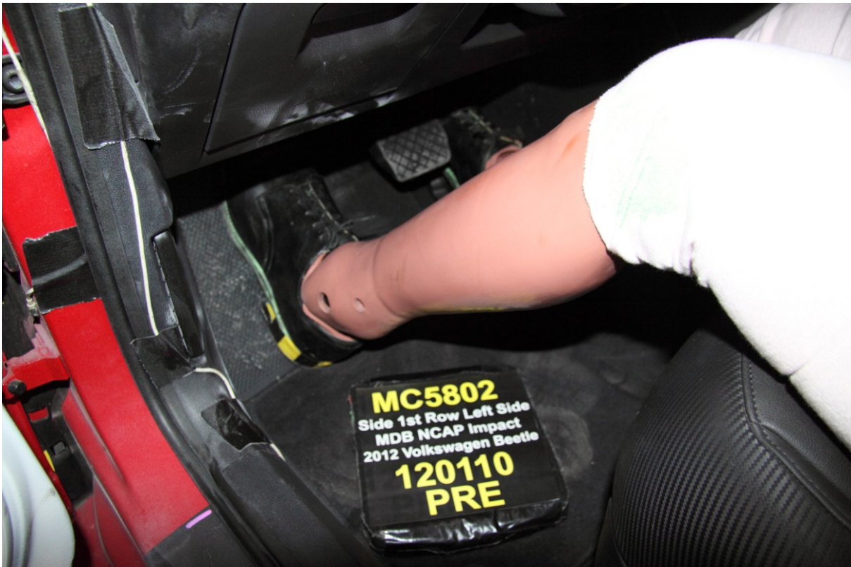
034 Pre-Test Placement of Driver Dummy Feet
