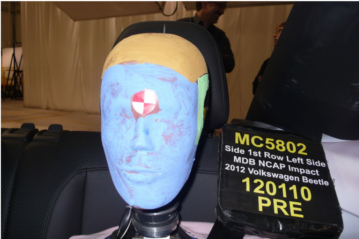
058 Pre-Test Frontal View of Rear Passenger Dummy Head and Shoulders in Relation to Head Restraint
