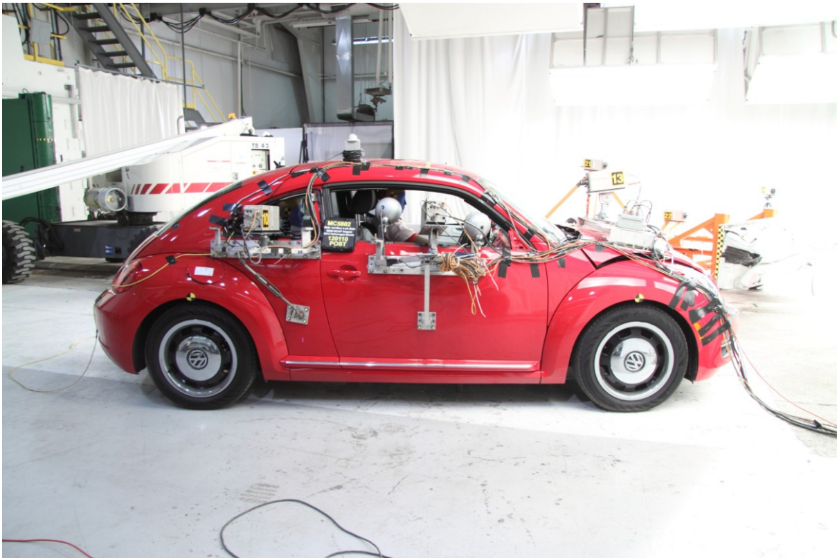
014 Post-Test Right Side View of Test Vehicle
