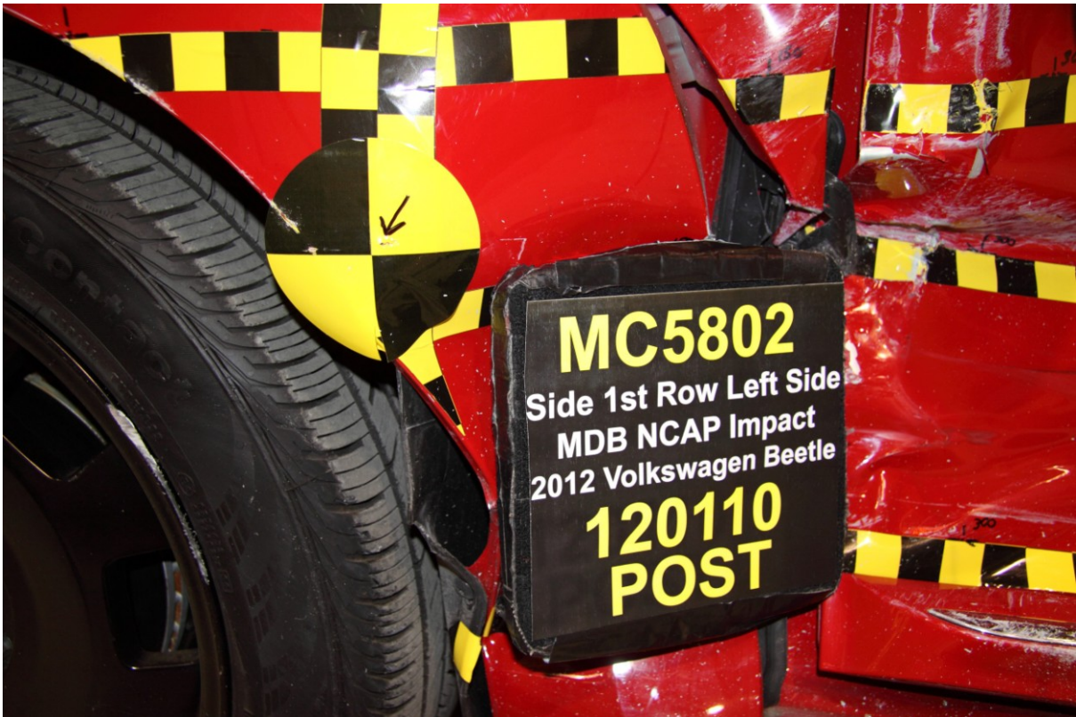
020 Post-Test Close-up View of Impact Point Target
