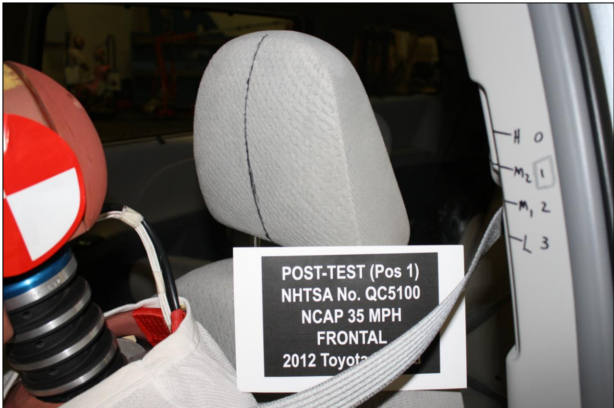
Figure A-45: Post-Test Driver Dummy Contact with Headrest (Headrest disconnected from seatback during the event, Head hit the back of headrest)
