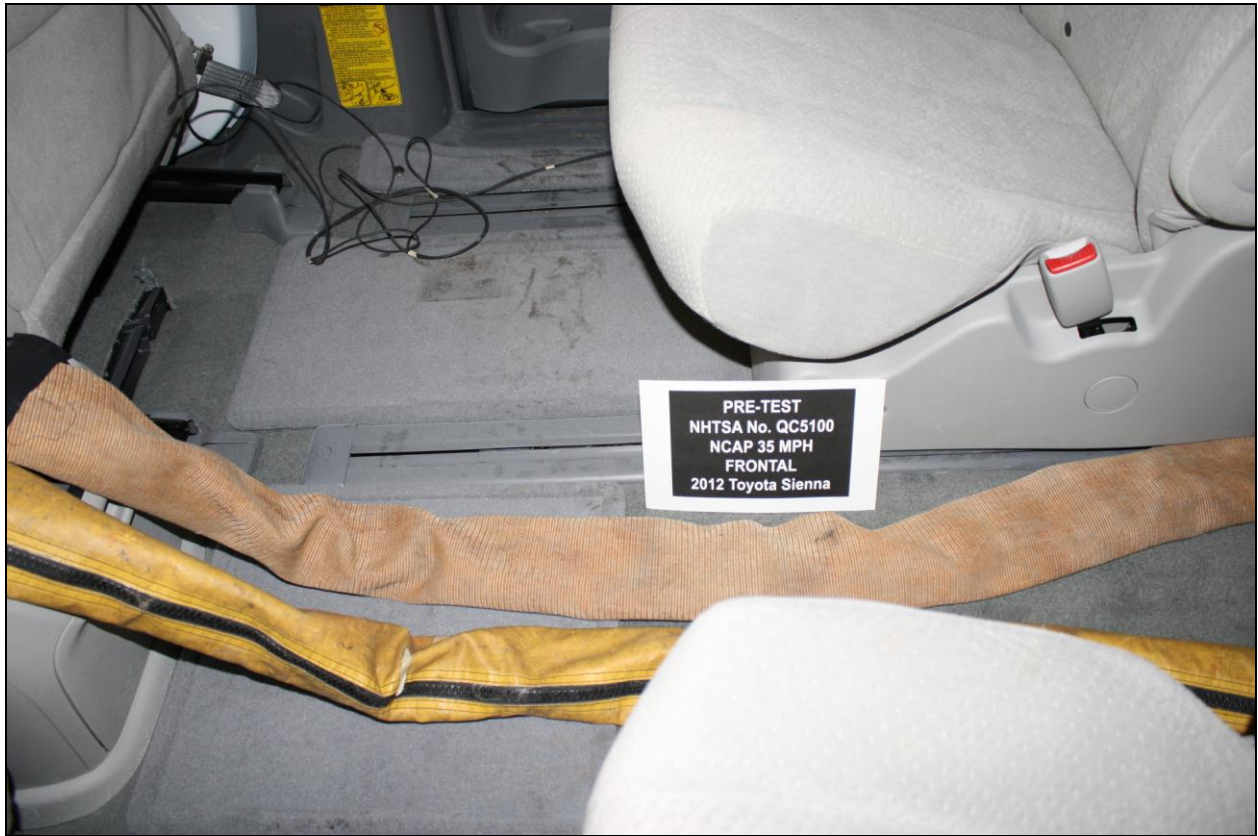
Figure A-27: Pre-Test Dummy Cable Routing
