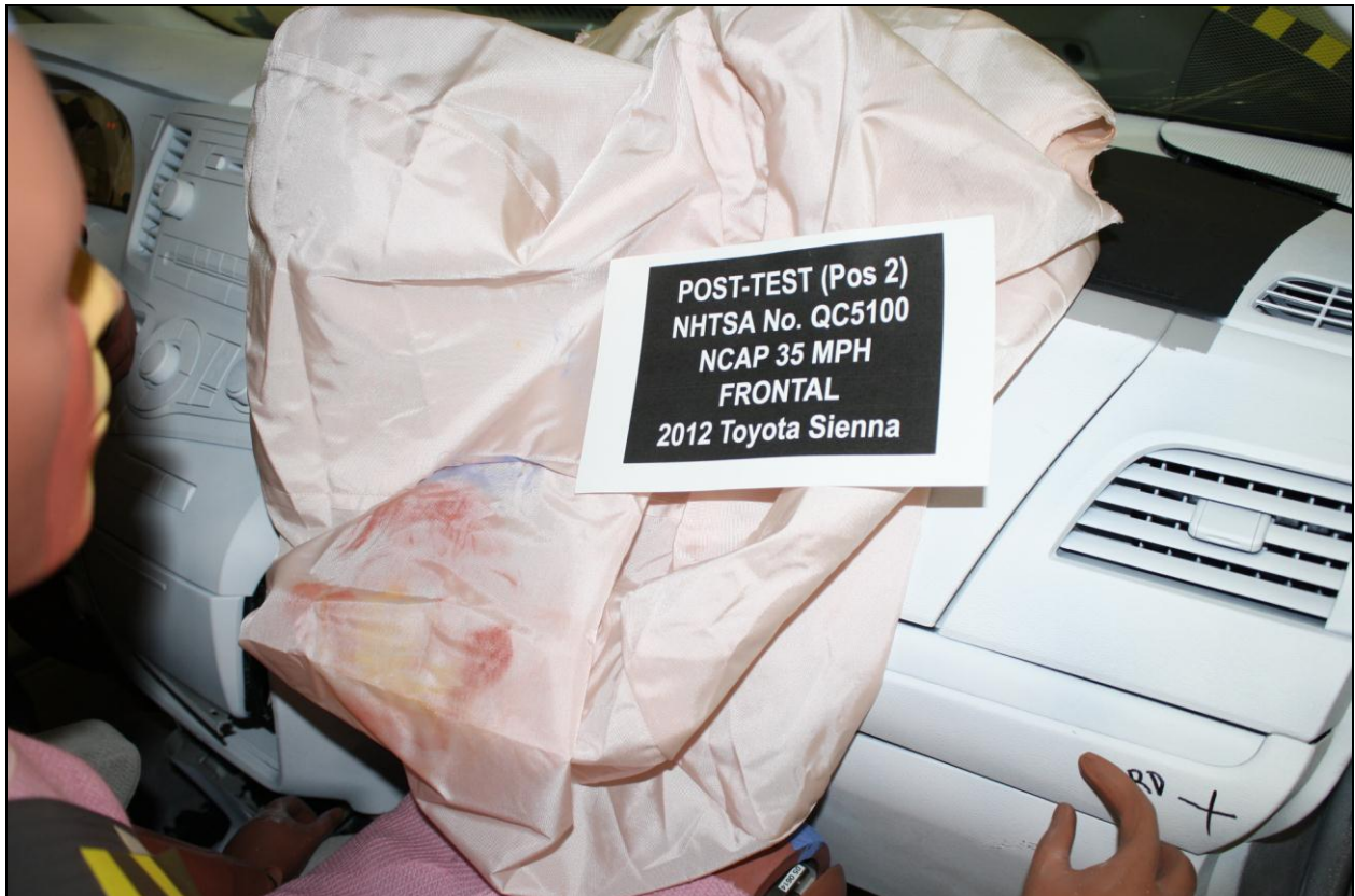
Figure A-62: Post-Test Passenger Dummy Contact with Airbag
