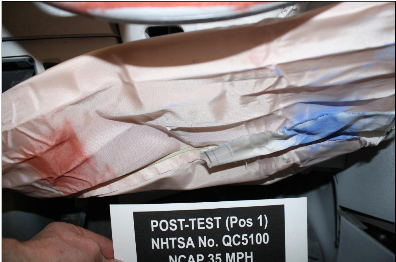
Figure A-40: Post-Test Driver's Side Knee Bolster
