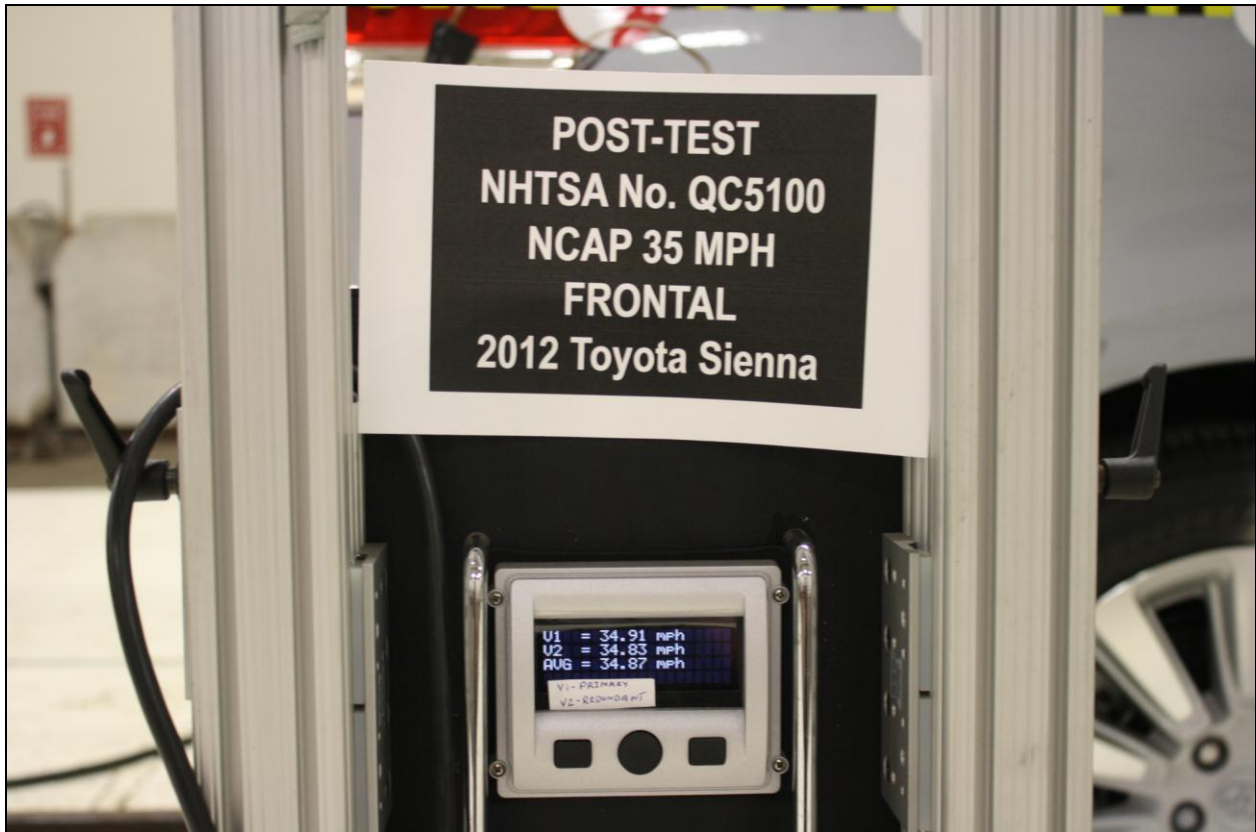
Figure A-65: Post-Test Speed Trap Read-Out
