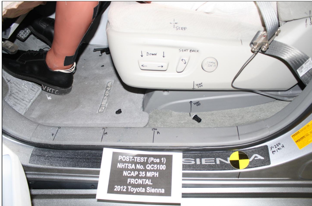
Figure A-36: Post-Test Driver's Seat Fore-Aft Markings
