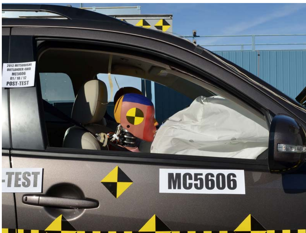
FIGURE 51. Post-Test Passenger Dummy Window View
