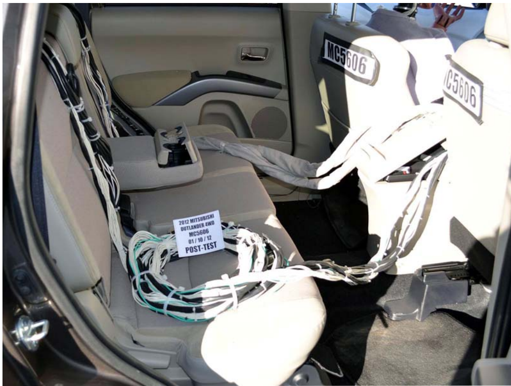
FIGURE 28. Post-Test Dummy Cable Routing
