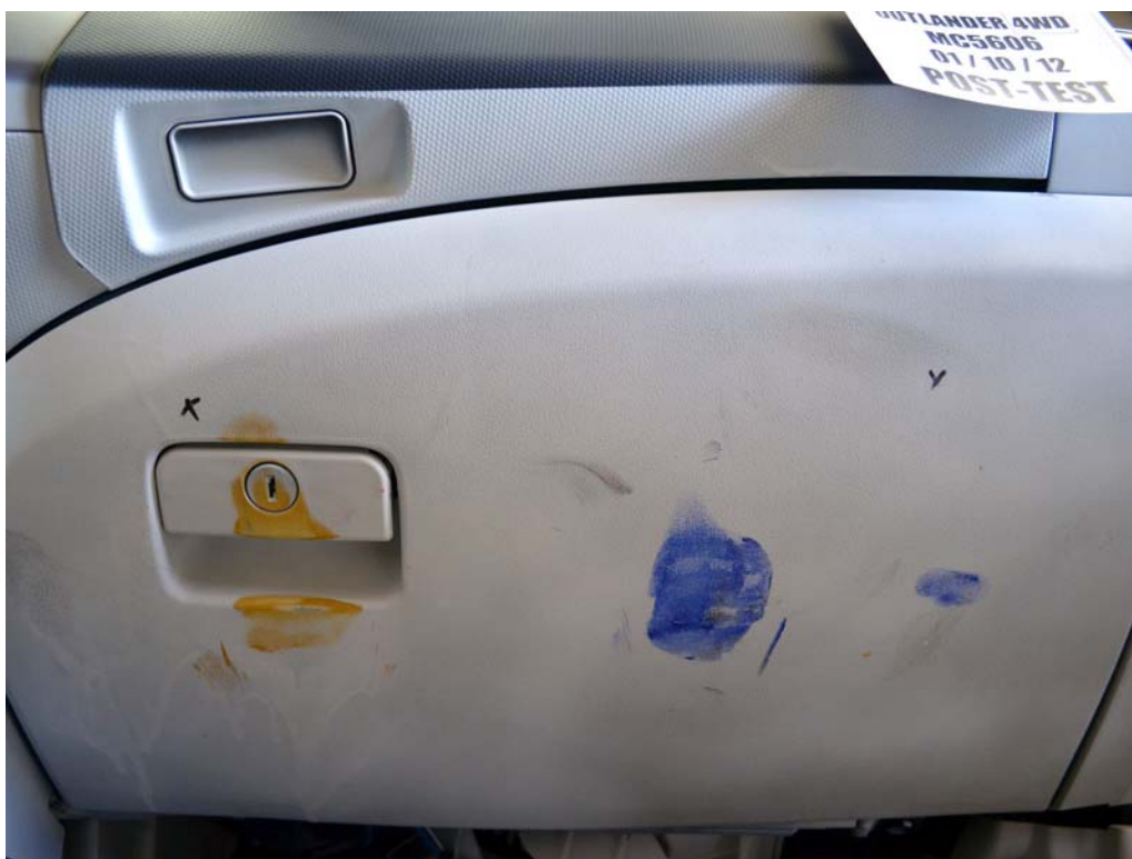
FIGURE 62b. Post-Test Passenger Dummy Contact Glovebox
