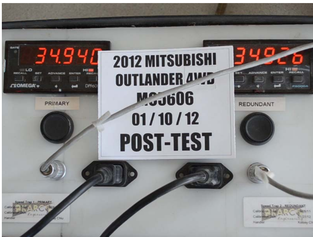
FIGURE 65. Post-Test Speed Trap Read Out
