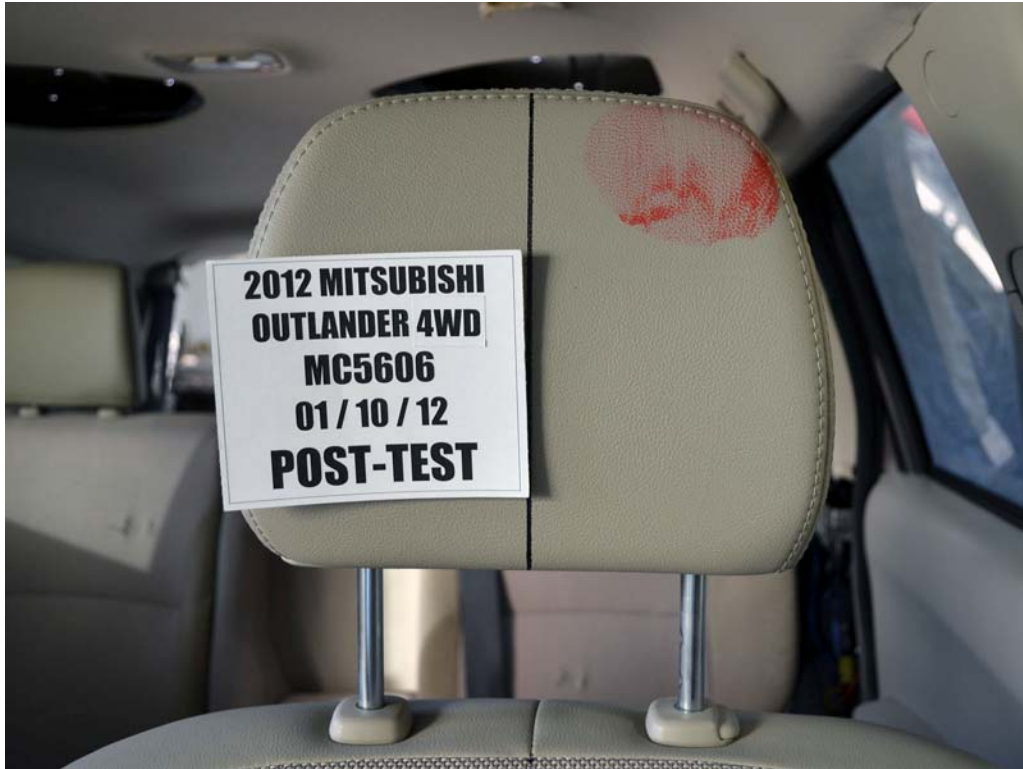
FIGURE 45. Post-Test Driver Dummy Contact With Headrest
