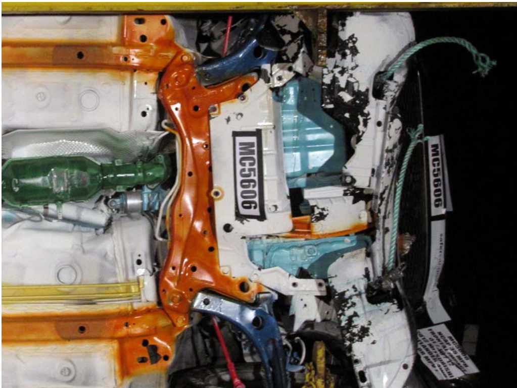
FIGURE 24. Post-Test Front Underbody View
