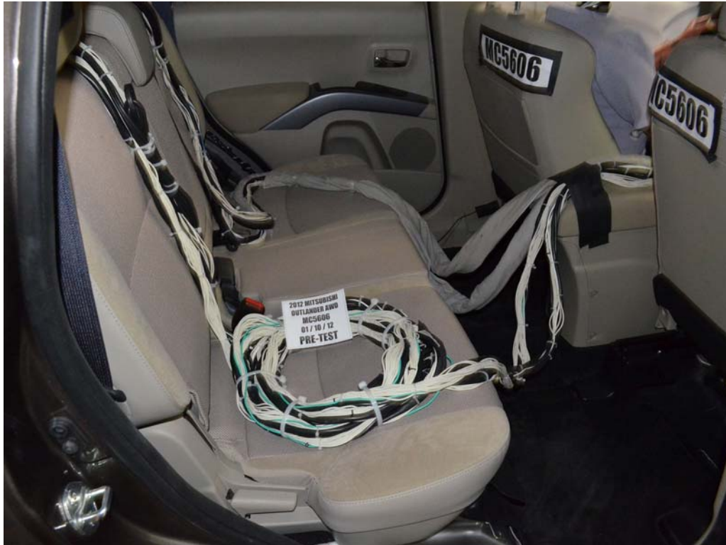
FIGURE 27. Pre-Test Dummy Cable Routing
