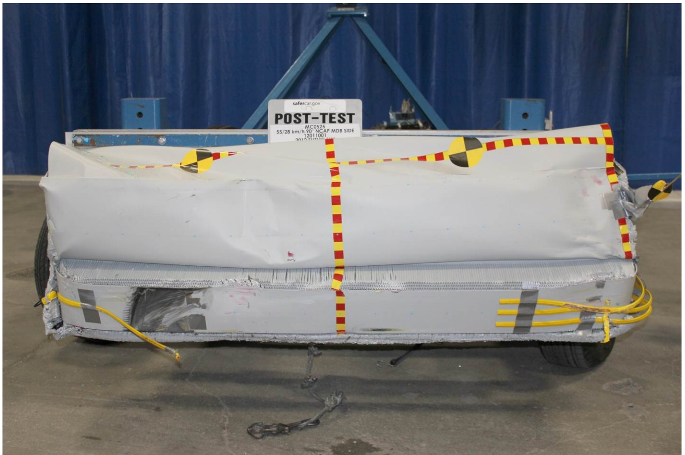
Post-Test Front View of MDB Impactor Face
