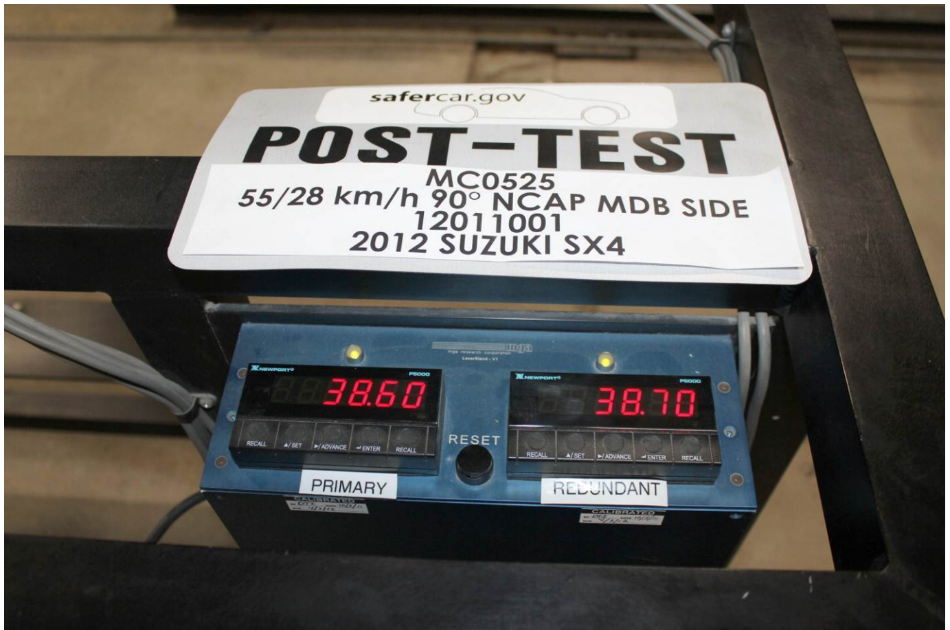
Post-Test Primary and Redundant Speed Trap Read-Out
