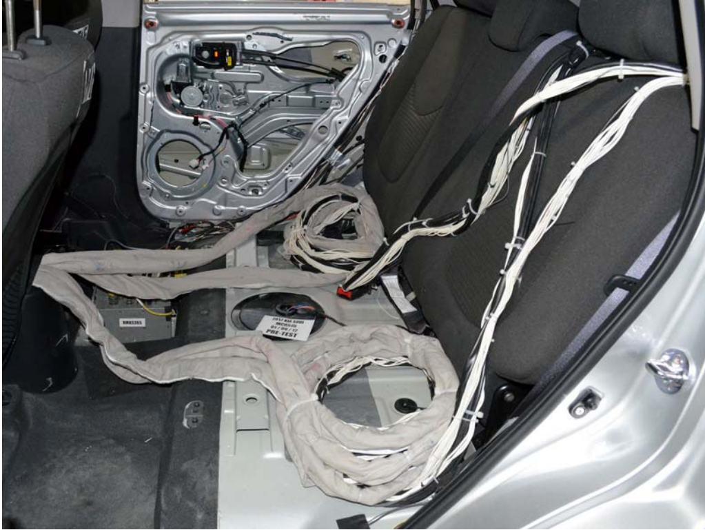
FIGURE 27. Pre-Test Dummy Cable Routing
