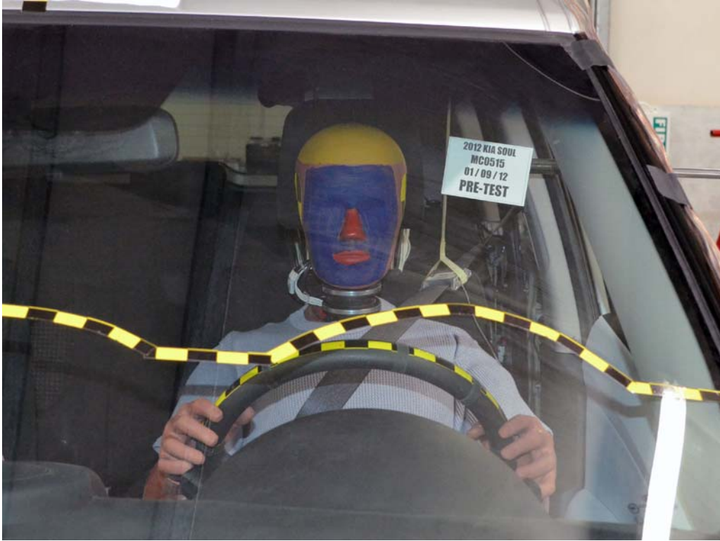
FIGURE 29. Pre-Test Driver Dummy Front View
