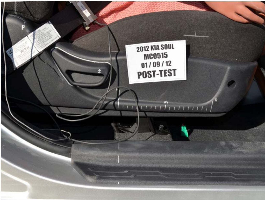
FIGURE 55. Post-Test Passenger's Seat Fore-Aft Markings
