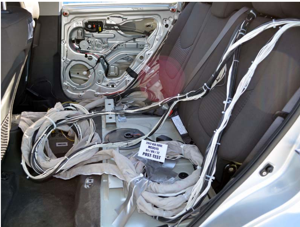
FIGURE 28. Post-Test Dummy Cable Routing
