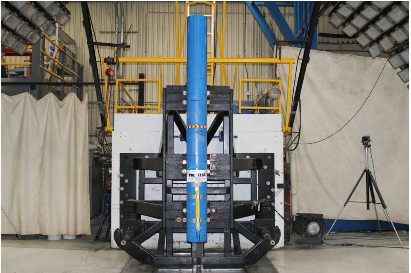
Pre-Test Pole Barrier Front View
