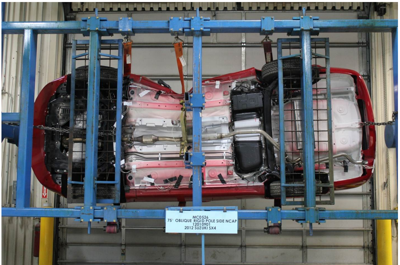
FMVSS No. 301 Static Rollover 270 Degrees
