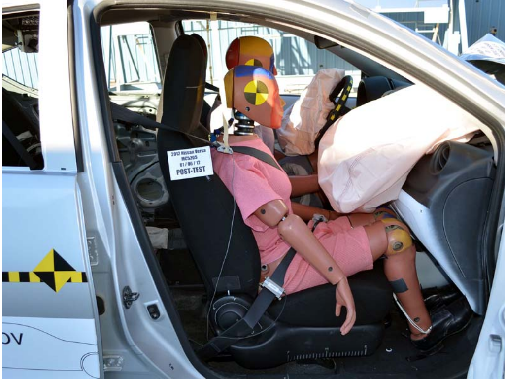
FIGURE 53. Post-Test Passenger Dummy and Vehicle Interior View
