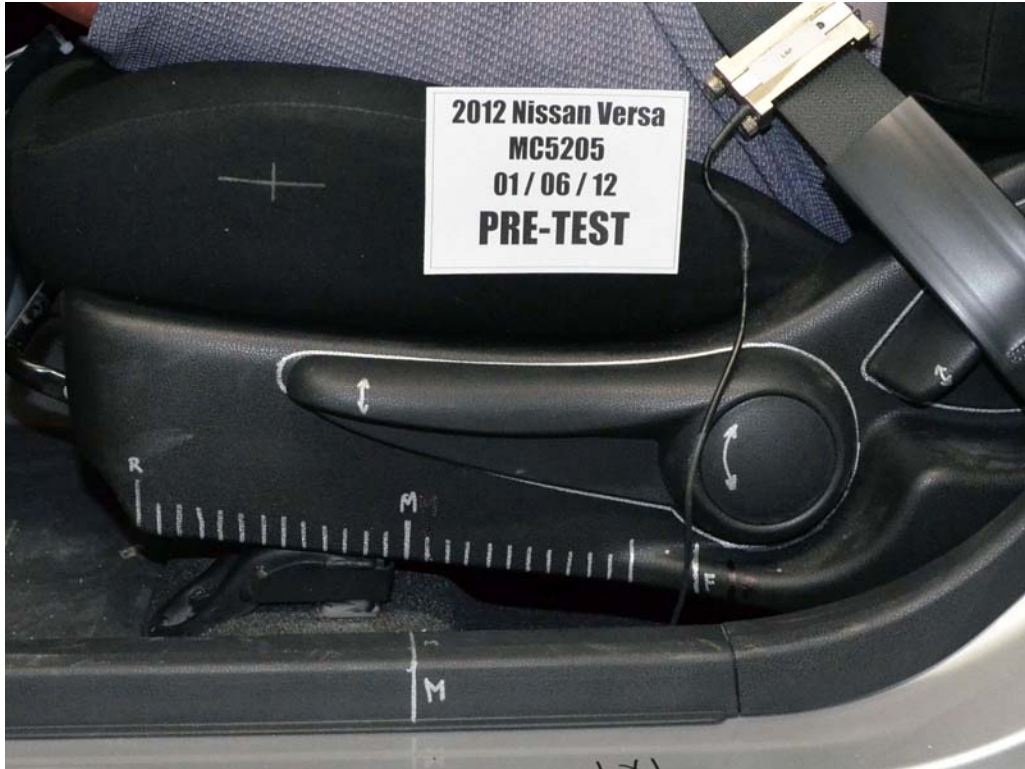
FIGURE 35. Pre-Test Driver's Seat Fore-Aft Markings
