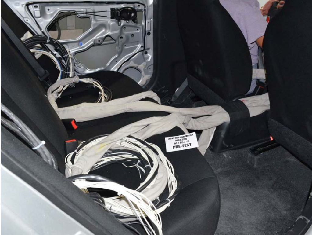
FIGURE 27. Pre-Test Dummy Cable Routing
