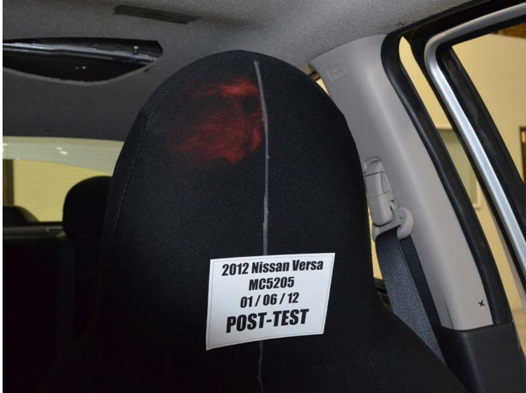
FIGURE 45. Post-Test Driver Dummy Contact With Head Rest
