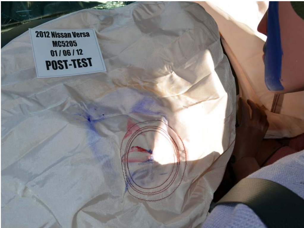
FIGURE 44. Post-Test Driver Dummy Contact With Airbag
