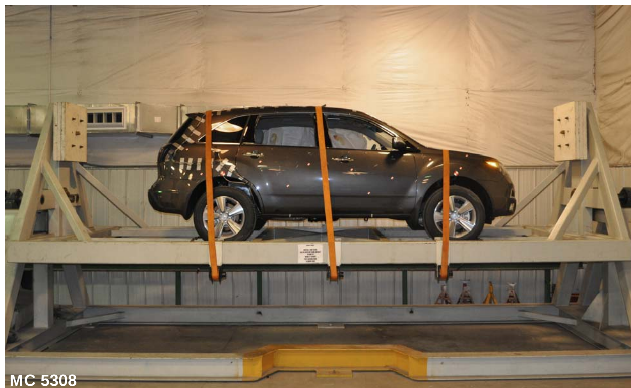
Figure A-94: FMVSS No. 301 Static Rollover 0 Degrees
