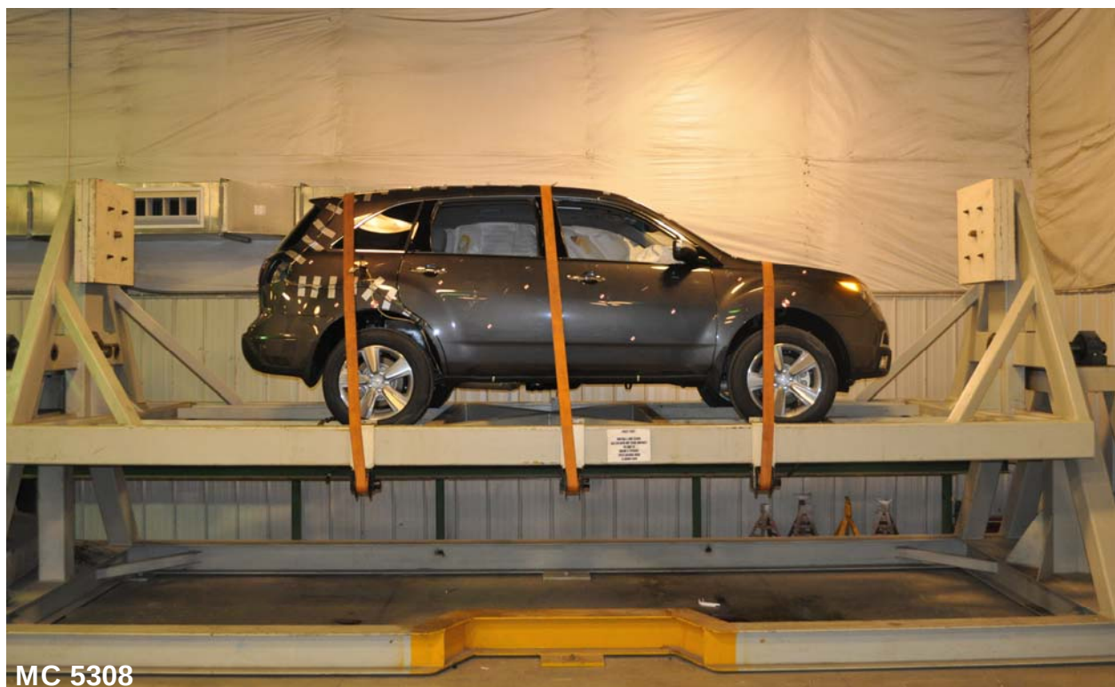
Figure A-98: FMVSS No. 301 Static Rollover 360 Degrees
