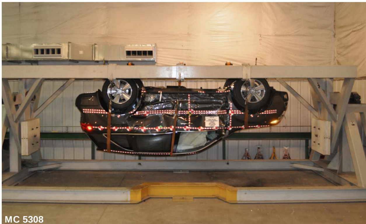
Figure A-96: FMVSS No. 301 Static Rollover 180 Degrees
