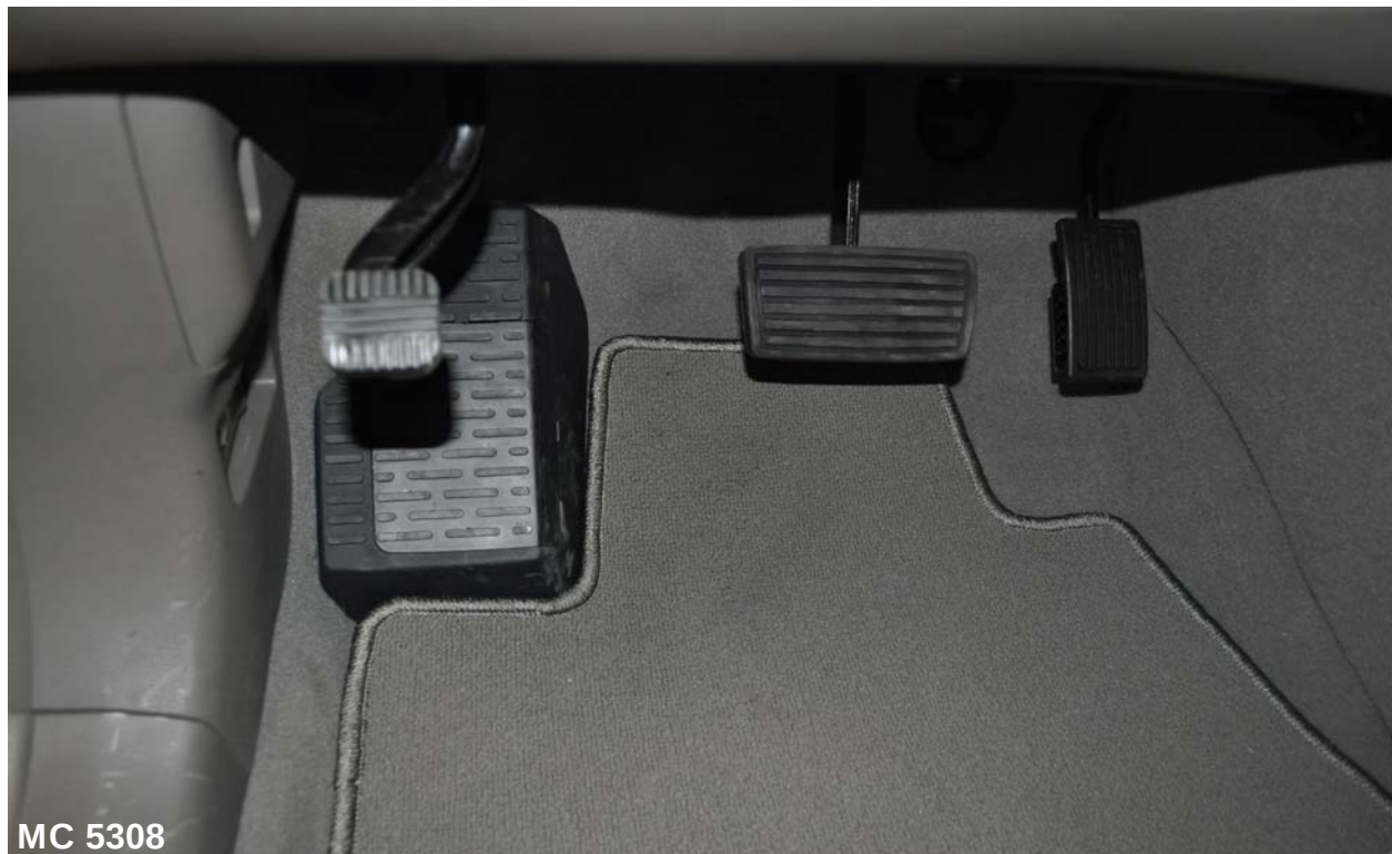
Figure A-37: View of Disengaged Parking Brake
