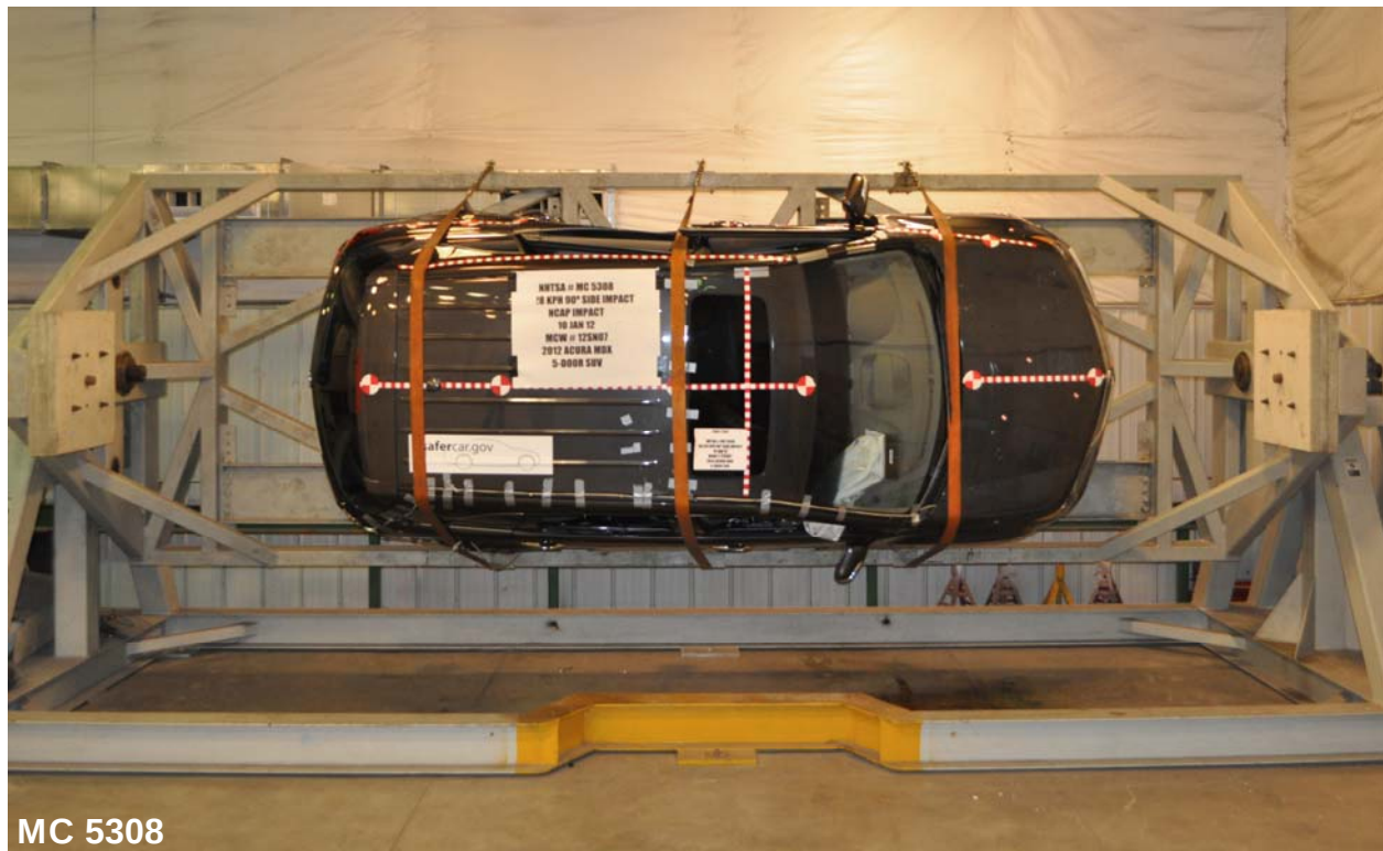
Figure A-97: FMVSS No. 301 Static Rollover 270 Degrees
