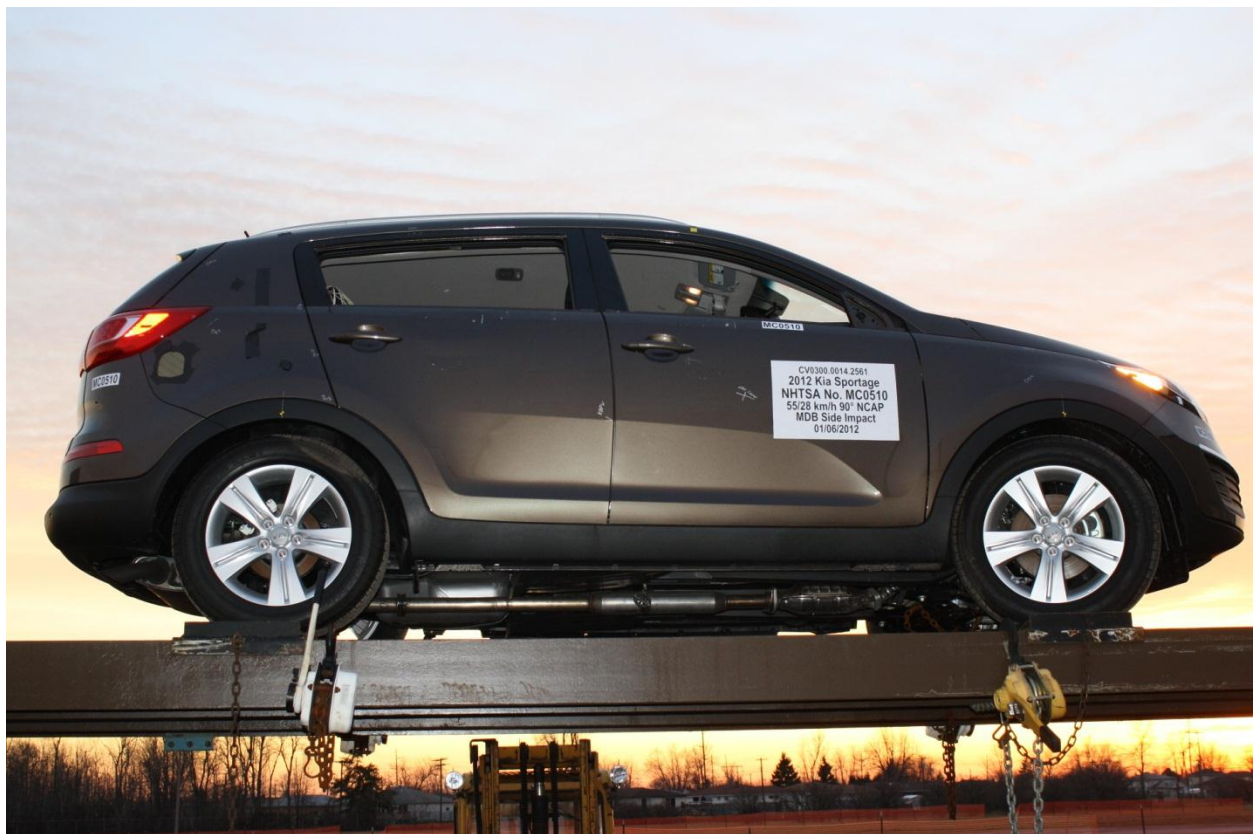
Figure A-98: FMVSS No. 301 Static Rollover 360 Degrees
