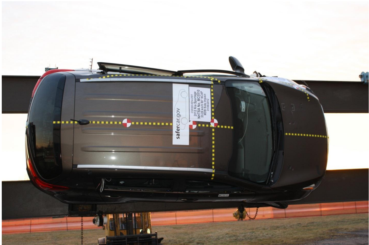
Figure A-97: FMVSS No. 301 Static Rollover 270 Degrees
