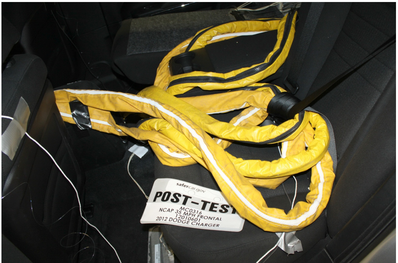
Post-Test Dummy Cable Routing
