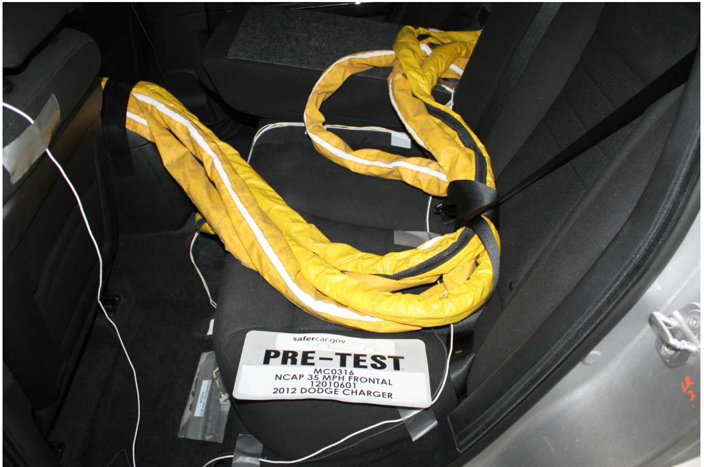
Pre-Test Dummy Cable Routing
