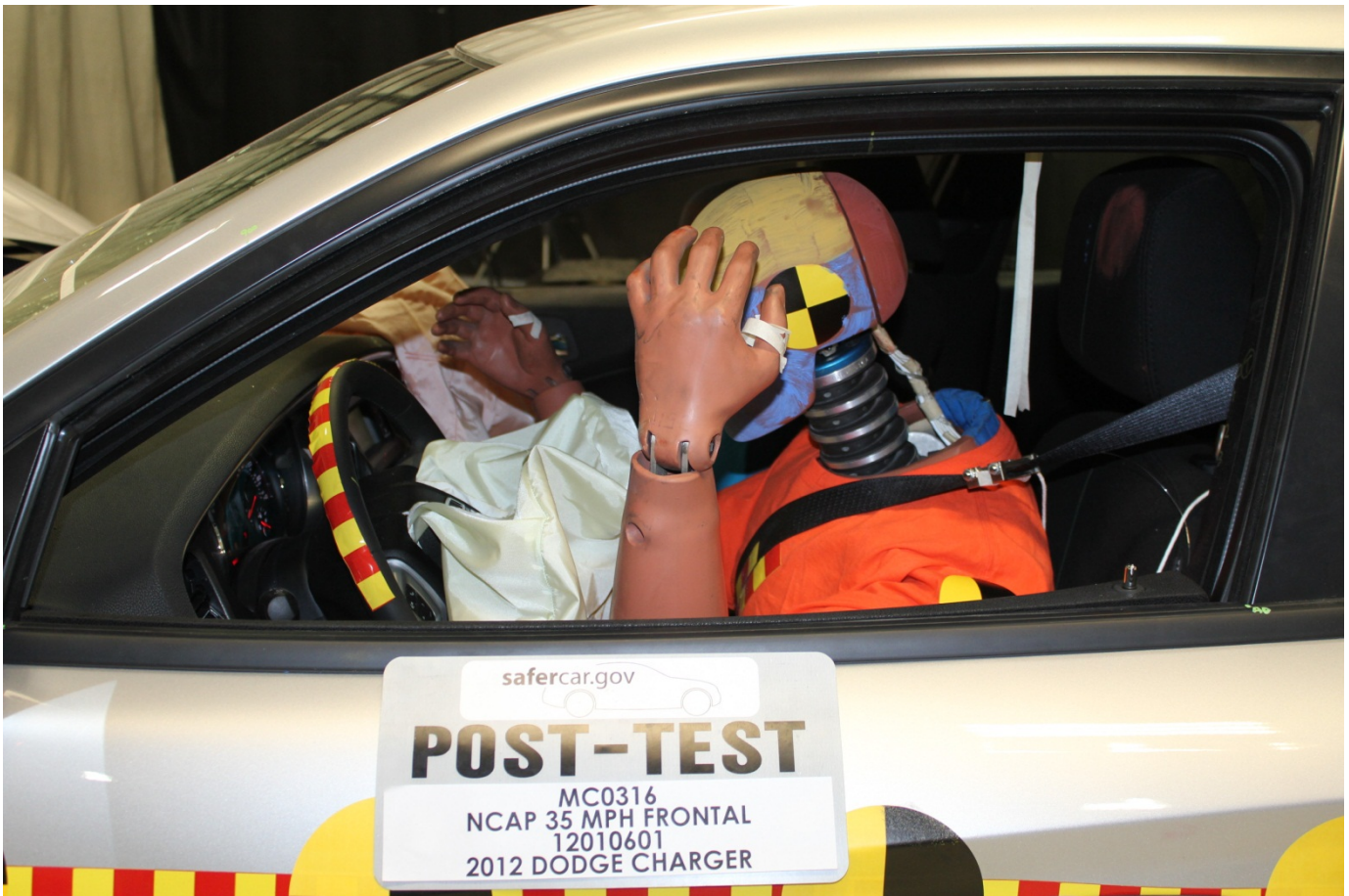
Post-Test Driver Dummy Window View
