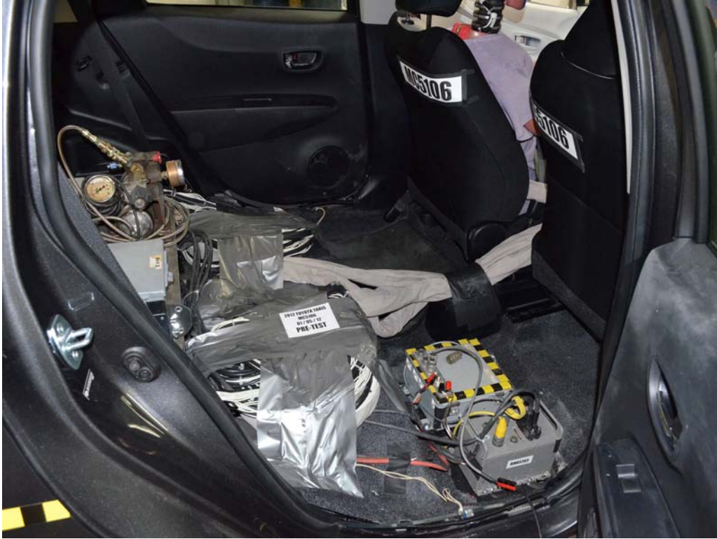
FIGURE 27. Pre-Test Dummy Cable Routing
