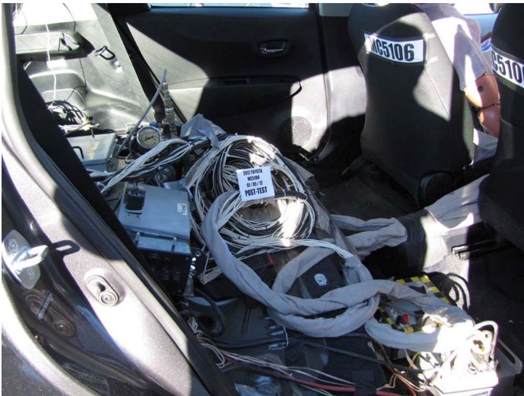
FIGURE 28. Post-Test Dummy Cable Routing
