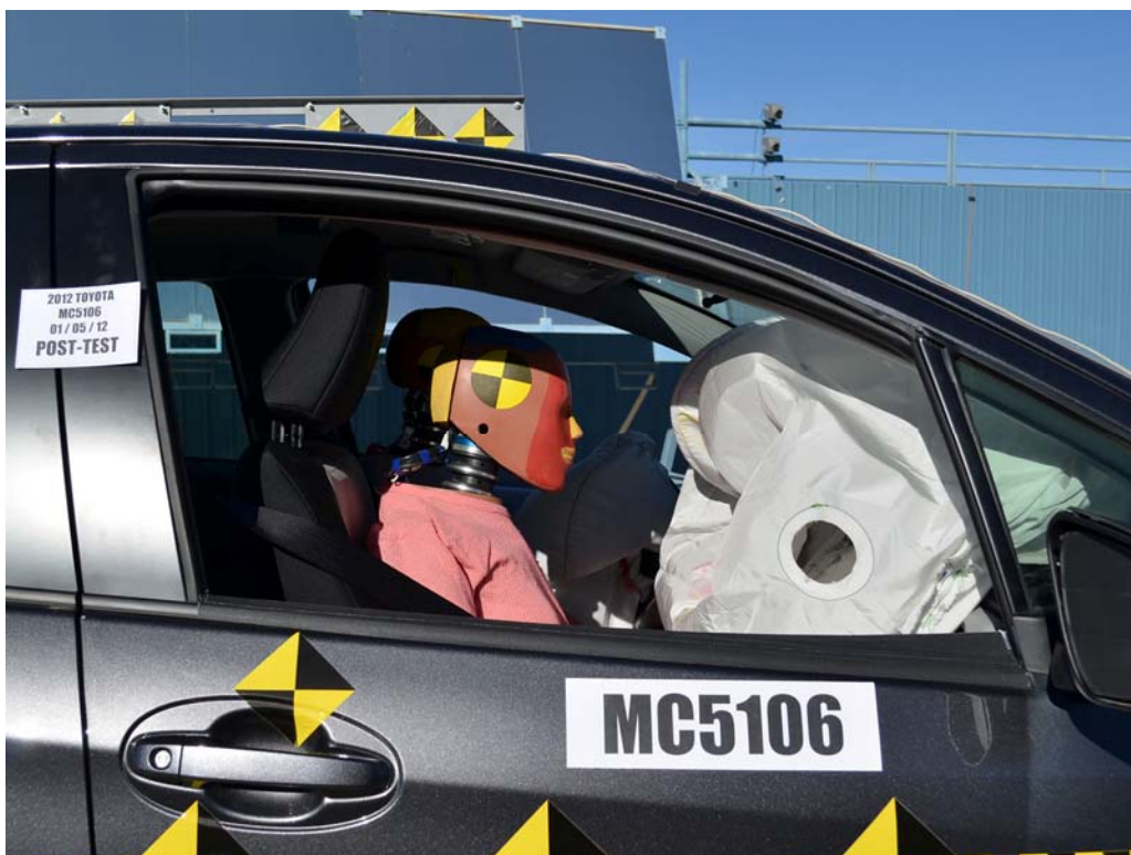
FIGURE 51. Post-Test Passenger Dummy Window View
