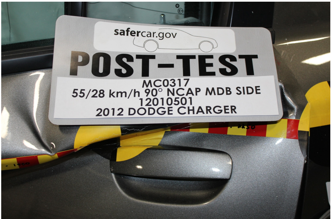
Post-Test Left Rear Door Latch Close-Up
