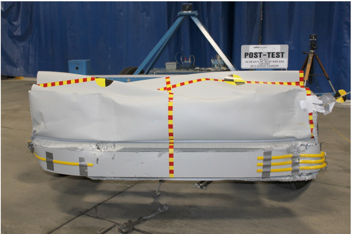
Post-Test Front View of MDB Impactor Face
