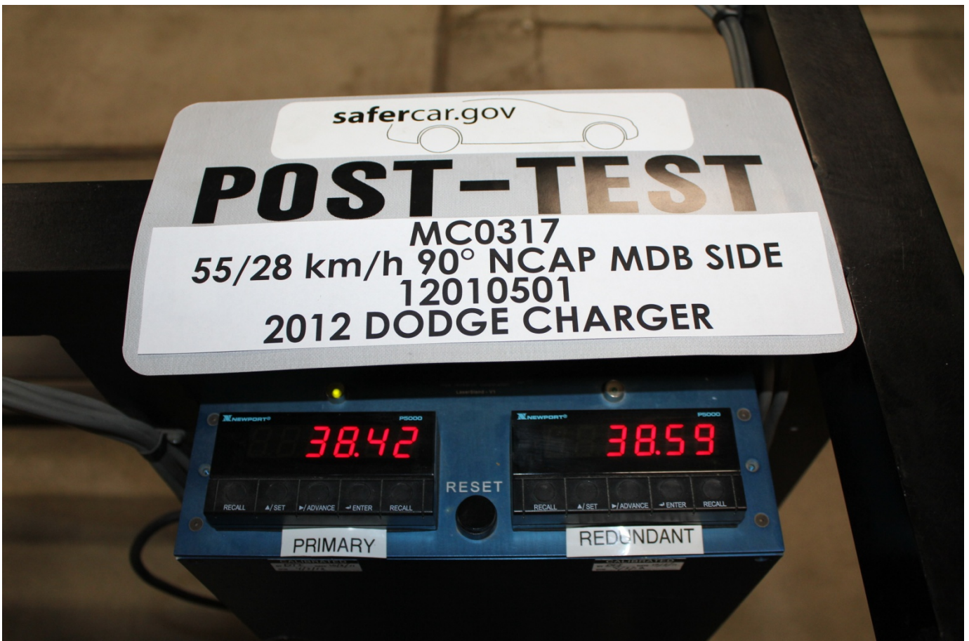
Post-Test Primary and Redundant Speed Trap Read-Out
