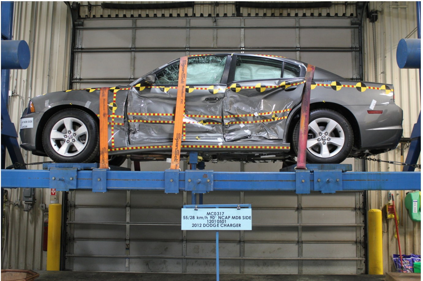
FMVSS No. 301 Static Rollover 0 Degrees
