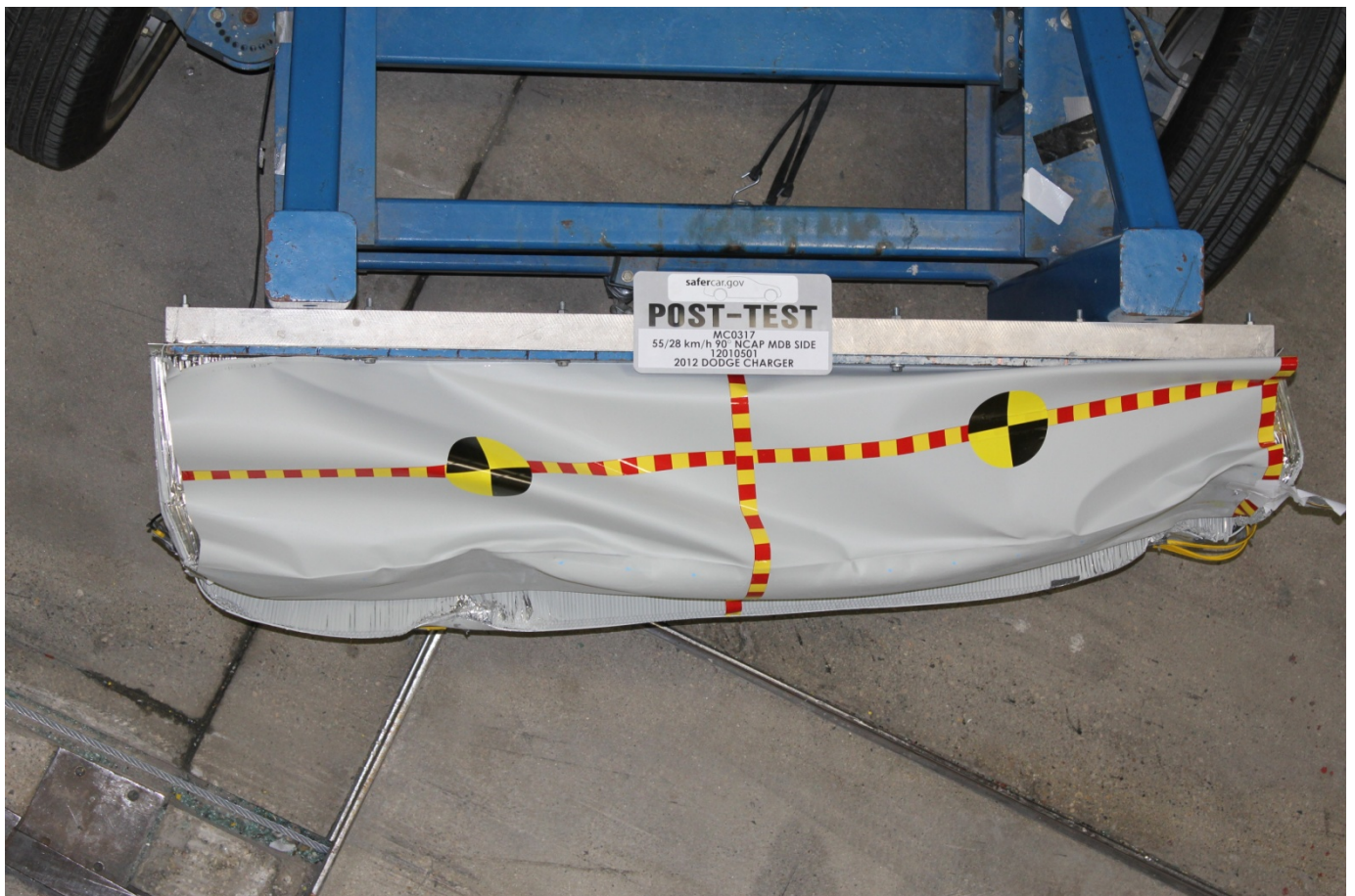
Post-Test Top View of MDB Impactor Face
