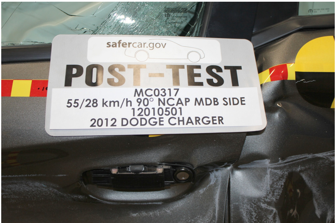
Post-Test Left Front Door Latch Close-Up
