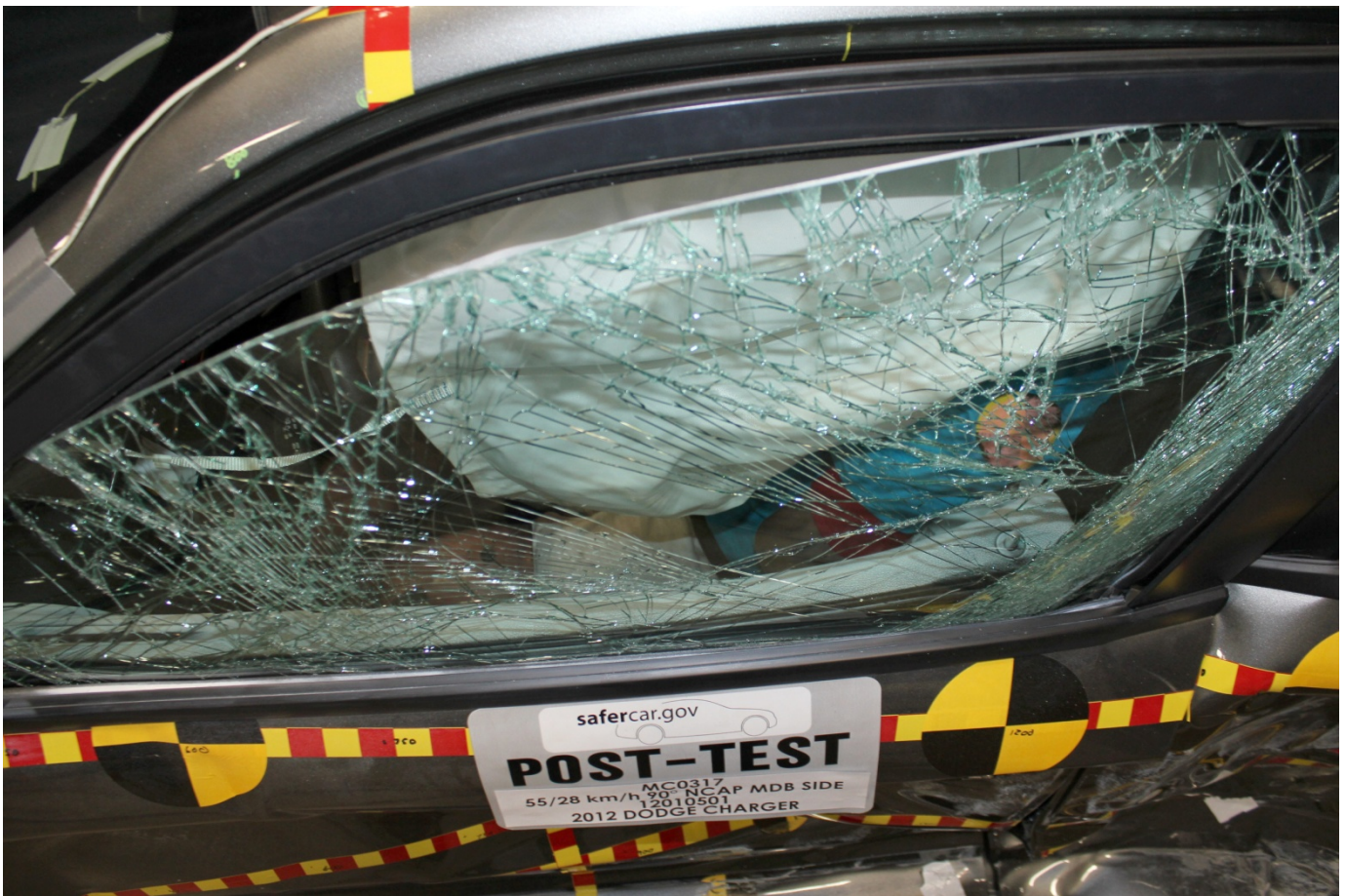
Post-Test Driver Dummy and Door Clearance View
