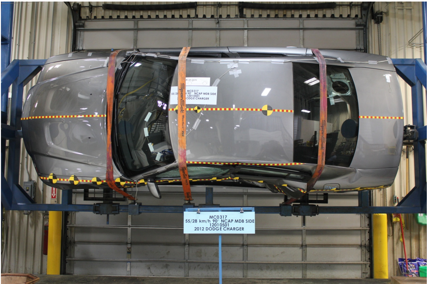
FMVSS No. 301 Static Rollover 90 Degrees
