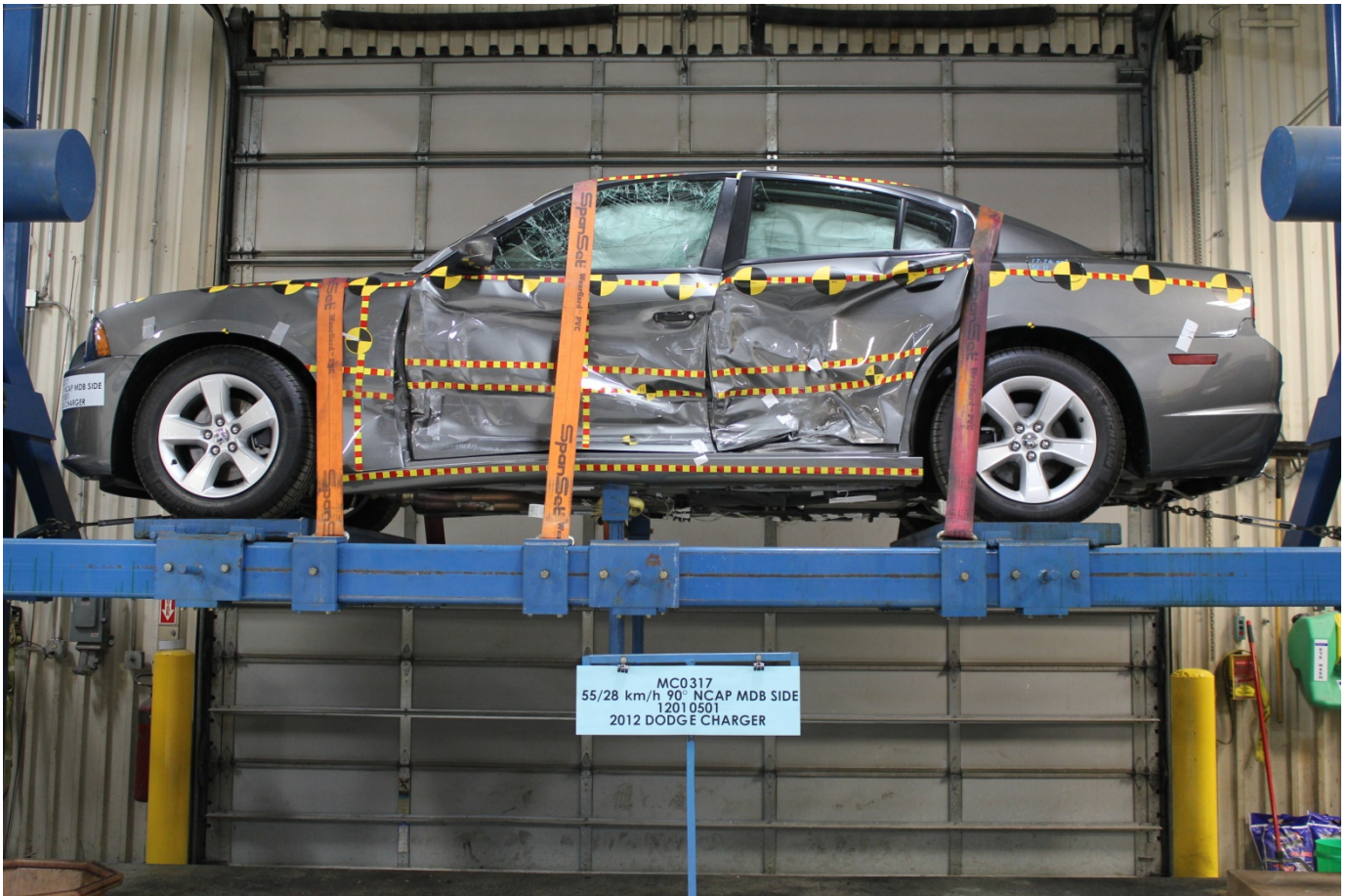
FMVSS No. 301 Static Rollover 360 Degrees
