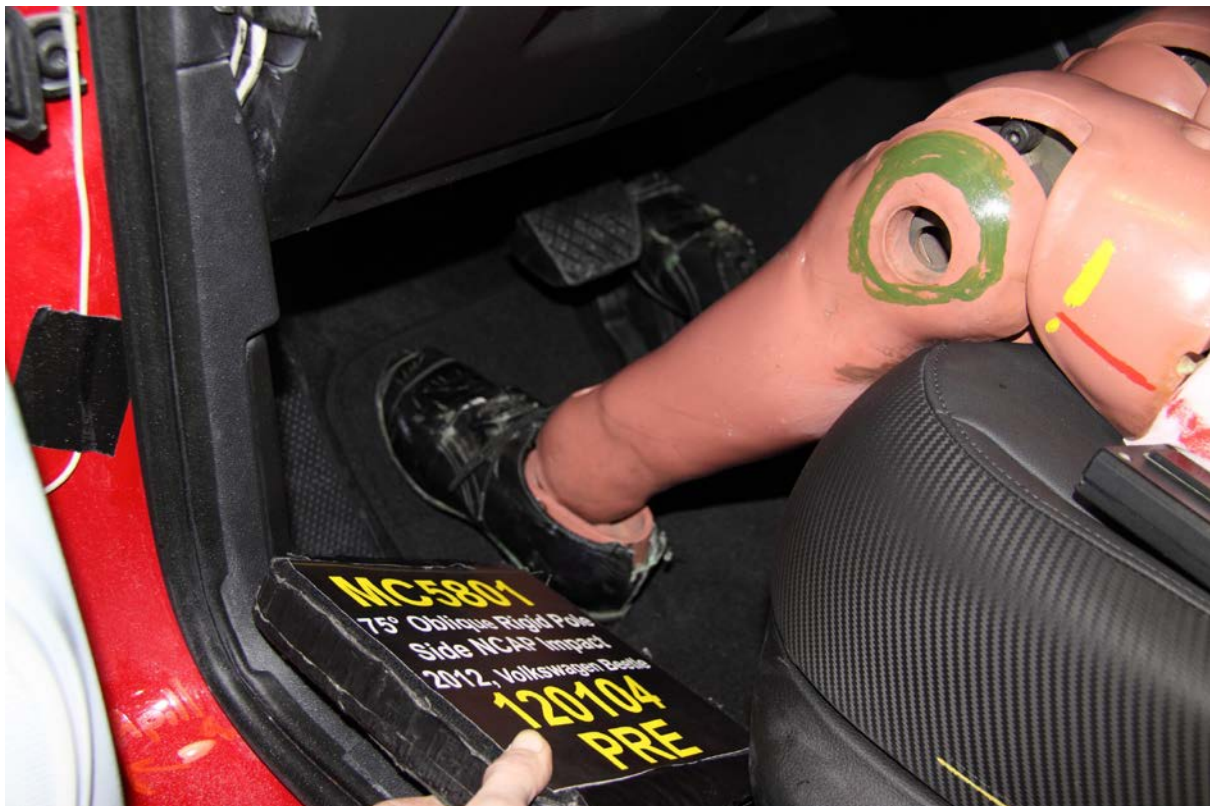
032 Pre-Test Placement of Dummy's Feet
