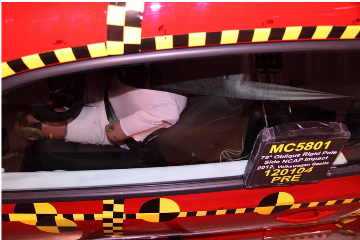
040 Pre-Test Dummy and Door Clearance View
