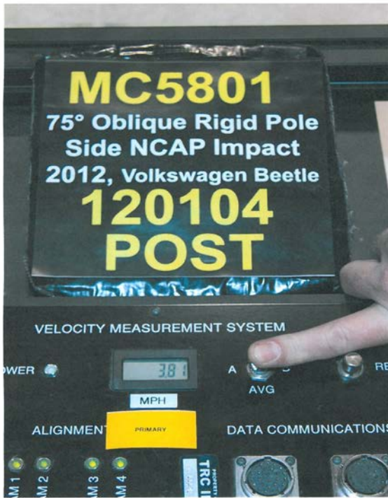
061 Post-Test Primary and Redundant Speed Trap Read-Out
