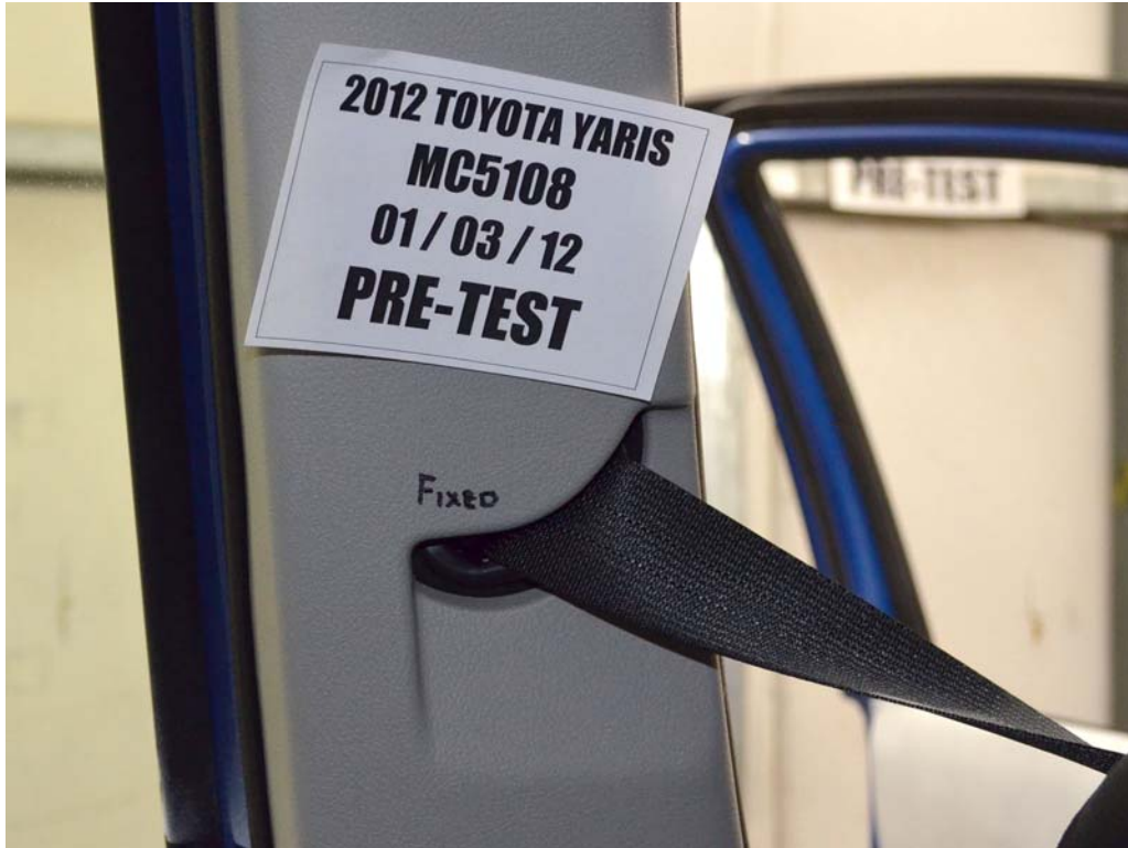
FIGURE 33. Pre-Test View of Belt Anchorage for Dummy
