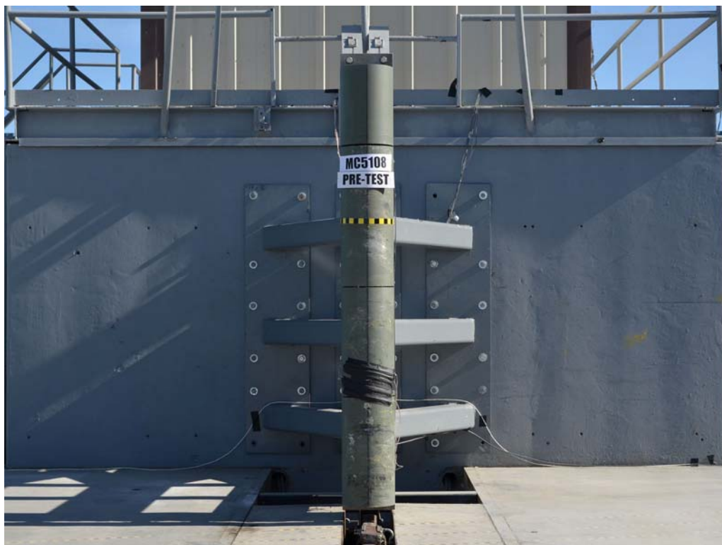
FIGURE 56. Pre-Test Pole Barrier Front View
