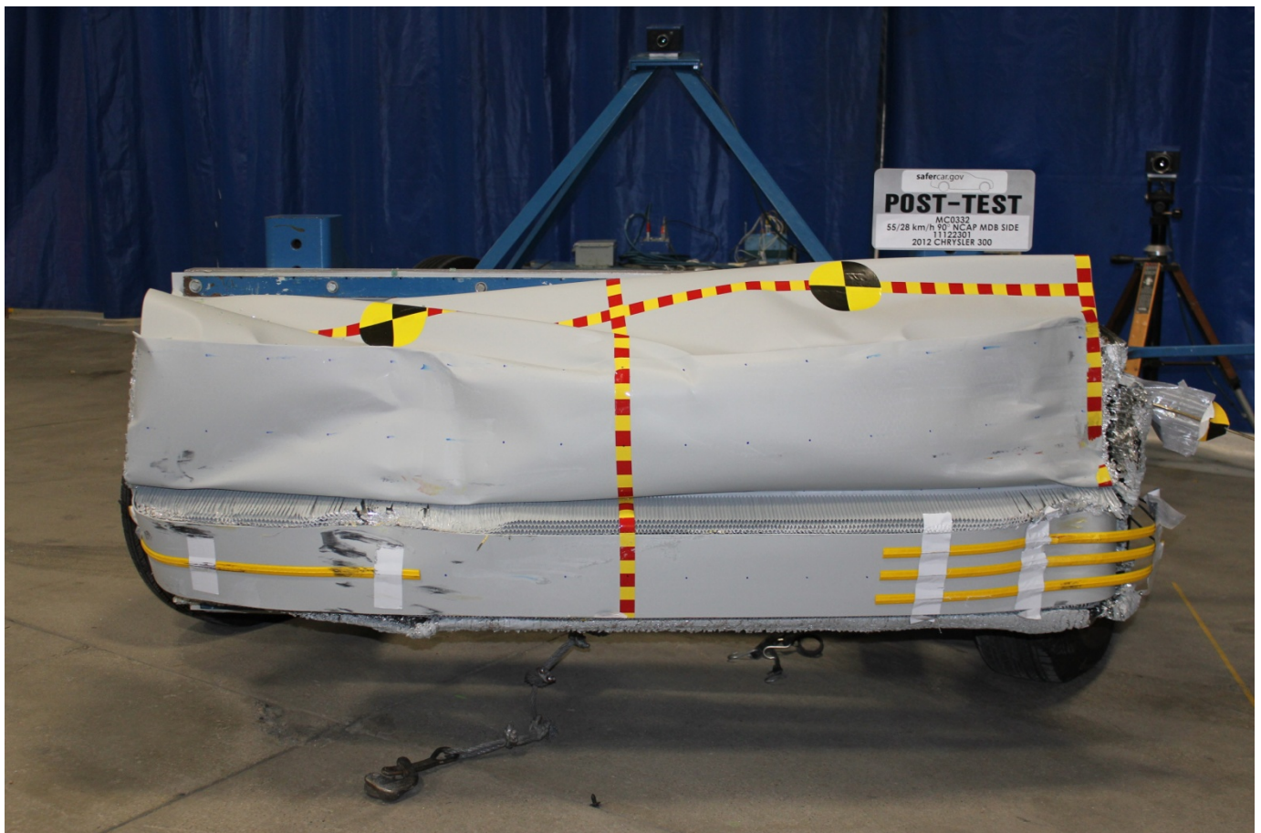
Post-Test Front View of MDB Impactor Face
