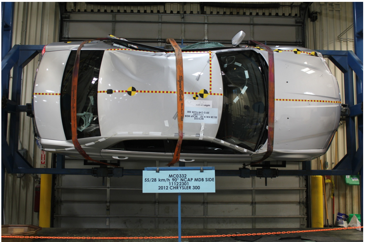
FMVSS No. 301 Static Rollover 270 Degrees
