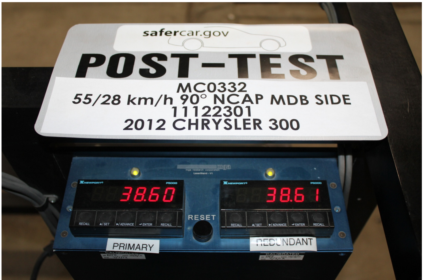
Post-Test Primary and Redundant Speed Trap Read-Out
