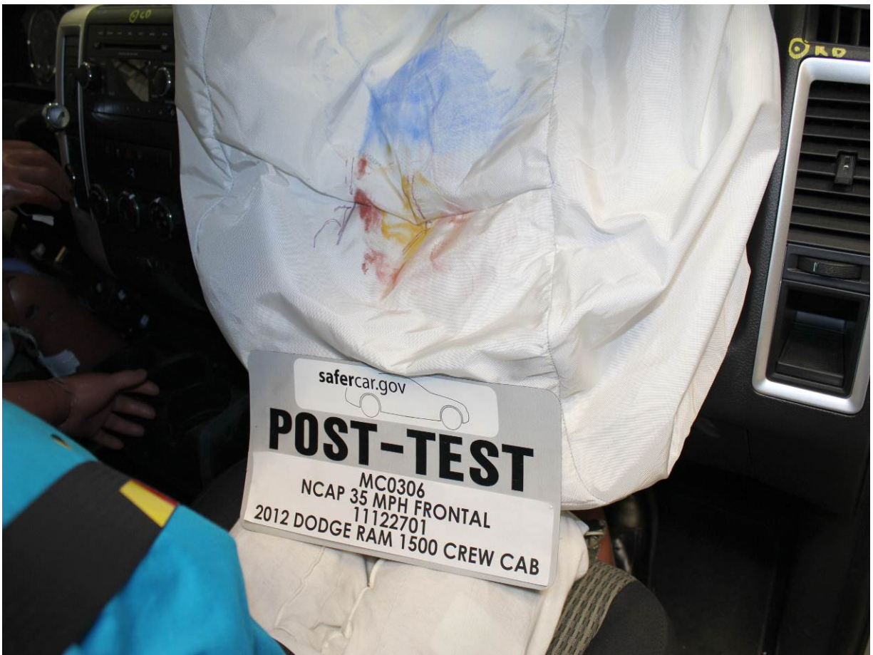
Post-Test Passenger Dummy Contact with Airbag
