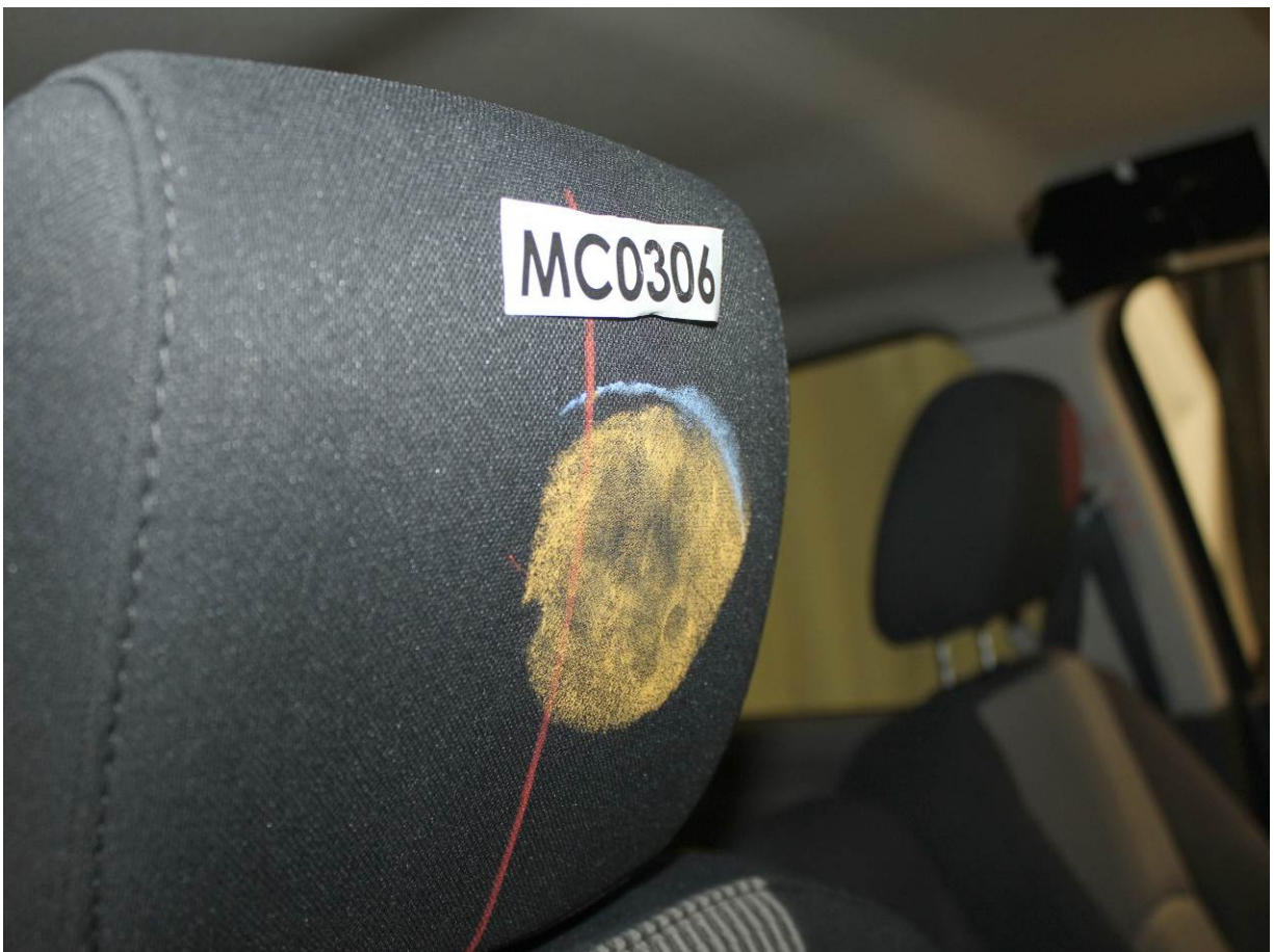
Post-Test Passenger Dummy Contact with Headrest
