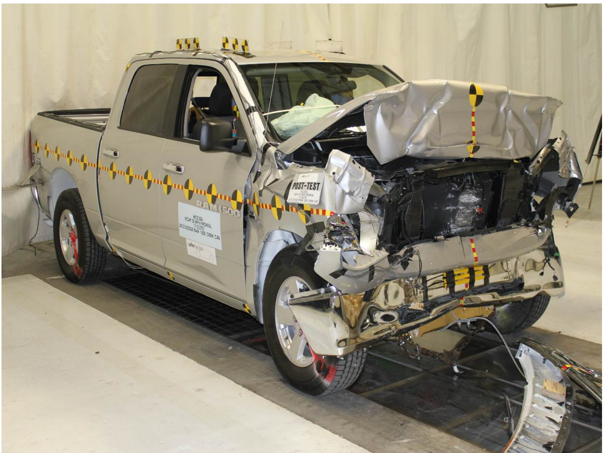
Post-Test Right Front Three-Quarter View
