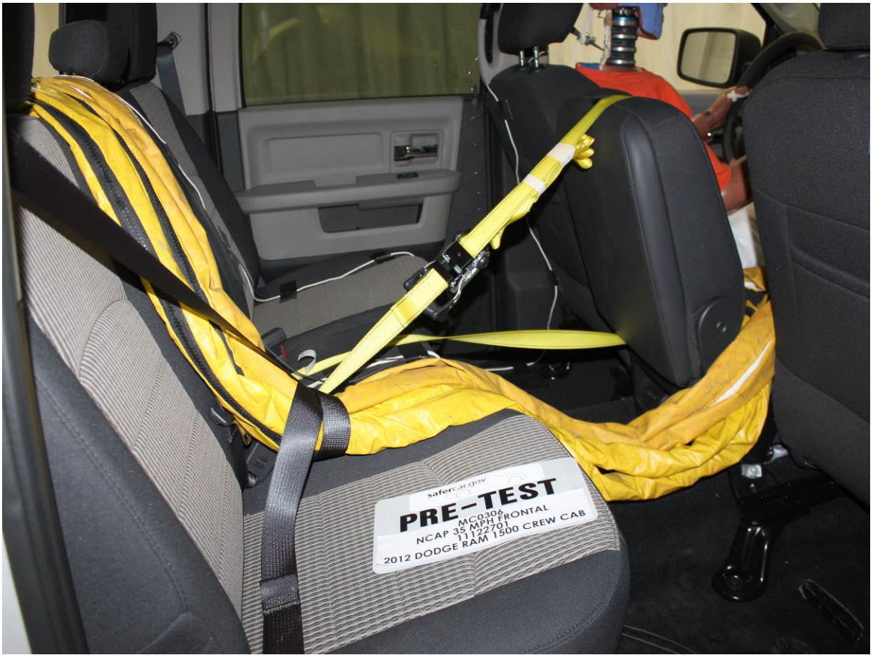
Pre-Test Dummy Cable Routing
