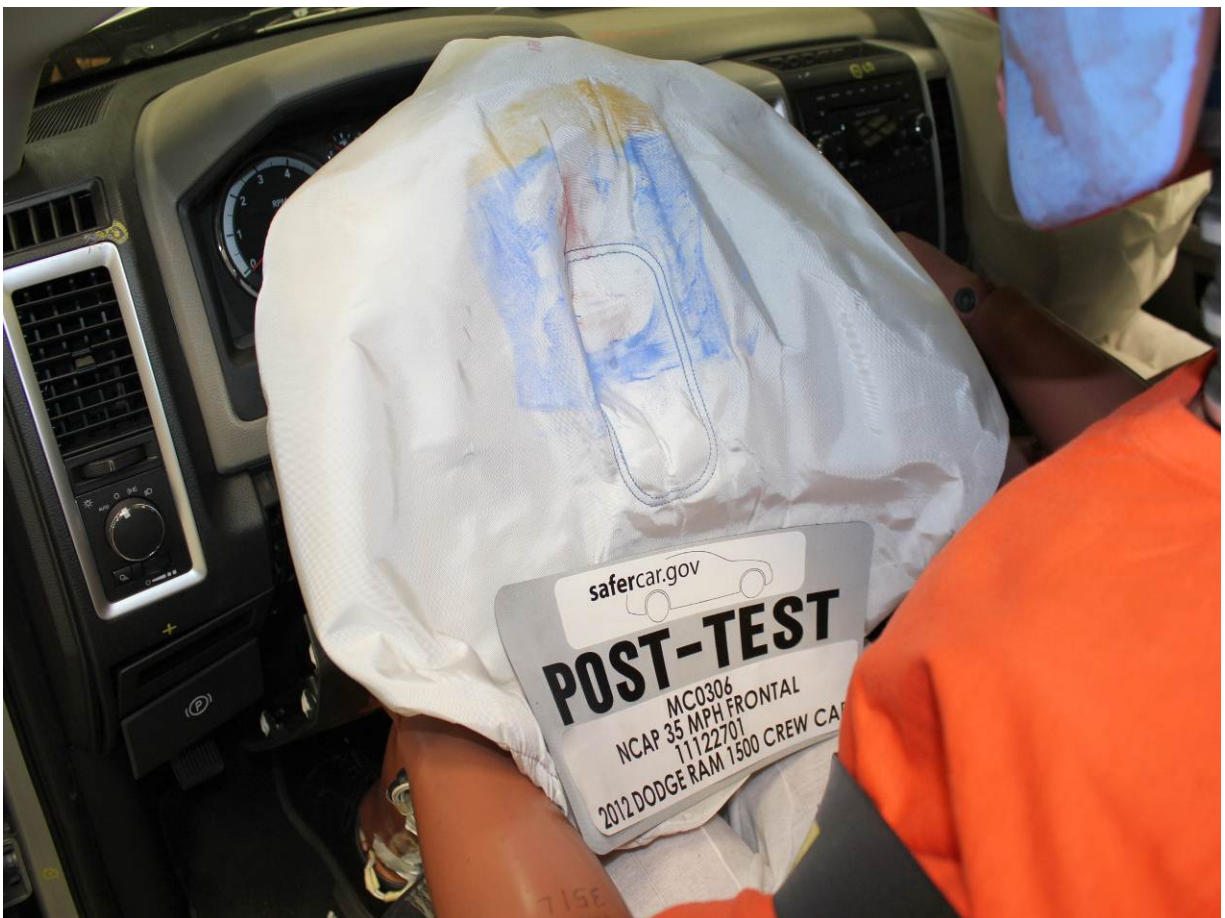
Post-Test Driver Dummy Contact with Airbag
