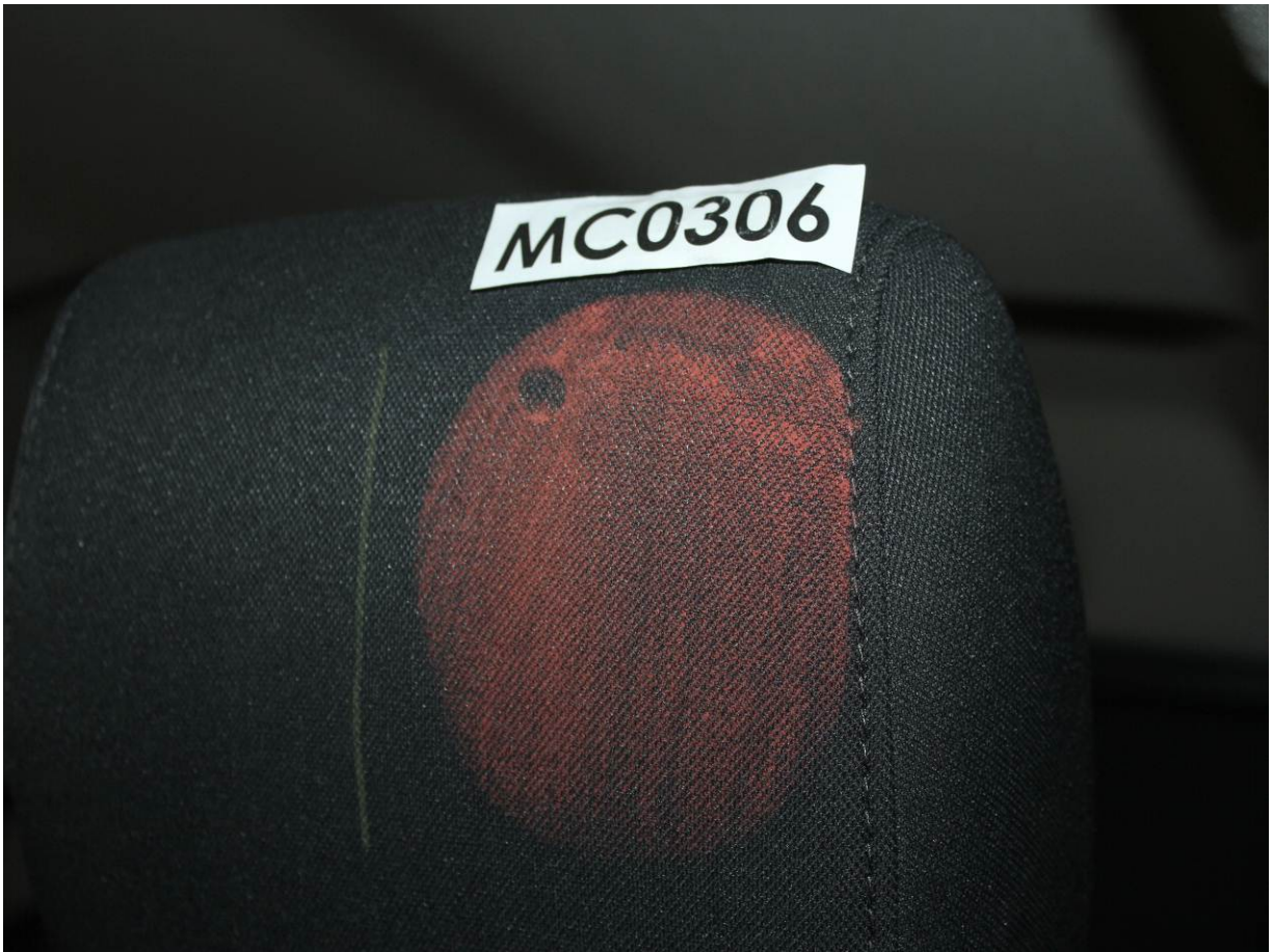
Post-Test Driver Dummy Contact with Headrest
