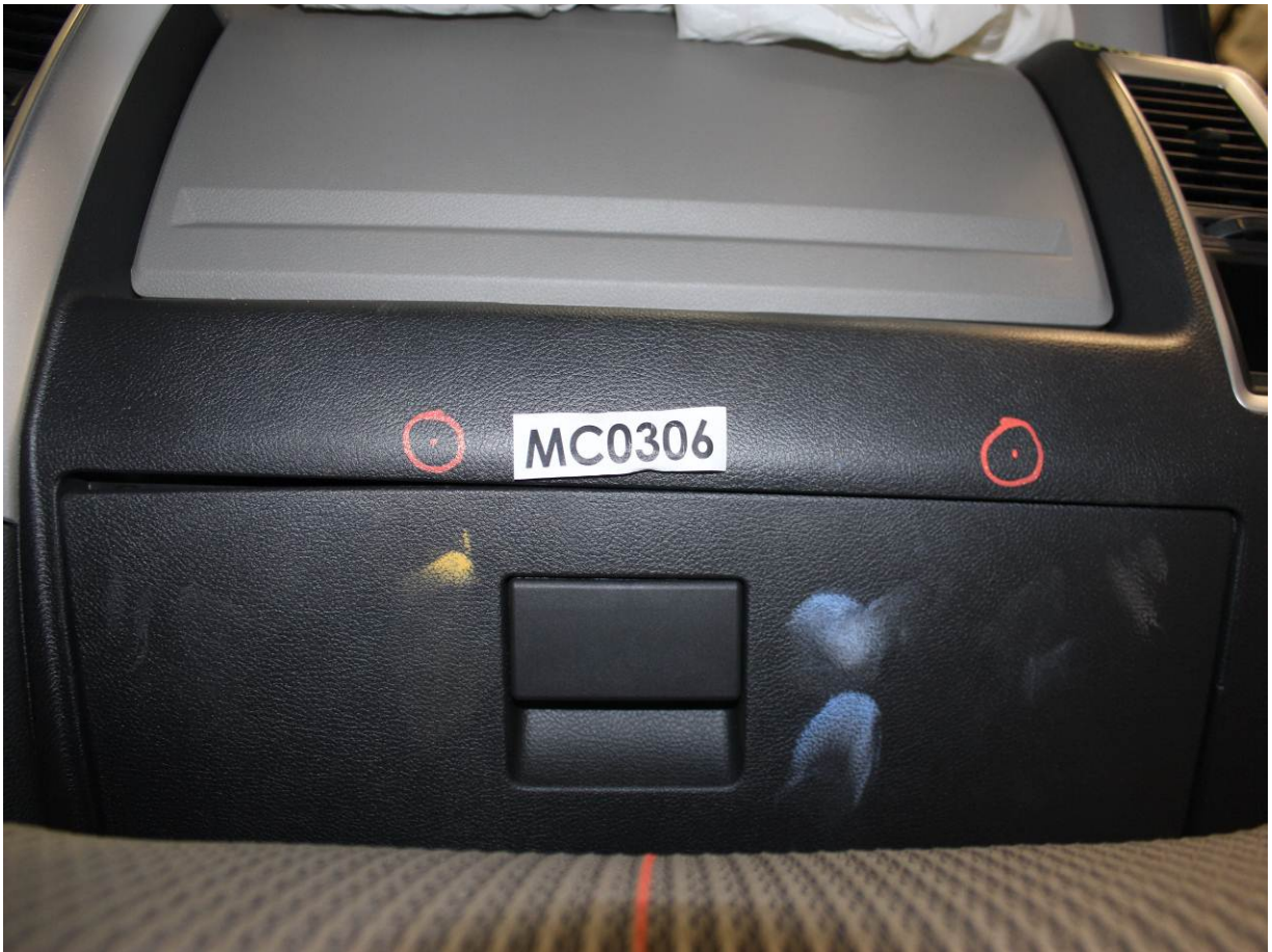
Post-Test Passenger Dummy Contact with Knee Bolster
