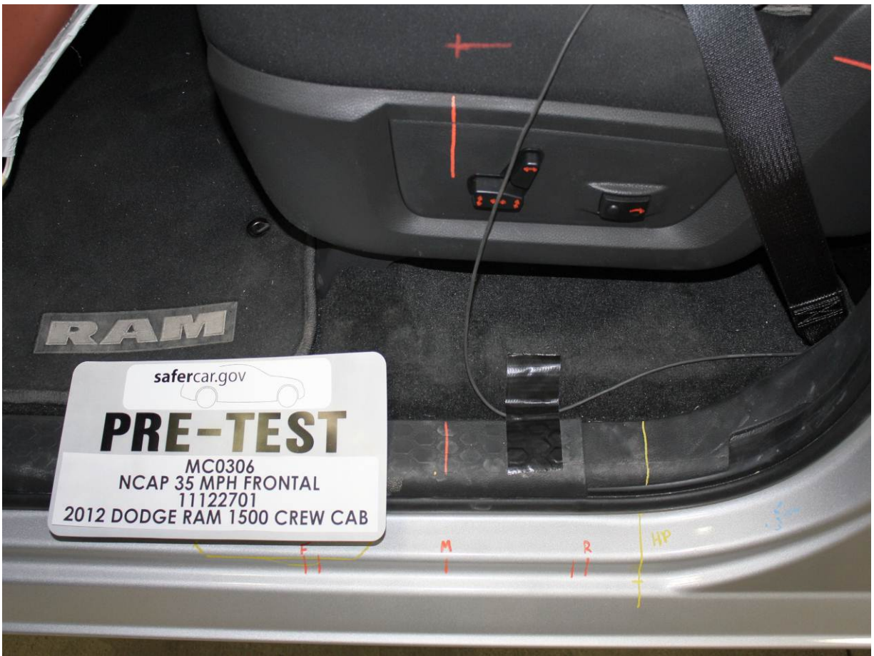
Pre-Test Driver's Seat Fore-Aft Markings
