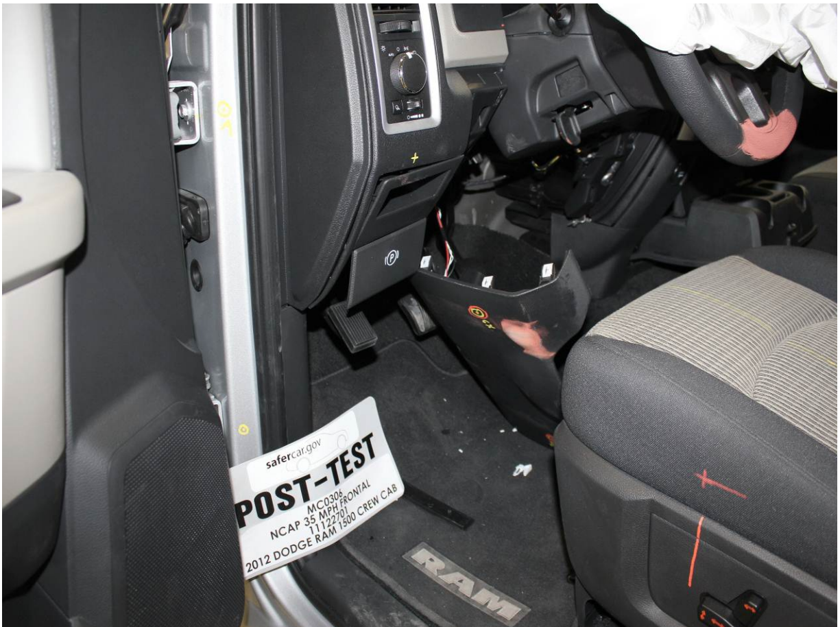
Post-Test Driver's Side Knee Bolster (without dummy)
