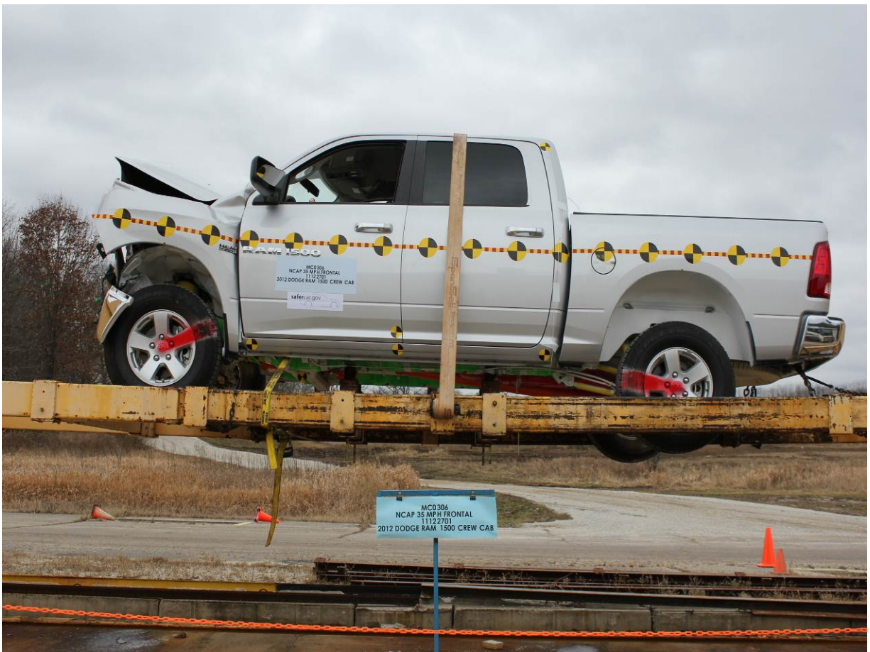
Vehicle at 0 Degrees on Static Rollover Device
