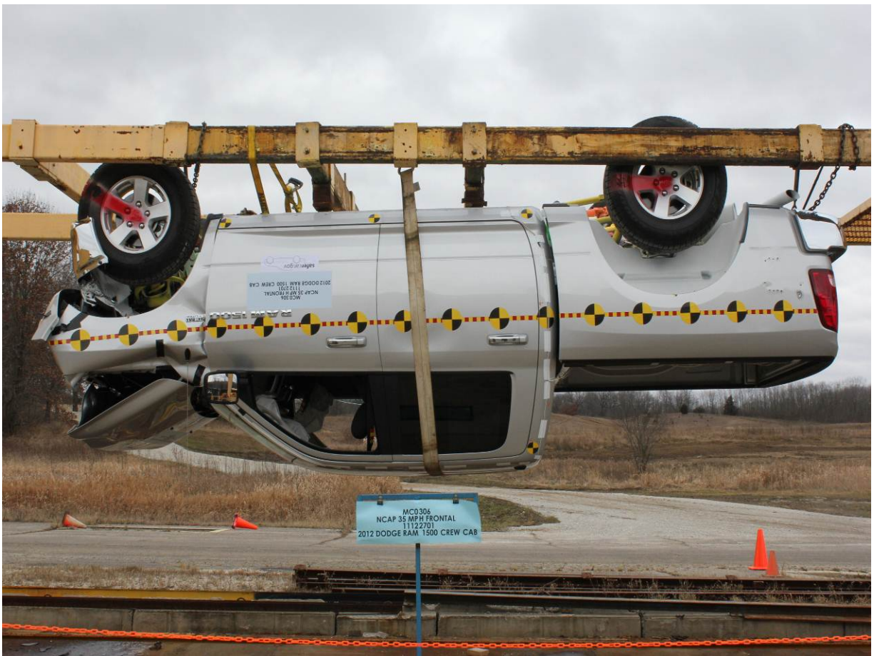
Vehicle at 180 Degrees on Static Rollover Device
