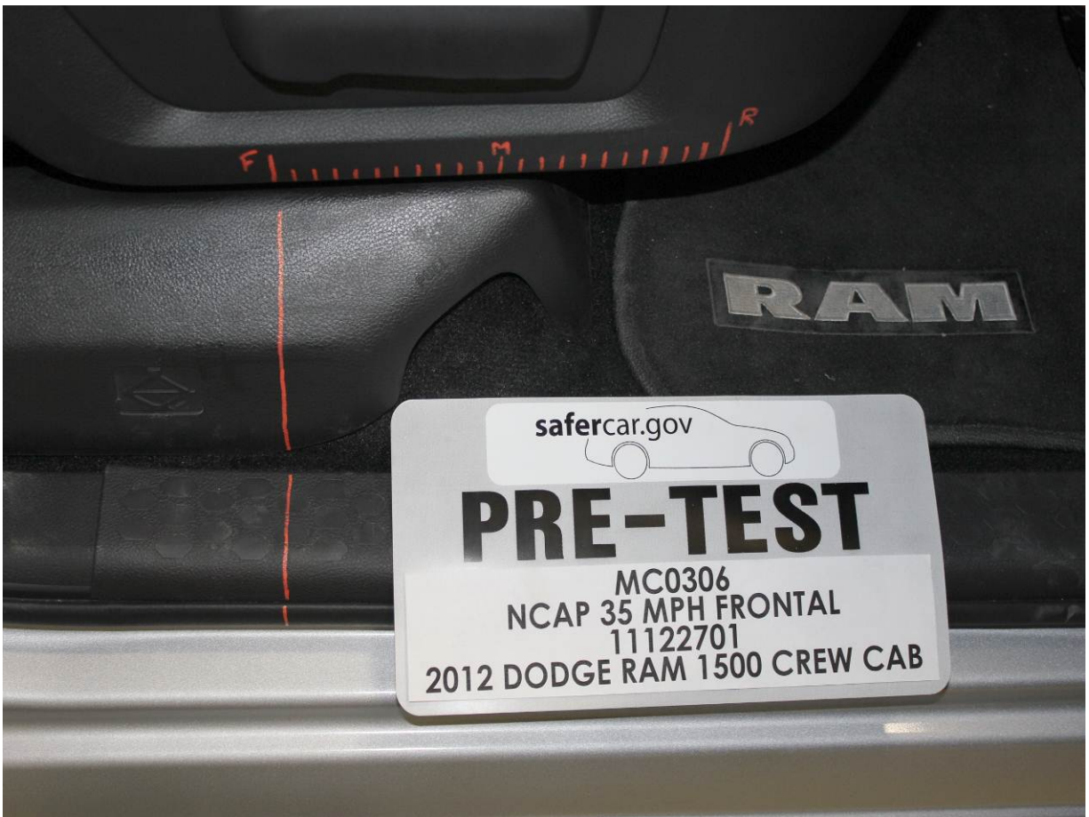
Pre-Test Passenger's Seat Fore-Aft Markings
