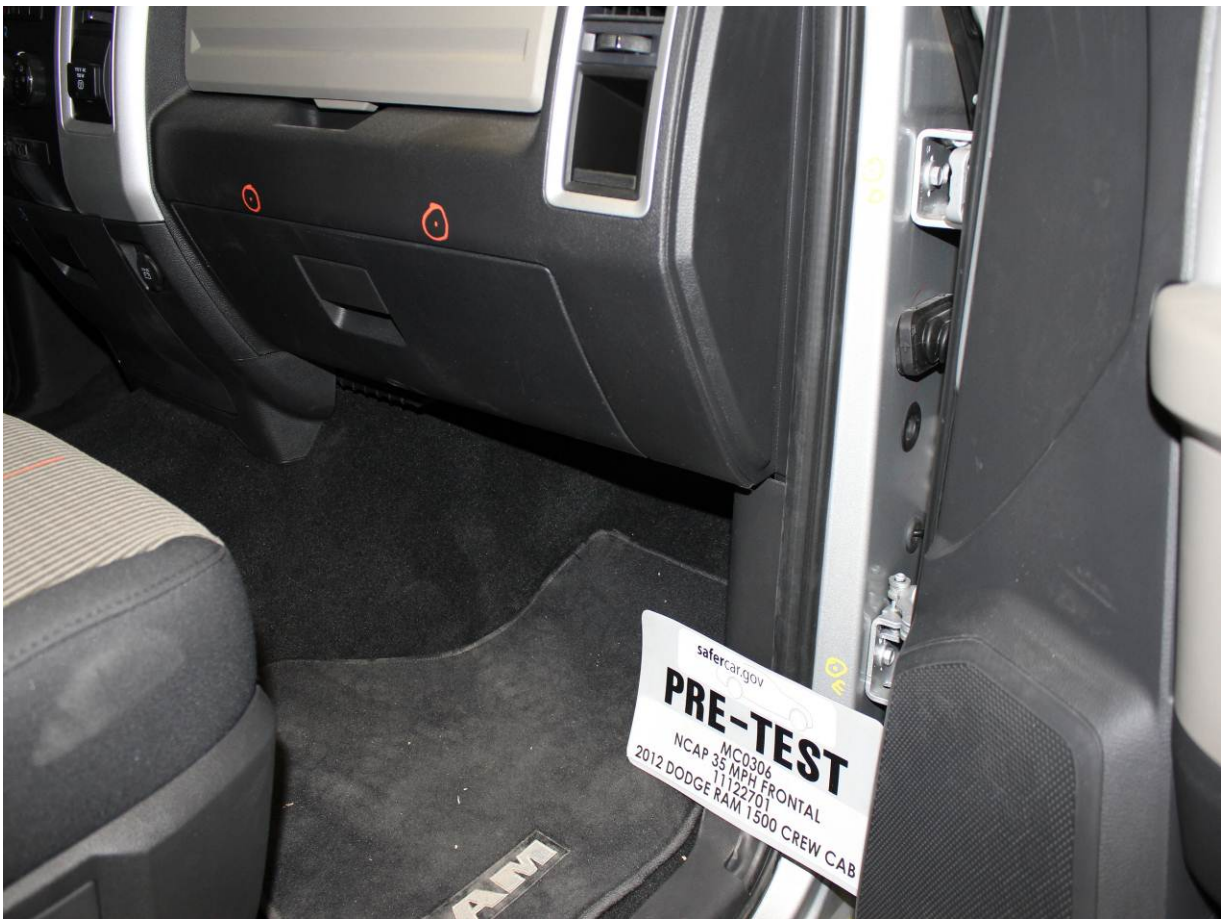
Pre-Test Passenger's Side Knee Bolster (without dummy)
