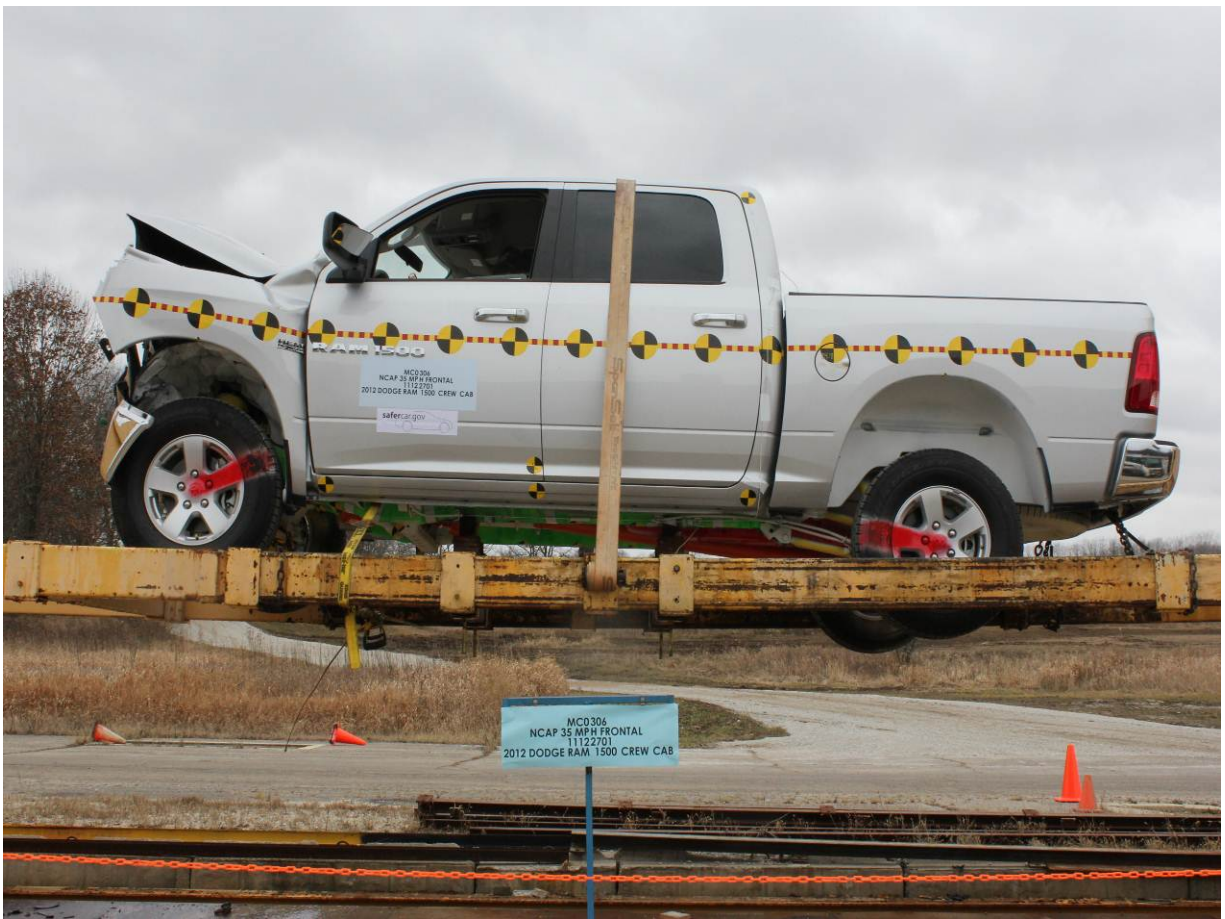
Vehicle at 360 Degrees on Static Rollover Device
