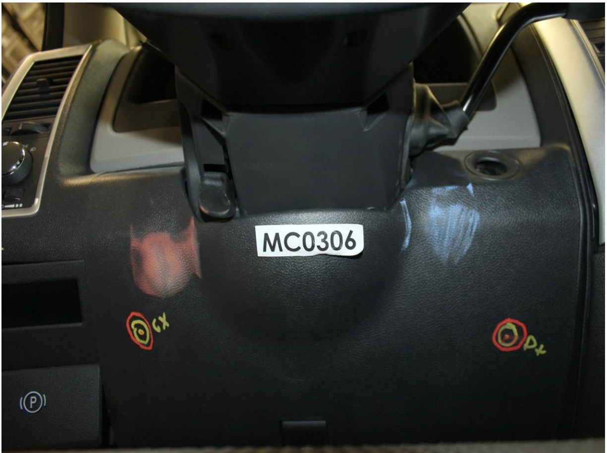
Post-Test Driver Dummy Contact with Knee Bolster
