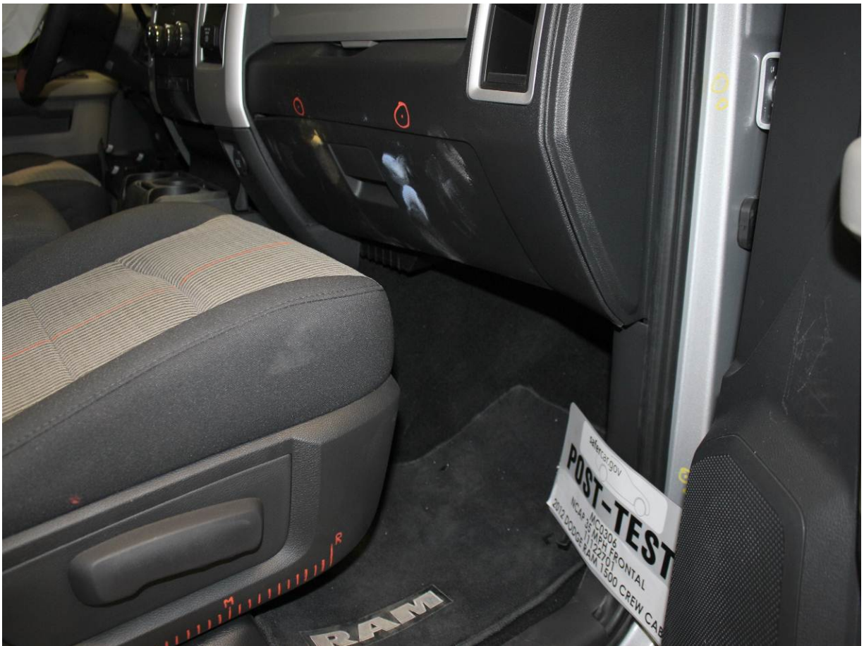
Post-Test Passenger's Side Knee Bolster (without dummy)
