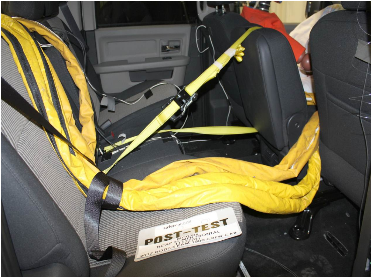
Post-Test Dummy Cable Routing
