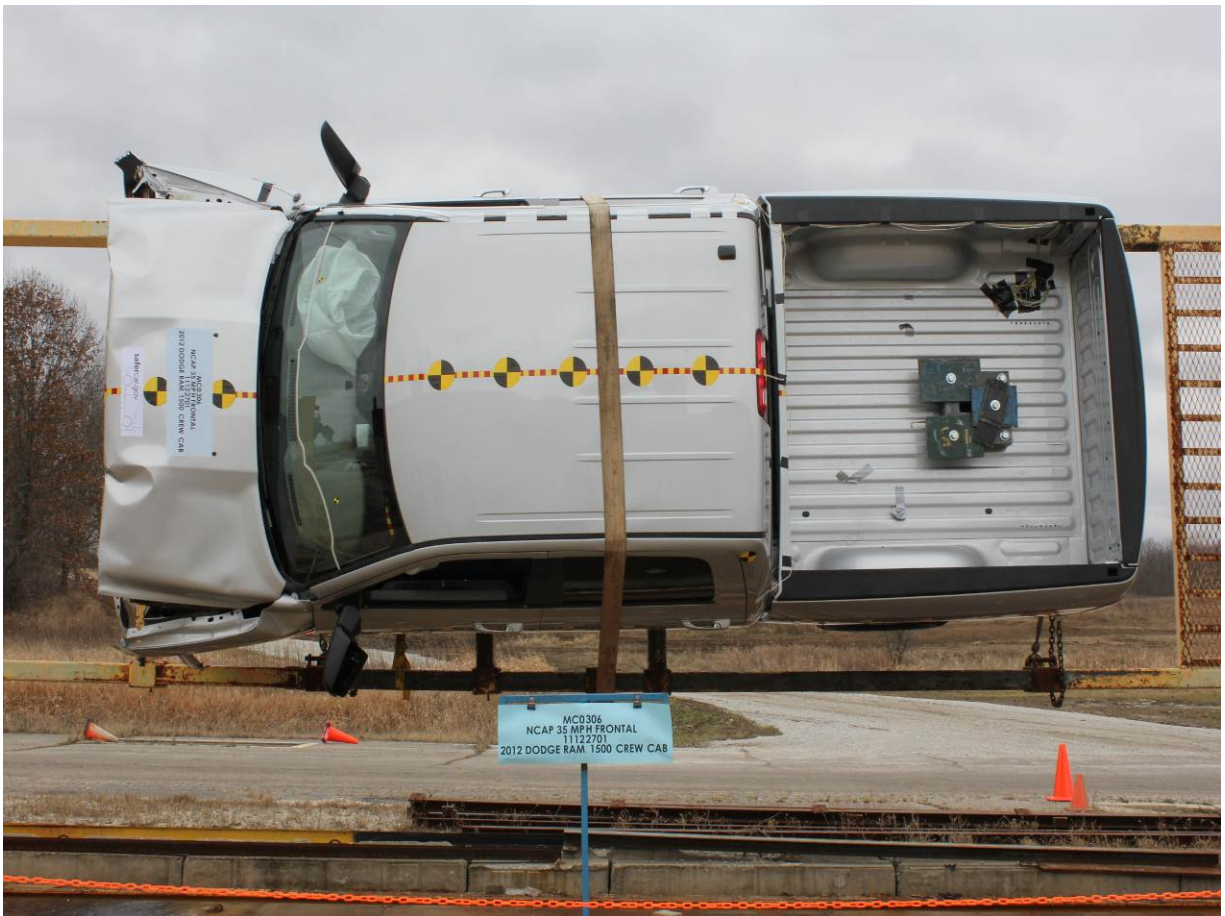
Vehicle at 90 Degrees on Static Rollover Device
