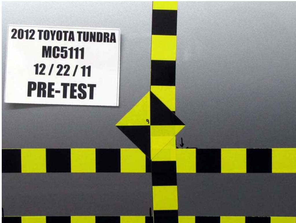
FIGURE 19. Pre-Test Close-Up View of Impact Point Target
