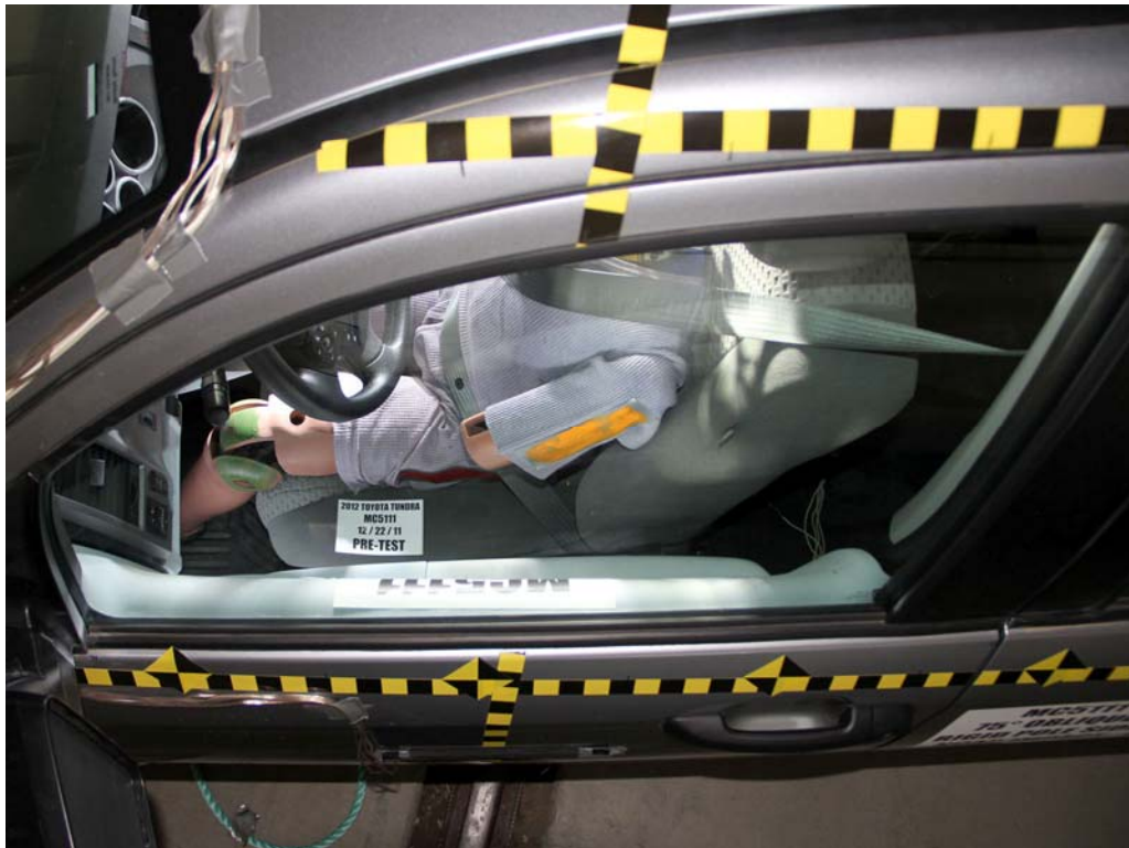
FIGURE 40. Pre-Test Driver Dummy and Door Clearance
