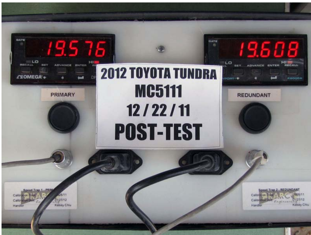
FIGURE 61. Post-Test Primary and Redundant Speed Trap Read-Out
