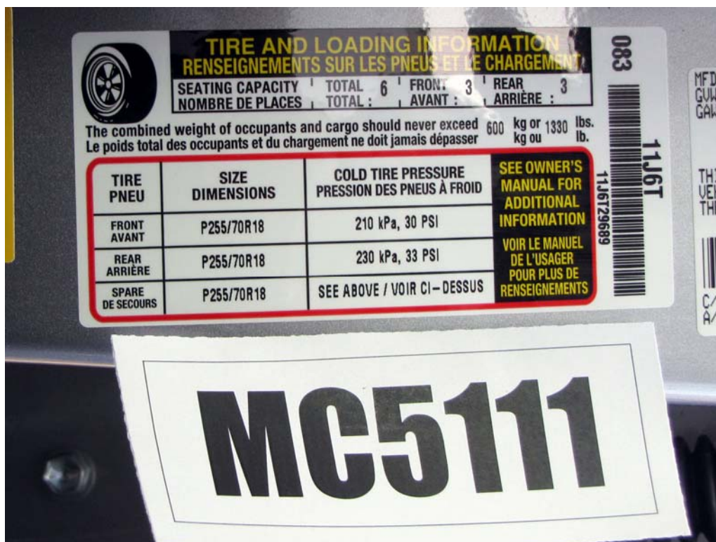
FIGURE 55. Close-Up View of Vehicle's Tire Information Placard
