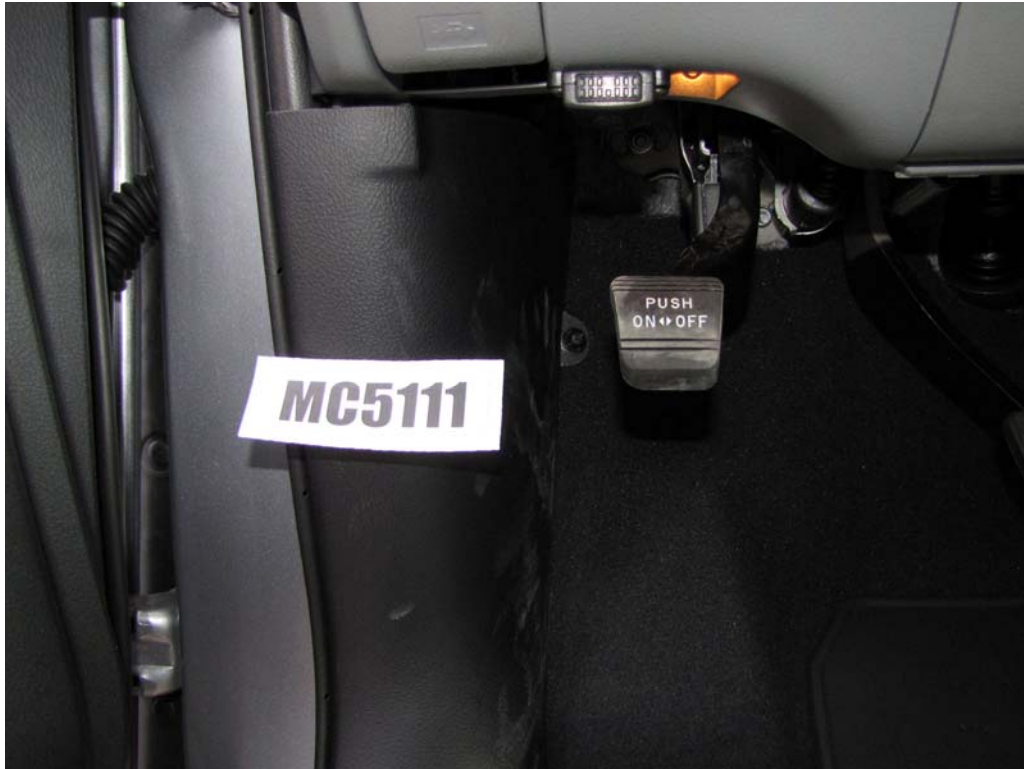
FIGURE 35. View of Disengaged Parking Brake
