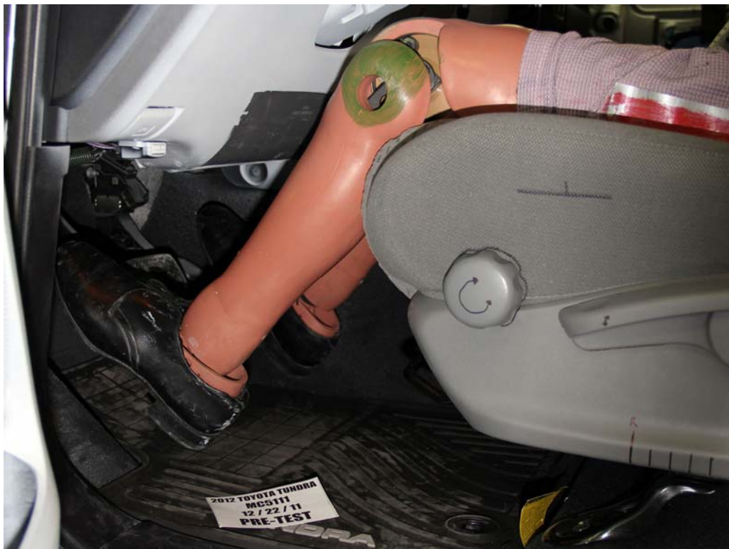
FIGURE 32. Pre-Test Placement of Dummy's Feet
