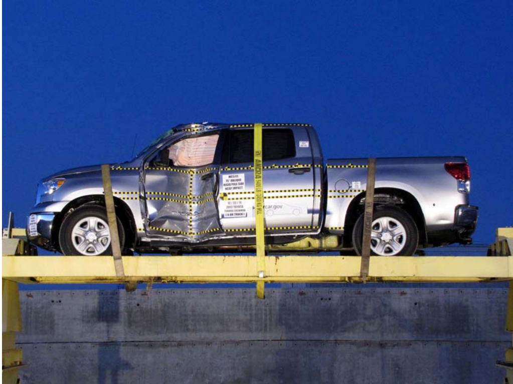
FIGURE 62. FMVSS No. 301-305 Rollover 0 Degrees
