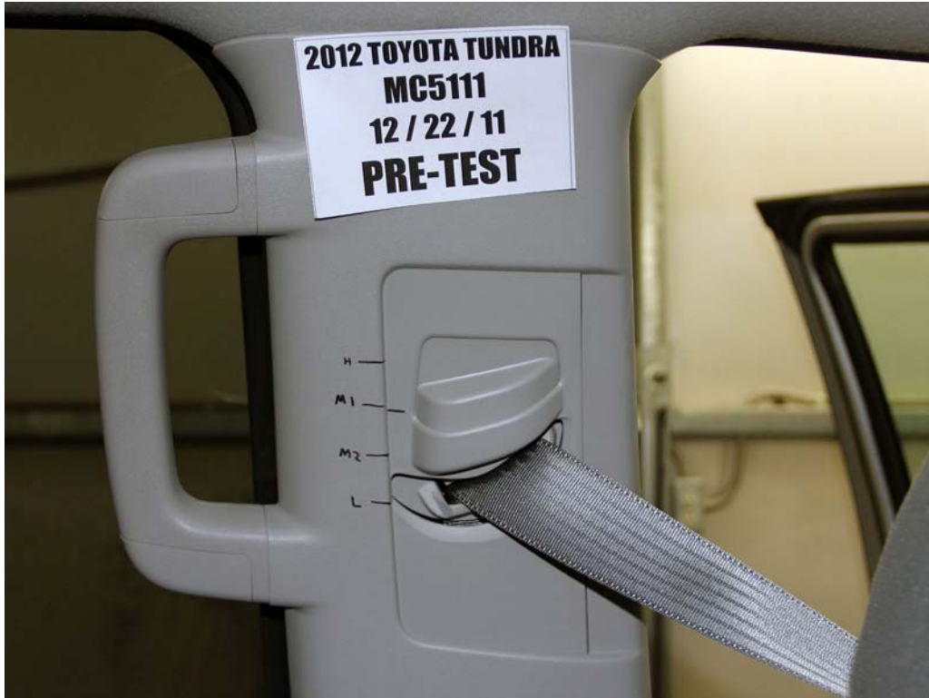
FIGURE 33. Pre-Test View of Belt Anchorage for Dummy
