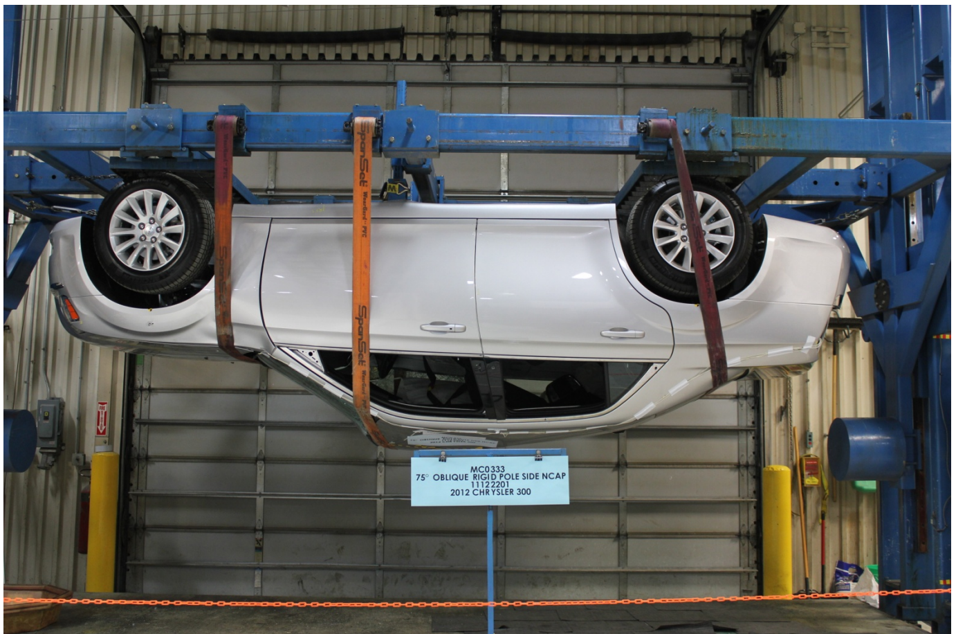
FMVSS No. 301 Static Rollover 180 Degrees
