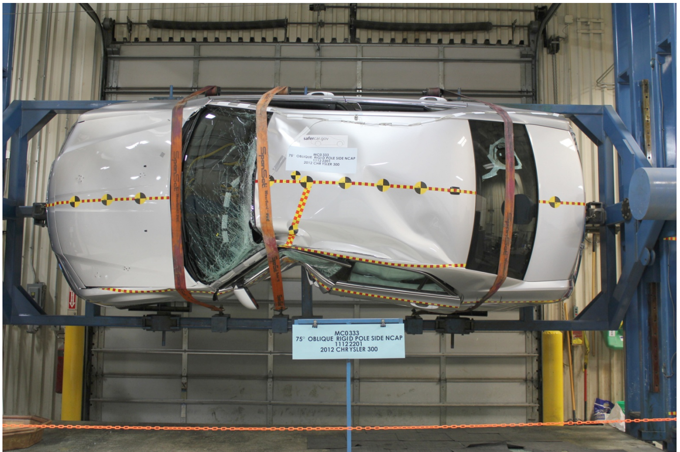
FMVSS No. 301 Static Rollover 90 Degrees
