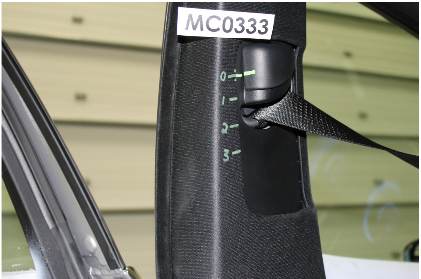
Pre-Test View of Belt Anchorage for Dummy
