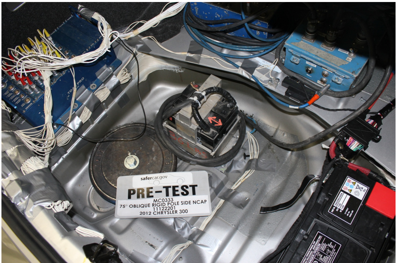
Pre-Test Ballast View
