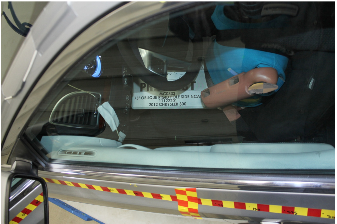
Pre-Test Dummy and Door Clearance View
