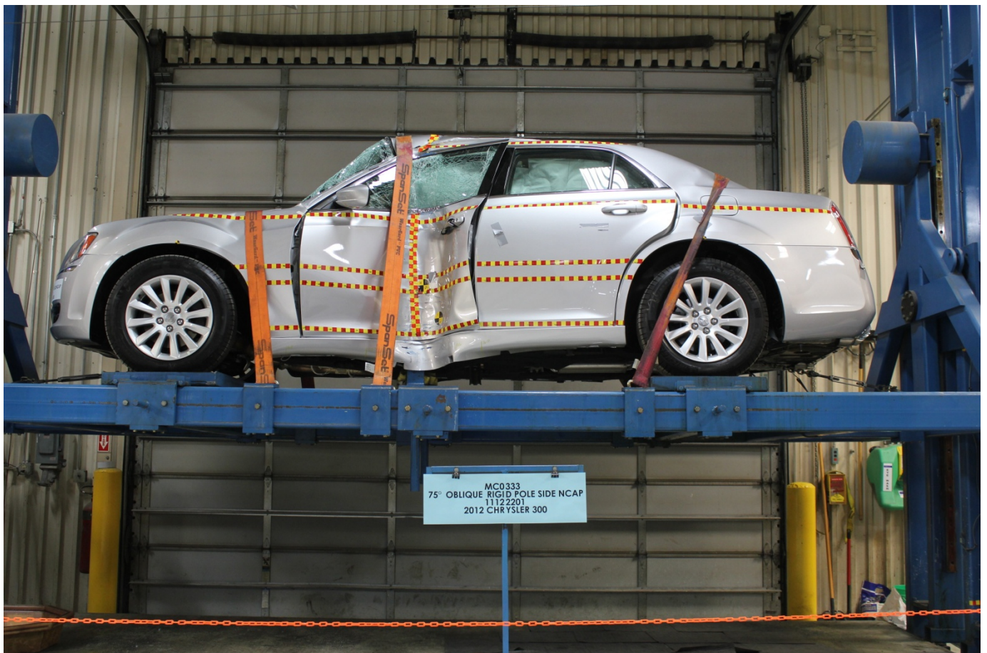
FMVSS No. 301 Static Rollover 0 Degrees
