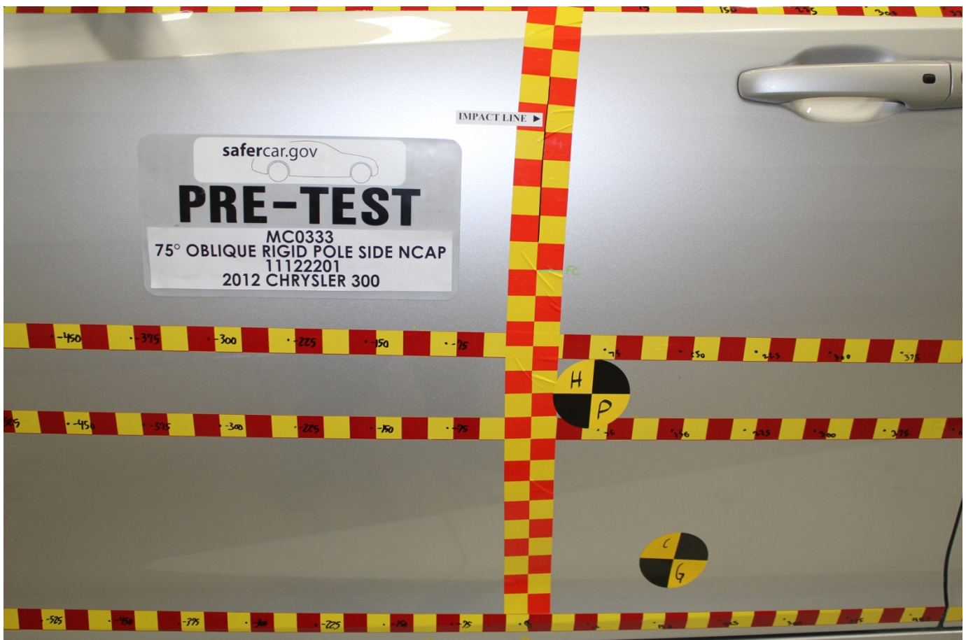
Pre-Test Close-Up View of Impact Point Target
