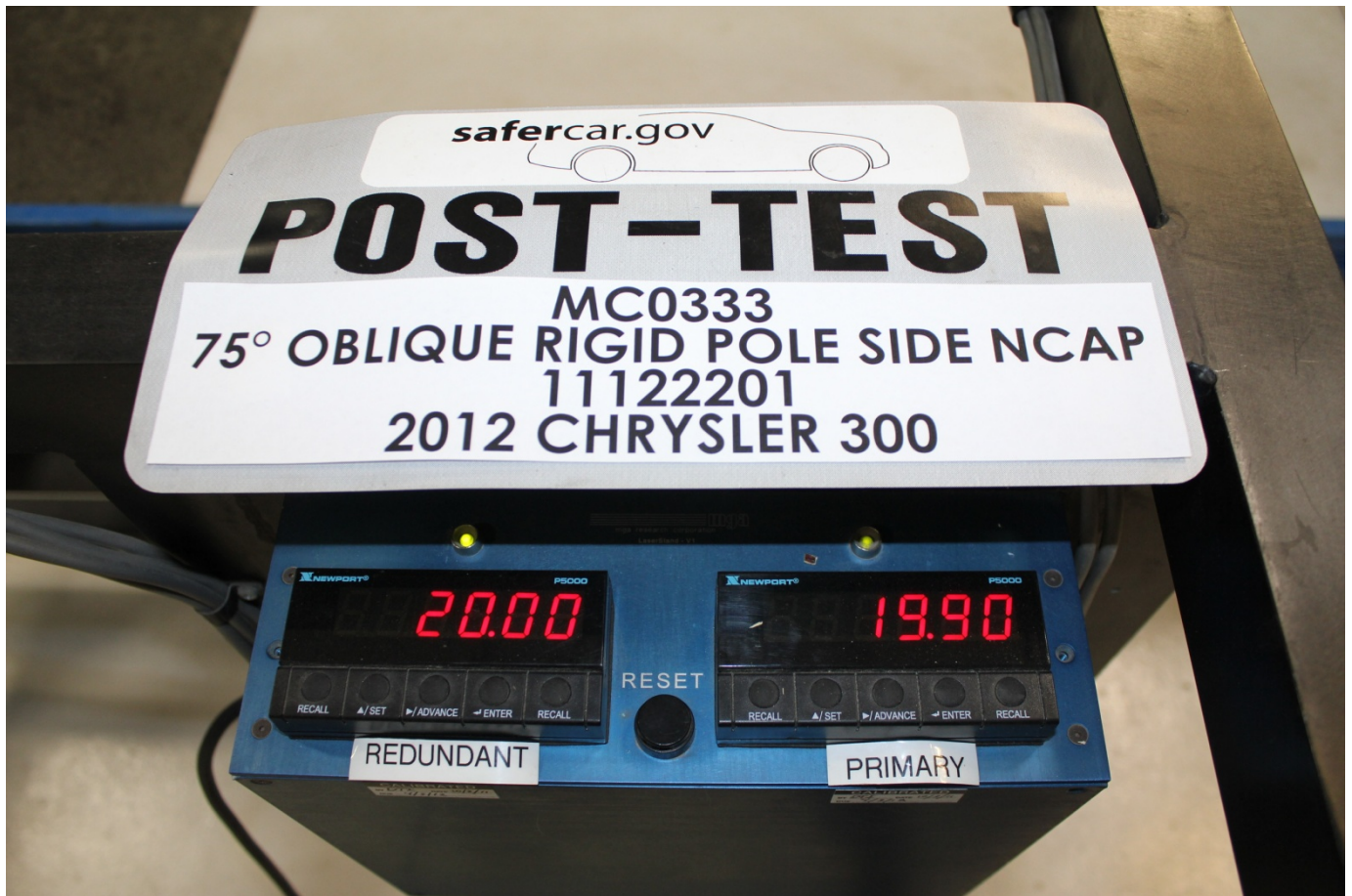
Post-Test Primary and Redundant Speed Trap Read-Out
