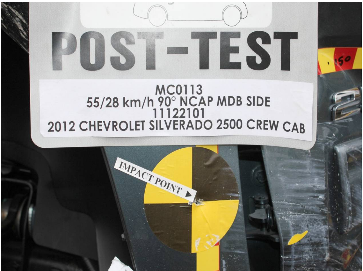
Post-Test Close-Up View of Impact Point Target
