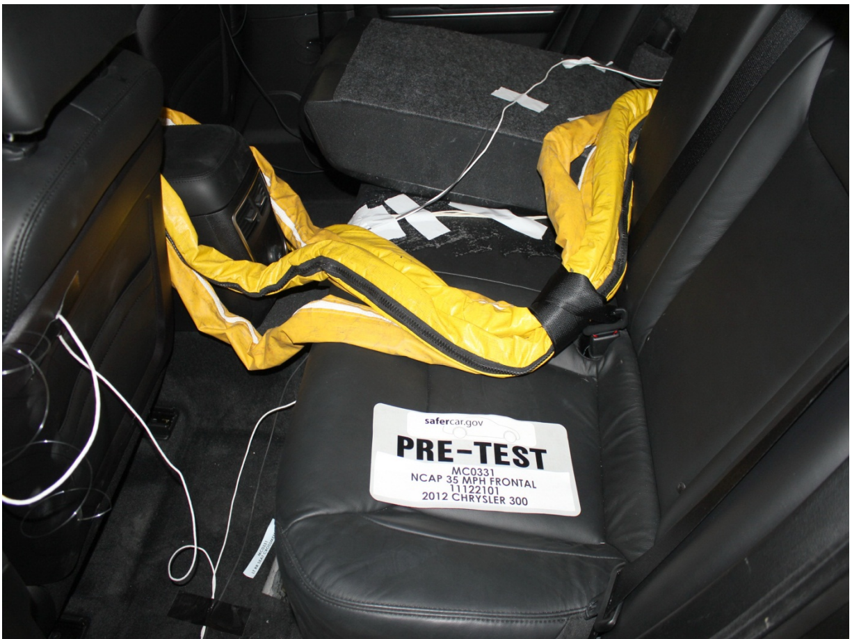
Pre-Test Dummy Cable Routing
