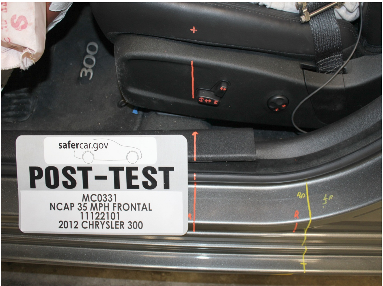
Post-Test Driver's Seat Fore-Aft Markings
