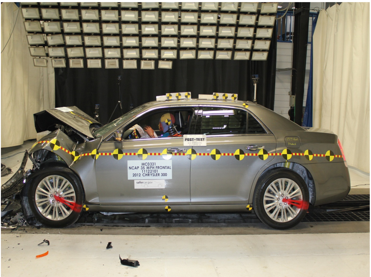
Post-Test Left View of Test Vehicle
