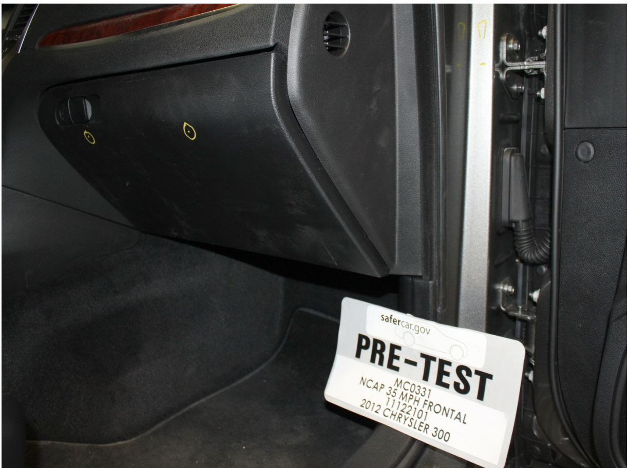
Pre-Test Passenger's Side Knee Bolster (without dummy)
