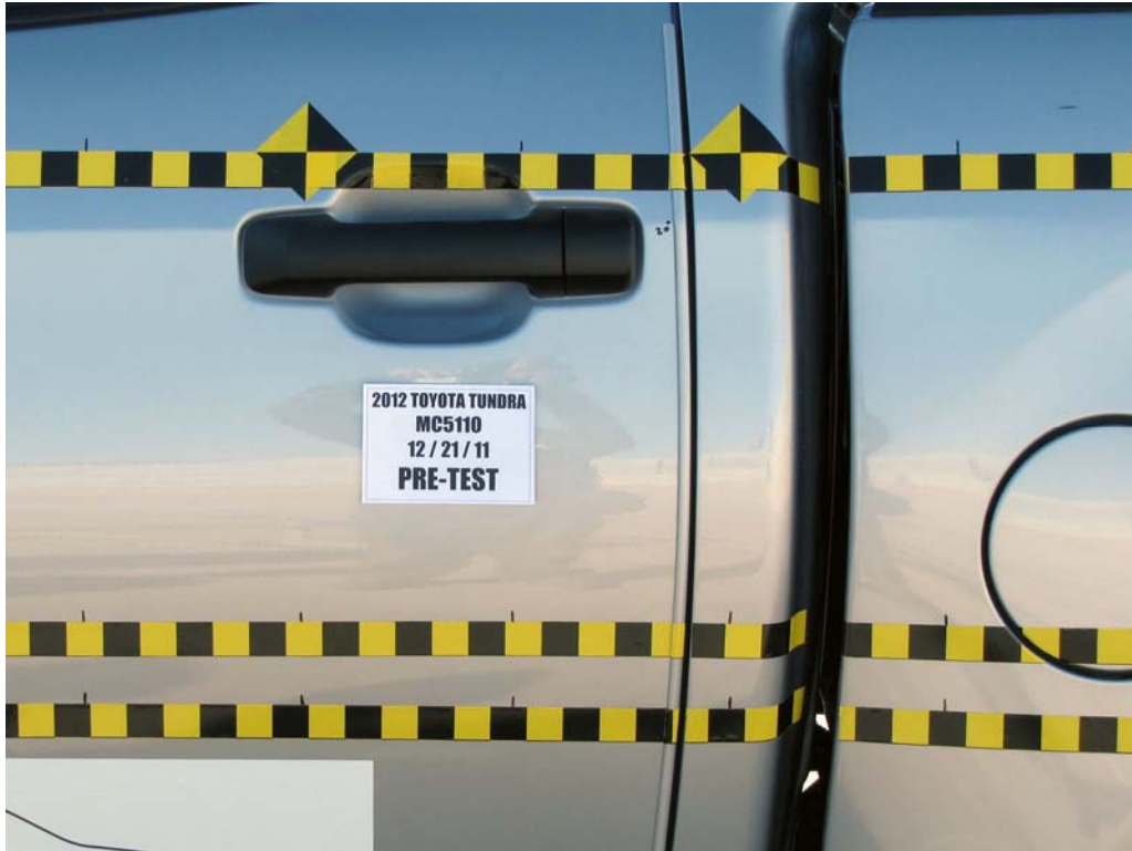
FIGURE 23. Pre-Test Left Rear Door Latch Close-Up
