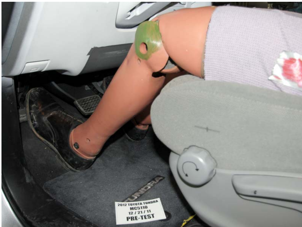
FIGURE 34. Pre-Test Placement of Driver Dummy's Feet
