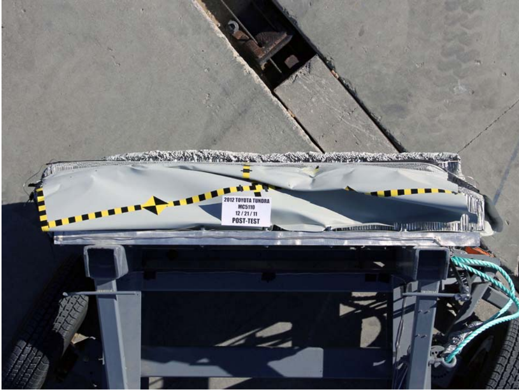
FIGURE 85. Post-Test Top View of MDB Impactor Face
