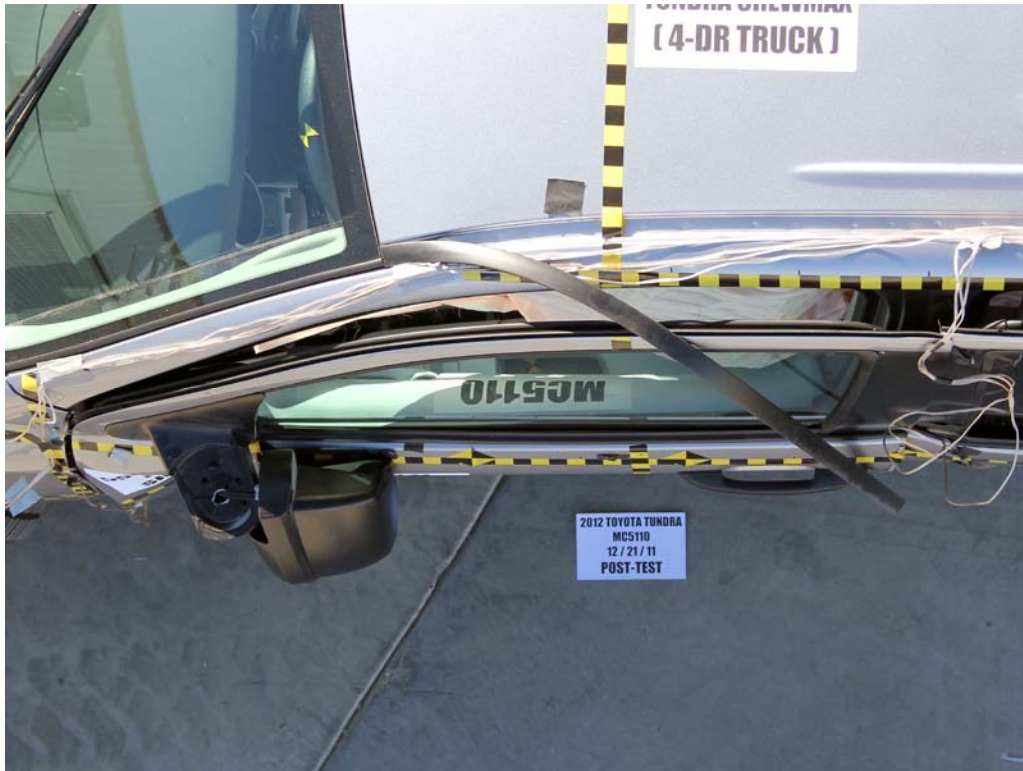
FIGURE 43. Post-Test Driver Dummy and Door Clearance View
