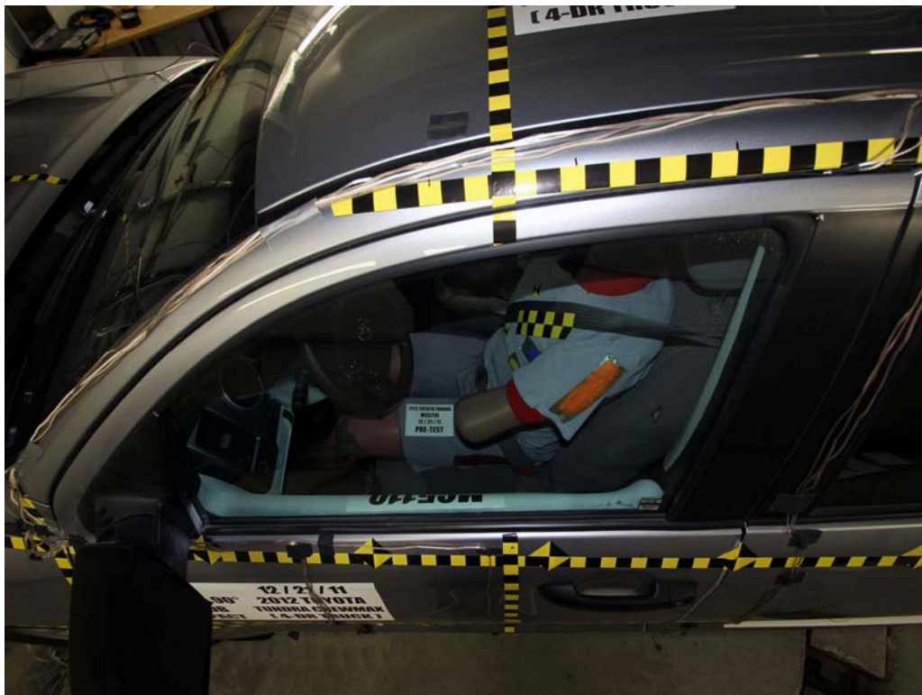
FIGURE 42. Pre-Test Driver Dummy and Door Clearance View
