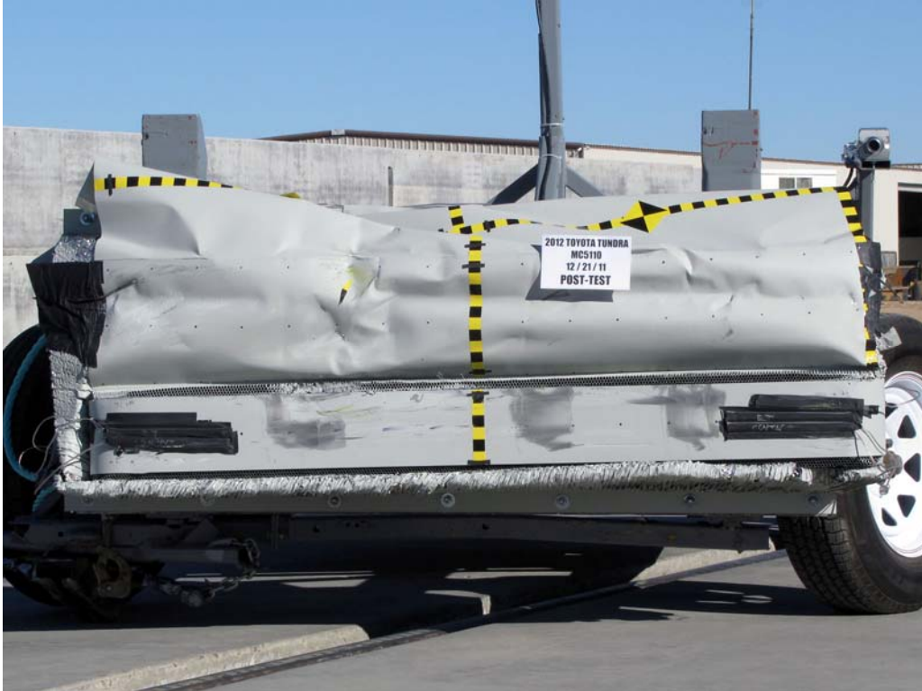
FIGURE 83. Post-Test Front View of MDB Impactor Face
