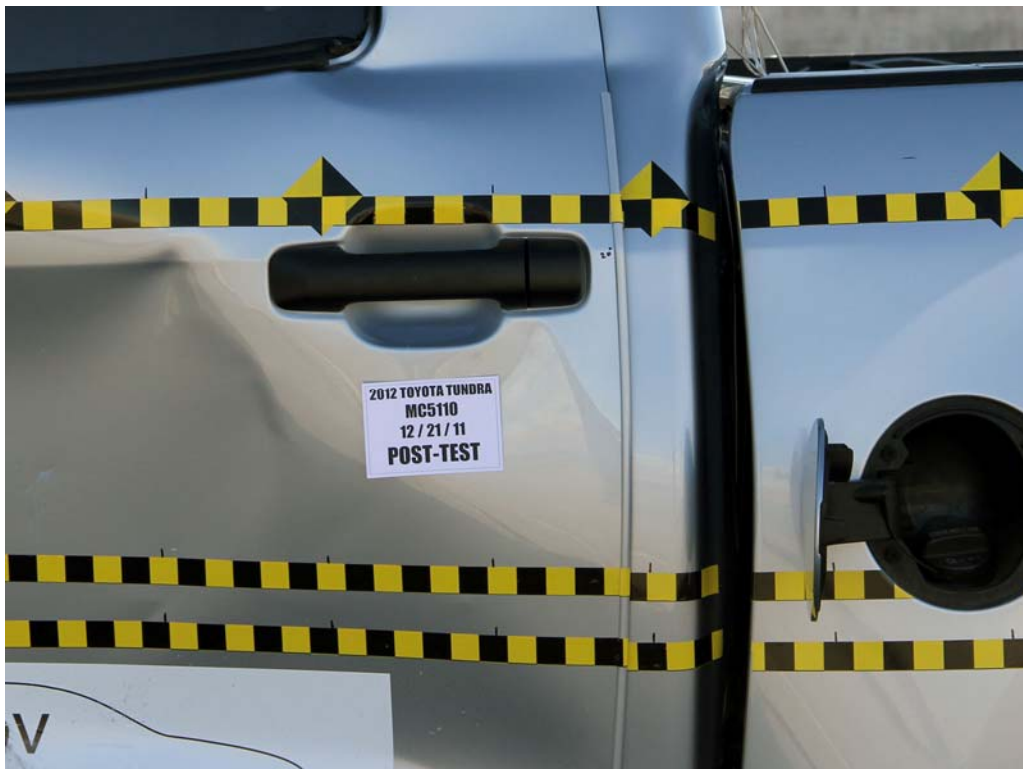
FIGURE 24. Post-Test Left Rear Door Latch Close-Up
