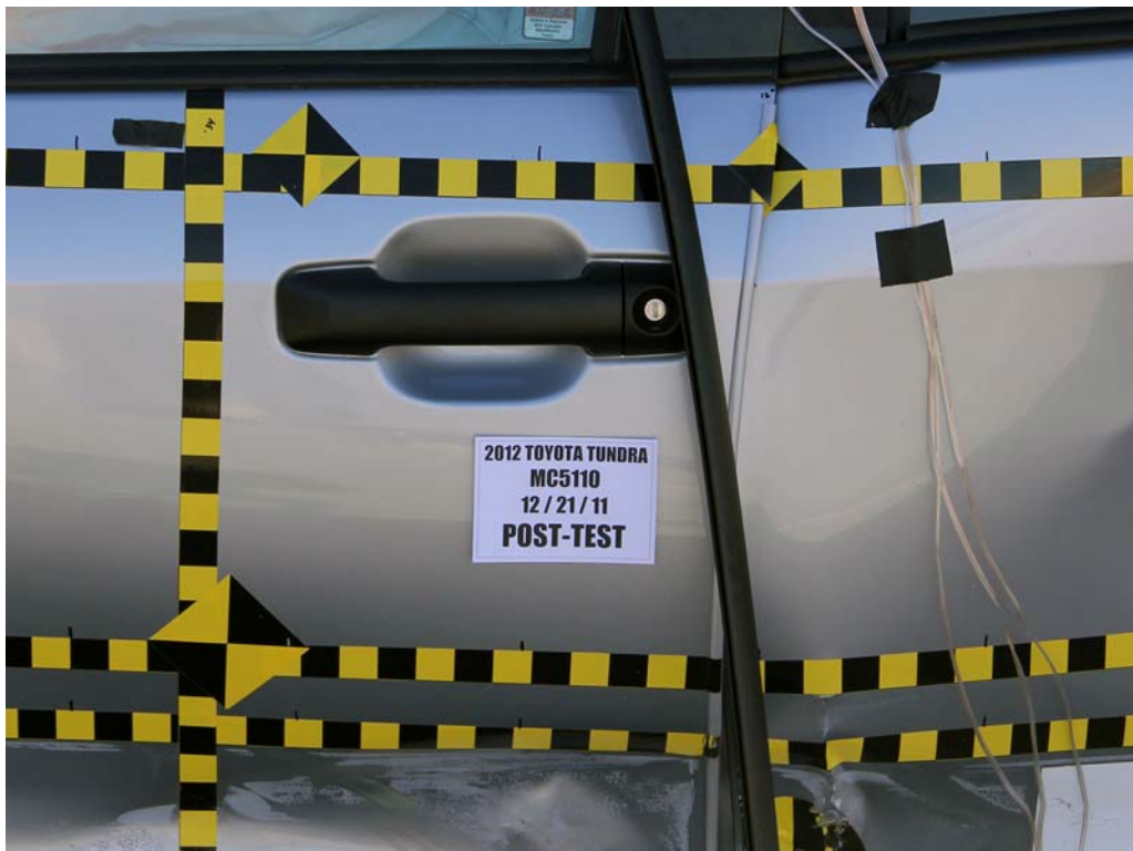
FIGURE 22. Post-Test Left Front Door Latch Close-Up
