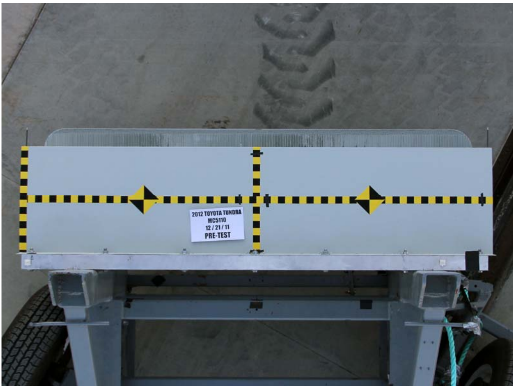
FIGURE 84. Pre-Test Top View of MDB Impactor Face
