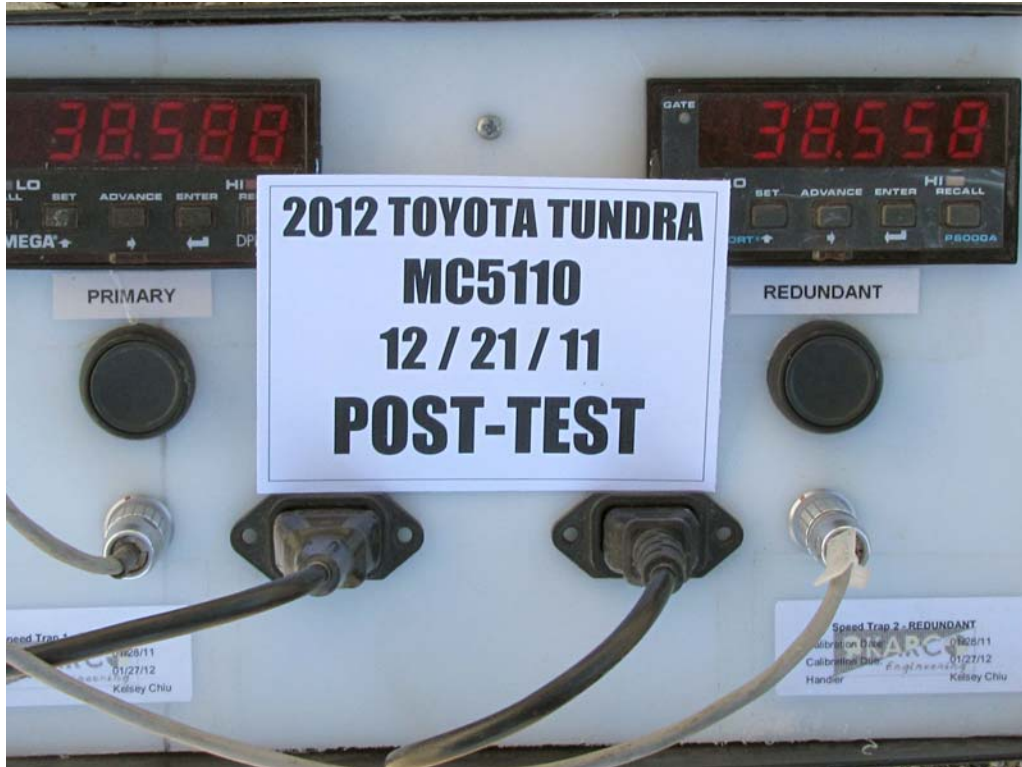
FIGURE 93. Post-Test Primary and Redundant Speed Trap Read-Out
