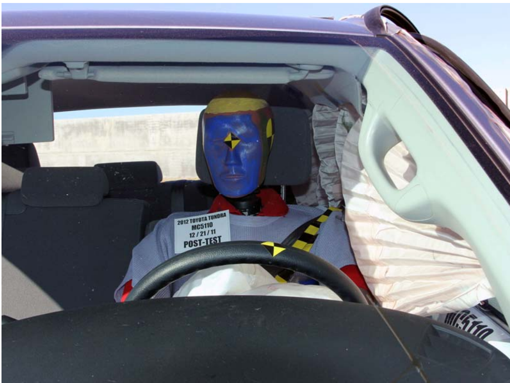
FIGURE 26. Post-Test Front Close-Up View of Driver Dummy
