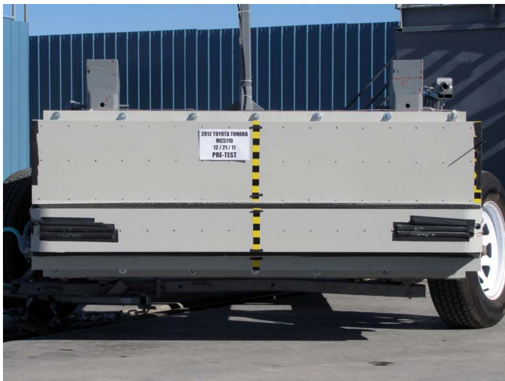
FIGURE 82. Pre-Test Front View of MDB Impactor Face
