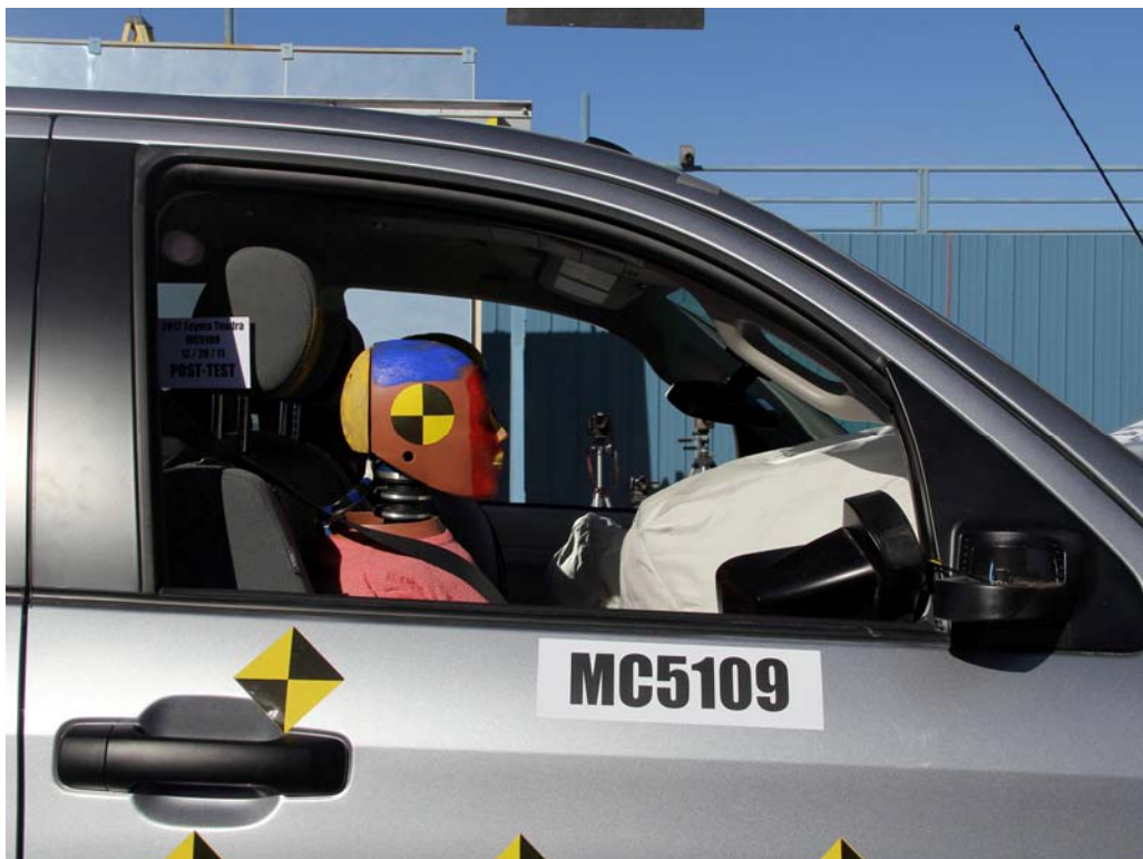
FIGURE 51. Post-Test Passenger Dummy Window View
