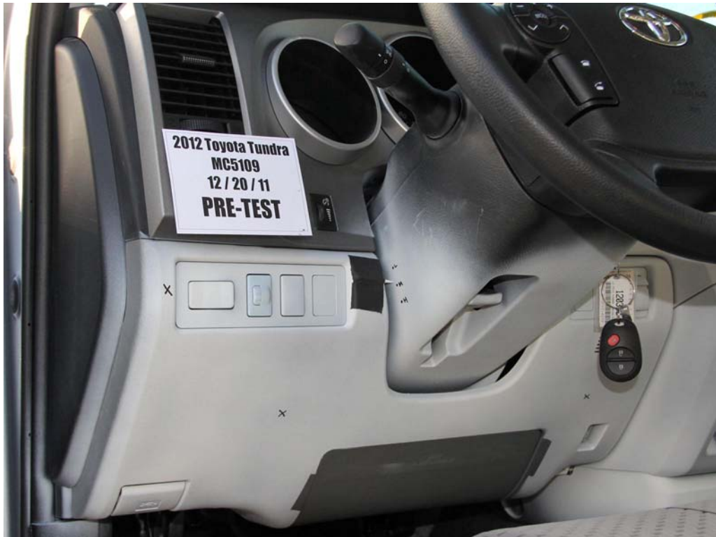
FIGURE 39. Pre-Test Driver's Side Knee Bolster
