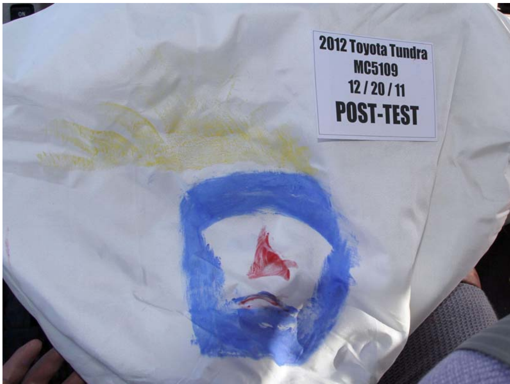
FIGURE 44. Post-Test Driver Dummy Contact With Airbag
