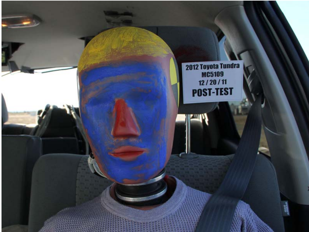
FIGURE 43. Post-Test Driver Dummy Face
