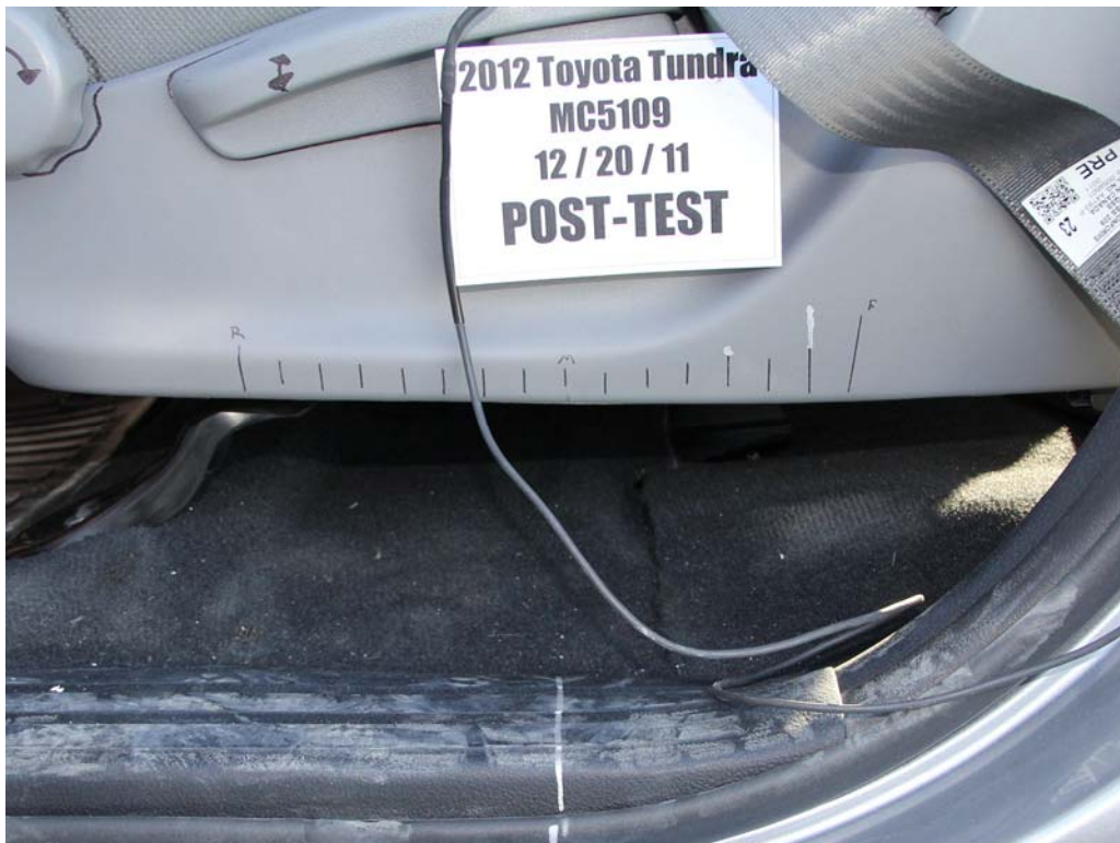
FIGURE 36. Post-Test Driver's Seat Fore-Aft Markings
