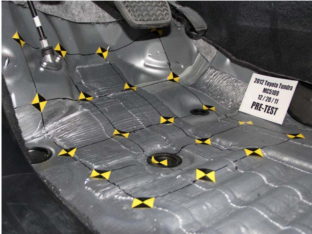
FIGURE 41. Pre-Test Driver's Side Floorpan
