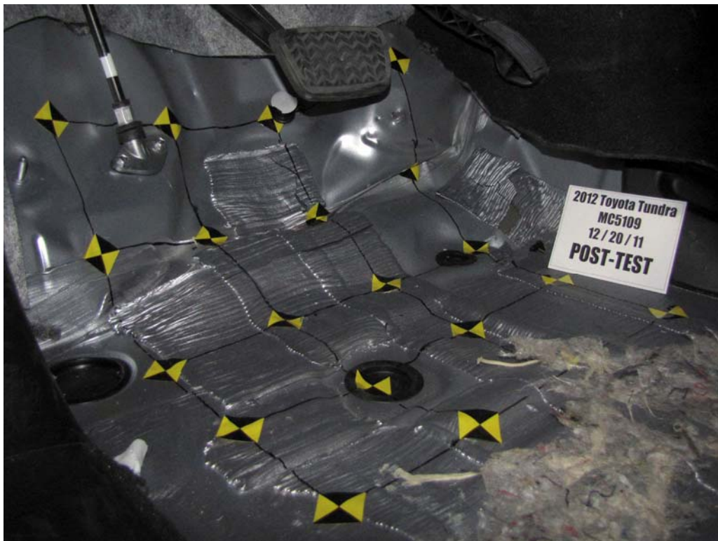
FIGURE 42. Post-Test Driver's Side Floorpan
