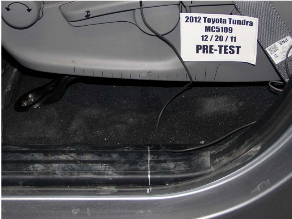
FIGURE 35. Pre-Test Driver's Seat Fore-Aft Markings
