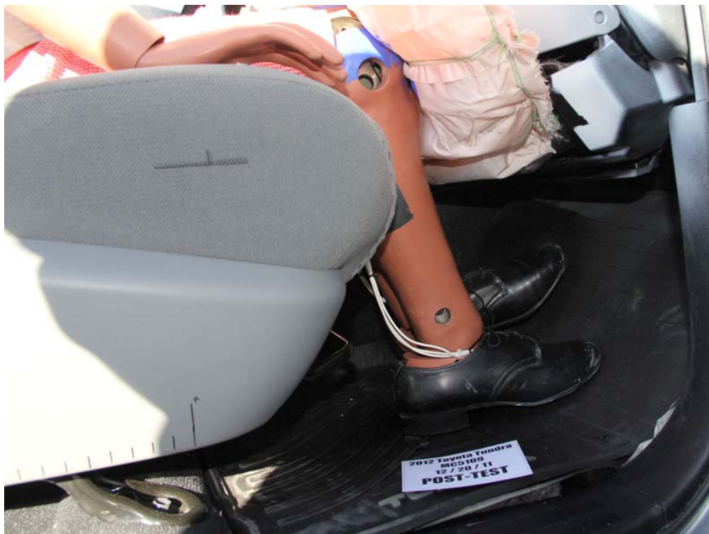
FIGURE 57. Post-Test Passenger Dummy Feet
