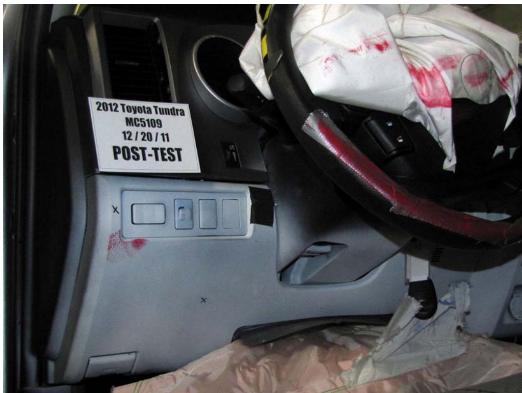
FIGURE 40. Post-Test Driver's Side Knee Bolster
