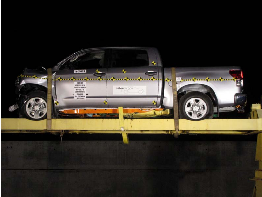
FIGURE 70. Vehicle at 360° on Static Rollover Device
