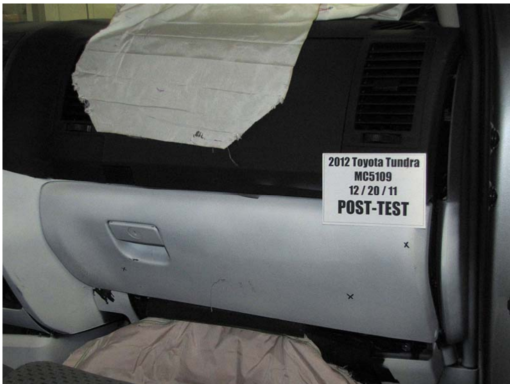
FIGURE 59. Post-Test Passenger's Side Knee Bolster
