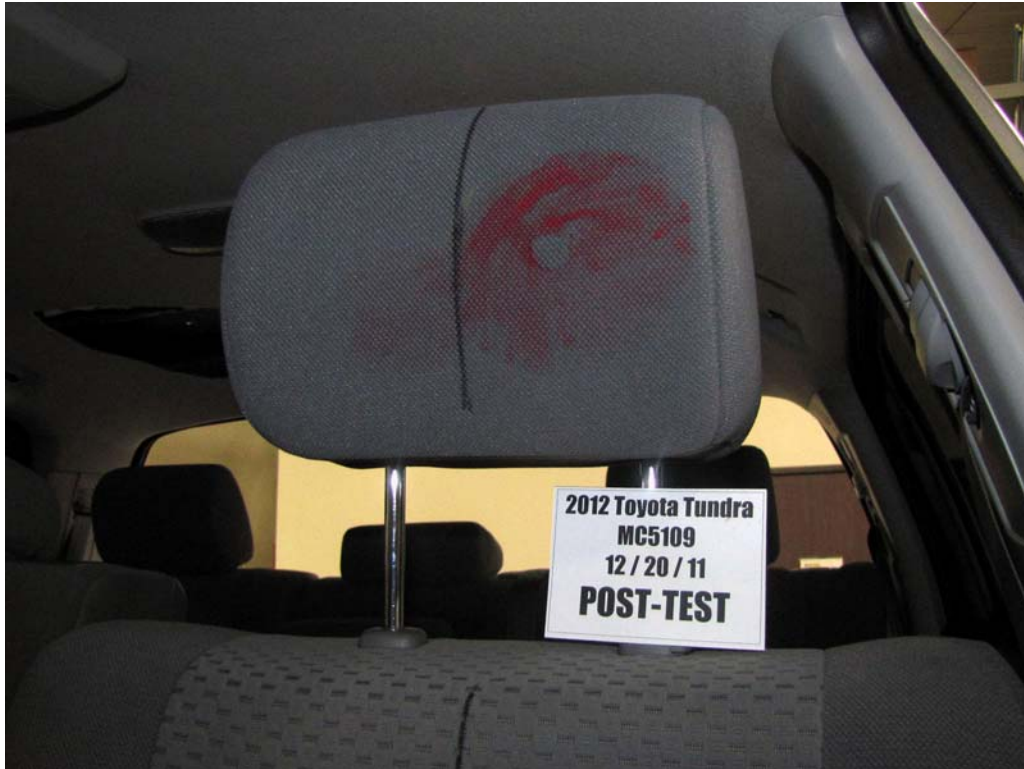
FIGURE 45. Post-Test Driver Dummy Contact With Headrest
