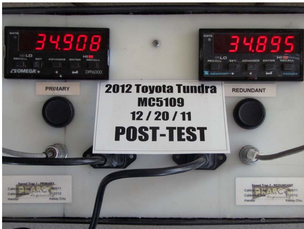
FIGURE 65. Post-Test Speed Trap Read Out
