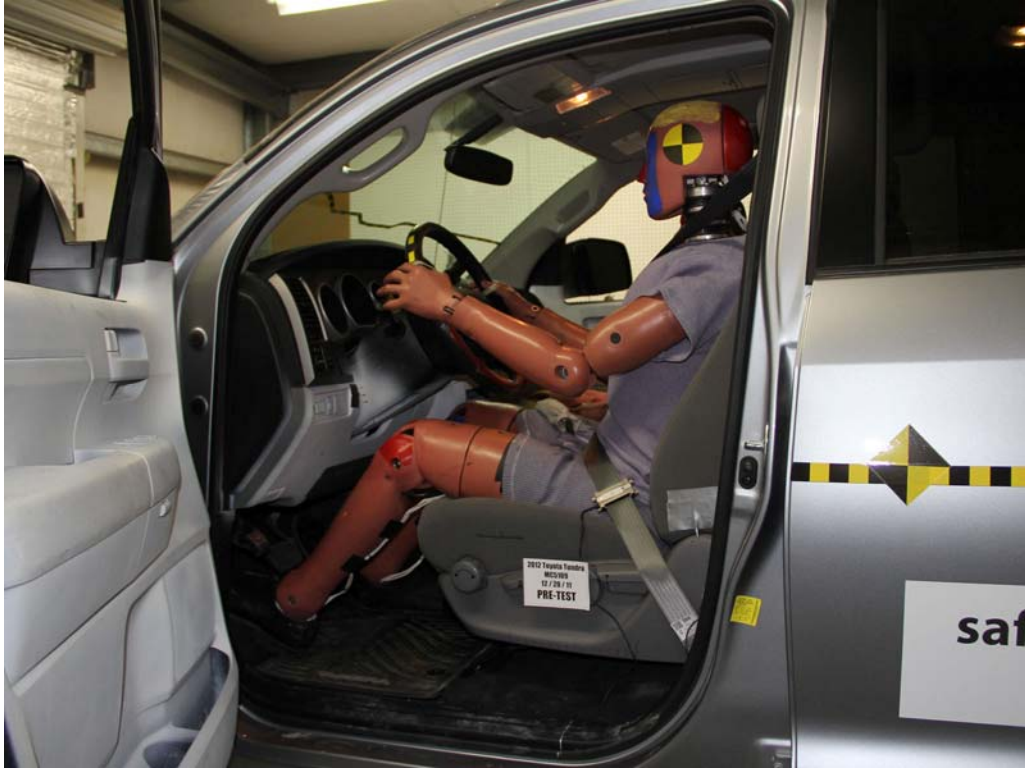
FIGURE 33. Pre-Test Driver Dummy and Vehicle Interior View
