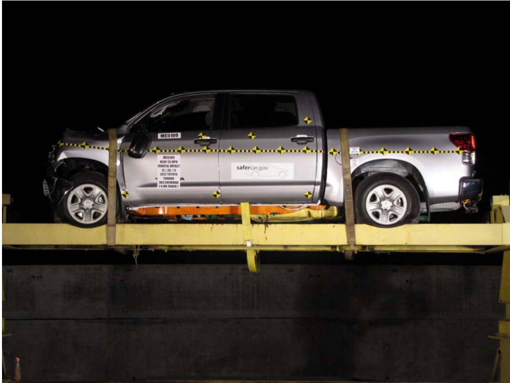
FIGURE 66. Vehicle at 0°on Static Rollover Device
