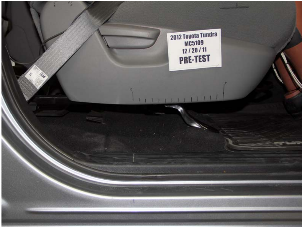
FIGURE 54. Pre-Test Passenger's Seat Fore-Aft Markings
