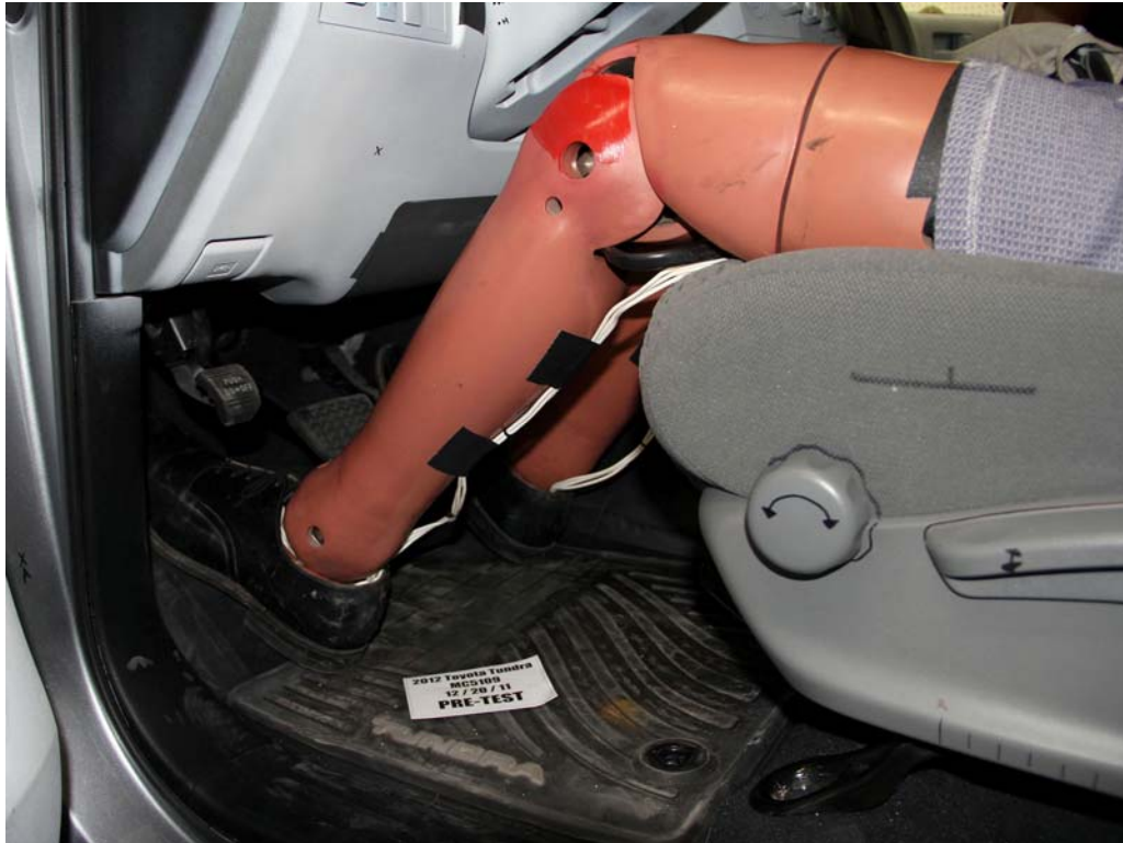
FIGURE 37. Pre-Test Driver Dummy Feet
