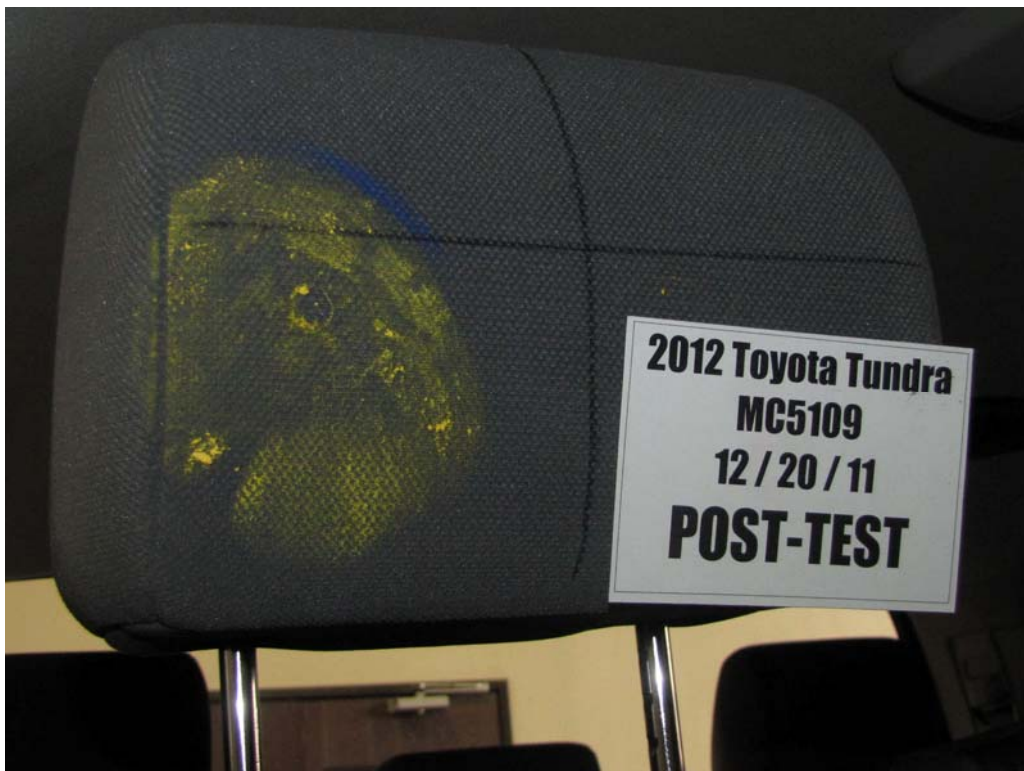
FIGURE 62a. Post-Test Passenger Dummy Contact With Headrest
