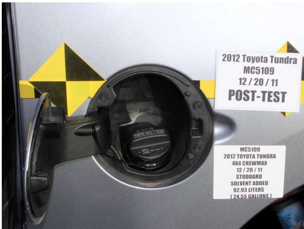
FIGURE 22. Post-Test Fuel Filler Cap View
