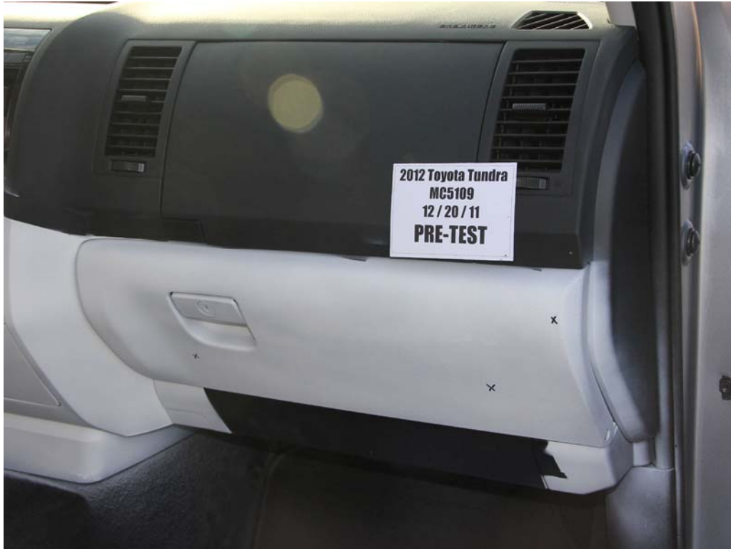
FIGURE 58. Pre-Test Passenger's Side Knee Bolster
