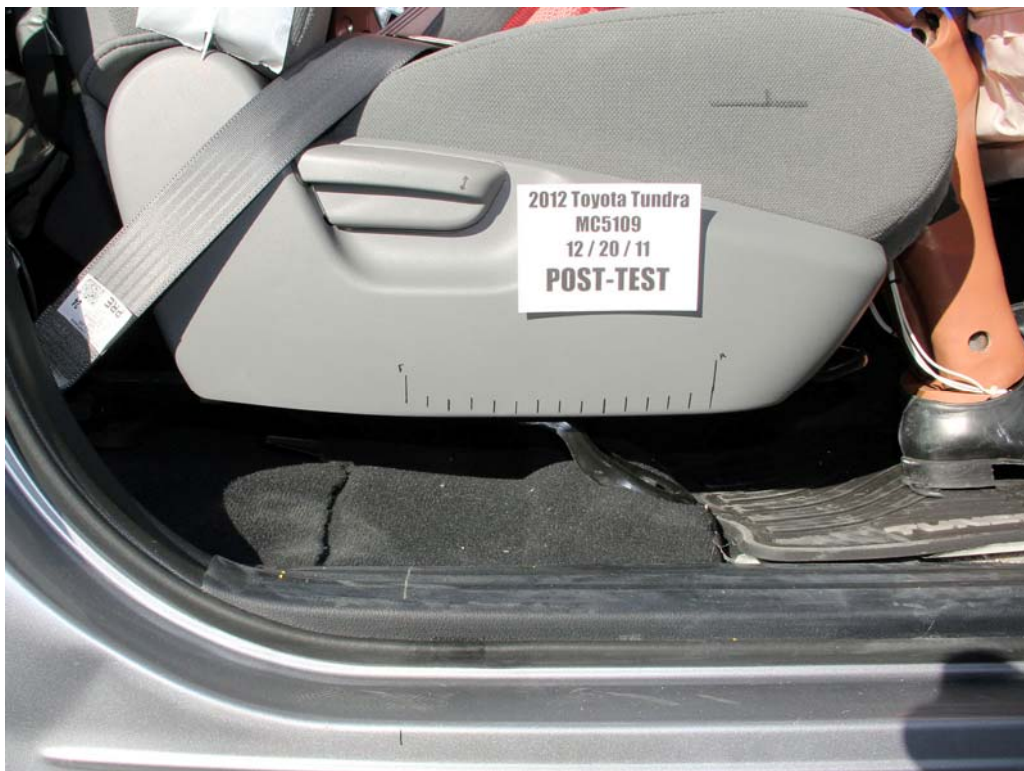
FIGURE 55. Post-Test Passenger's Seat Fore-Aft Markings
