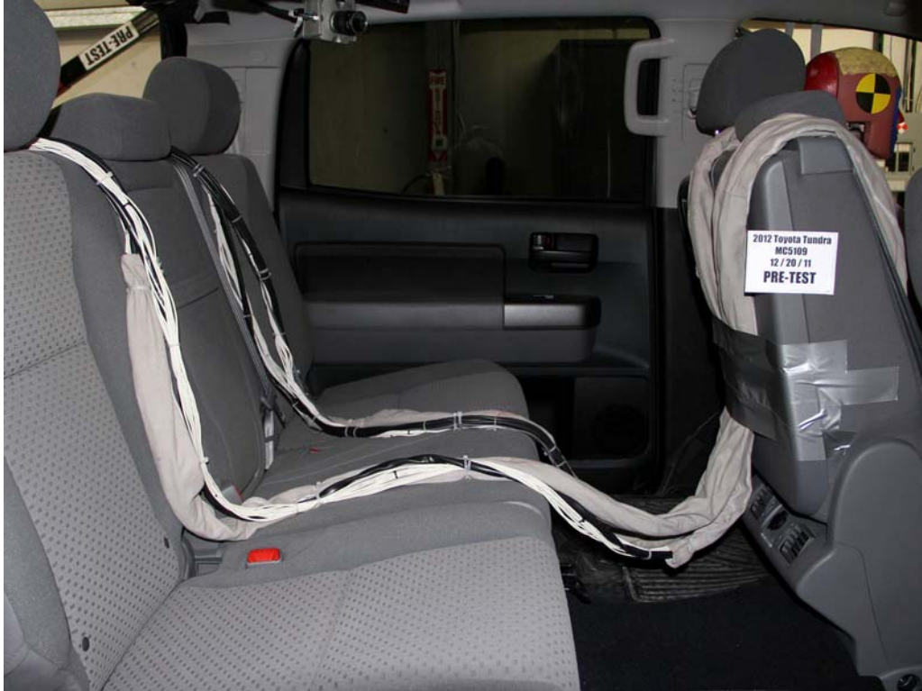
FIGURE 27. Pre-Test Dummy Cable Routing
