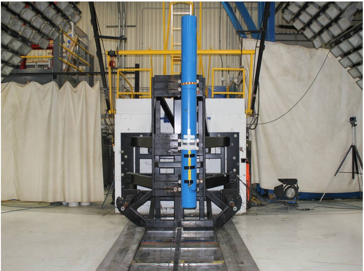
Pre-Test Pole Barrier Front View
