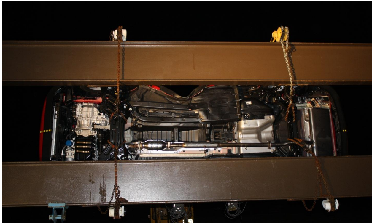
Figure A-65: FMVSS No. 301 Static Rollover 270 Degrees
