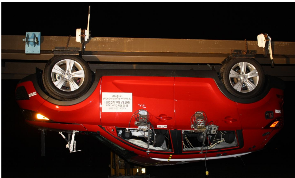
Figure A-64: FMVSS No. 301 Static Rollover 180 Degrees
