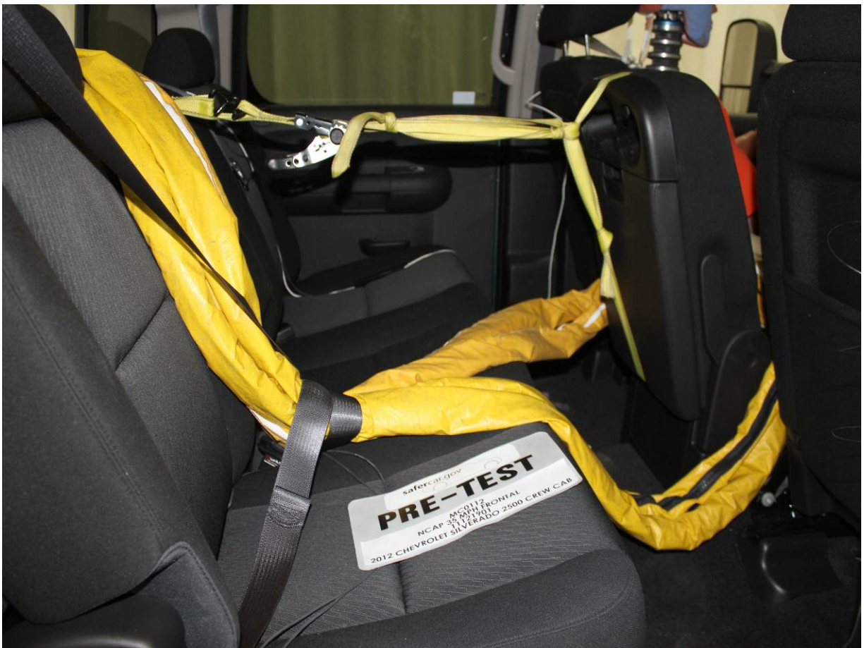
Pre-Test Dummy Cable Routing
