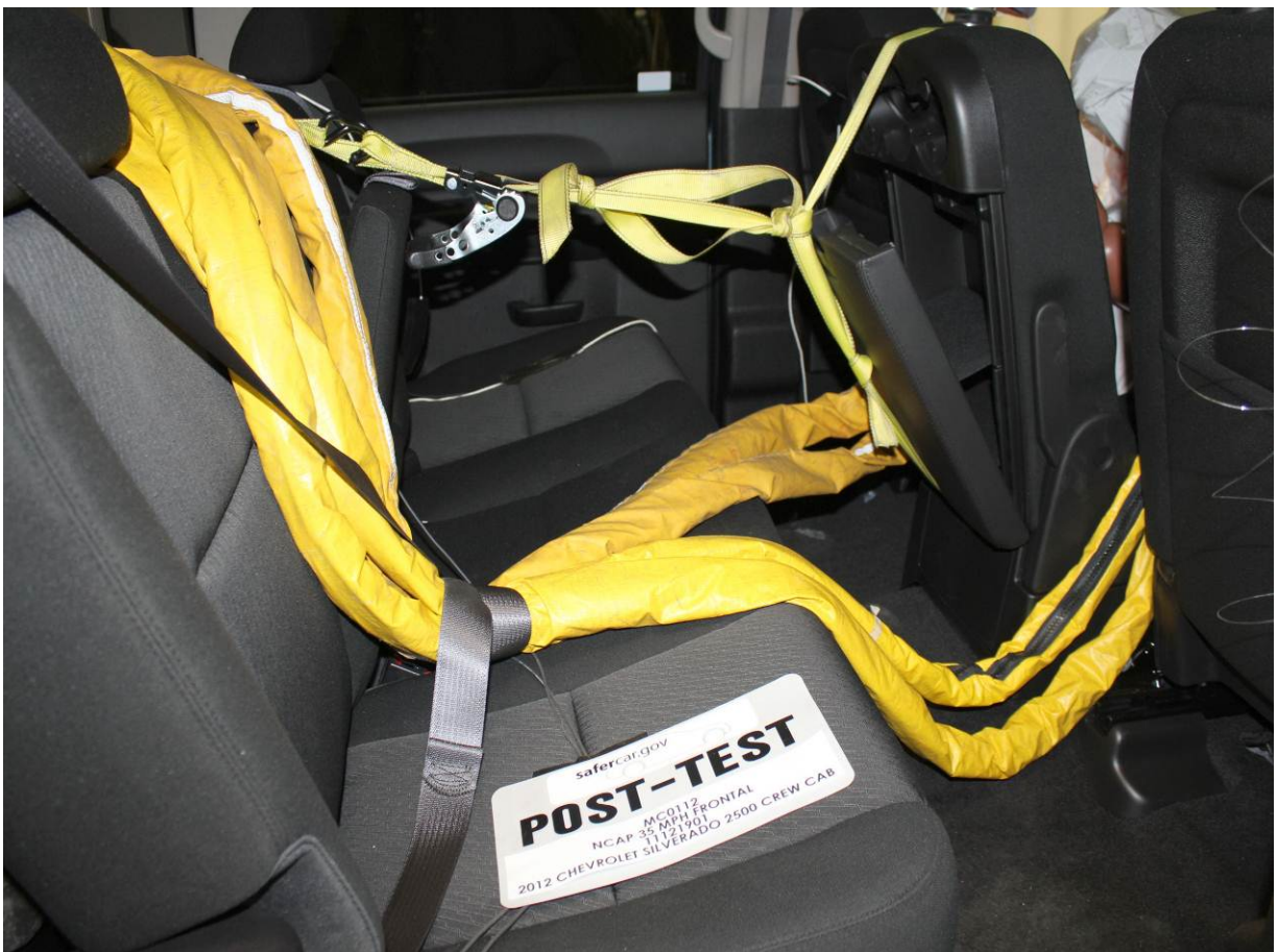
Post-Test Dummy Cable Routing
