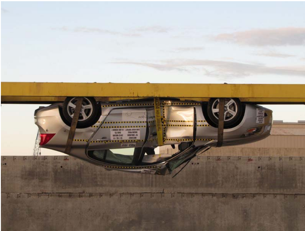
FIGURE 64. FMVSS No. 301-305 Rollover 180 Degrees
