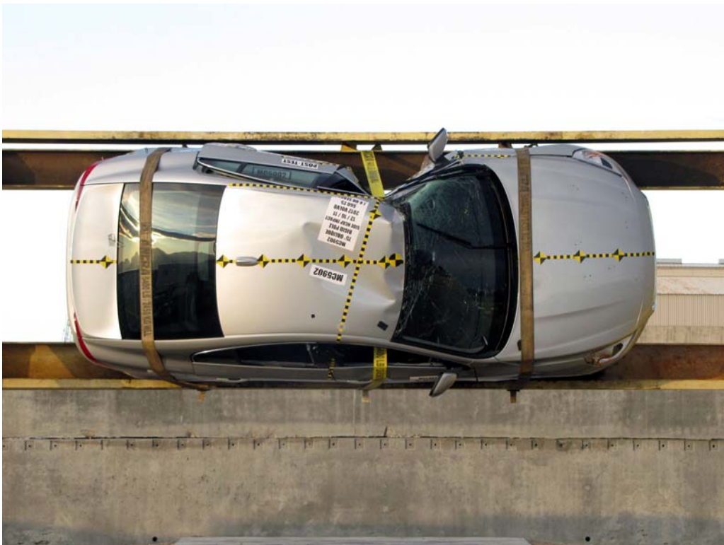
FIGURE 63. FMVSS No. 301-305 Rollover 90 Degrees
