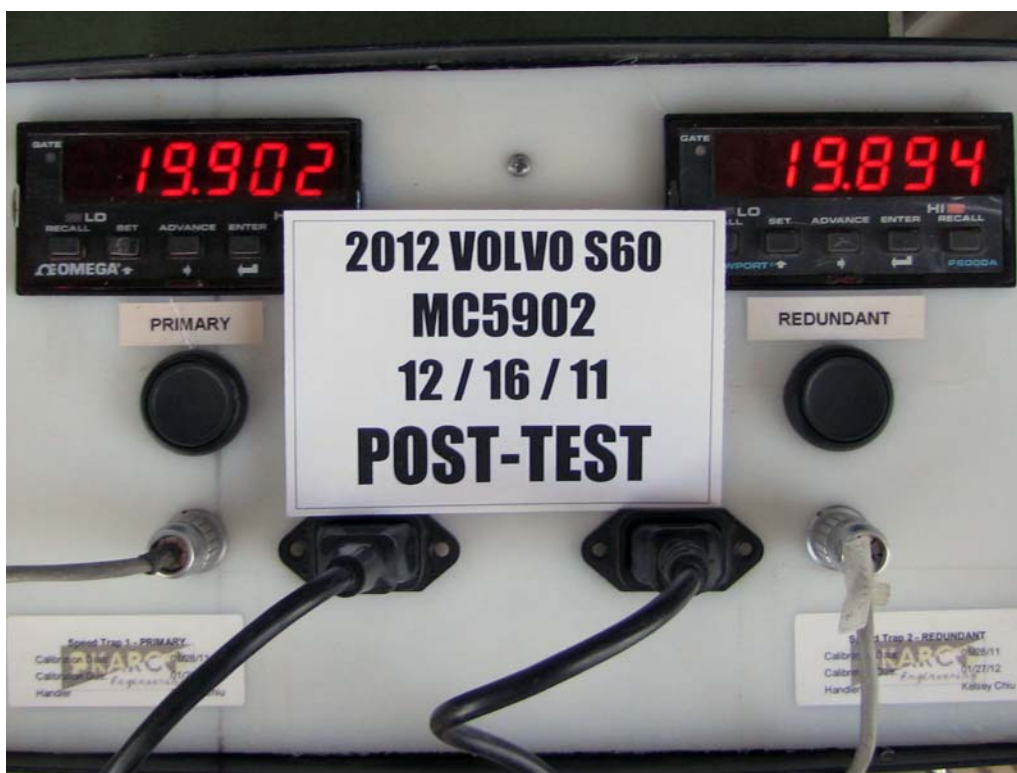
FIGURE 61. Post-Test Primary and Redundant Speed Trap Read-Out
