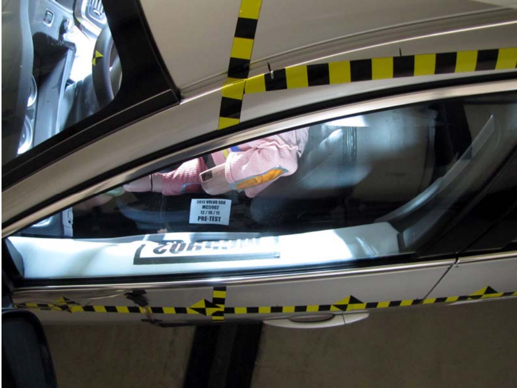
FIGURE 40. Pre-Test Driver Dummy and Door Clearance
