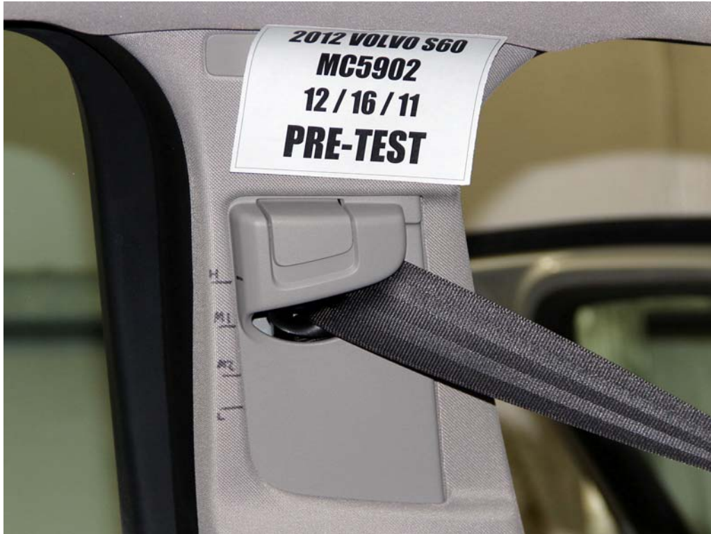
FIGURE 33. Pre-Test View of Belt Anchorage for Dummy
