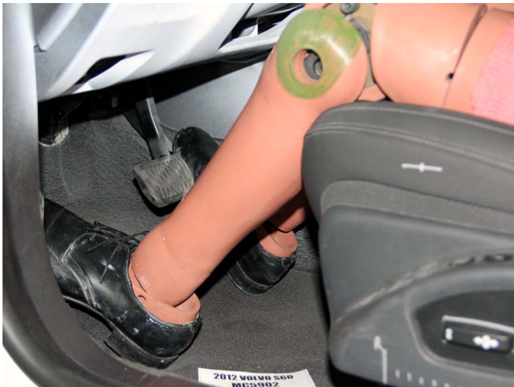
FIGURE 32. Pre-Test Placement of Dummy's Feet
