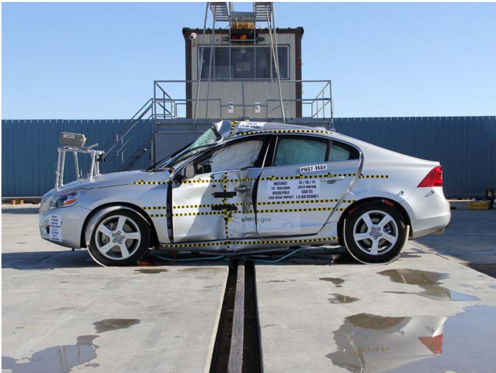
FIGURE 8. Post-Test Left Side View of Test Vehicle
