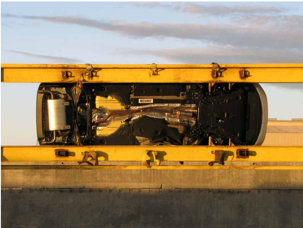
FIGURE 65. FMVSS No. 301-305 Rollover 270 Degrees
