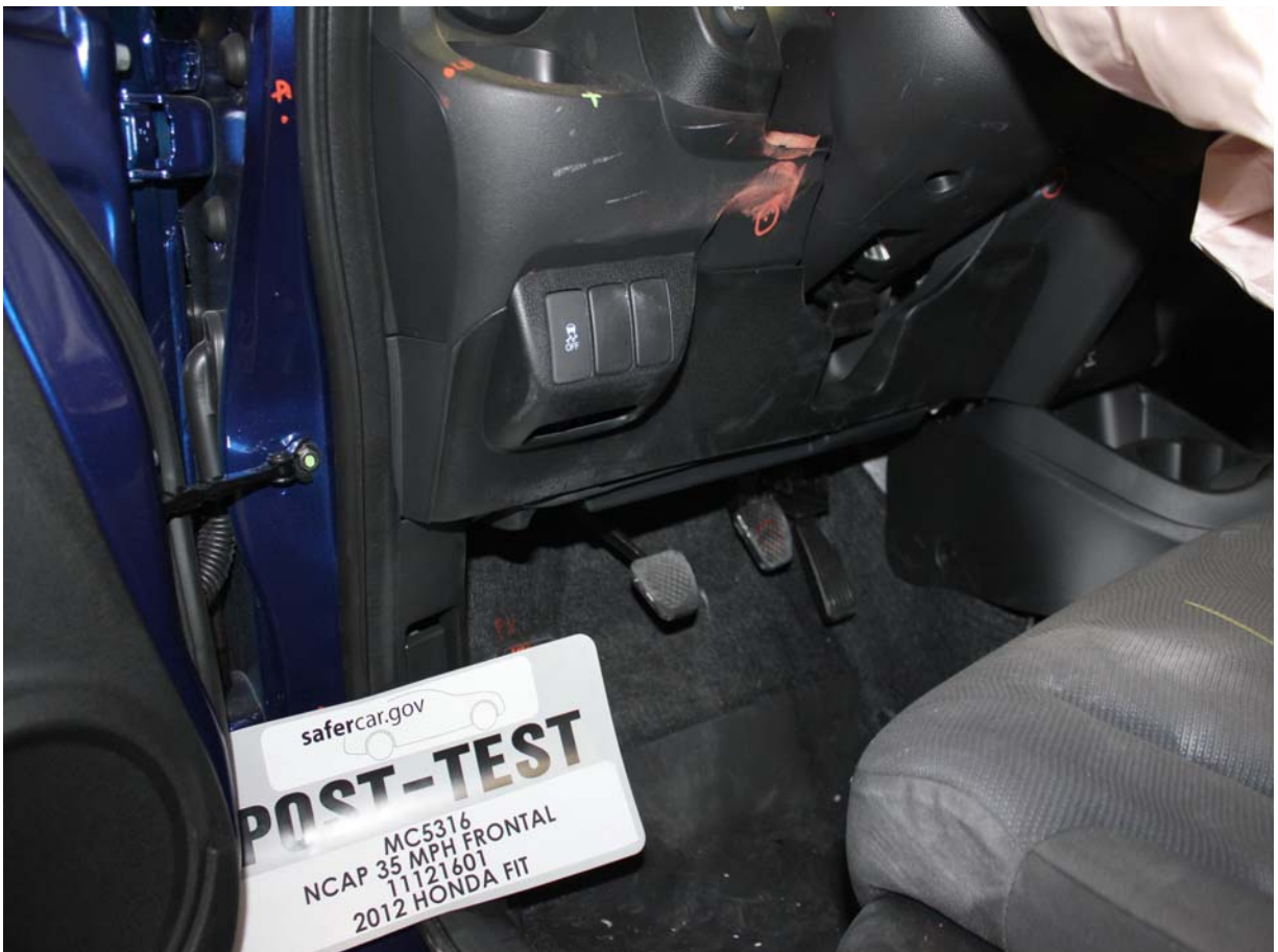
Post-Test Driver's Side Knee Bolster (without dummy)
