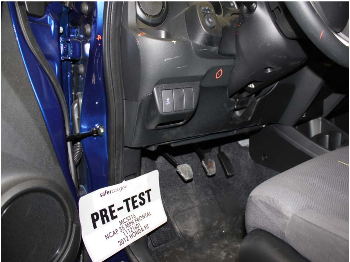
Pre-Test Driver's Side Knee Bolster (without dummy)
