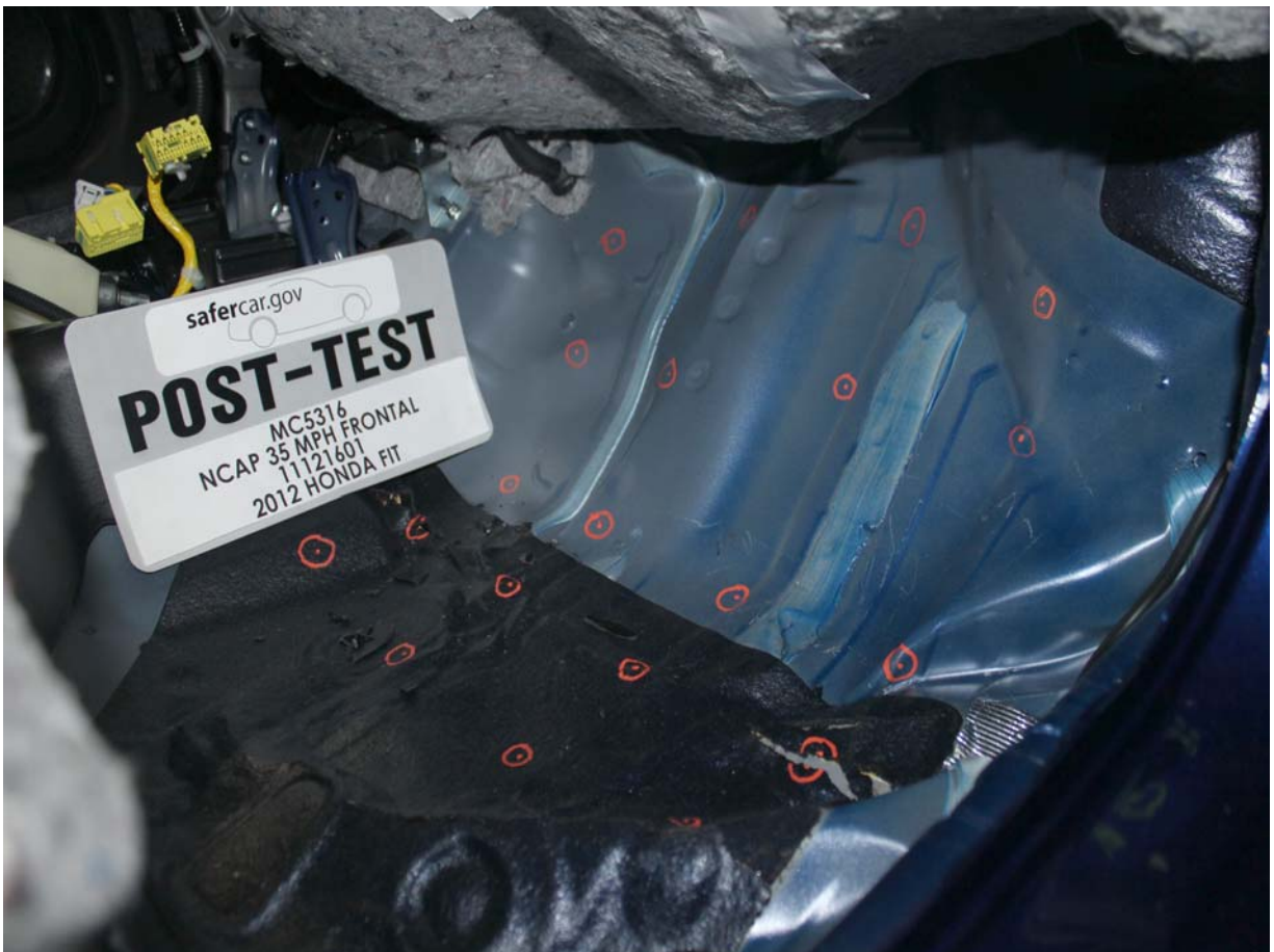
Post-Test Passenger's Side Floorpan
