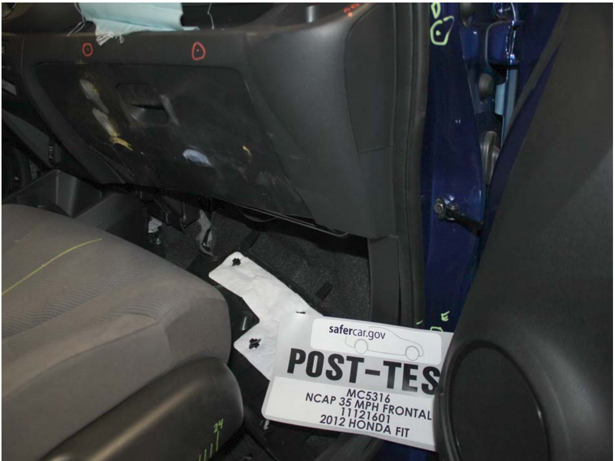
Post-Test Passenger's Side Knee Bolster (without dummy)
