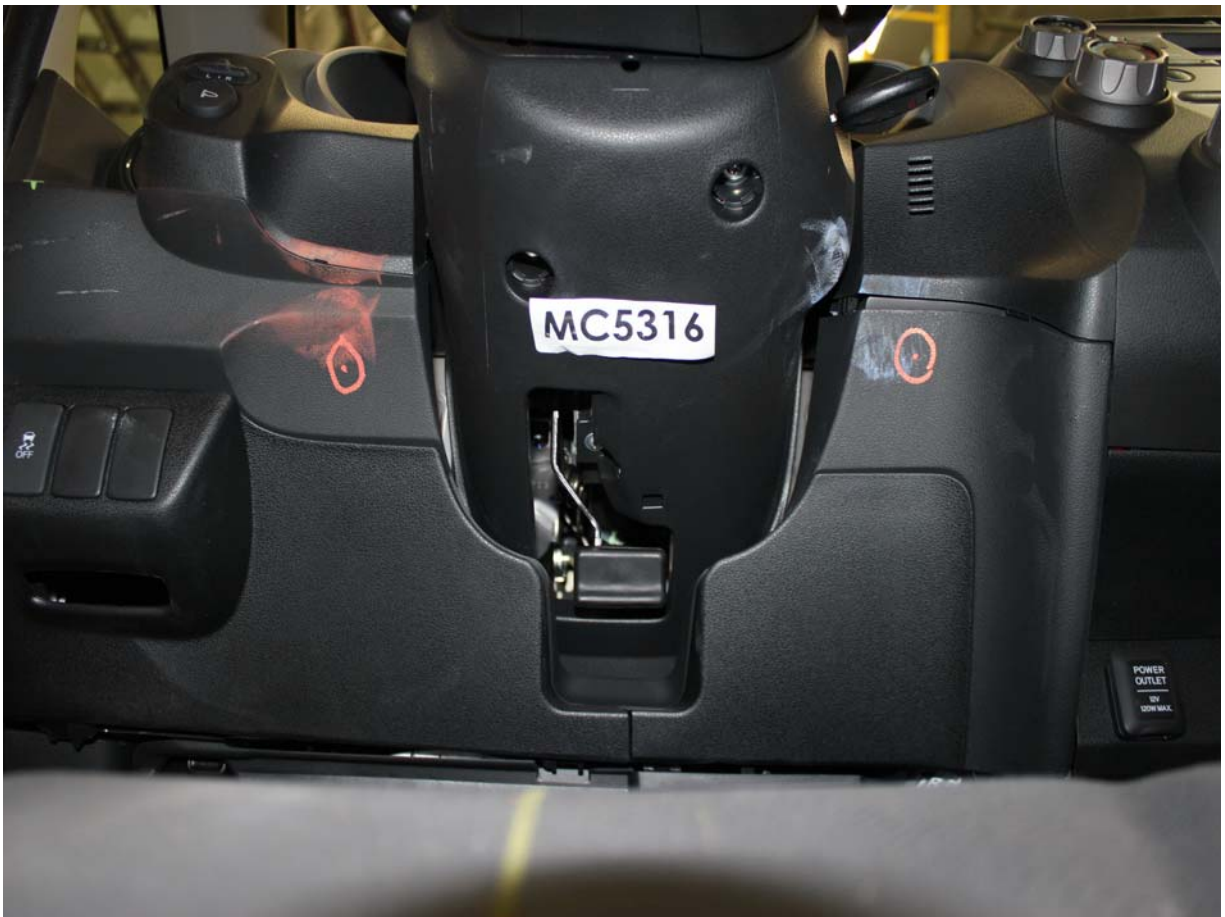
Post-Test Driver's Side Knee Bolster (without dummy)
