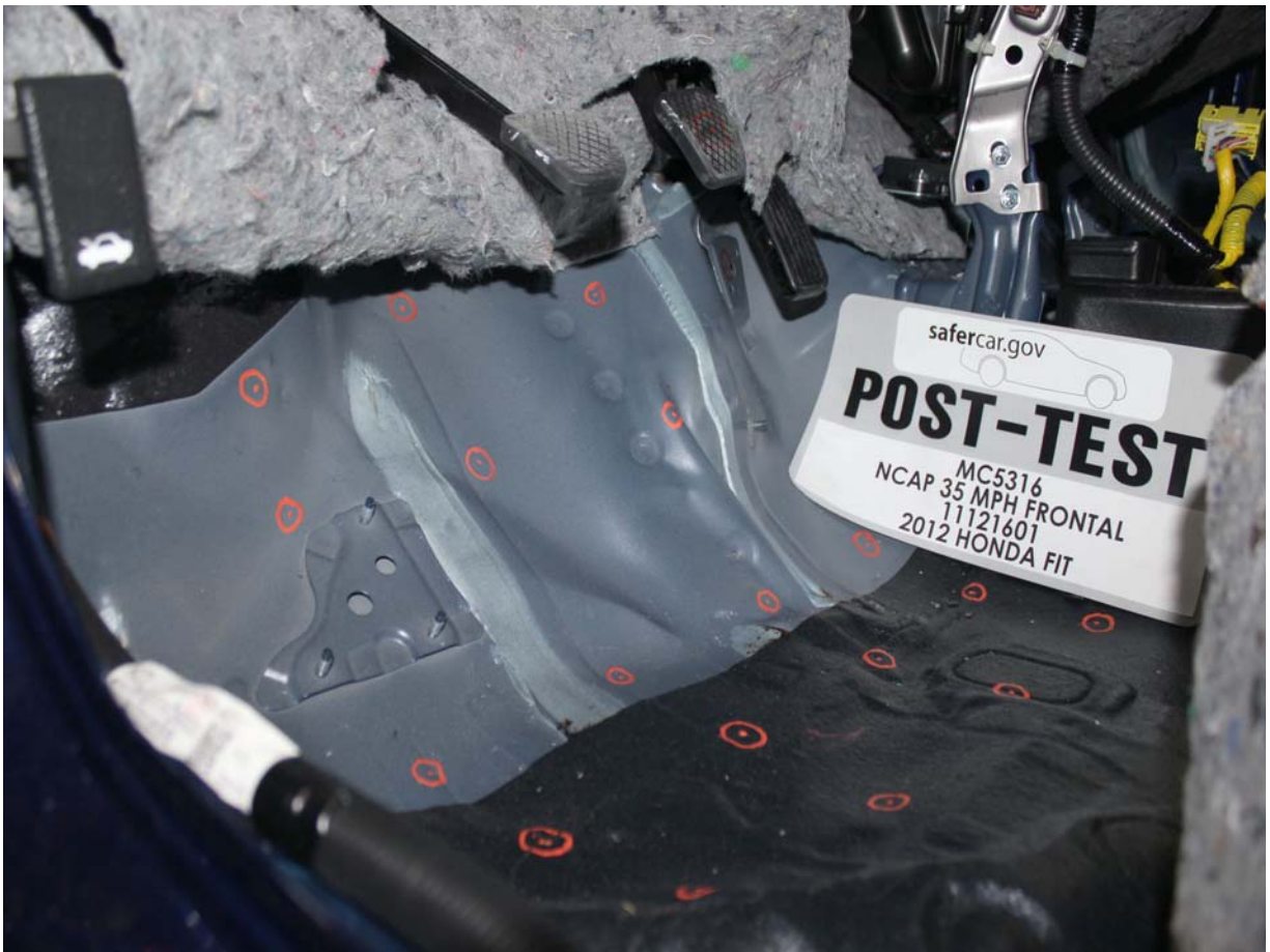
Post-Test Driver's Side Floorpan
