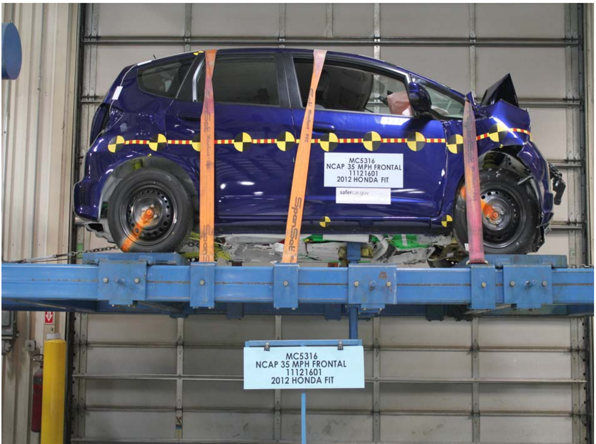
Vehicle at 0 Degrees on Static Rollover Device
