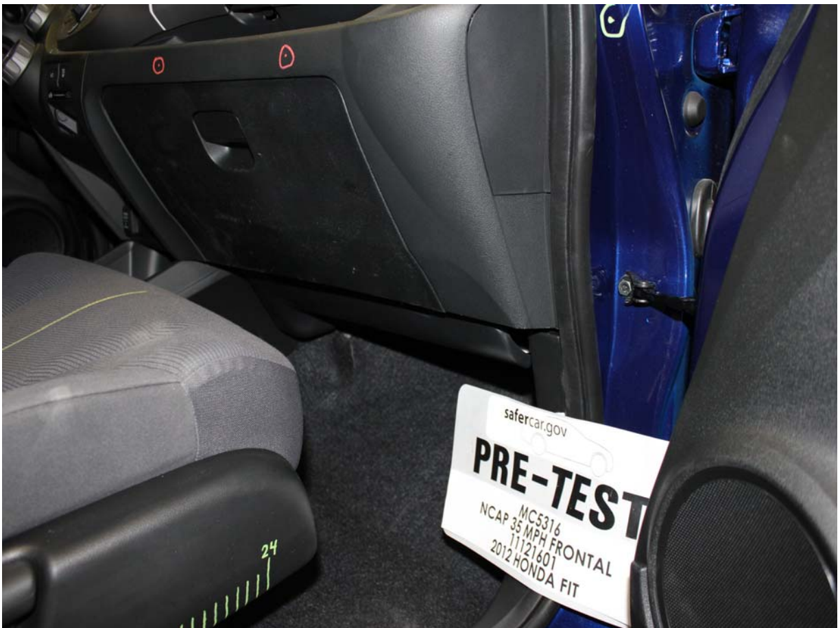
Pre-Test Passenger's Side Knee Bolster (without dummy)
