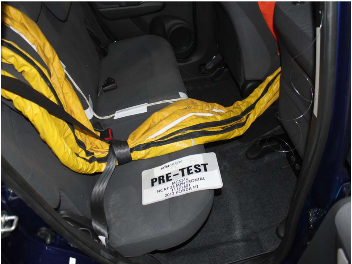
Pre-Test Dummy Cable Routing
