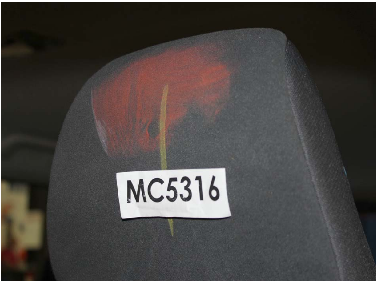
Post-Test Driver Dummy Contact with Headrest
