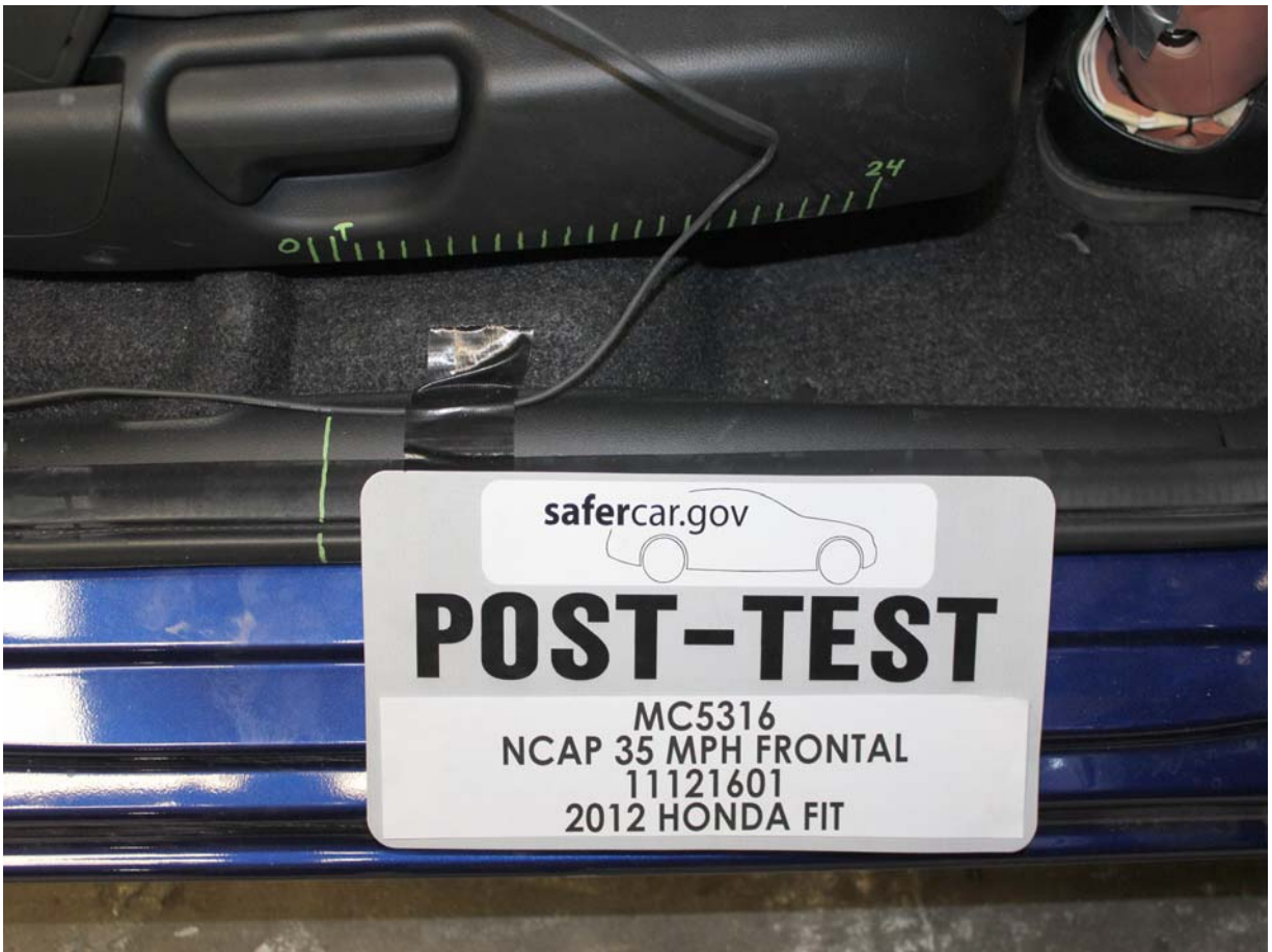
Post-Test Passenger's Seat Fore-Aft Markings
