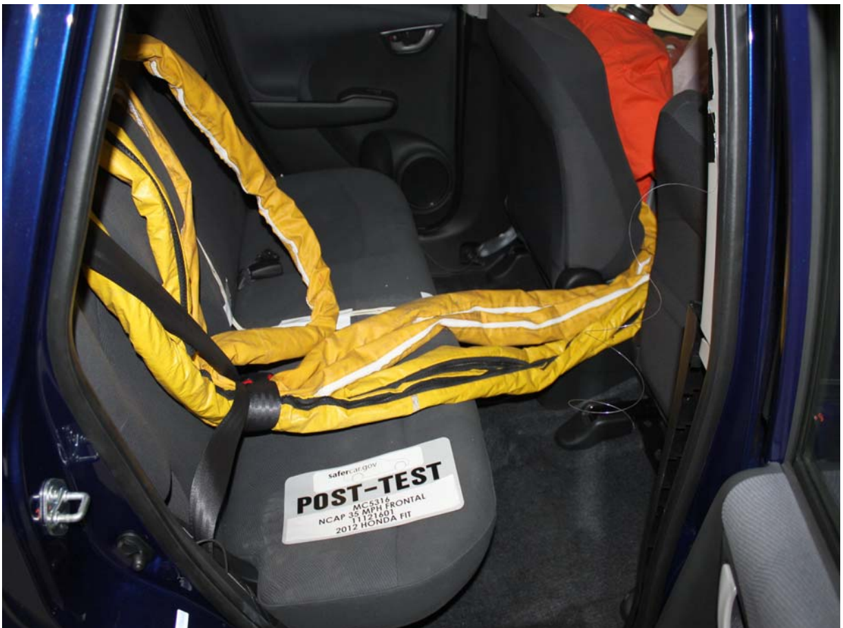
Post-Test Dummy Cable Routing
