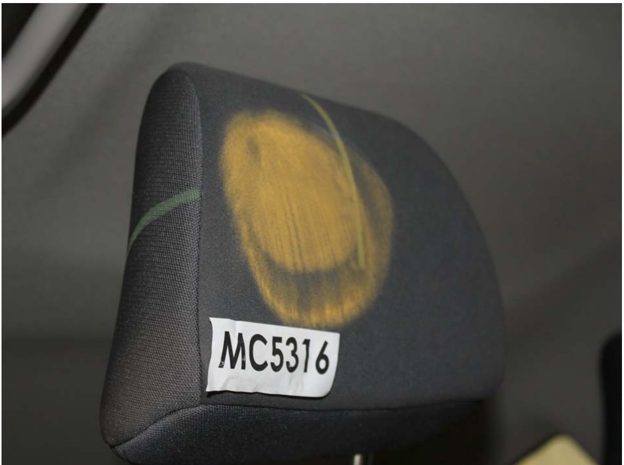
Post-Test Passenger Dummy Contact with Headrest
