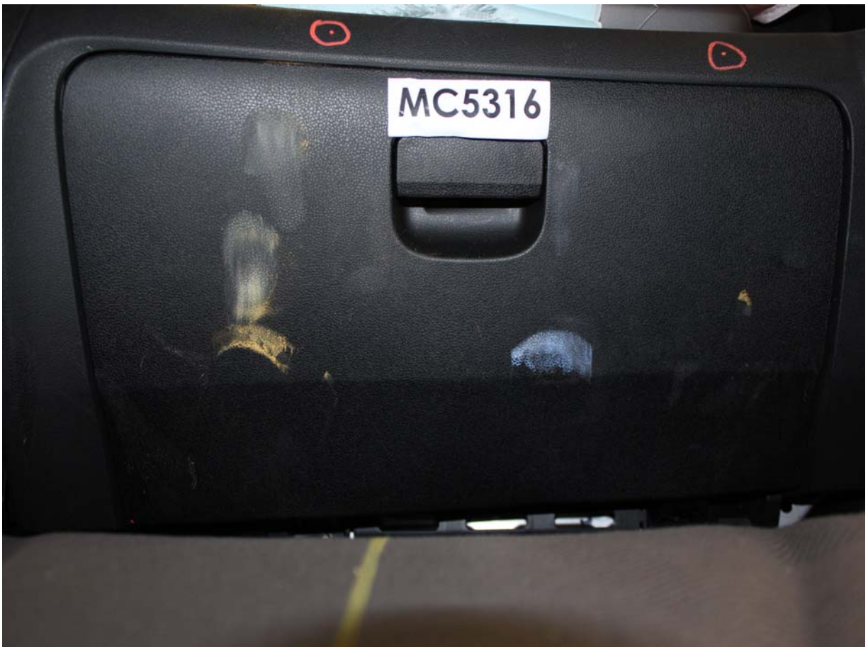
Post-Test Passenger's Side Knee Bolster (without dummy)
