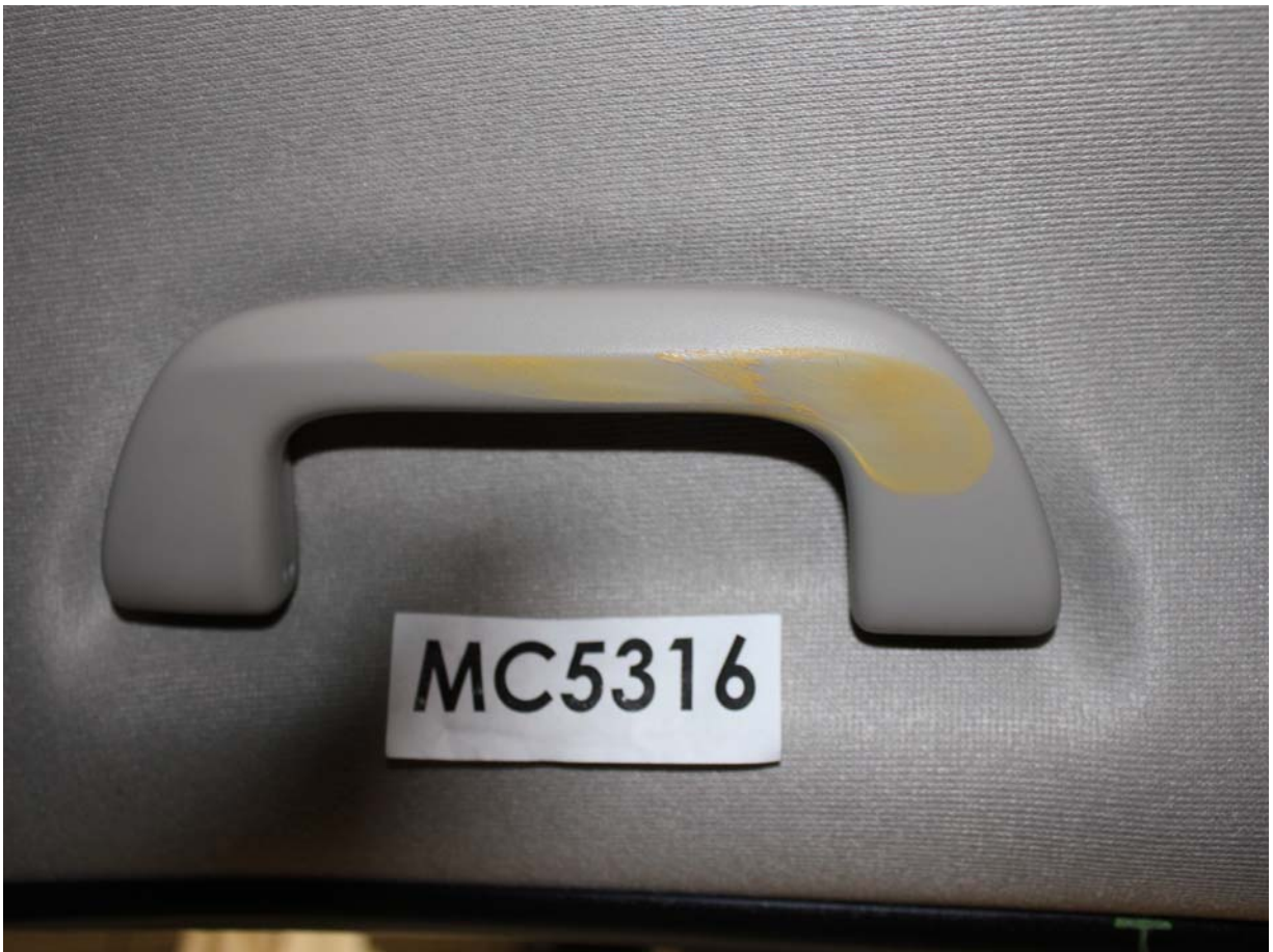
Post-Test Driver Dummy Contact with Handle on Ceiling
