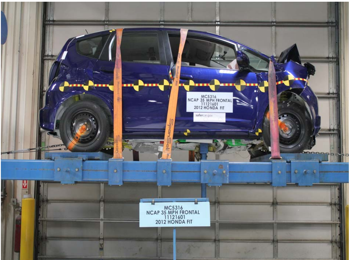
Vehicle at 360 Degrees on Static Rollover Device
