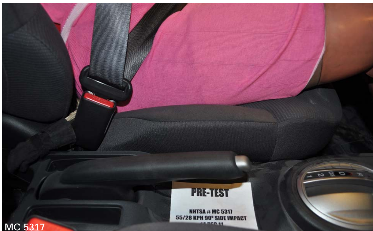
Figure A-37: View of Disengaged Parking Brake
