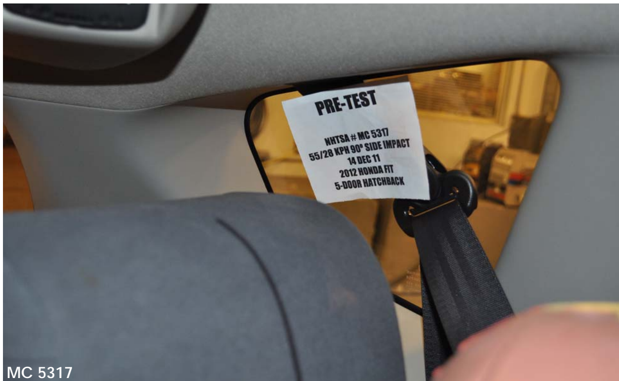
Figure A-64: Pre-Test View of Belt Anchorage for Rear Passenger Dummy
