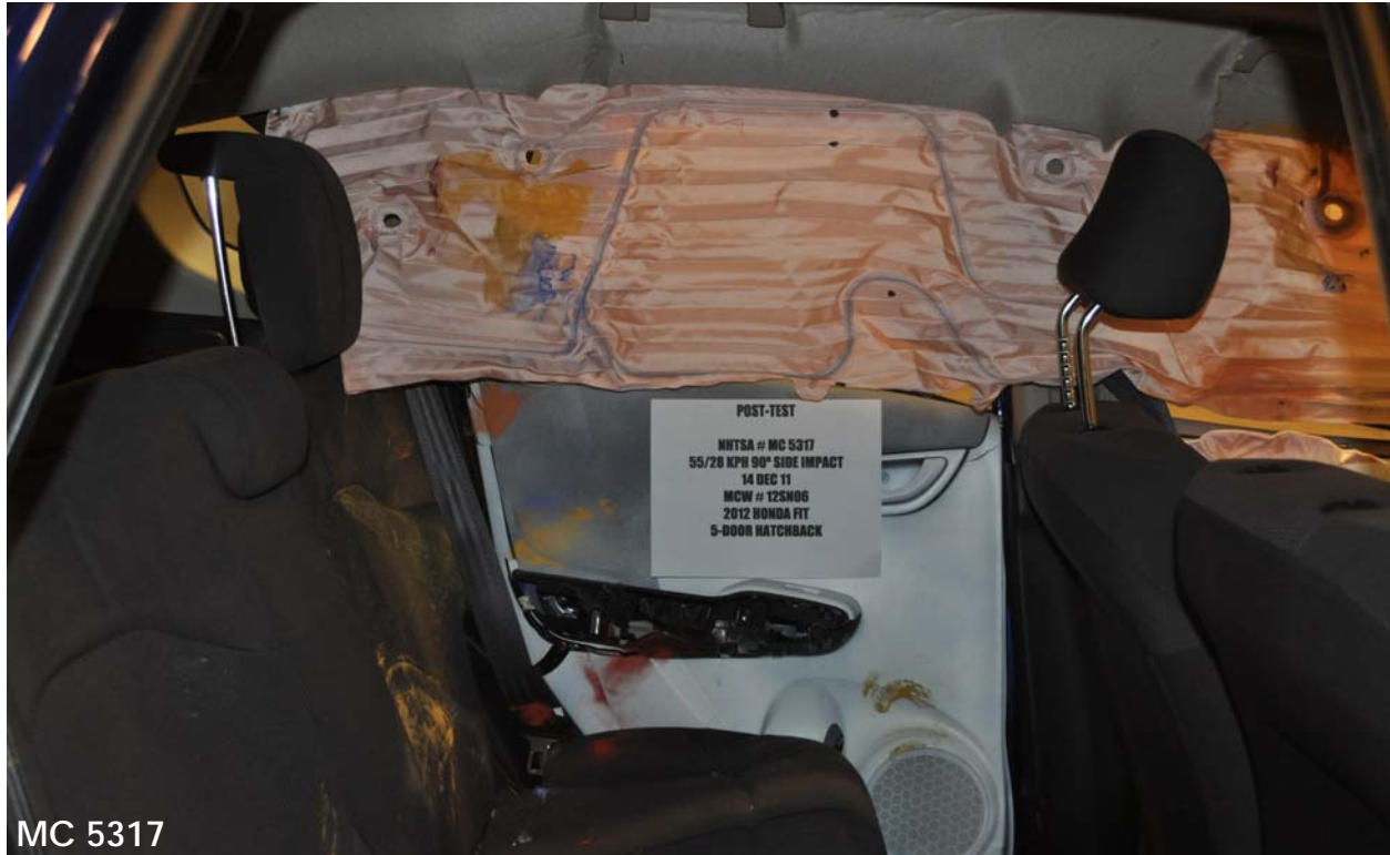
Figure A-73: Post-Test Rear Passenger Inner Door Panel View Showing Dummy Contact Locations
