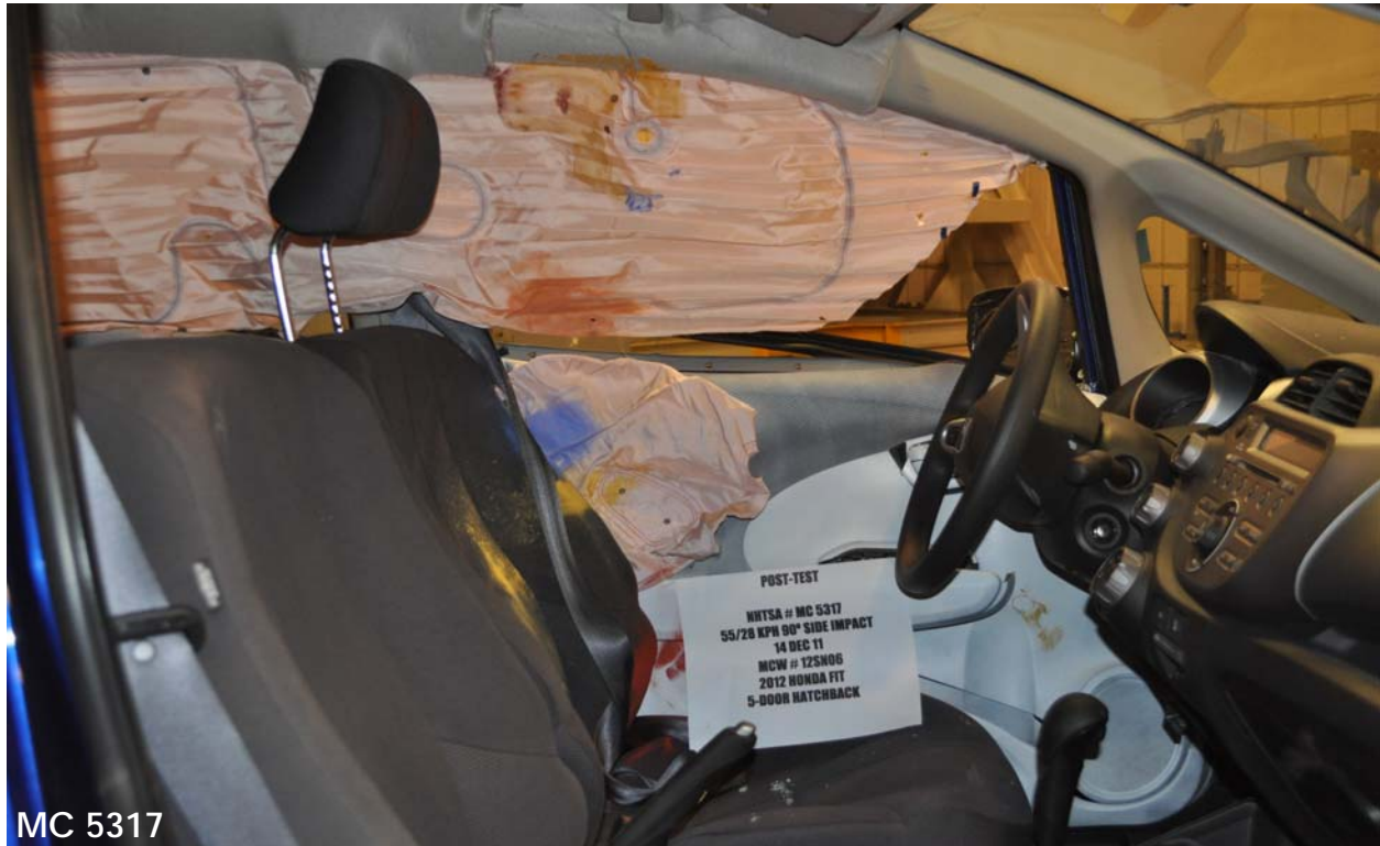
Figure A-47: Post-Test Driver Inner Door Panel View Showing Driver Dummy Contact Locations
