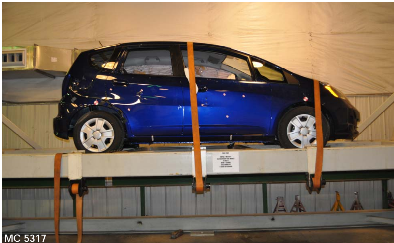
Figure A-98: FMVSS No. 301 Static Rollover 360 Degrees
