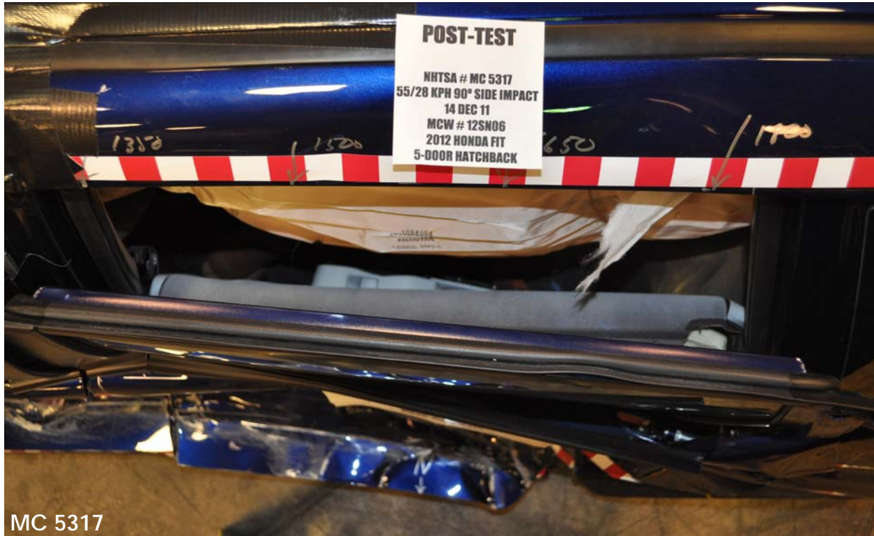
Figure A-69: Post-Test Rear Passenger Dummy and Door Clearance View
