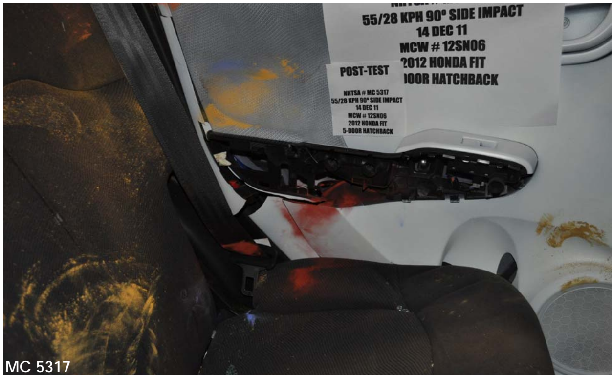
Figure A-78: Post-Test Rear Passenger Dummy Close-up Pelvis Contact with Vehicle Interior View
