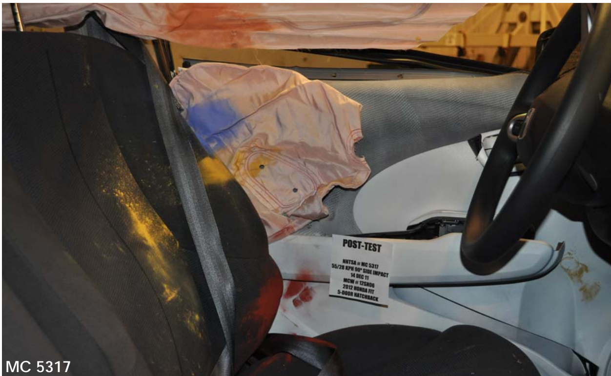
Figure A-50: Post-Test Driver Dummy Close-Up Torso Contact with Vehicle Interior View - N/a
