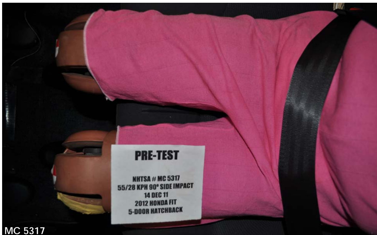
Figure A-60: Pre-Test Overhead View of Rear Passenger Dummy Thighs on Seat Pan
