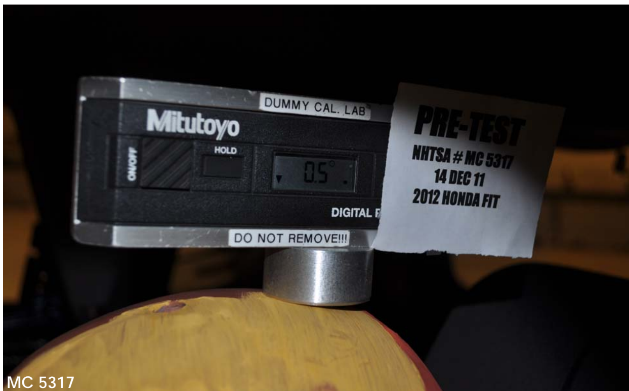
Figure A-62: Pre-Test View of Rear Passenger Dummy's Head Showing Dummy's Head is Level
