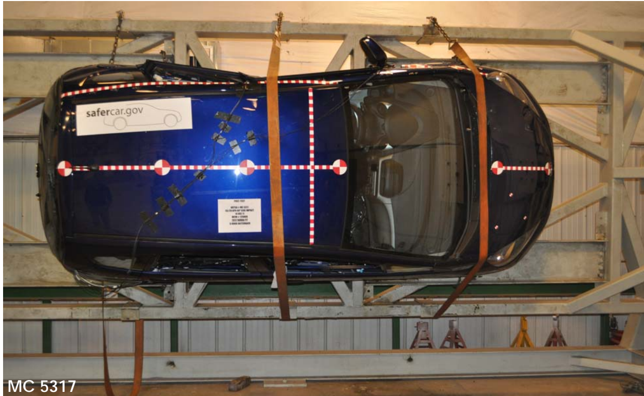
Figure A-97: FMVSS No. 301 Static Rollover 270 Degrees
