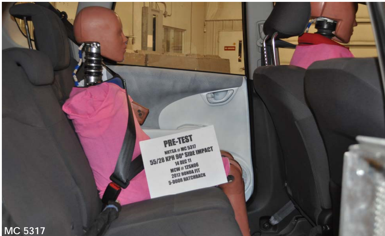
Figure A-70: Pre-Test Right Side View of Rear Passenger Dummy and Rear Seat Occupant Compartment
