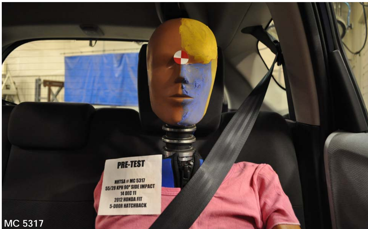
Figure A-58: Pre-Test Frontal View of Rear Passenger Dummy Head and Shoulders in Relation to Head Restraint
