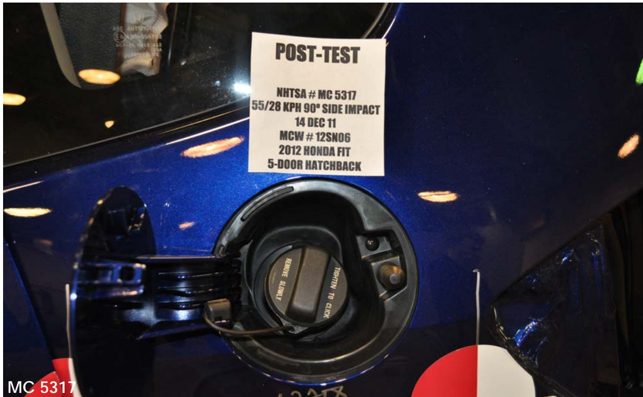
Figure A-81: Post-Test View of Fuel Filler Cap or Fuel Filler Neck
