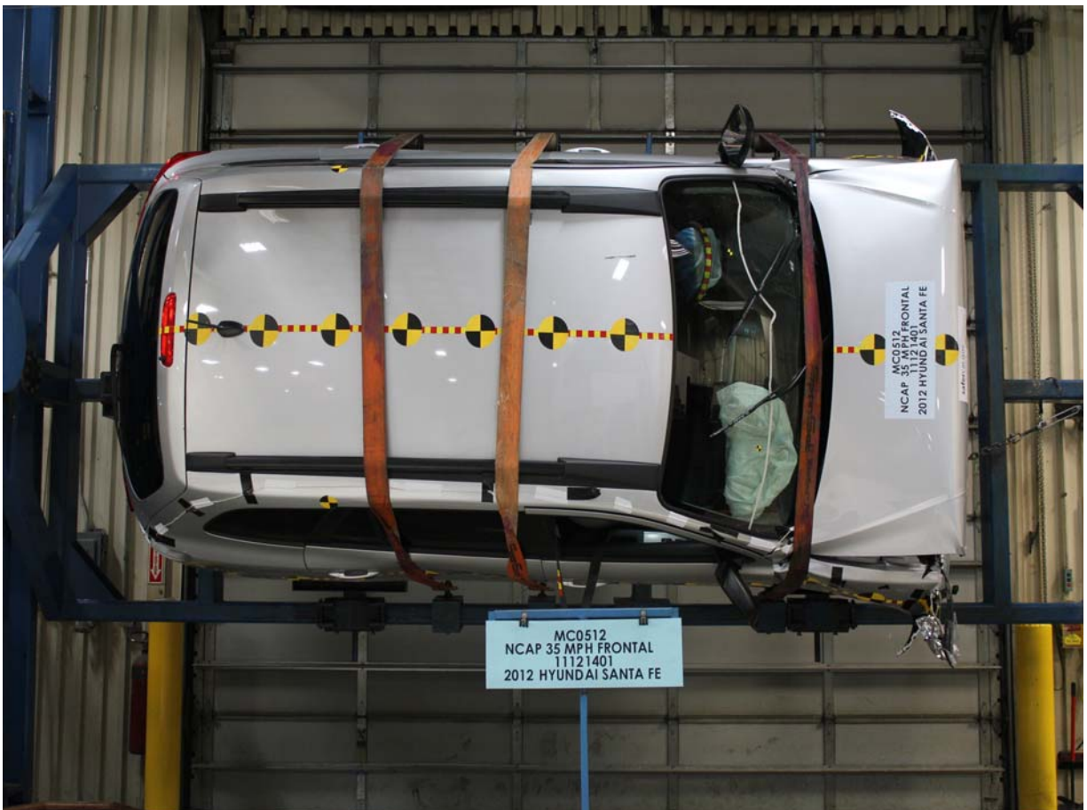
Vehicle at 270 Degrees on Static Rollover Device
