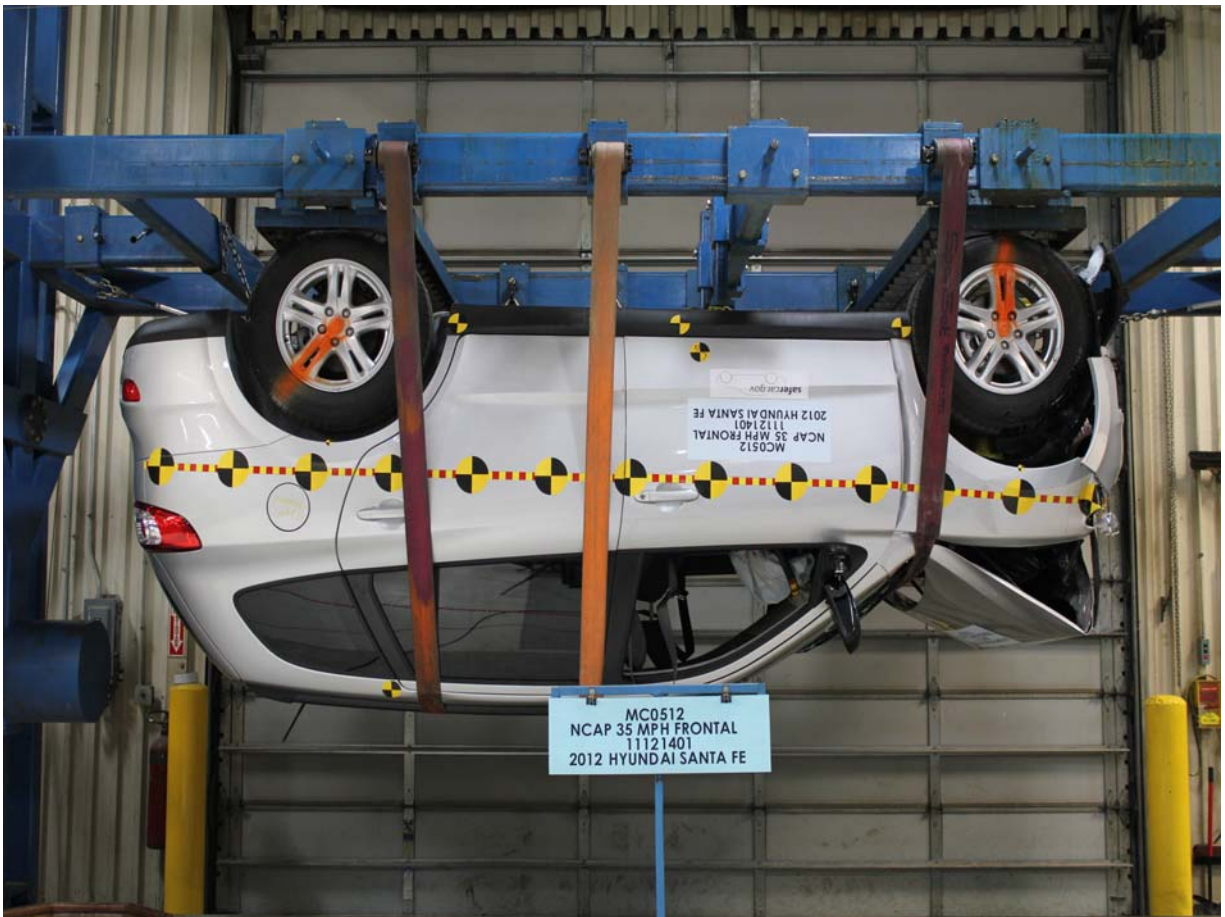
Vehicle at 180 Degrees on Static Rollover Device
