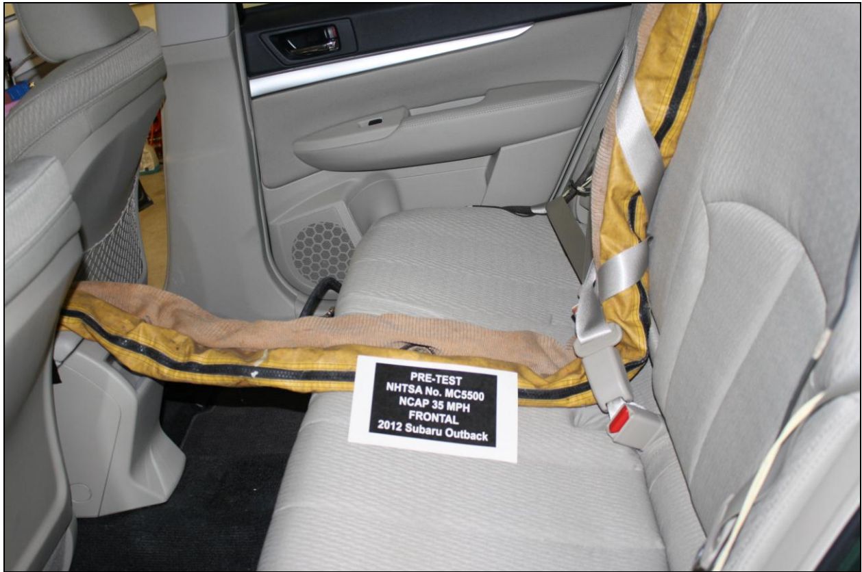
Figure A-27: Pre-Test Dummy Cable Routing
