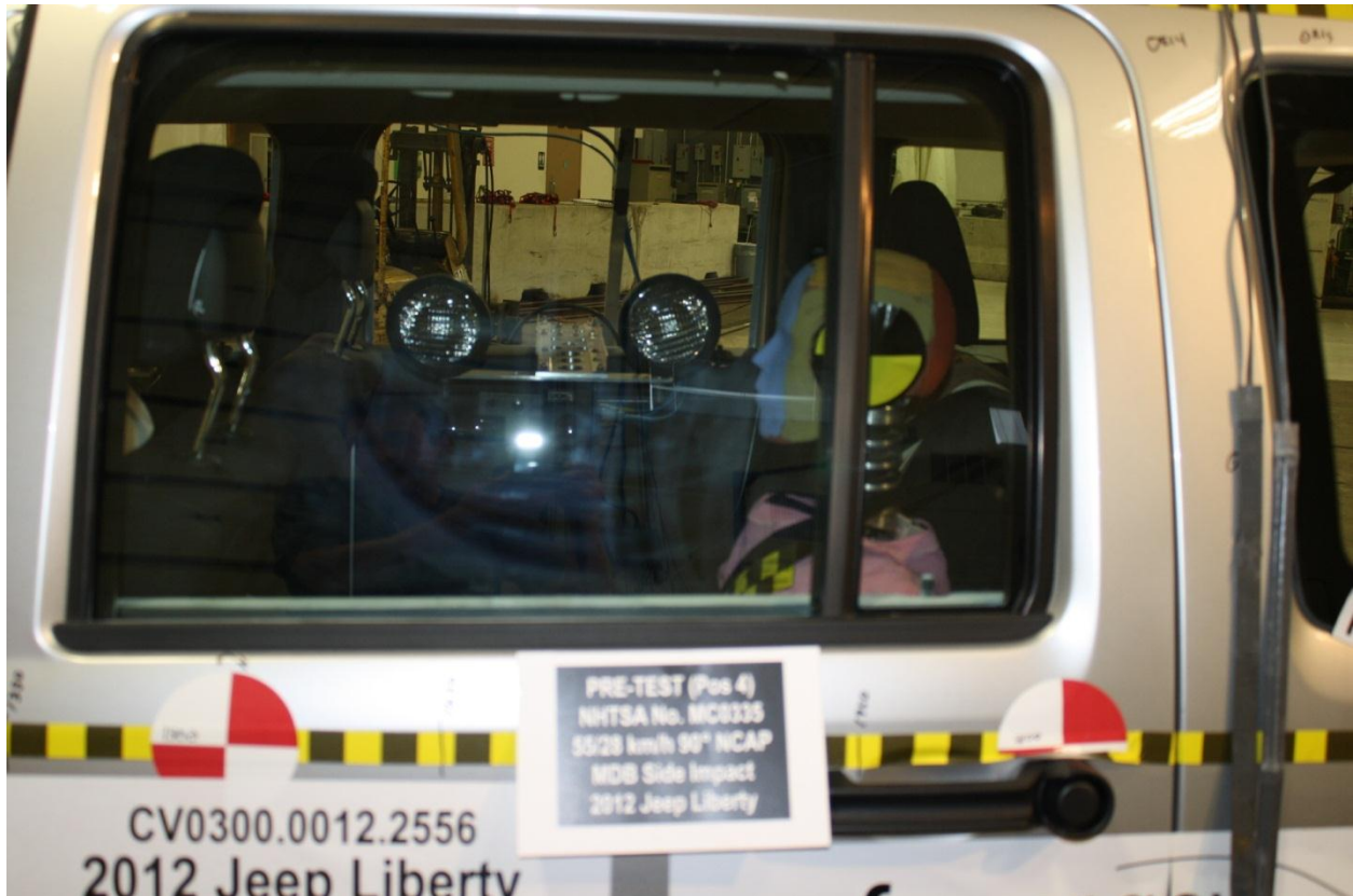
Figure A-55: Pre-Test Left Side View of Passenger Dummy Shoulder and Door Top View
