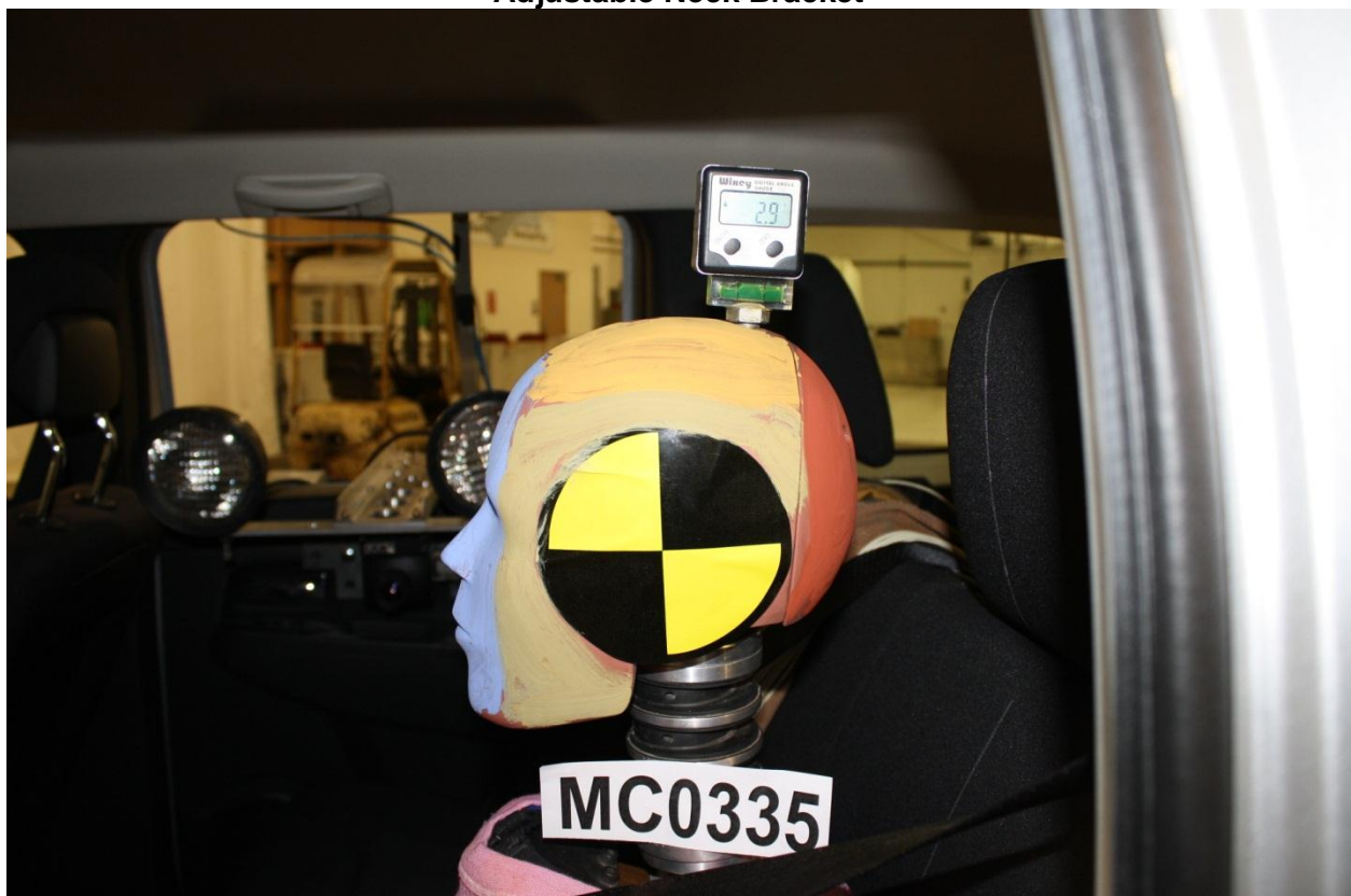
Figure A-62: Pre-Test View of Rear Passenger Dummy's Head Showing Dummy's Head is Level
