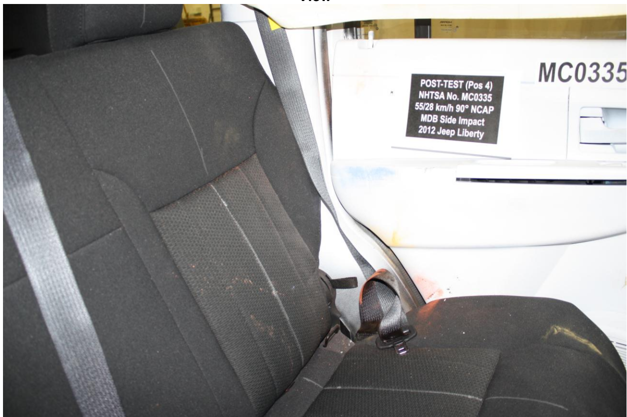
Figure A-76: Post-Test Rear Passenger Dummy Close-Up Torso Contact with Vehicle Interior View
