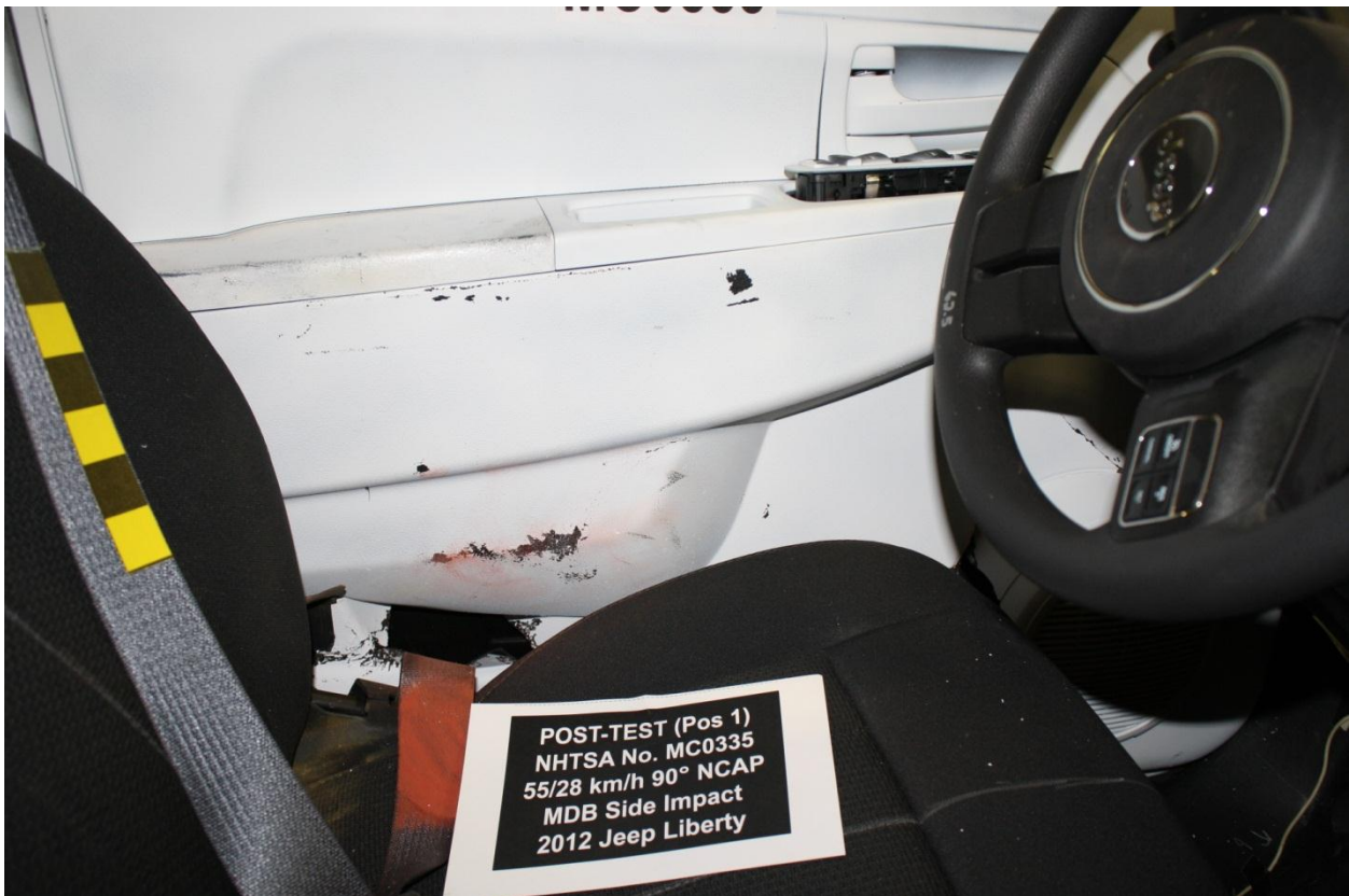
Figure A-52: Post-Test Driver Dummy Close-Up Pelvis Contact with Vehicle Interior View
