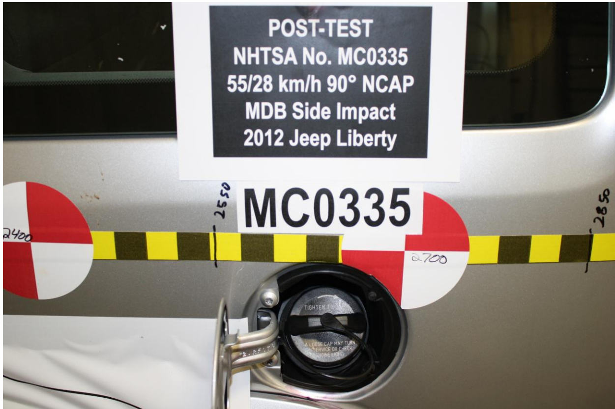
Figure A-81: Post-Test View of Fuel Filler Cap or Fuel Filler Neck
