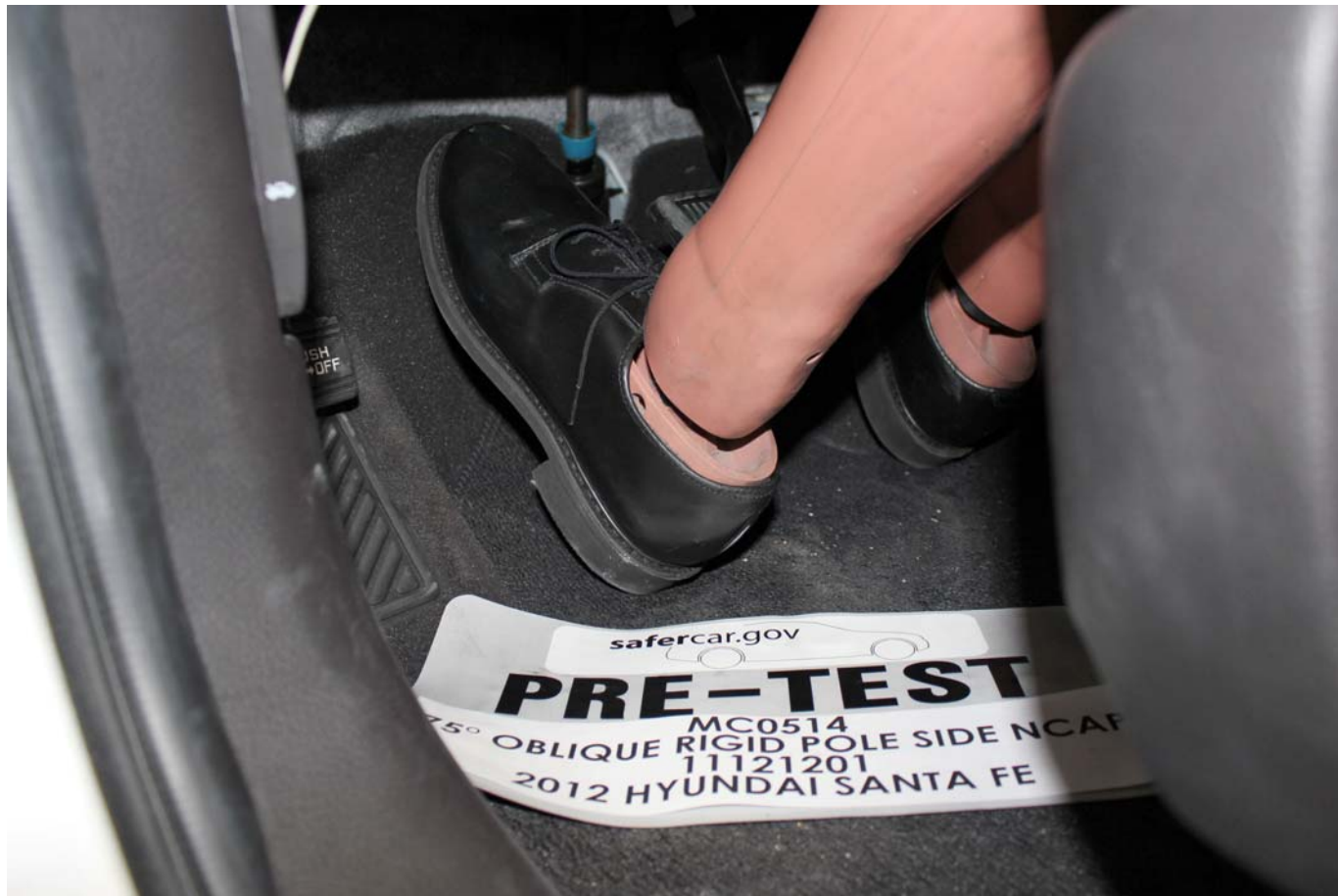
Pre-Test Placement of Dummy's Feet
