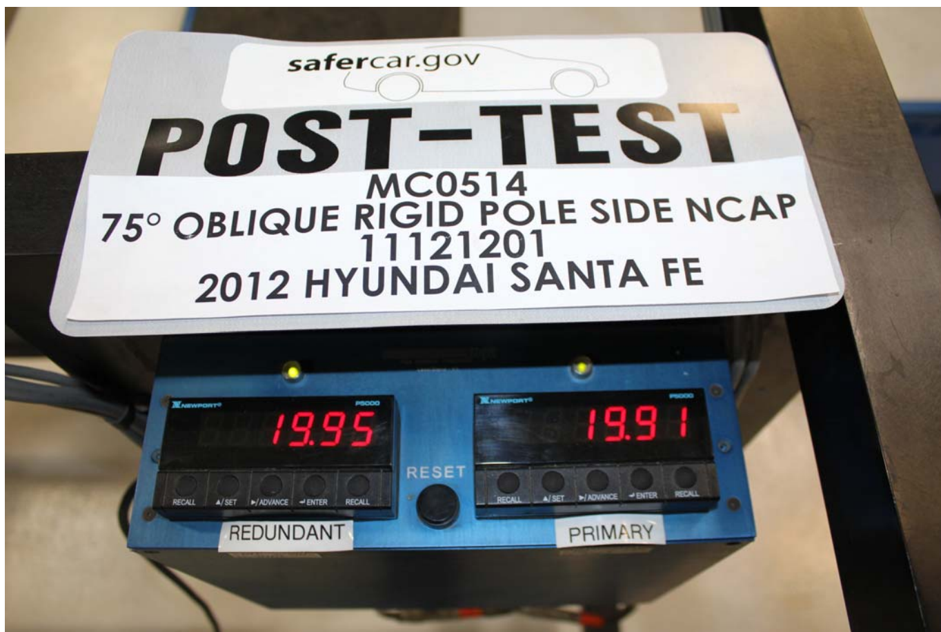
Post-Test Primary and Redundant Speed Trap Read-Out
