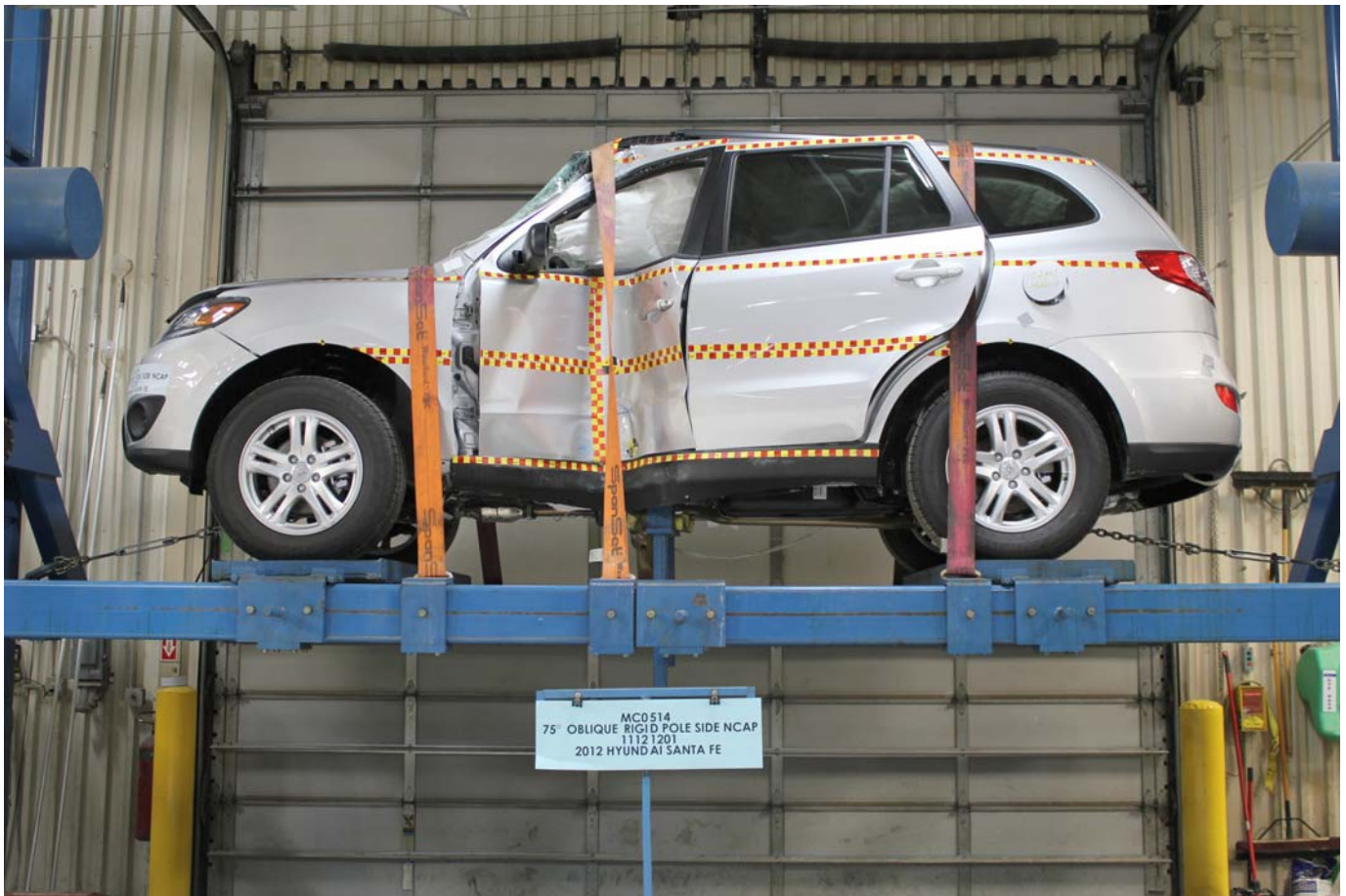
FMVSS No. 301 Static Rollover 360 Degrees
