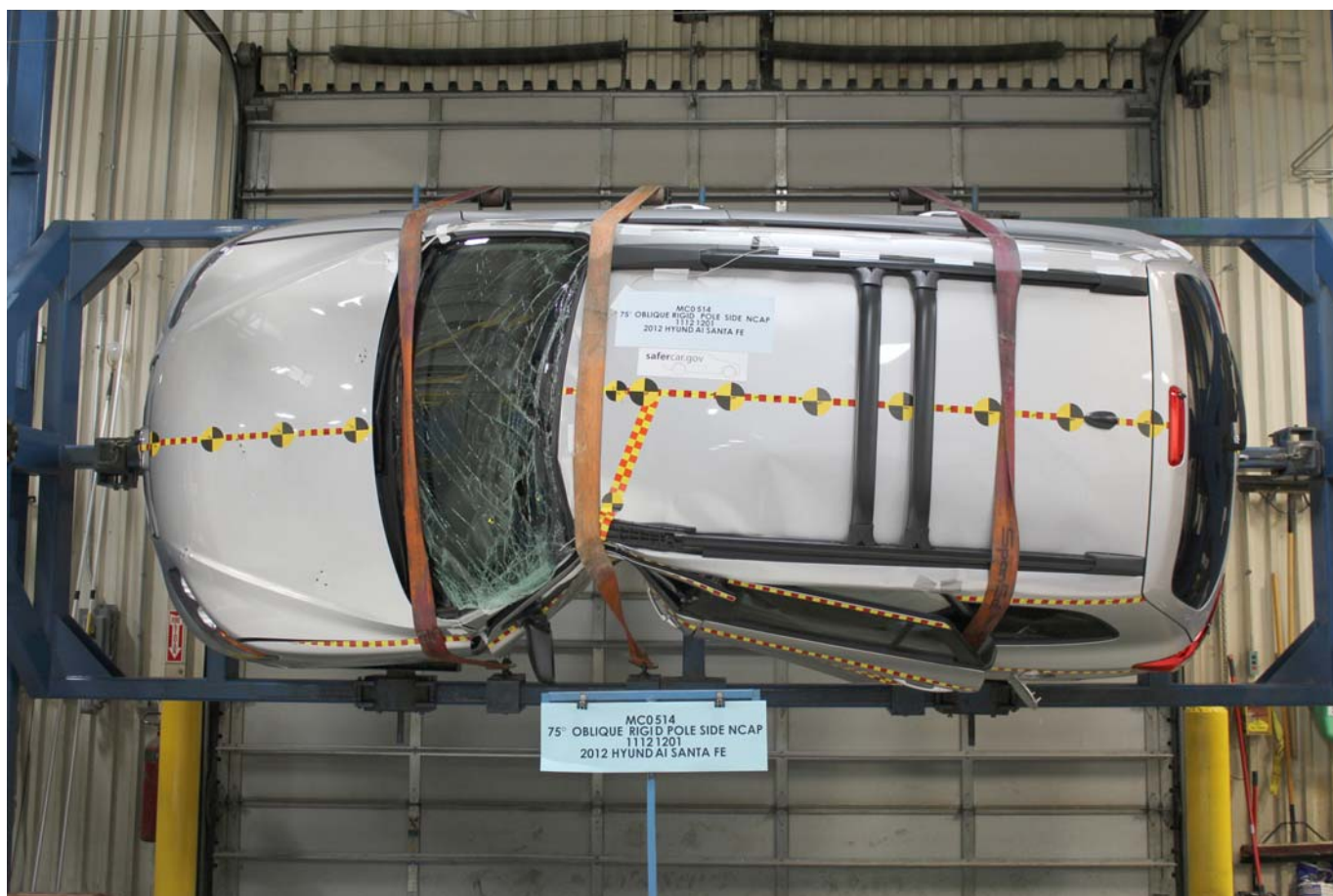
FMVSS No. 301 Static Rollover 90 Degrees
