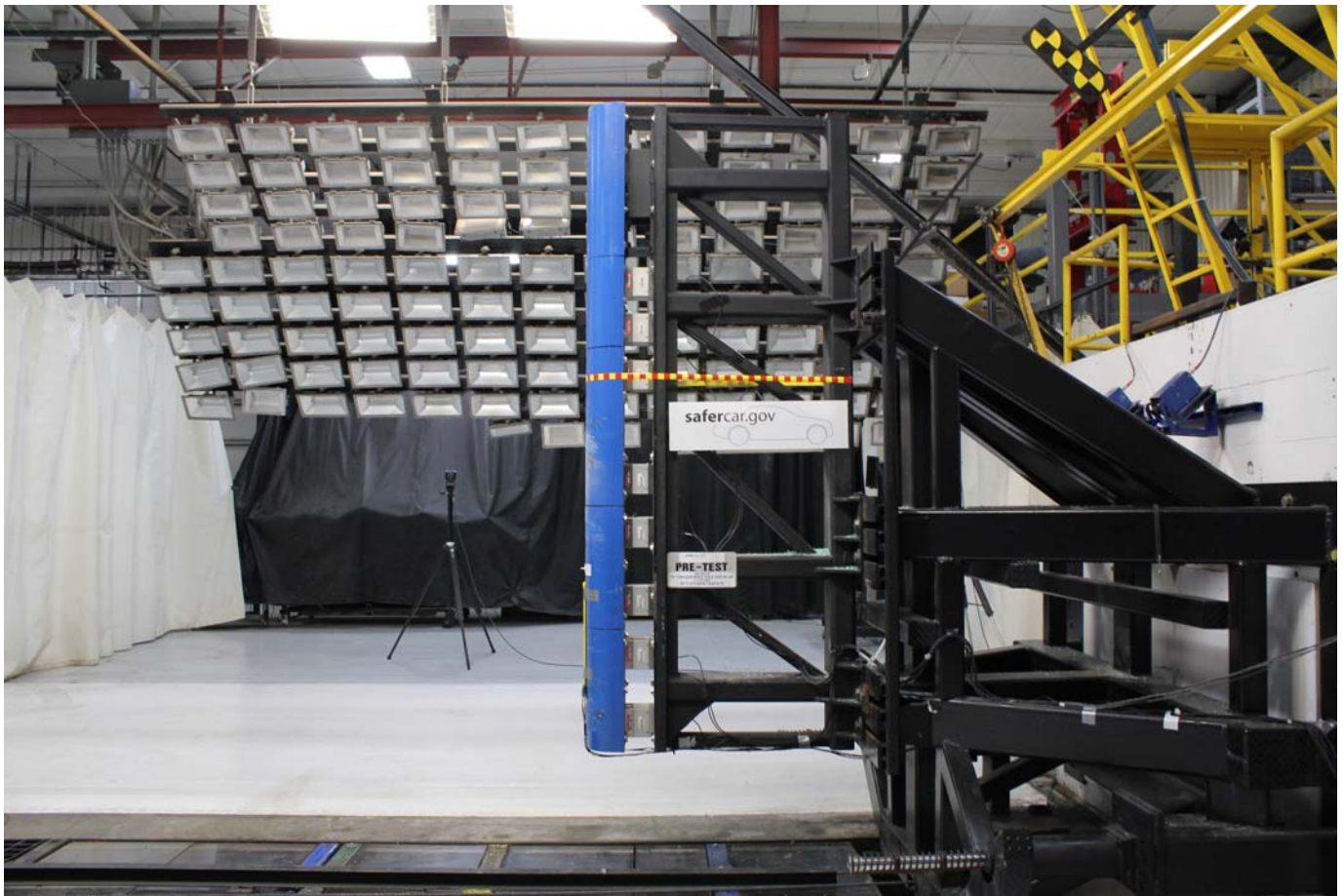
Pre-Test Pole Barrier Side View
