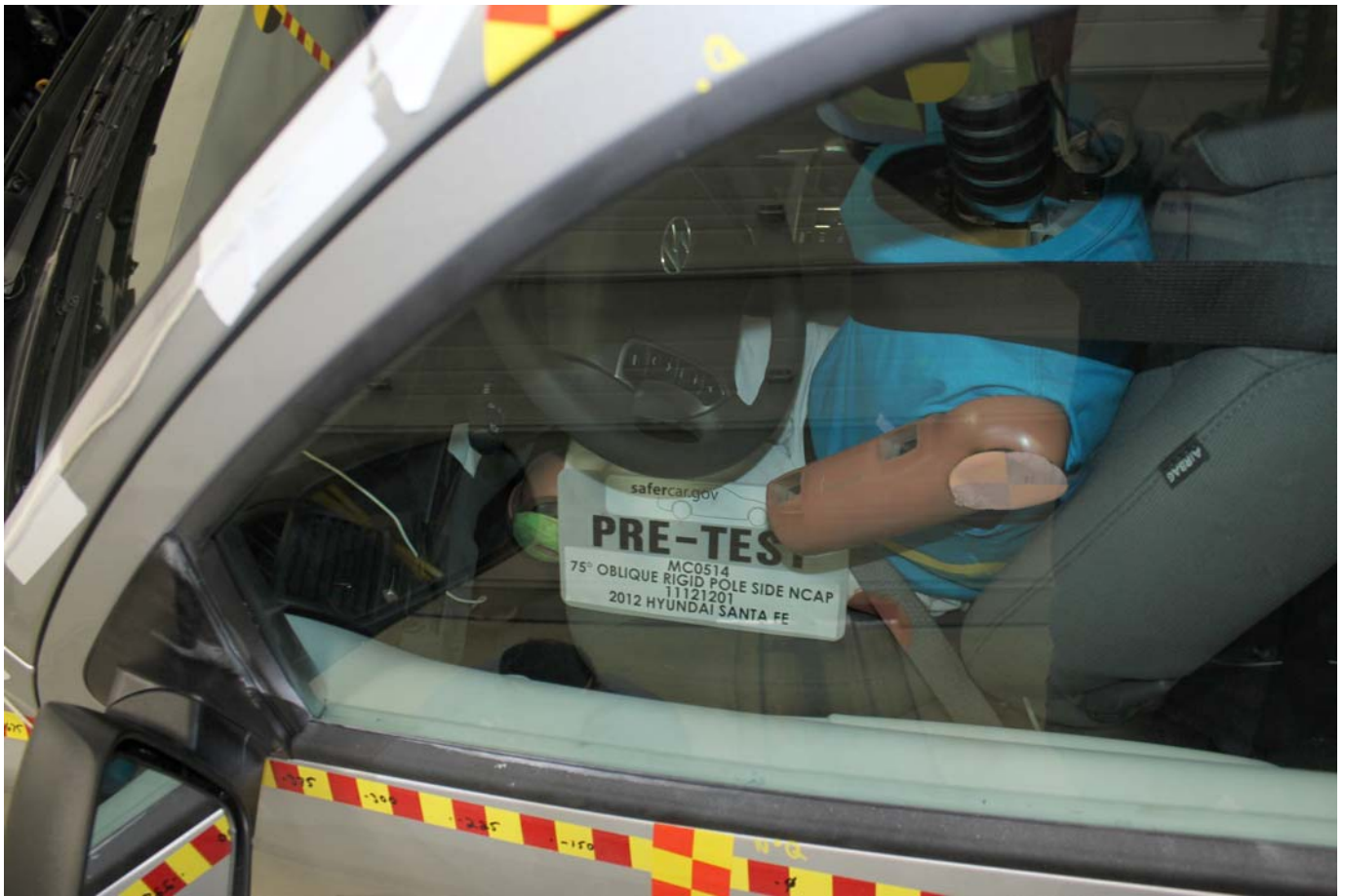
Pre-Test Dummy and Door Clearance View
