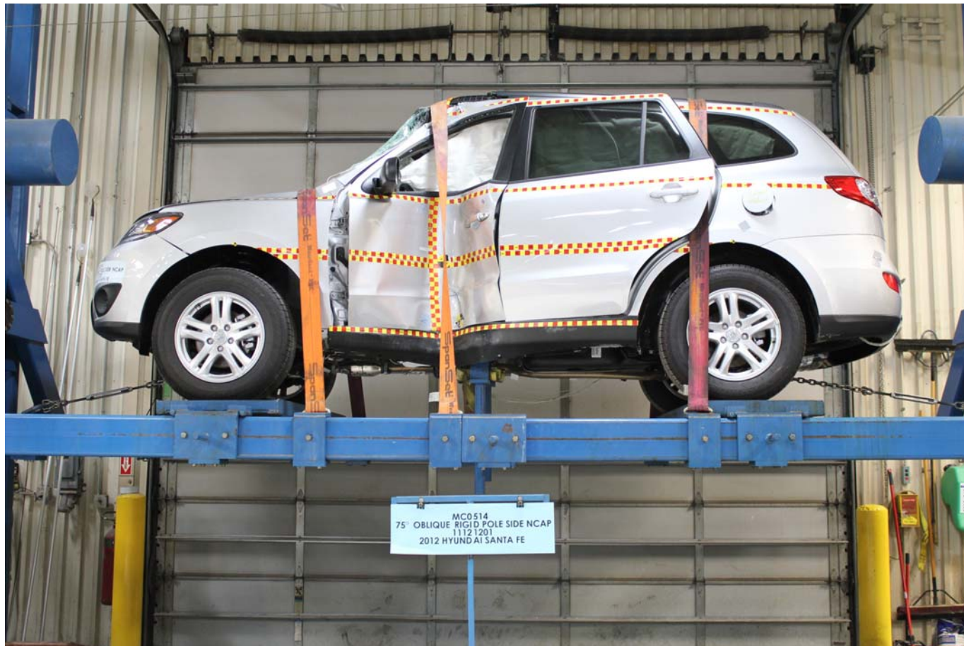
FMVSS No. 301 Static Rollover 0 Degrees
