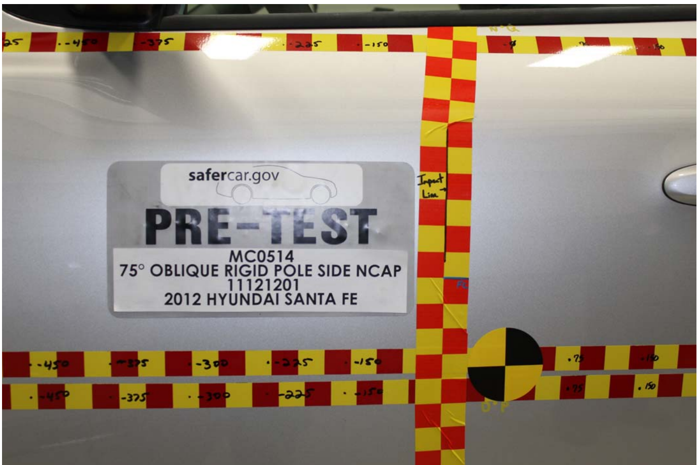
Pre-Test Close-Up View of Impact Point Target
