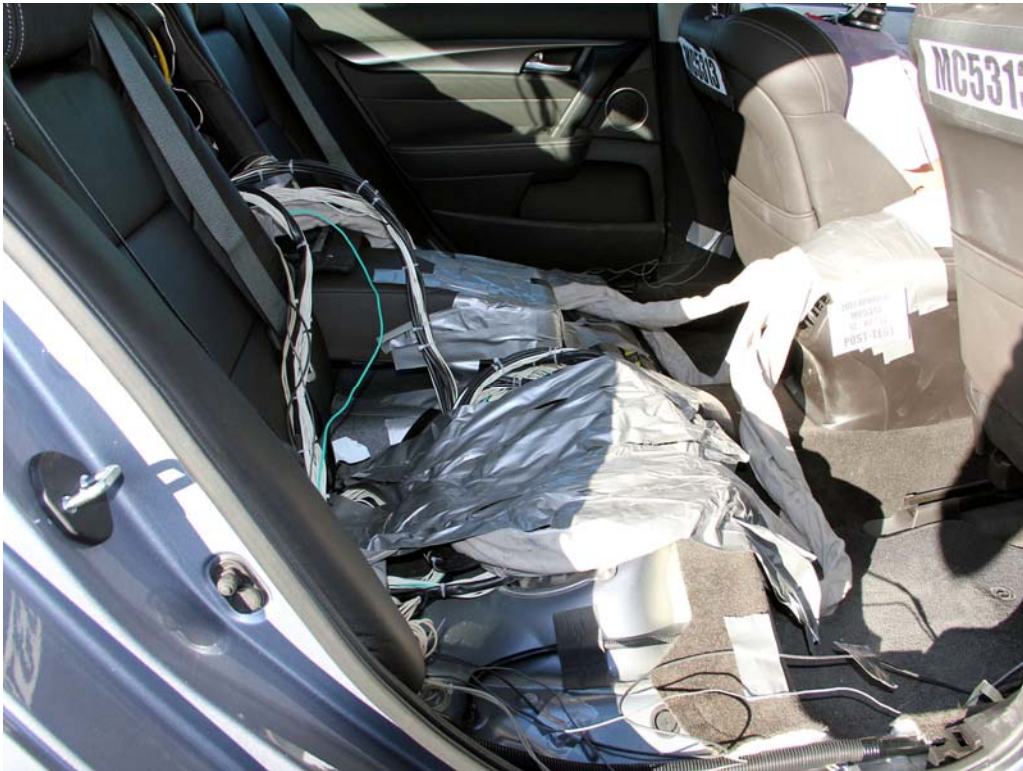
FIGURE 28. Post-Test Dummy Cable Routing
