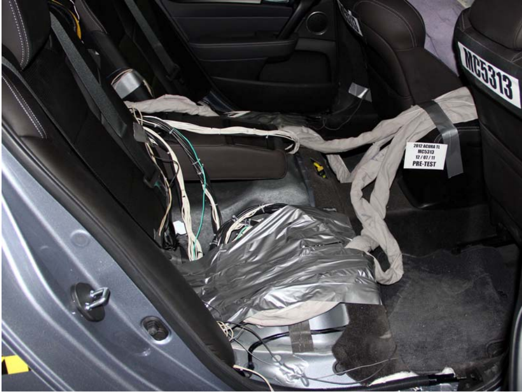
FIGURE 27. Pre-Test Dummy Cable Routing
