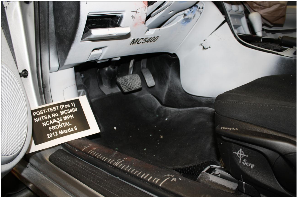
Figure A-42: Post-Test Driver's Side Floorpan
