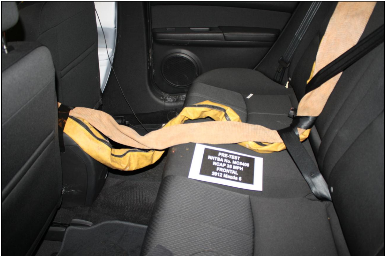
Figure A-27: Pre-Test Dummy Cable Routing
