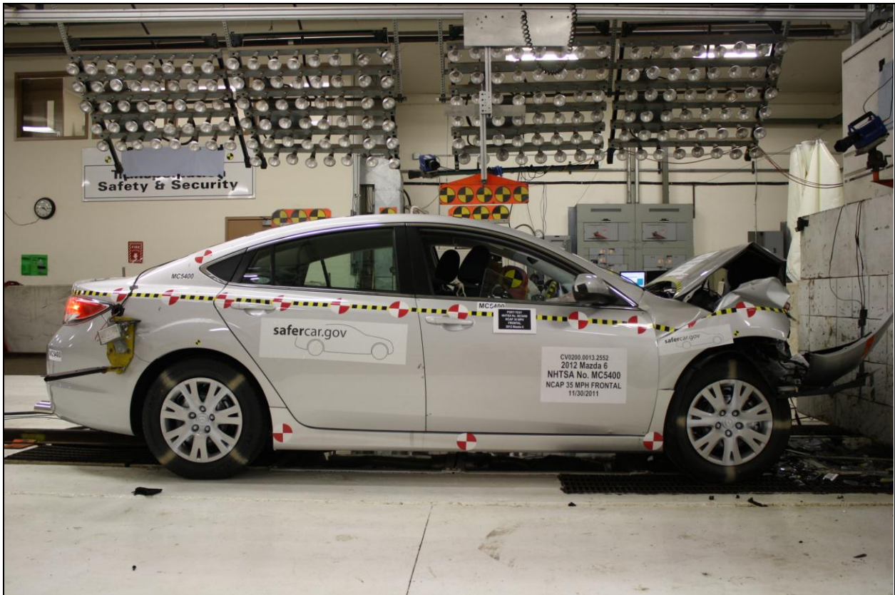
Figure A-12: Post-Test Right View of Test Vehicle
