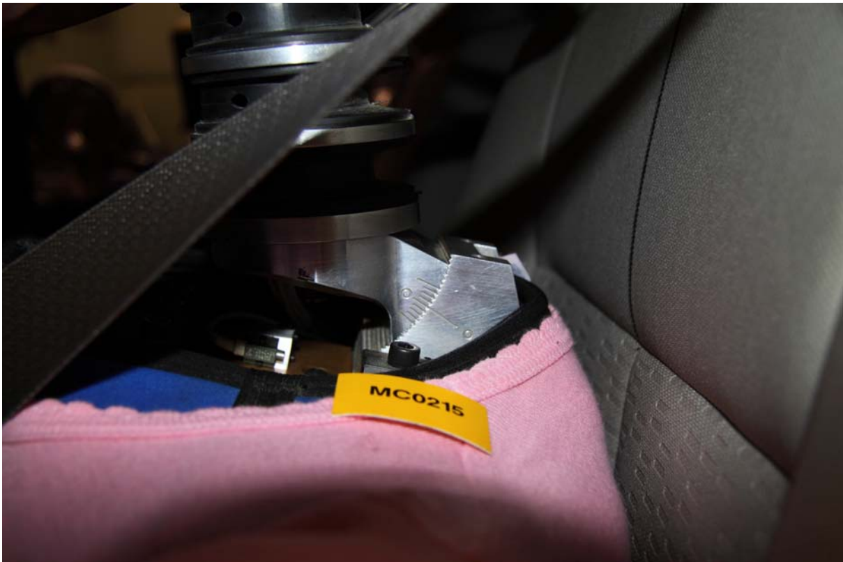
030 Pre-Test Left Side View of Dummy's Neck Showing Position of Adjustable Neck Bracket
