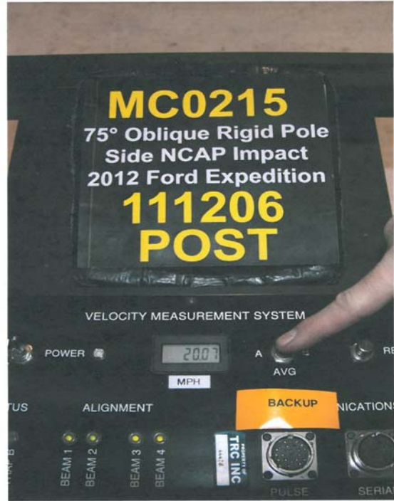
061 Post-Test Primary and Redundant Speed Trap Read-Out
