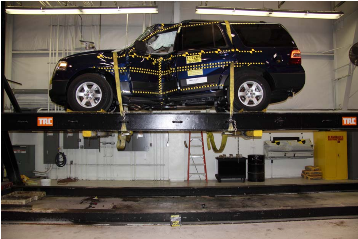
066 FMVSS No. 301 Static Rollover 360 Degrees
