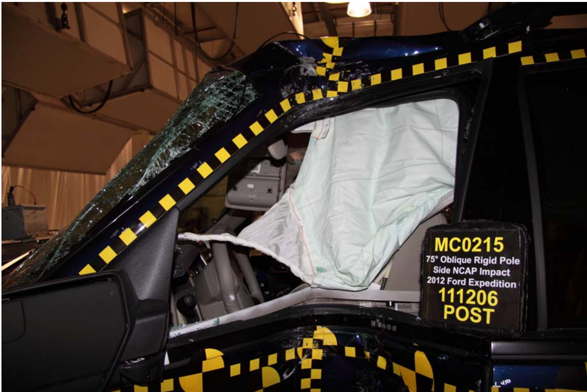
025 Post-Test Left Side View of Dummy Shoulder and Door Top View
