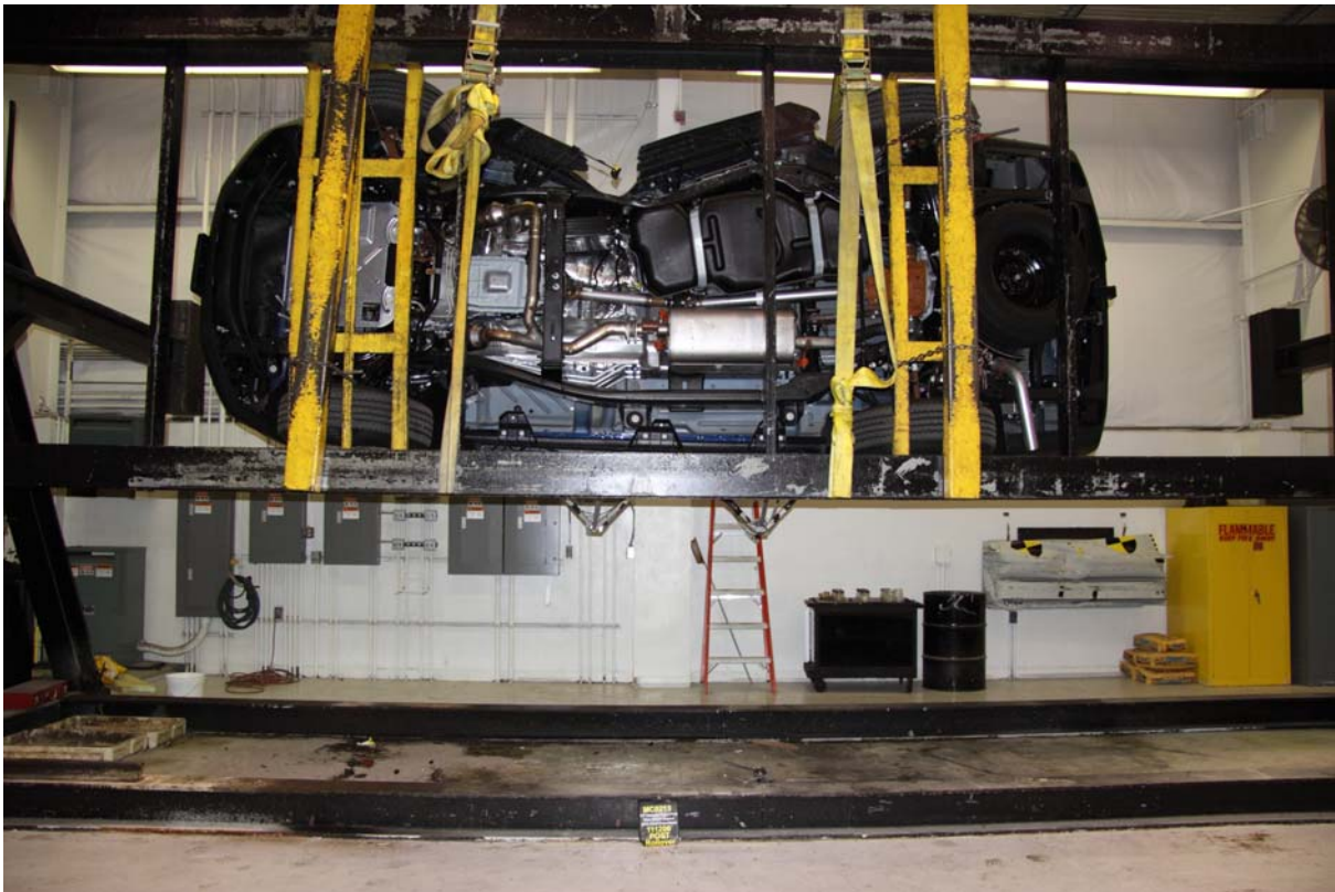
065 FMVSS No. 301 Static Rollover 270 Degrees
