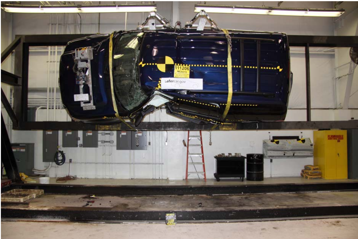
063 FMVSS No. 301 Static Rollover 90 Degrees
