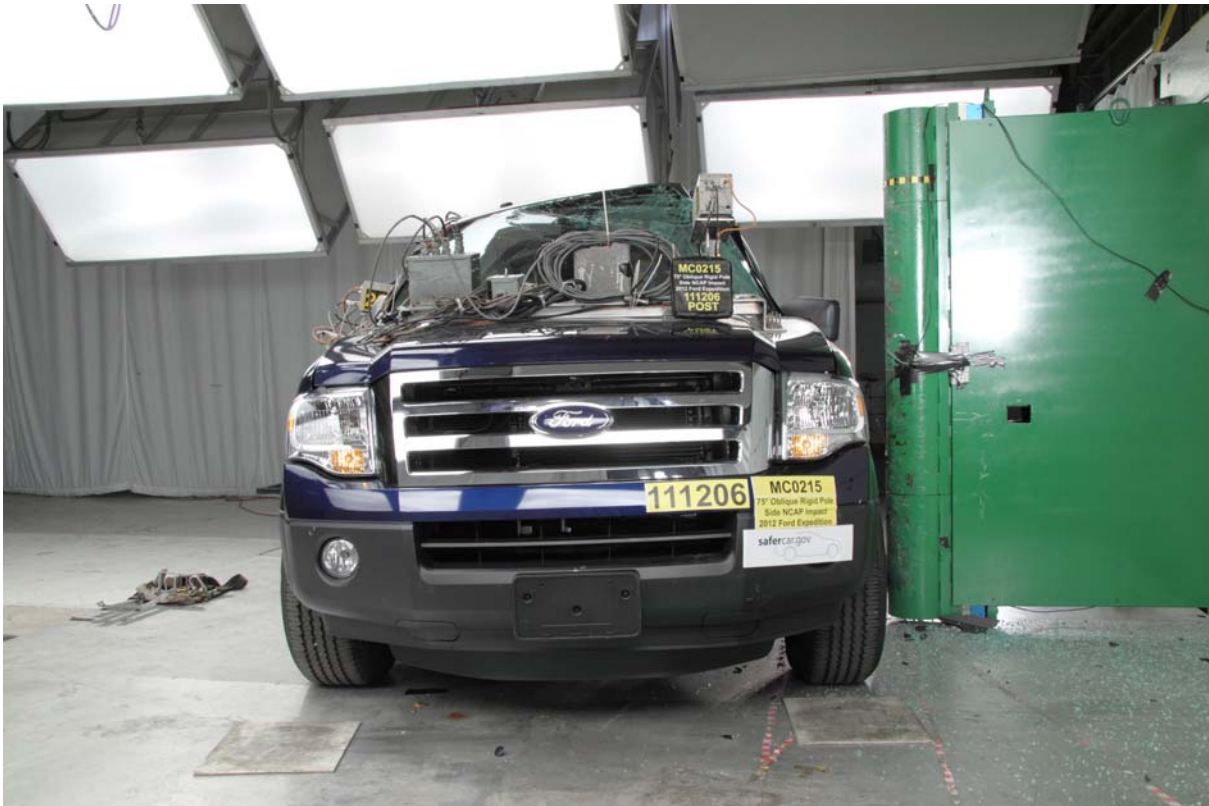
004 Post-Test Frontal View of Test Vehicle
