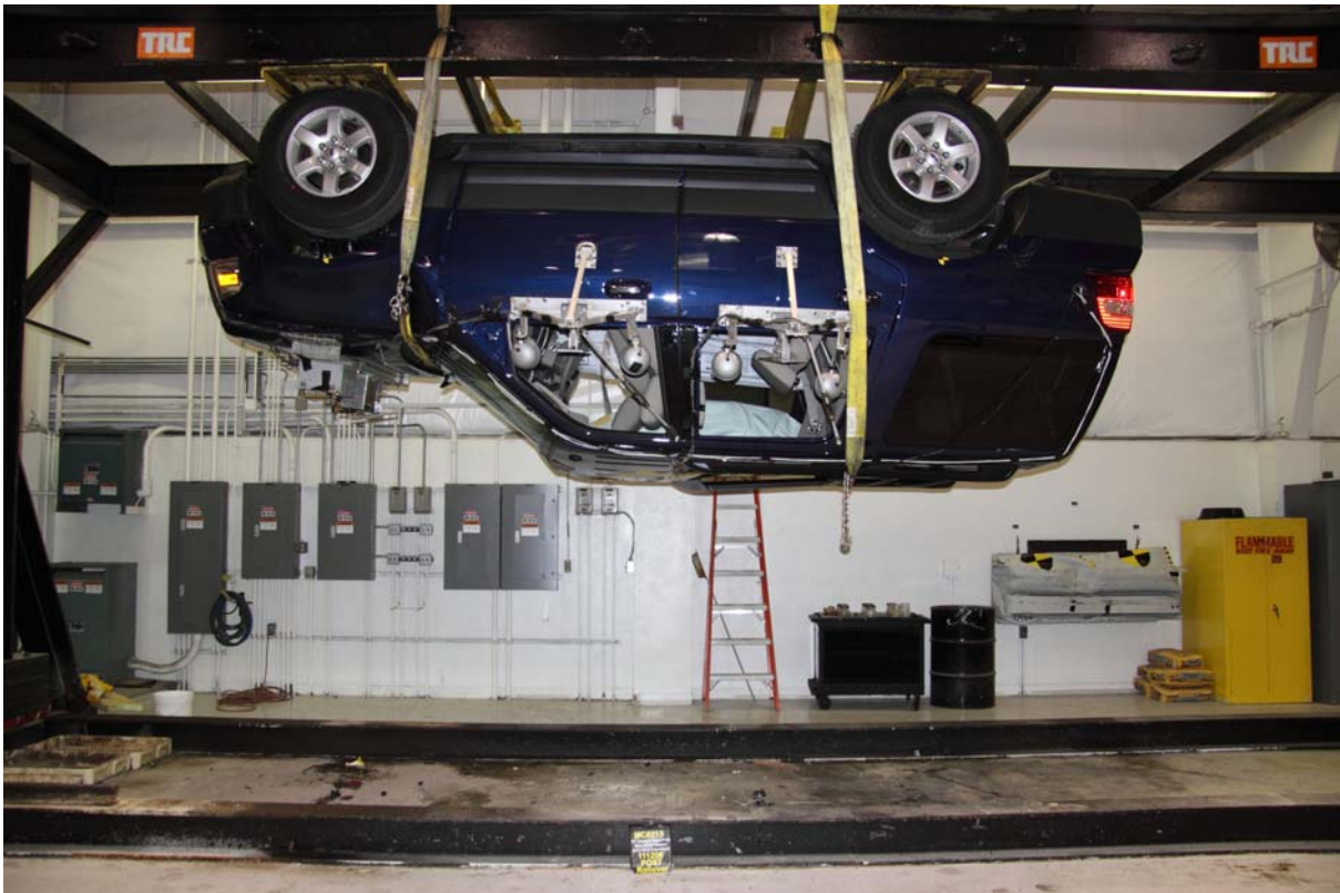
064 FMVSS No. 301 Static Rollover 180 Degrees
