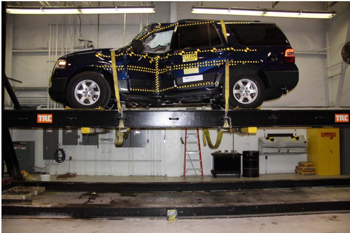
062 FMVSS No. 301 Static Rollover 0 Degrees
