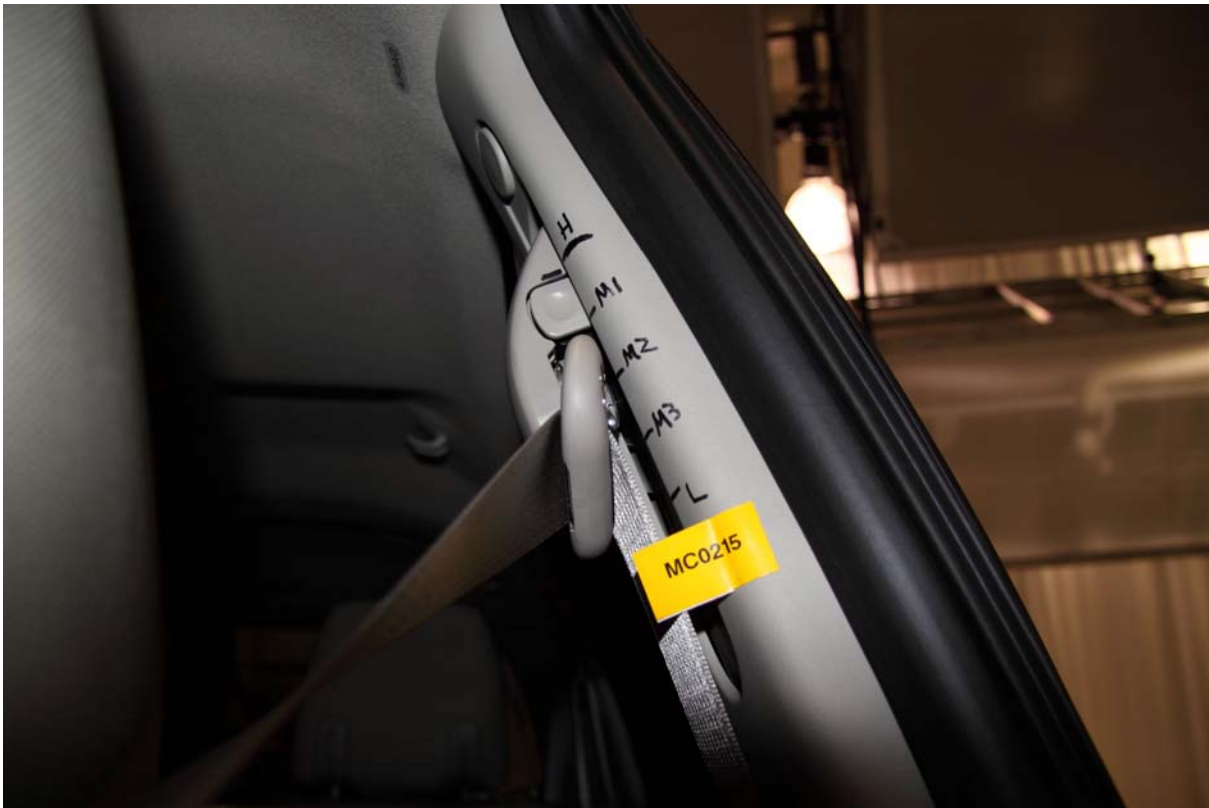
033 Pre-Test View of Belt Anchorage for Dummy
