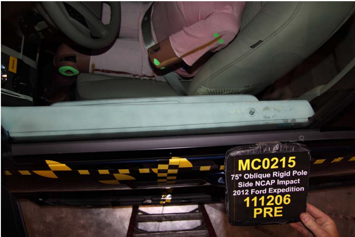
040 Pre-Test Dummy and Door Clearance View
