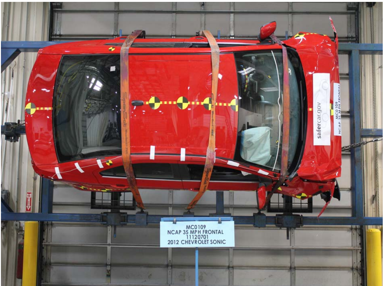
Vehicle at 90 Degrees on Static Rollover Device
