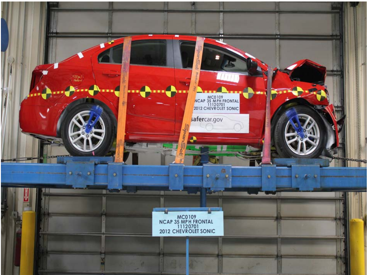
Vehicle at 0 Degrees on Static Rollover Device
