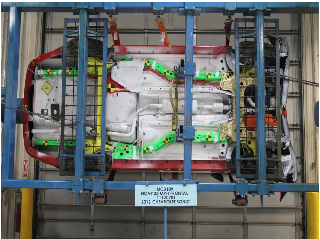
Vehicle at 270 Degrees on Static Rollover Device
