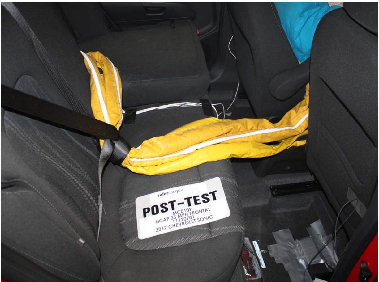
Post-Test Dummy Cable Routing
