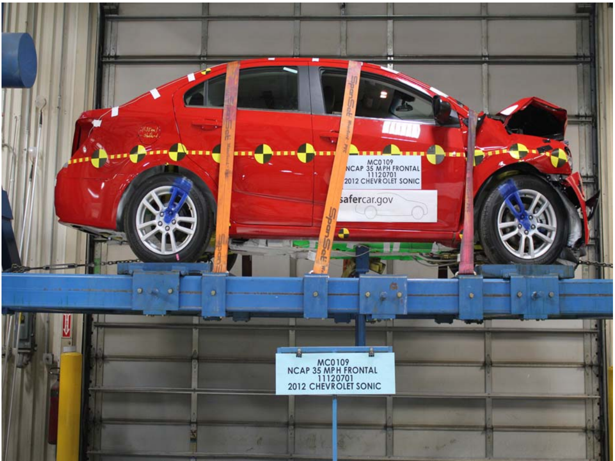
Vehicle at 360 Degrees on Static Rollover Device
