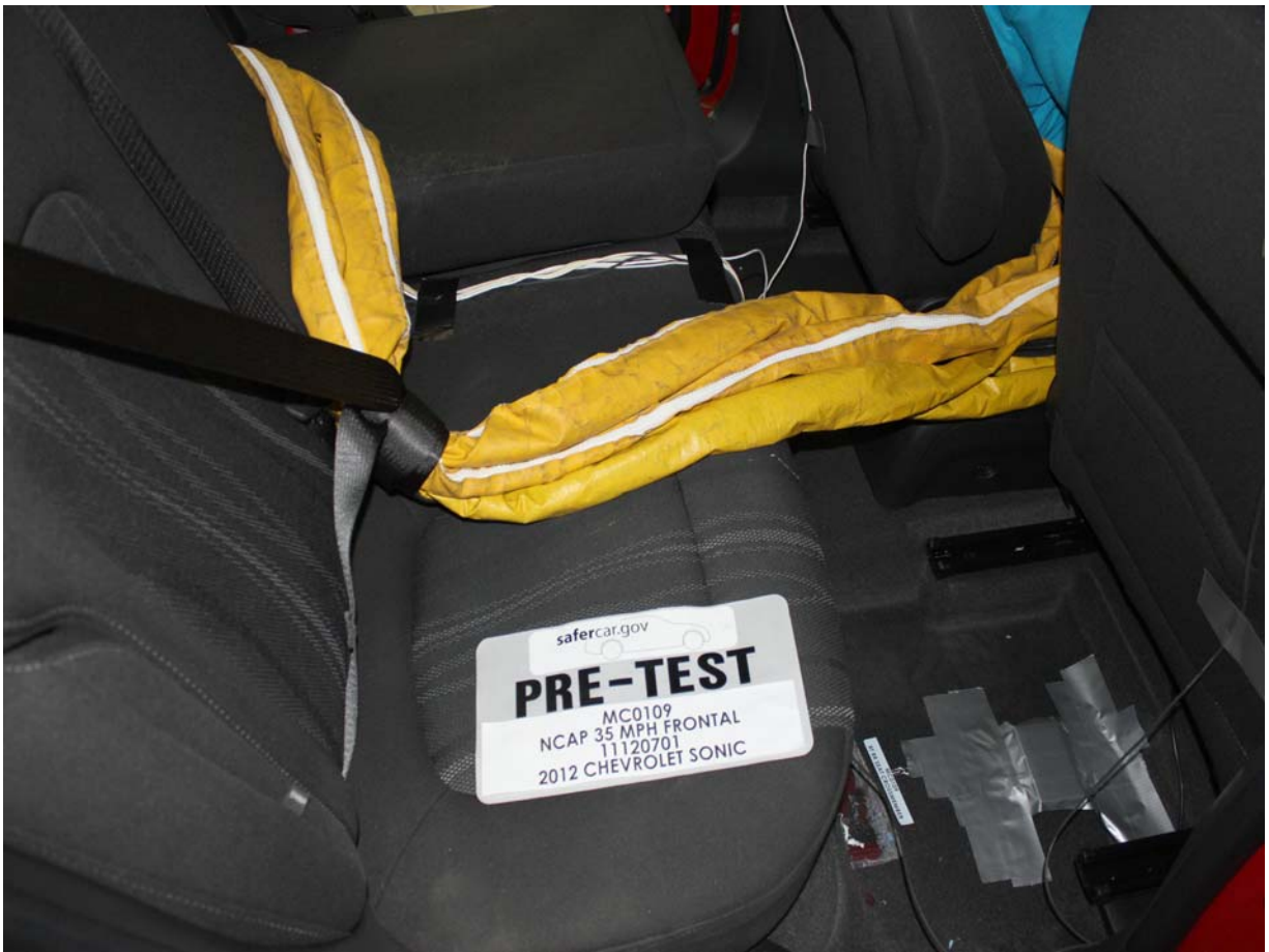
Pre-Test Dummy Cable Routing
