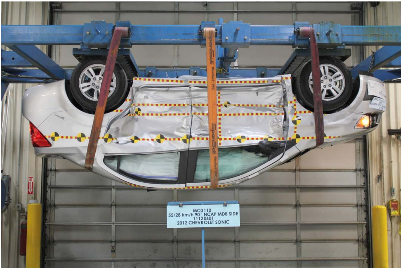
FMVSS No. 301 Static Rollover 180 Degrees
