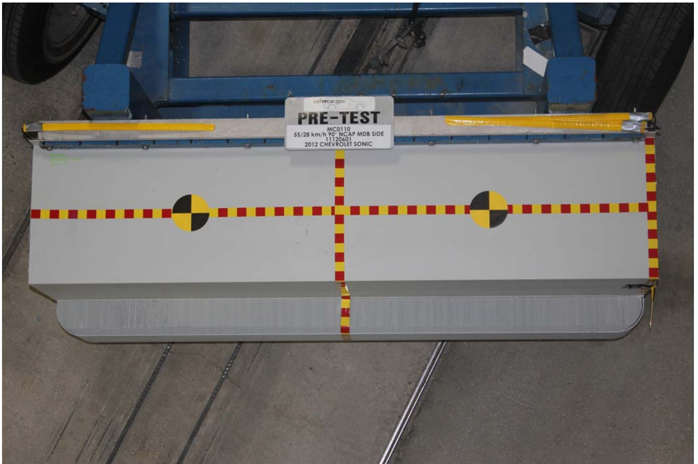
Pre-Test Top View of MDB Impactor Face
