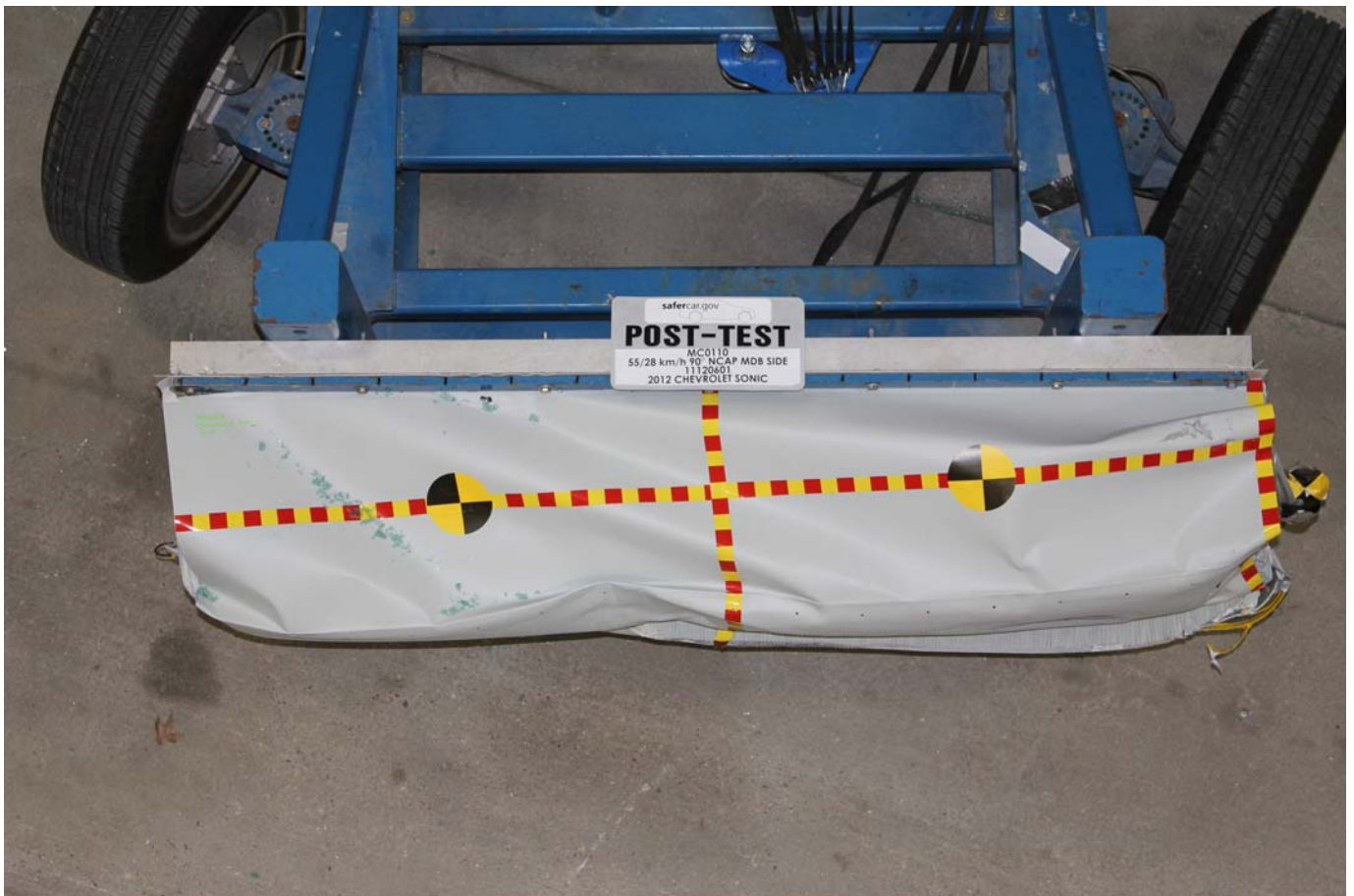
Post-Test Top View of MDB Impactor Face
