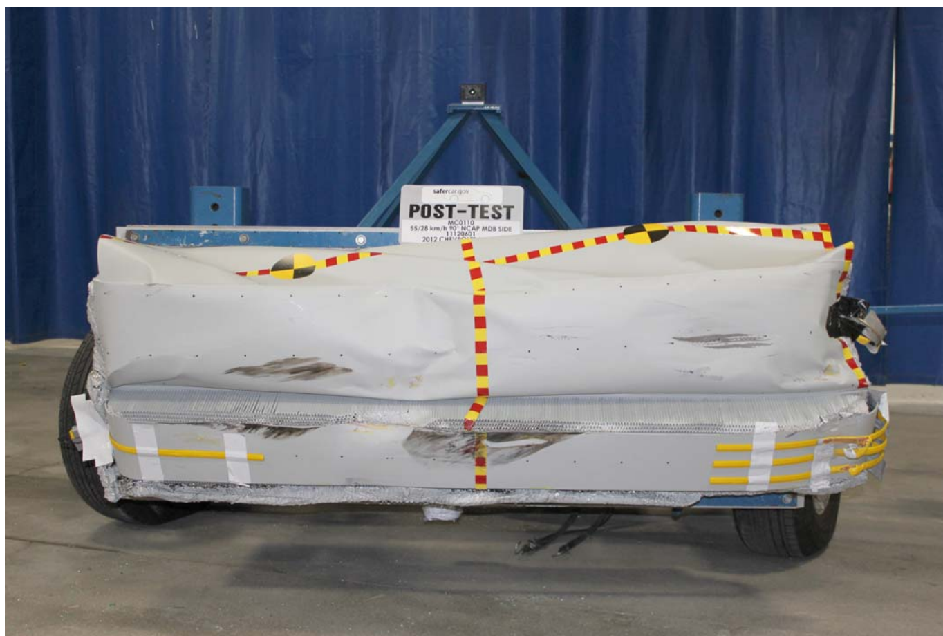
Post-Test Front View of MDB Impactor Face
