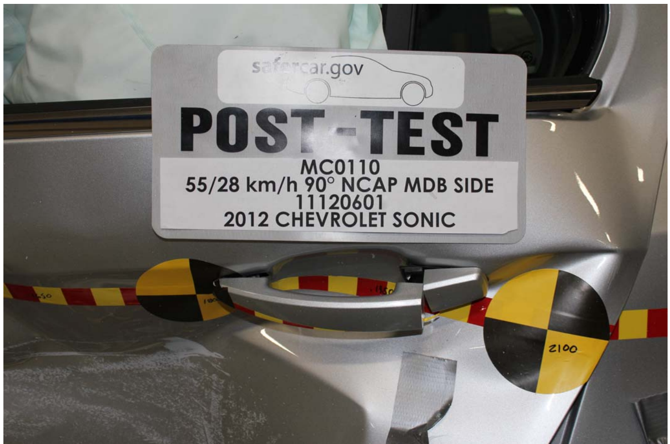
Post-Test Left Rear Door Latch Close-Up
