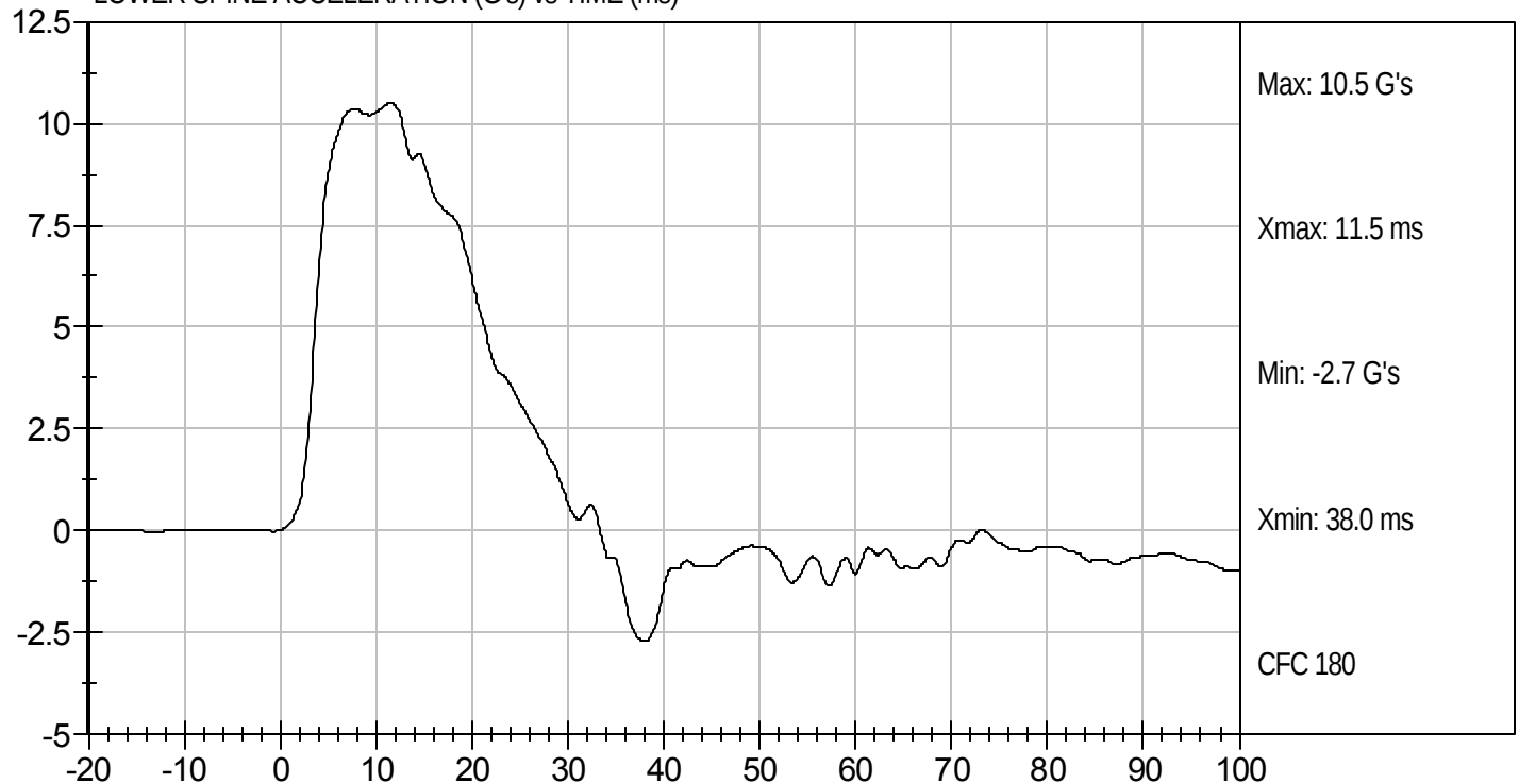
LOWER SPINE ACCELERATION (G's) vs TIME (ms)
