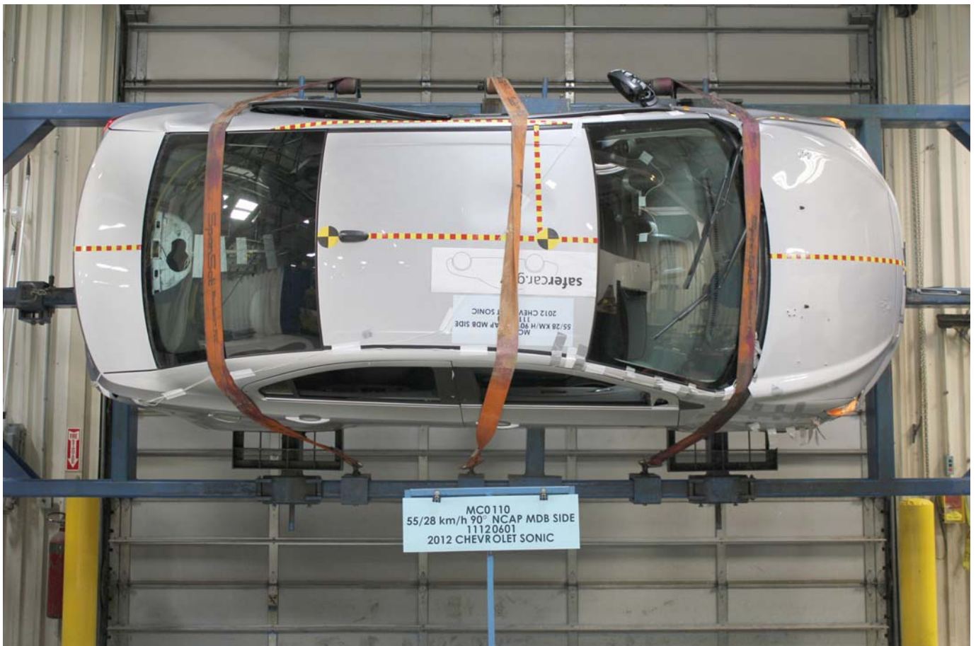
FMVSS No. 301 Static Rollover 90 Degrees
