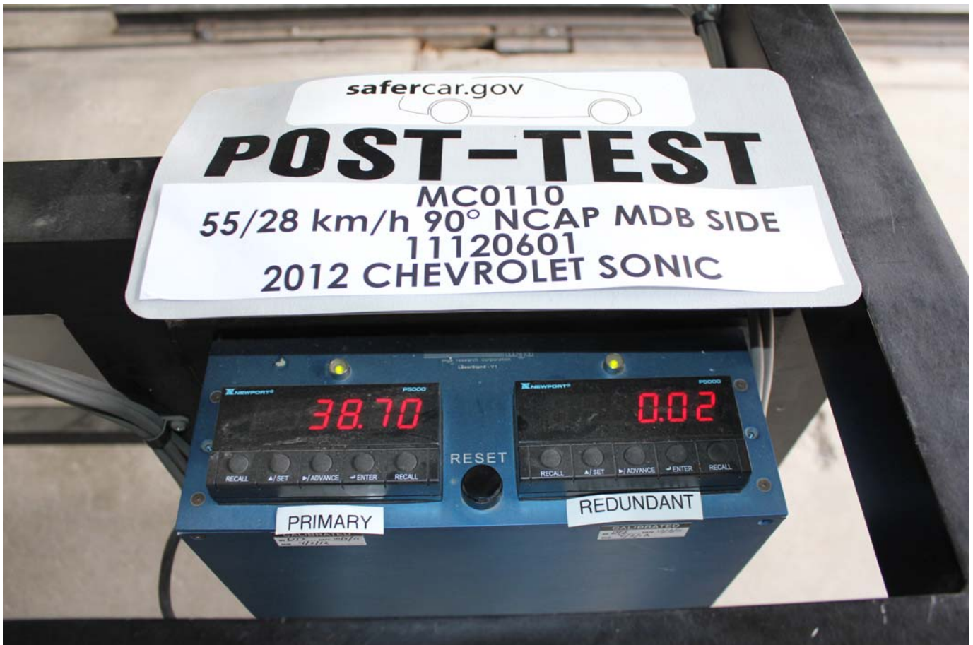
Post-Test Primary and Redundant Speed Trap Read-Out
