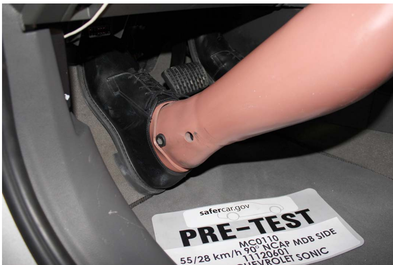
Pre-Test Placement of Driver Dummy's Feet
