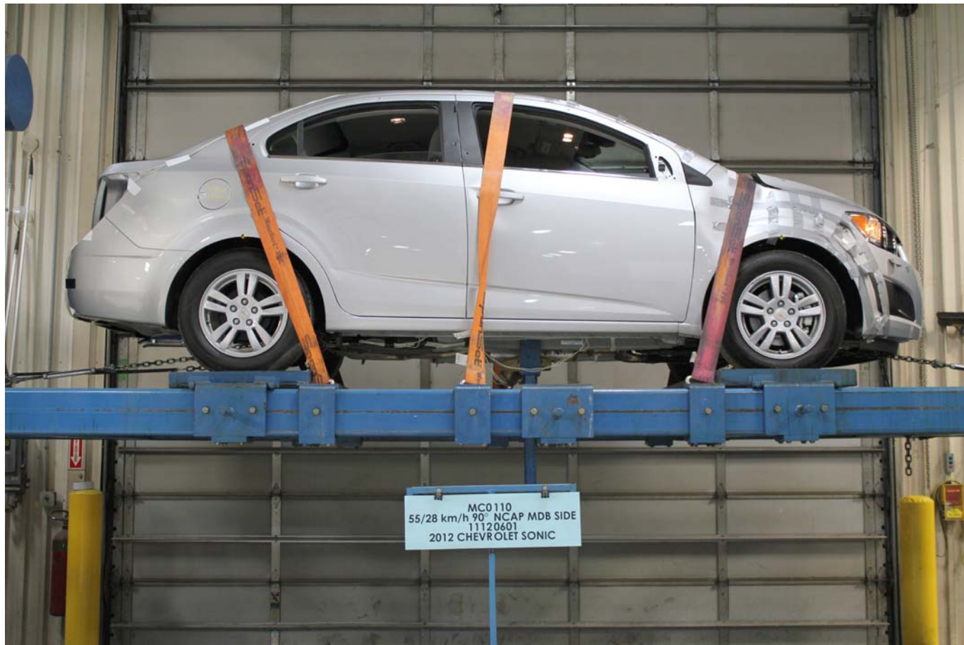
FMVSS No. 301 Static Rollover 360 Degrees
