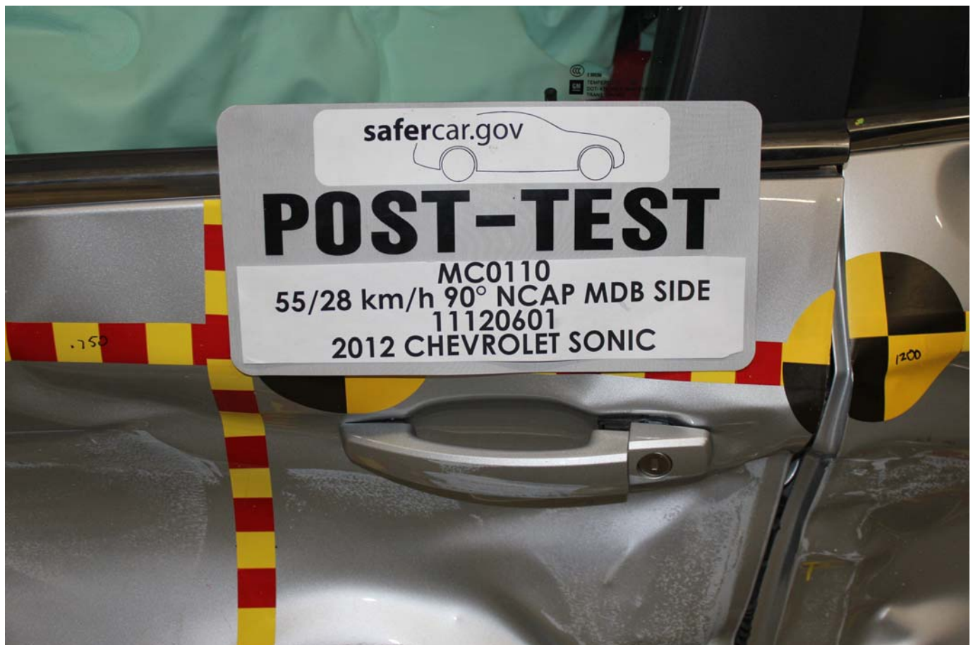
Post-Test Left Front Door Latch Close-Up
