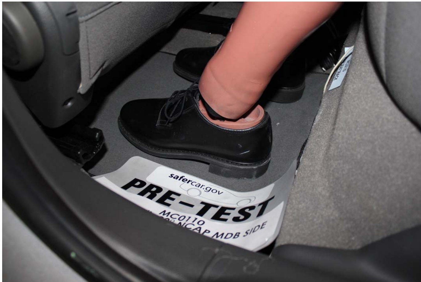
Pre-Test Placement of Rear Passenger Dummy's Feet
