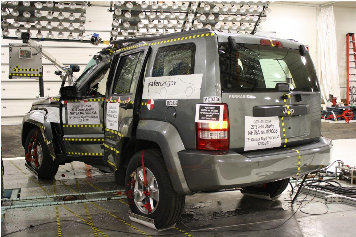
Figure A-10: Post-Test Left Rear ¾ View of Test Vehicle
