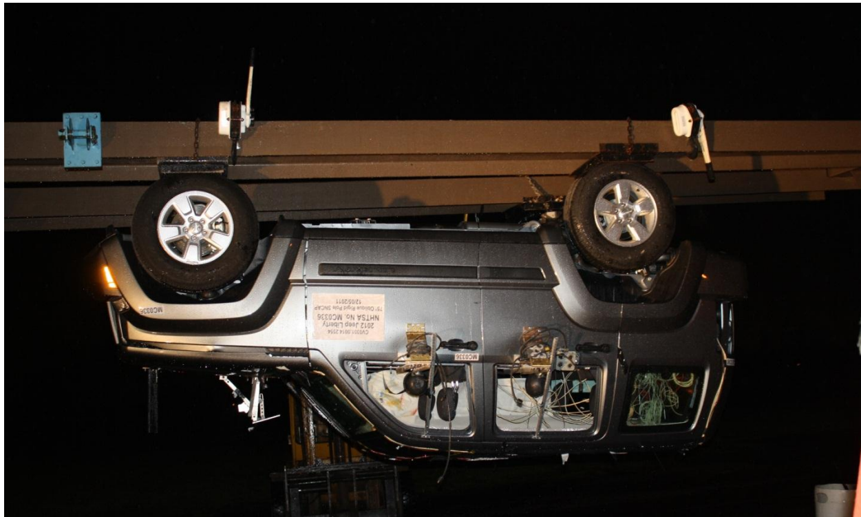
Figure A-64: FMVSS No. 301 Static Rollover 180 Degrees
