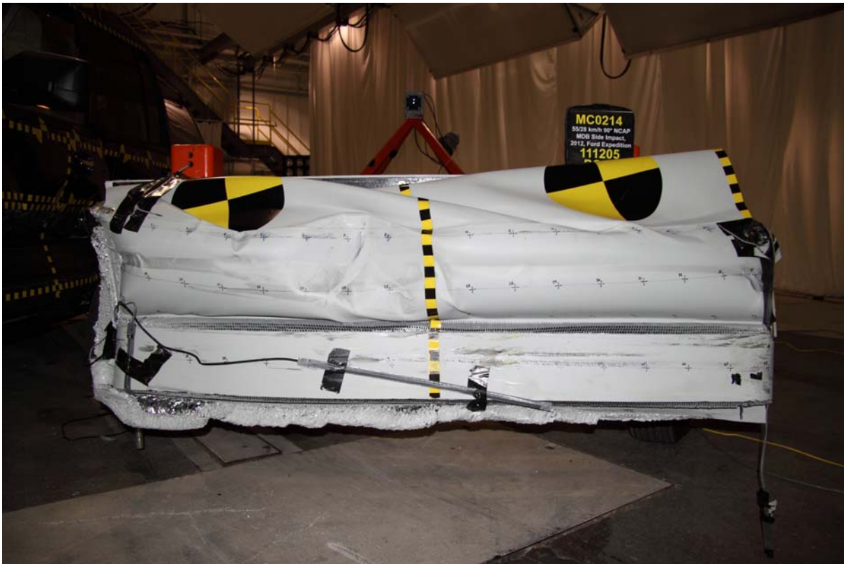
083 Post-Test Front View of MDB Impactor Face
