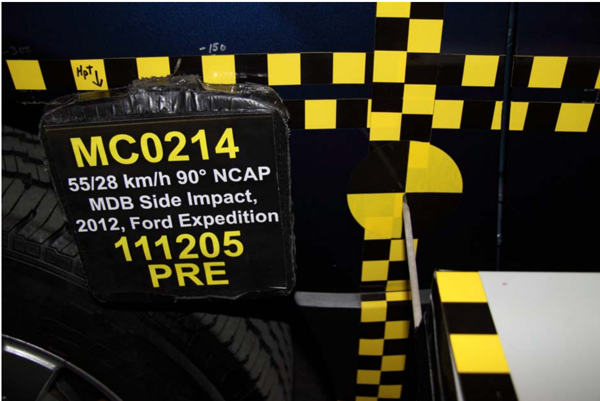
019 Pre-Test Close-up View of Impact Point Target
