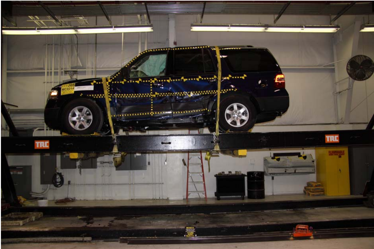
094 FMVSS No. 301 Static Rollover 0 Degrees
