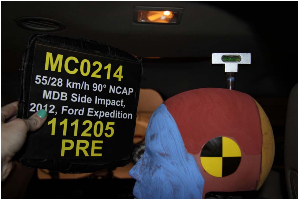
062 Pre-Test View of Rear Passenger Dummy Head Showing Dummy Head is Level
