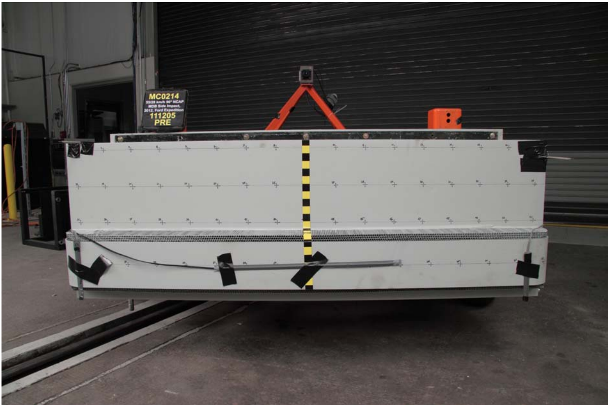
082 Pre-Test Front View of MDB Impactor Face
