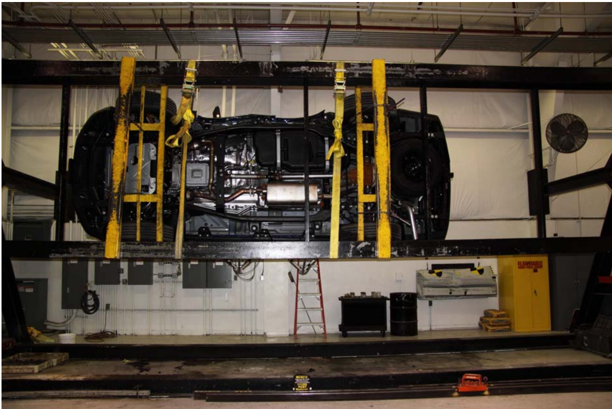
097 FMVSS No. 301 Static Rollover 270 Degrees
