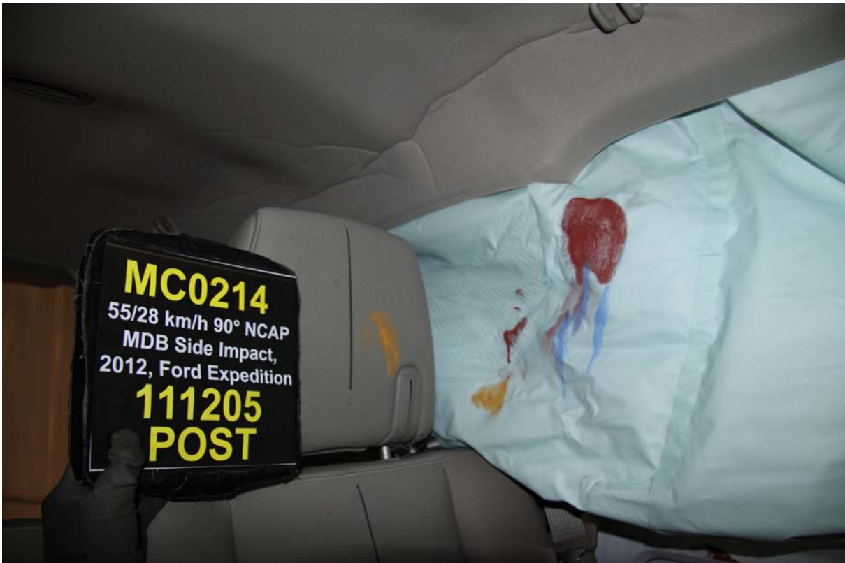
074 Post-Test Rear Passenger Dummy Close-Up Head Contact with Vehicle View
