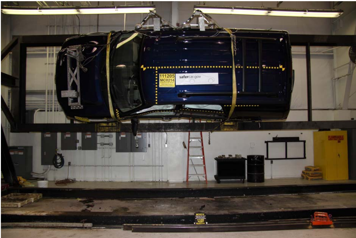
095 FMVSS No. 301 Static Rollover 90 Degrees
