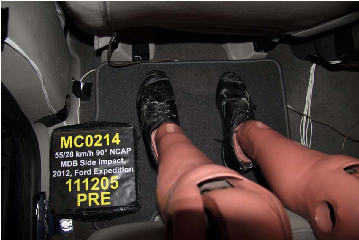
063 Pre-Test Placement of Rear Passenger Dummy Feet
