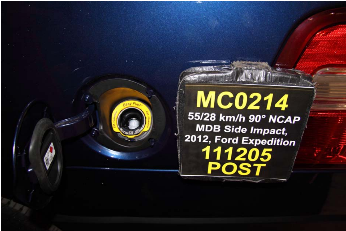
081 Post-Test View of Fuel Filler Cap or Fuel Filler Neck
