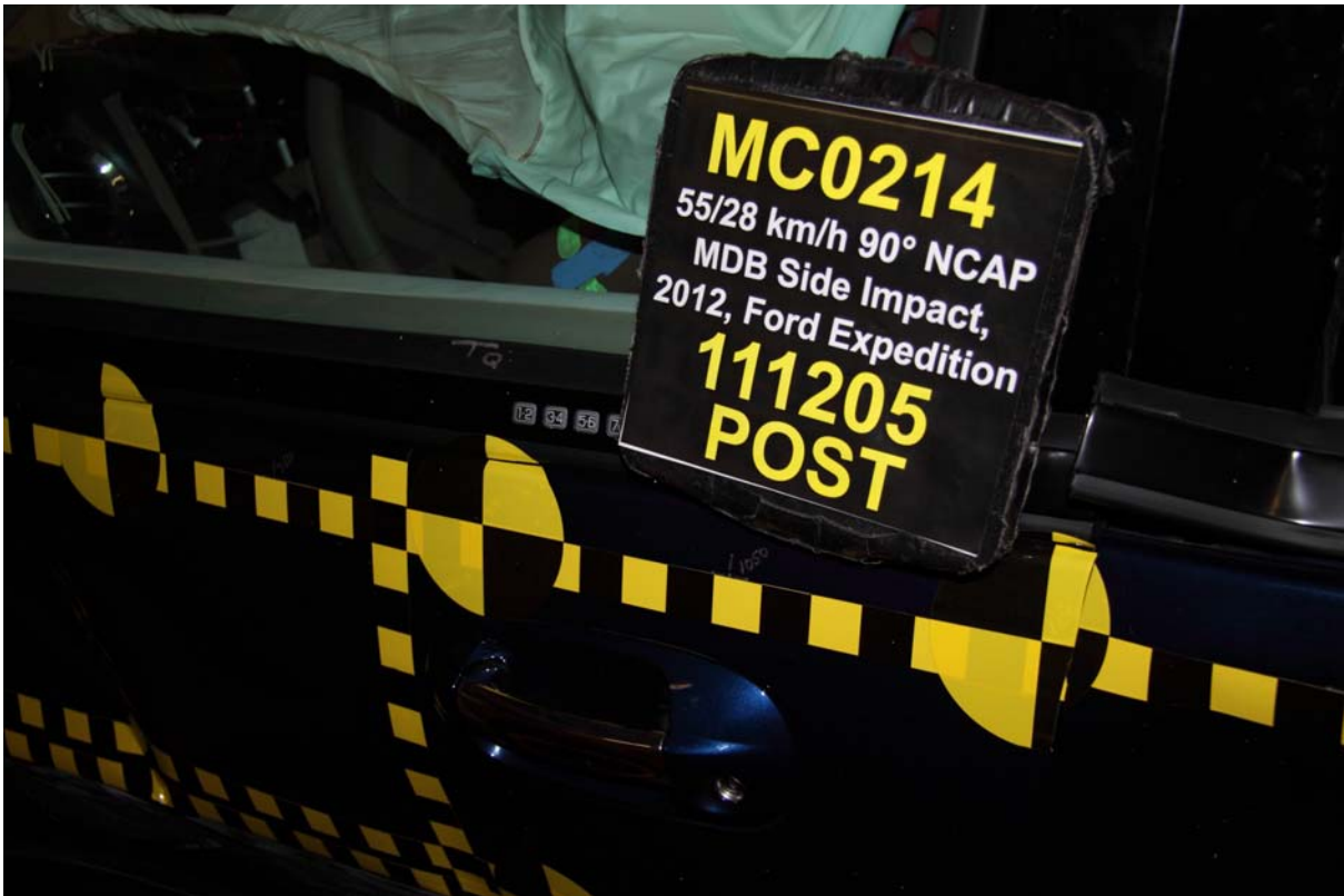
022 Post-Test Left Front Door Latch Close-up
