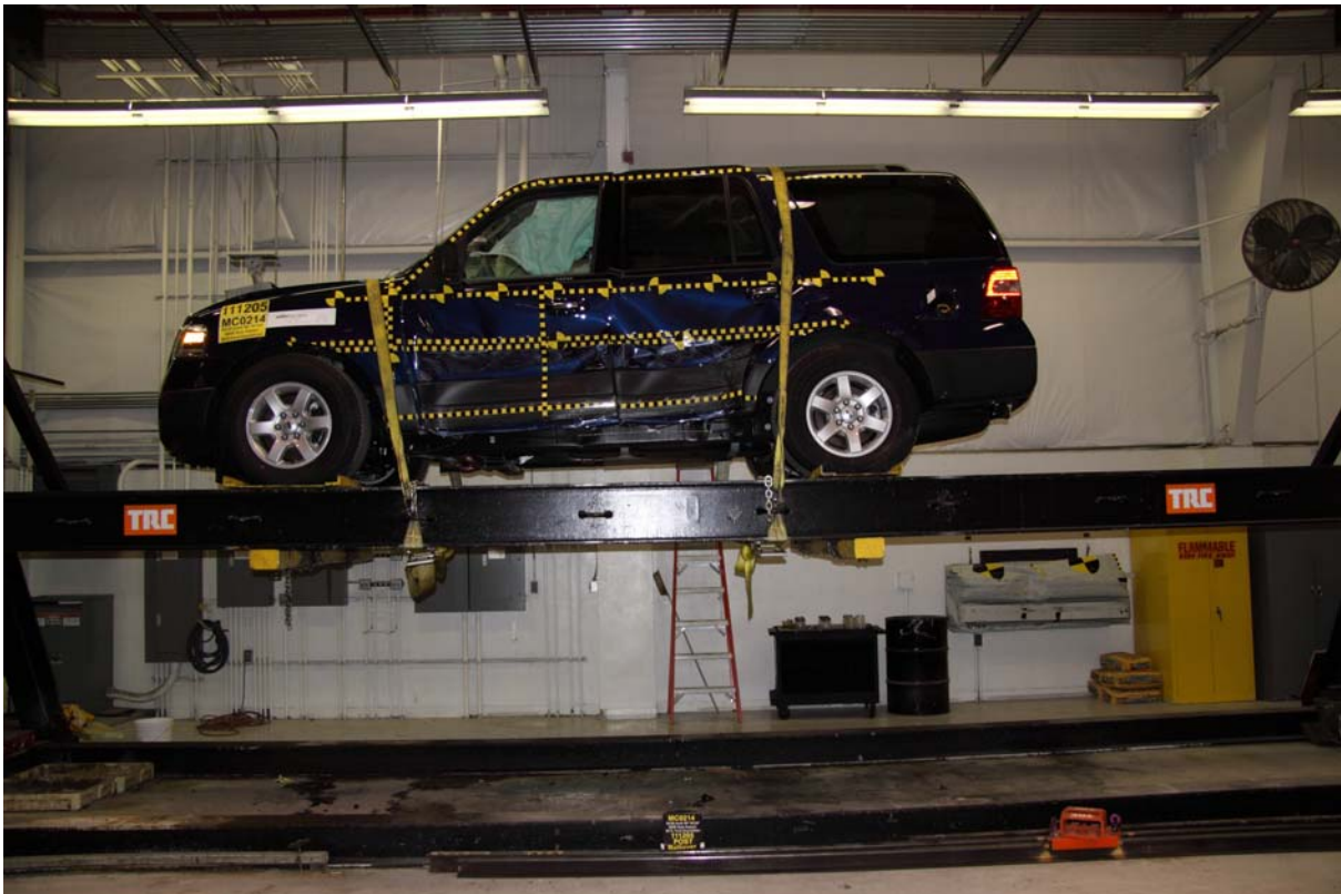
098 FMVSS No. 301 Static Rollover 360 Degrees
