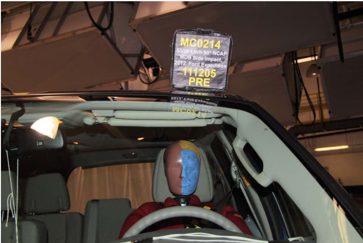
031 Pre-Test Frontal View of Driver Dummy Head and Shoulders in Relation to Head Restraint
