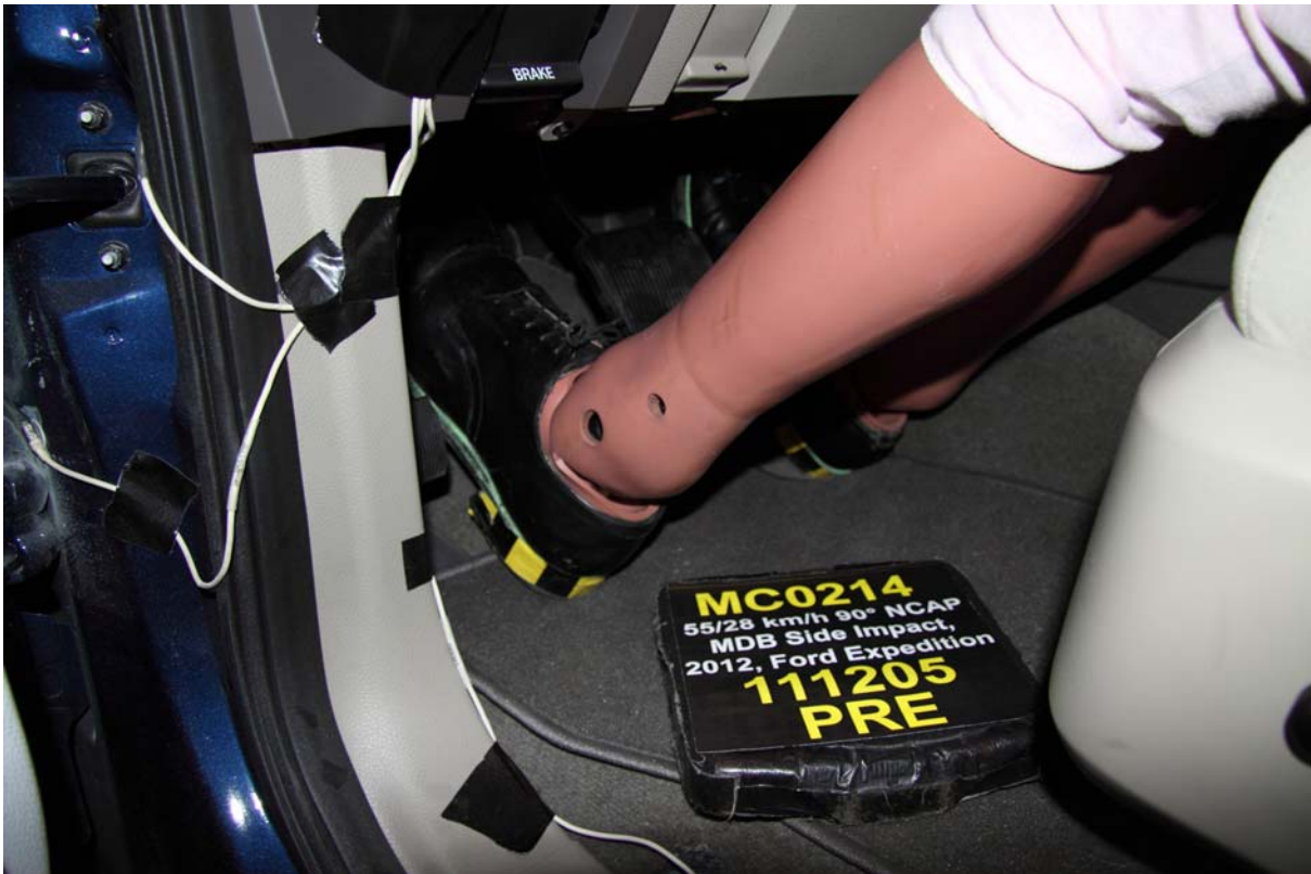
034 Pre-Test Placement of Driver Dummy Feet
