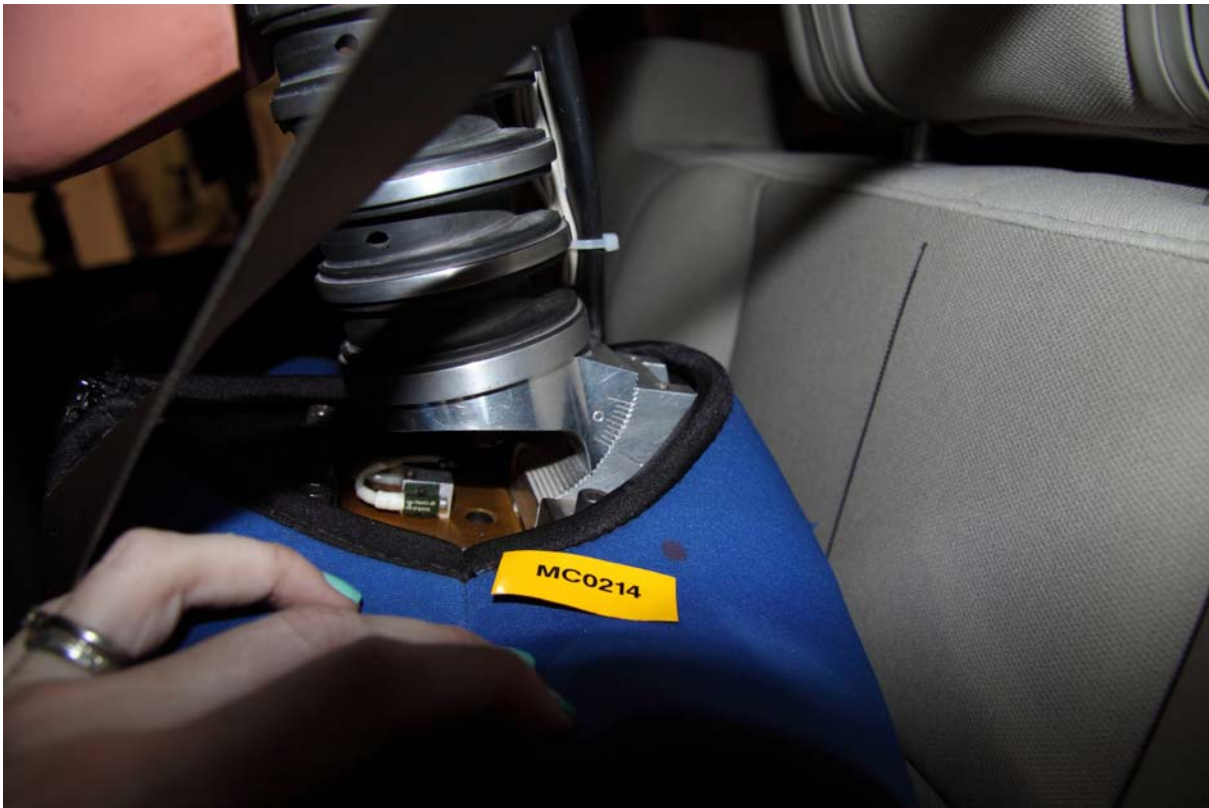
061 Pre-Test View of Rear Passenger Dummy Neck Showing Position of Adjustable Neck Bracket
