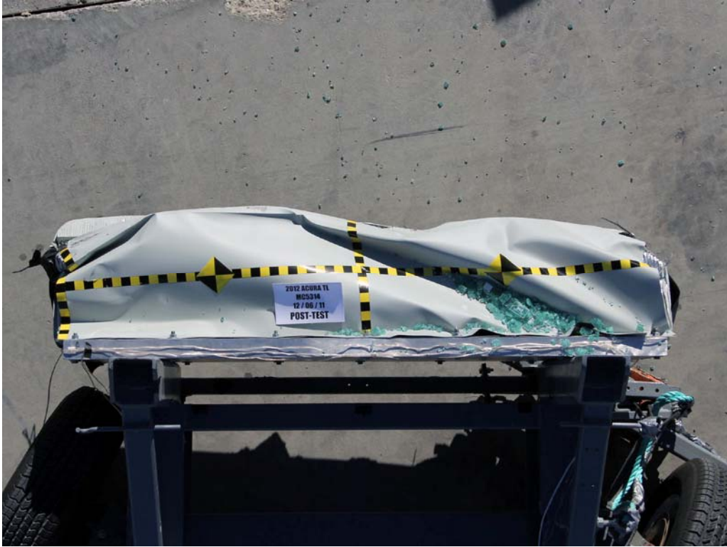
FIGURE 85. Post-Test Top View of MDB Impactor Face
