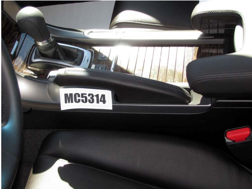
FIGURE 37. View of Disengaged Parking Brake
