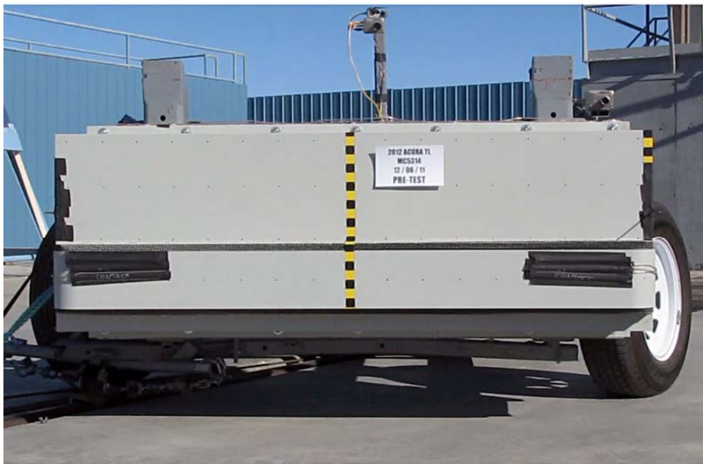
FIGURE 82. Pre-Test Front View of MDB Impactor Face
