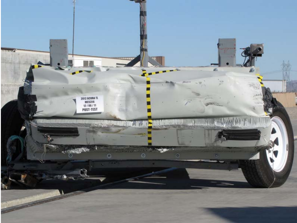
FIGURE 83. Post-Test Front View of MDB Impactor Face
