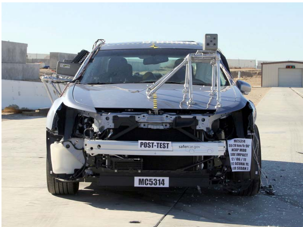
FIGURE 4. Post-Test Frontal View of Test Vehicle
