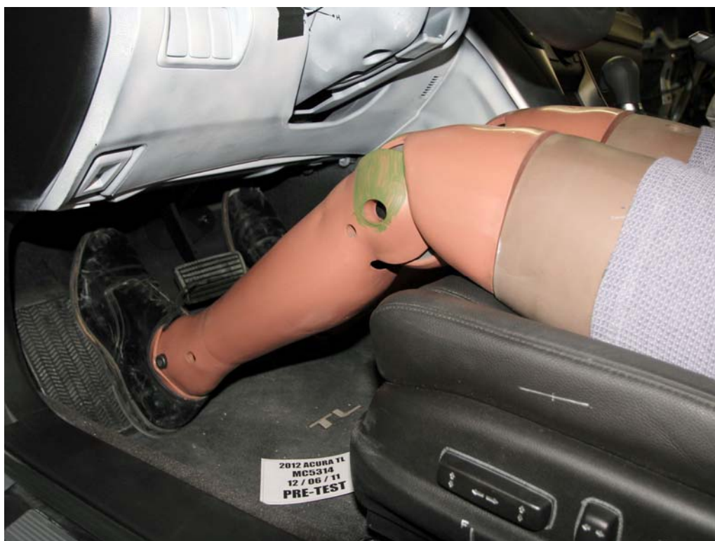
FIGURE 34. Pre-Test Placement of Driver Dummy's Feet
