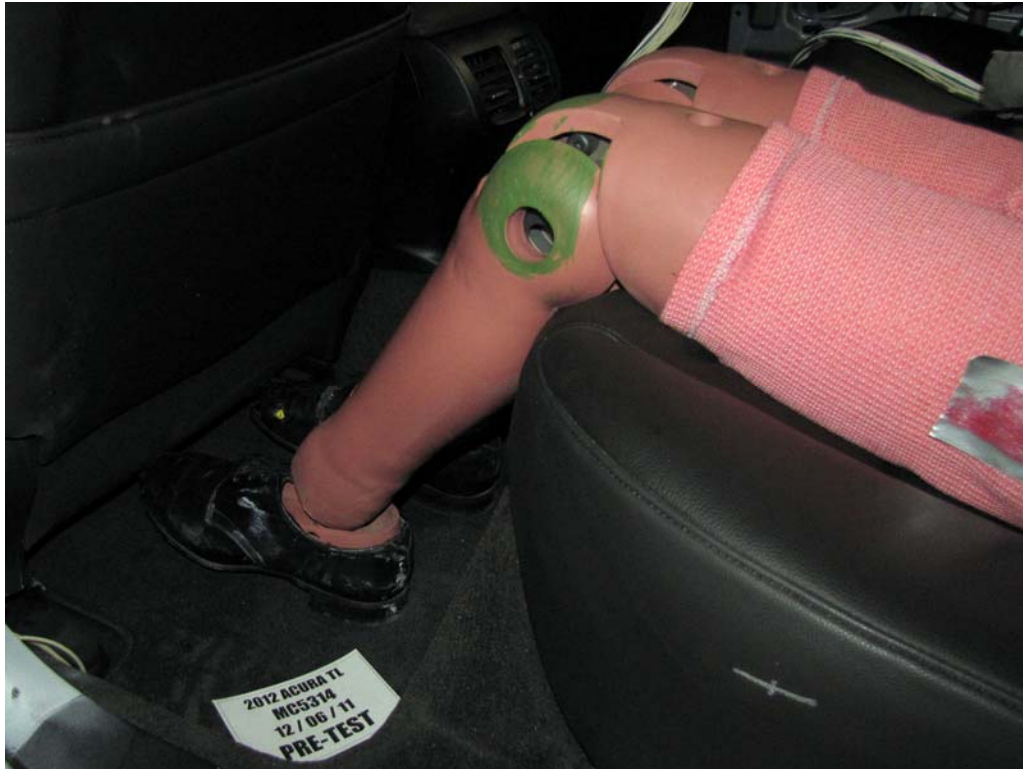
FIGURE 63. Pre-Test Placement of Rear Passenger Dummy's Feet
