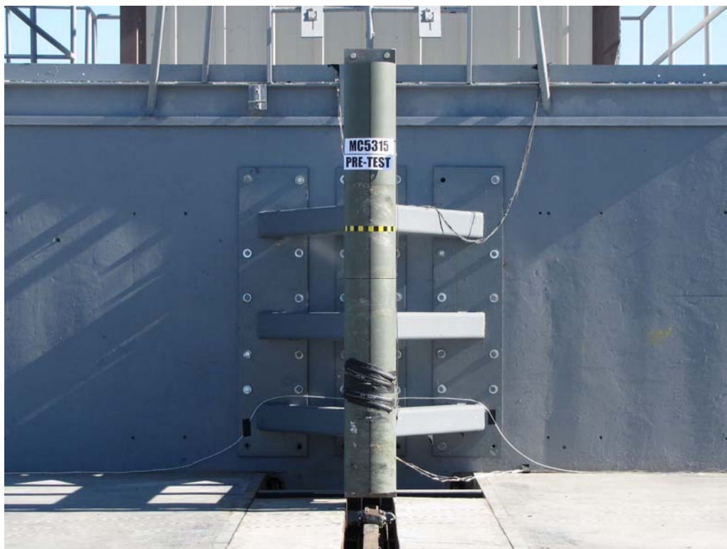
FIGURE 56. Pre-Test Pole Barrier Front View
