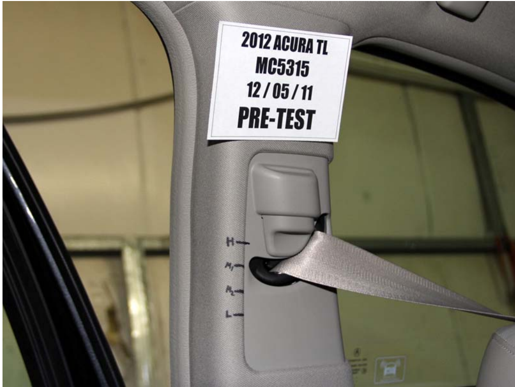
FIGURE 33. Pre-Test View of Belt Anchorage for Dummy
